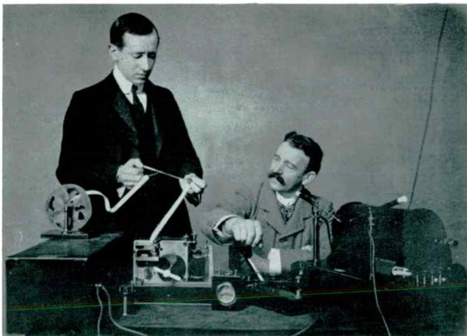
5 *Marconi and Kemp, about 1901, with apparatus including (right) the induction coil supplying high-voltage power for the transmitter and (centre left) the Morse inker recording the output of the coherer receiver*
