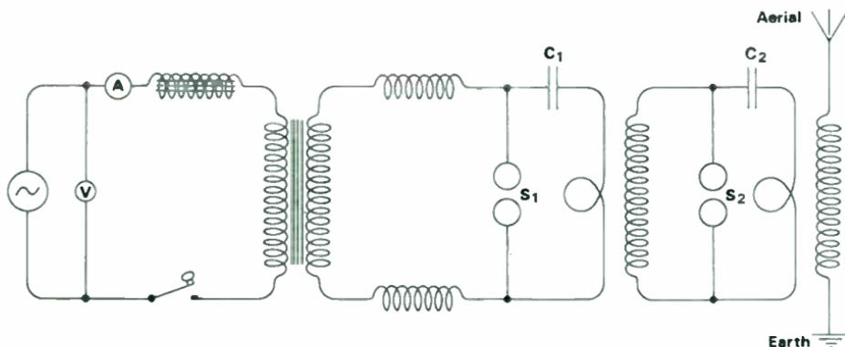
7 Circuit diagram of the transmitter used at Poldhu for the 1901 transatlantic experiments. The alternator charges the capacitor  $C_1$  through a circuit resonant at the alternator frequency. Spark-gap  $S_1$  then discharges  $C_1$  and charges  $C_2$ , through circuits resonant at an intermediate frequency. Finally,  $S_2$  discharges  $C_2$  through a circuit resonant at the radiated frequency, to which the aerial circuit is also tuned
