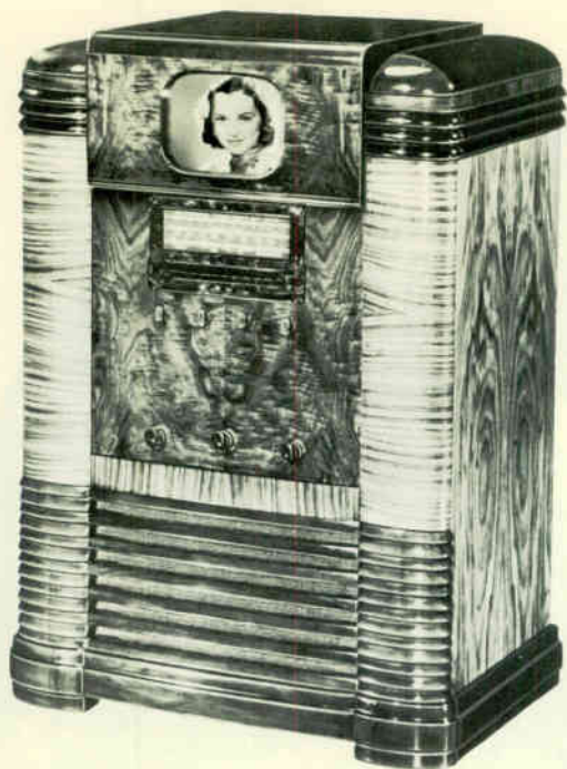
A 1939 RCA Victor television receiver. The 9-inch kinescope reproduced images 5\frac{1}{2} by 7\frac{1}{2} inches for direct viewing from the front of the cabinet.
