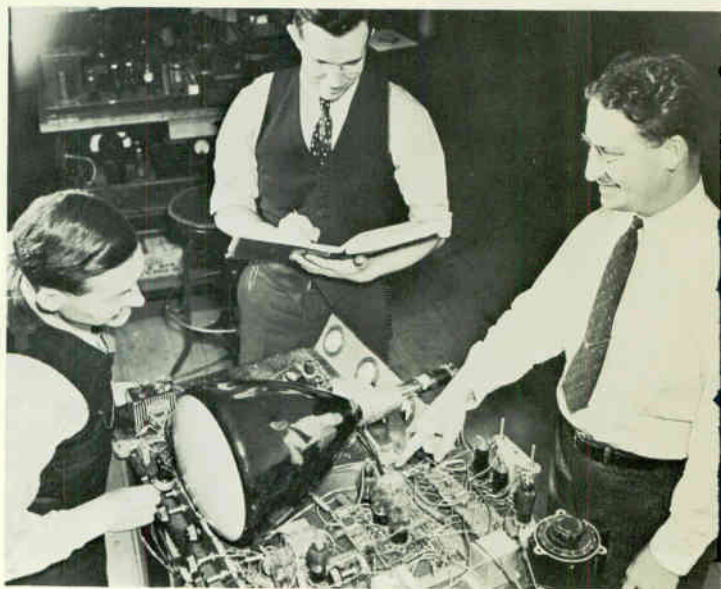
RCA engineers testing a 1939 black-and-white kinescope picture tube of the television receiver.
