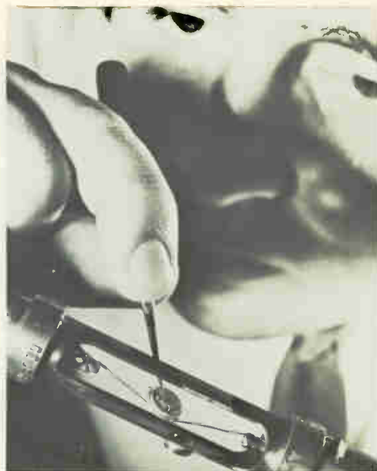
An RCA scientist points to an almost invisible speck of gallium arsenide hooked up to electric terminals. It functions as an FM radio transmitter.
