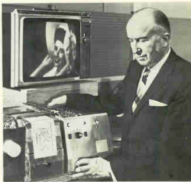
"Hitchhiking" on television, this RCA Experimental Home Facsimile System can deliver printed material in the home or office while a program is being viewed.
