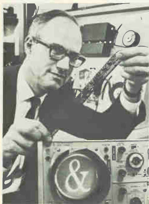
By linking computer and television techniques, an electronic type composition system can set text at 900 lines a minute.
