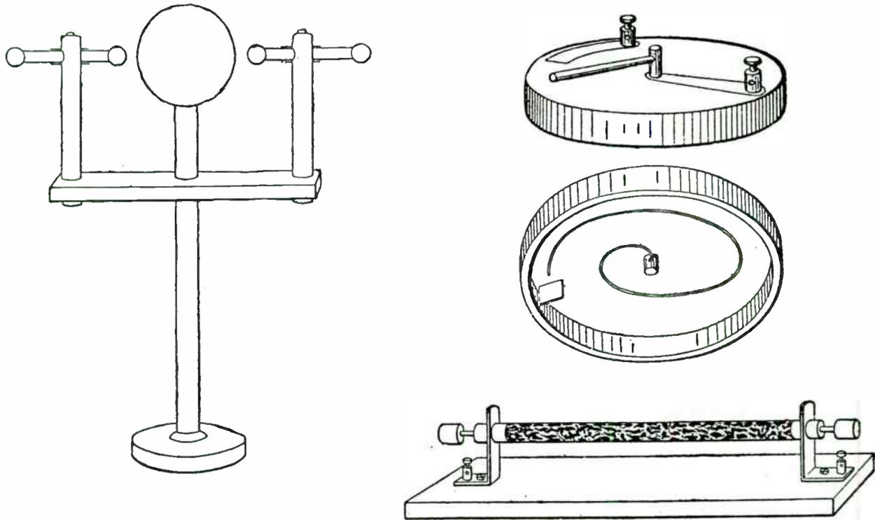
Fig 31. The Lodge spherical transmitter, borings tube, and spiral wire coherer.
