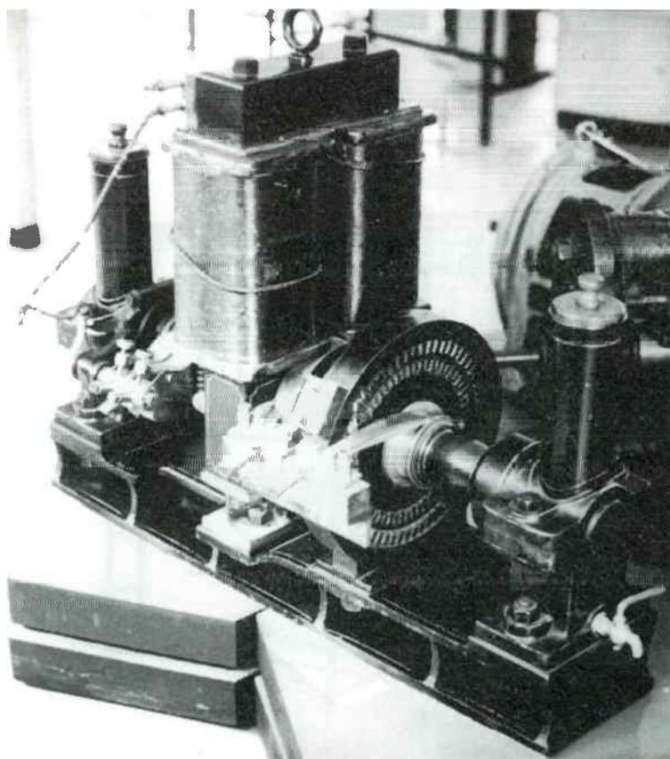
Fig 56. Lodge 3kHz alternator for high voltage generators.
