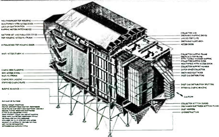
Fig 52. A 1923 advertisement showing the world's first blast furnace precipitator constructed at Skinningrove during WW1; a cut-away diagram of a modern Lodge-Cottrell installation.
