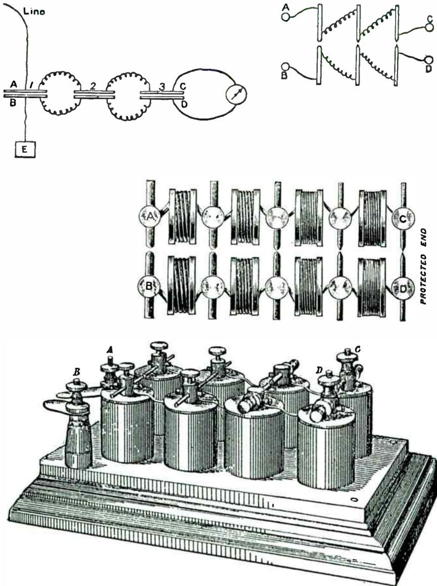
Fig 38. Diagrams of lightning guards for telegraphic instruments; Muirhead guard.
