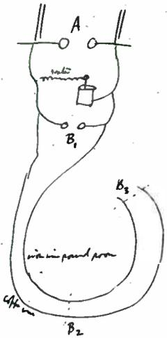
Putty the discharge at either B<sub>1</sub>, or B<sub>2</sub> or B<sub>3</sub>
