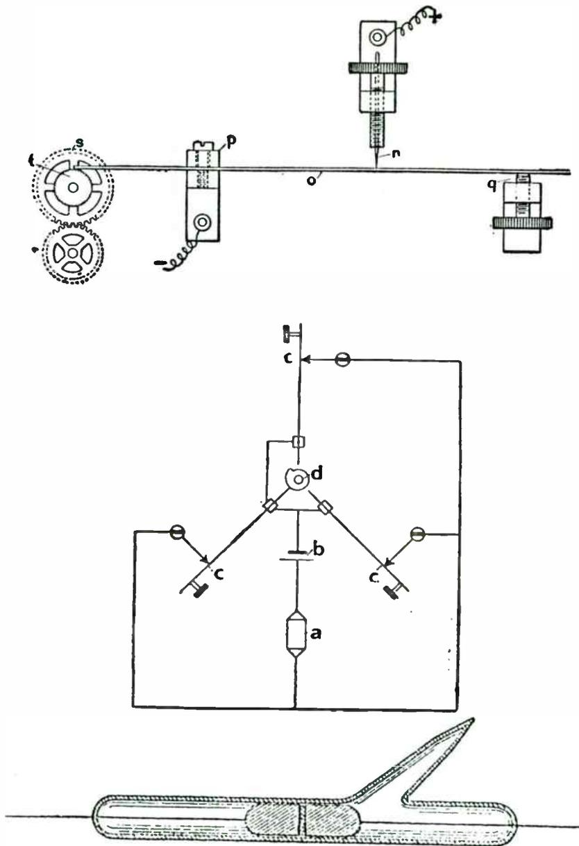
Fig 32. Lodge's single point spring coherer with clockwork decoherer and the Marconi coherer.
