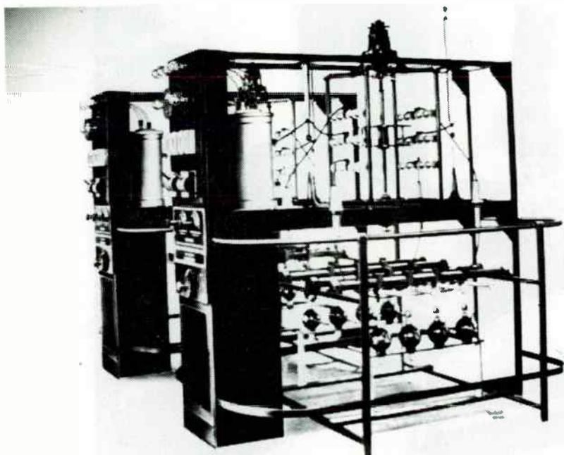
Fig 55. Power supply for agricultural electricity c 1906, using a bank of Lodge rectifier valves.
