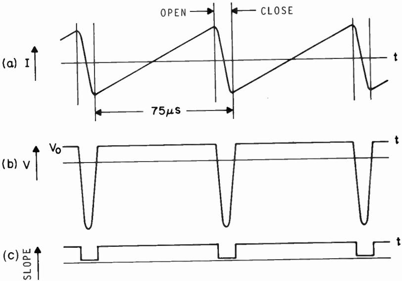
7.5 Fig. 1 — Sawtooth-current horizontal scanning.
