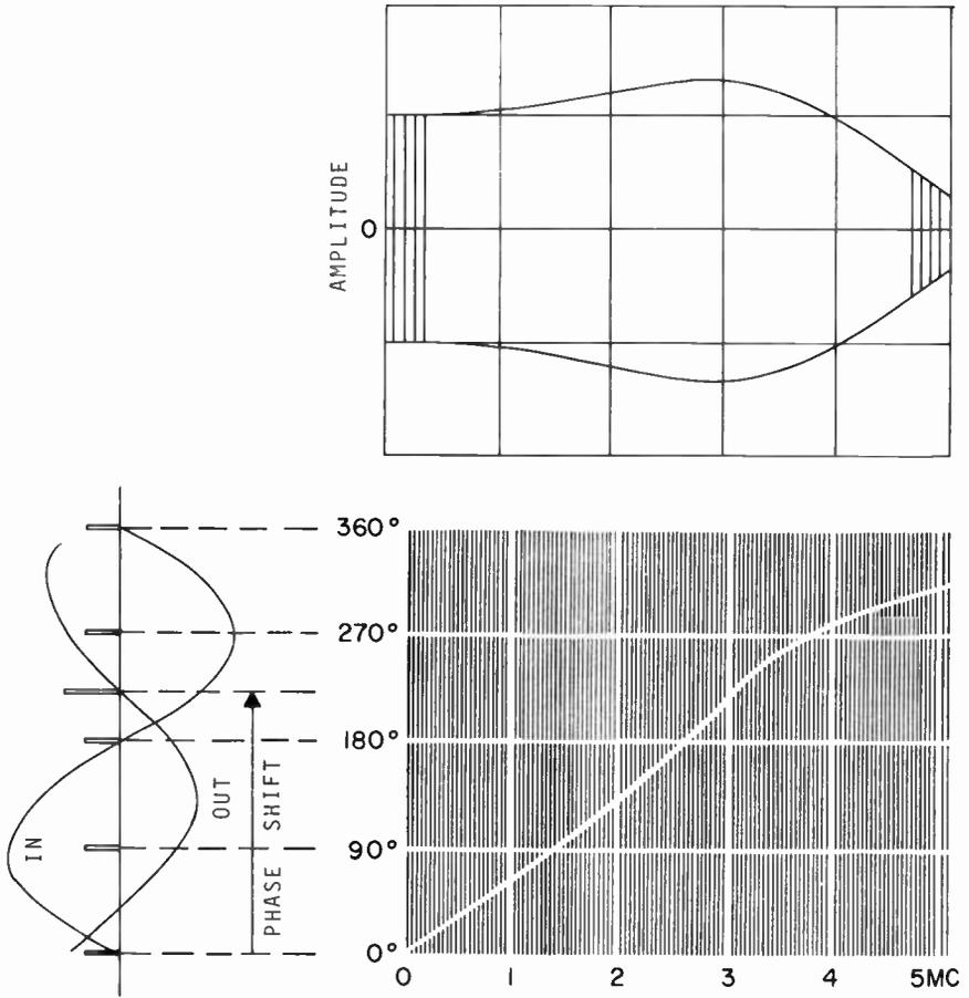
9.12 Fig. 1 — The display on the phase-curve tracer.
