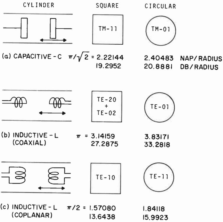
9.8 Fig. 1 — The principal types of piston attenuator.
