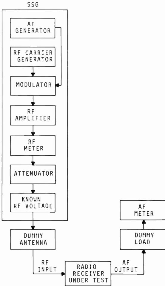
9.2 Fig. 1 — The equipment for testing a radio receiver.
