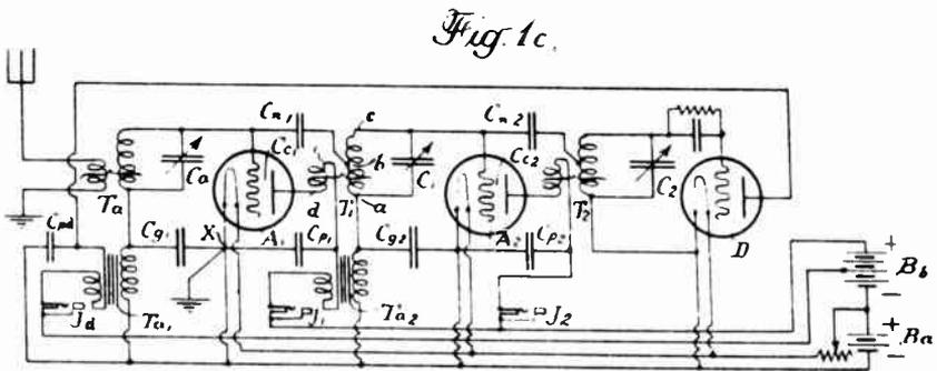
4.1 Fig. 7 — The original Neutrodyne receiver, as described in one patent [P6].
