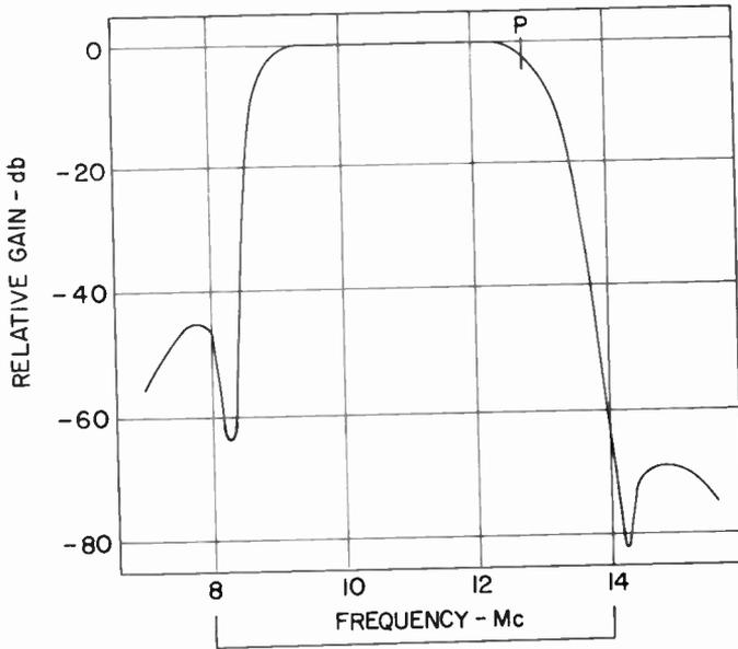
7.4 Fig. 7 — Picture IF wideband-amplifier response with sound IF traps.
