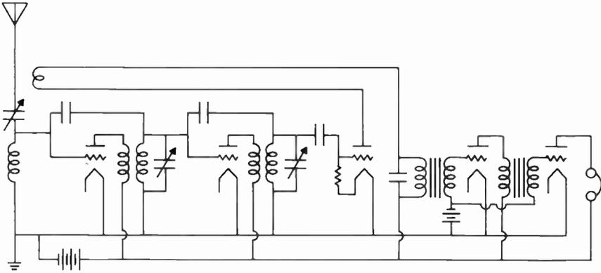
1.5 Fig. 1 — Proposed 5-tube receiver with neutralization (220817 HAW).
