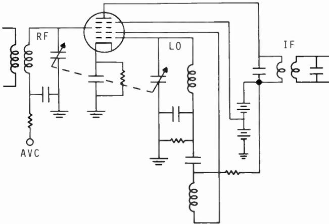
6.2 Fig. 3 — The hexode converter circuit.
