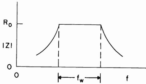
(a) The impedance of a dead-end filter.
