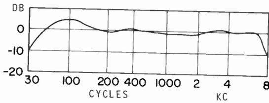
9.9 Fig. 1 — A record of acoustic response from a loudspeaker in the corner of a living room (average of three locations).
