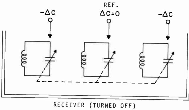
(b) Test of tracking error in unicontrol receiver.
