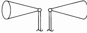
6.5 Fig. 2 — A conical dipole.
