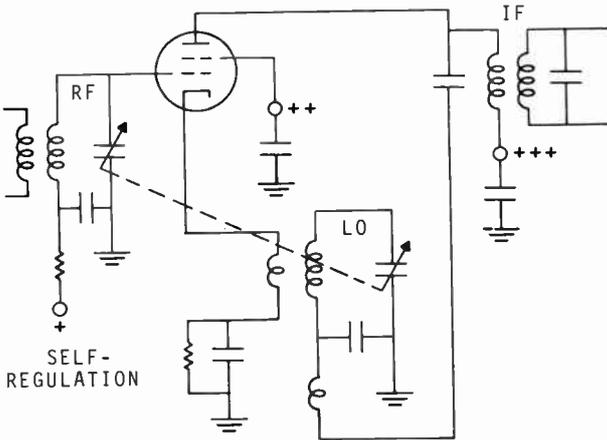
6.2 Fig. 1 — Converter with self-regulating oscillator.
