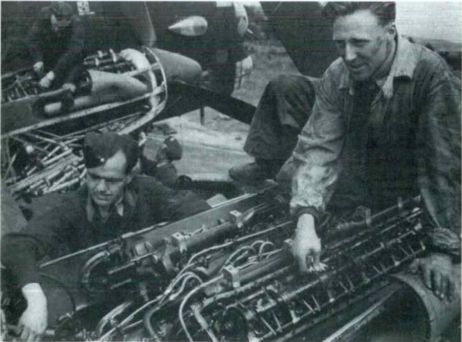
Figure 10.4 Tappets being adjusted on the starboard outer engine of a Halifax Mk.2 in the summer of 1942.
