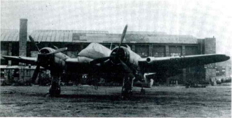
Figure 8.12 Bristol Beaufighter with AI Mk.IV aerials fitted to the nose of the aircraft and on the leading edge of the wings. (*Courtesy of EMI*)
