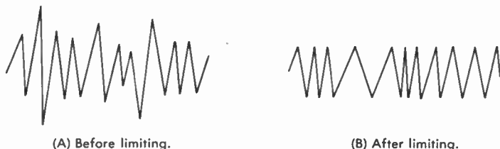
Fig. 11-3. FM signal before and after limiting.
