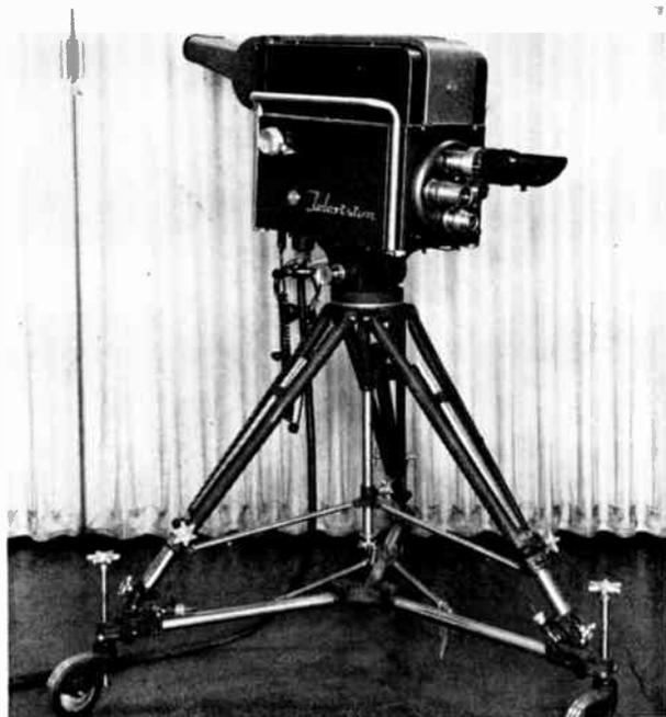
FIGURE 13. RCA Camera, TK-11A
