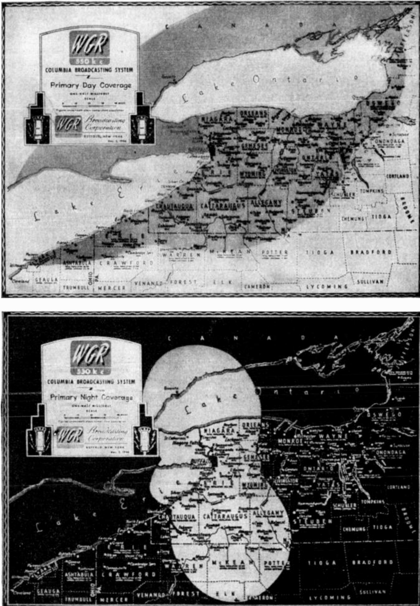
FIG. 15. Note the difference between the daytime coverage pattern of Radio Station WGR, Buffalo (when a nondirectional antenna is used) and the nighttime coverage pattern (when a directional antenna is used). Both the above maps are based on field-intensity measurement studies. (WGR.)
