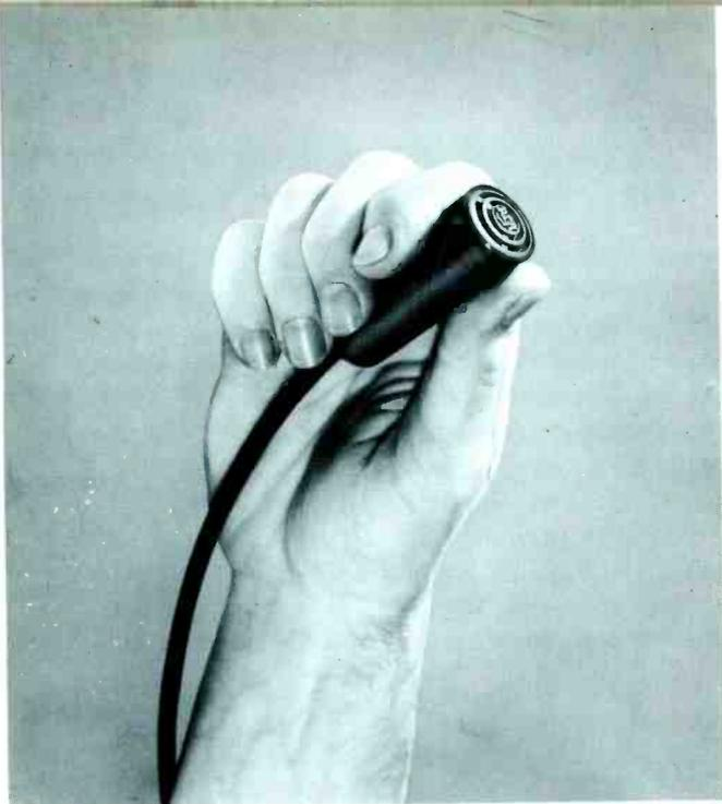
The RCA BK-6A, a miniature dynamic (pressure) microphone. This is used extensively in television as a necktie or lavalier microphone. (Courtesy RCA)
