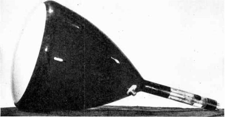
FIG. 7.—A type of Kinescope used in a television receiver of 1939.
