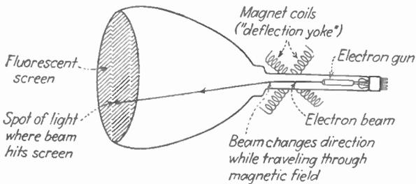
FIG. 8.—The principal parts of a Kinescope.
