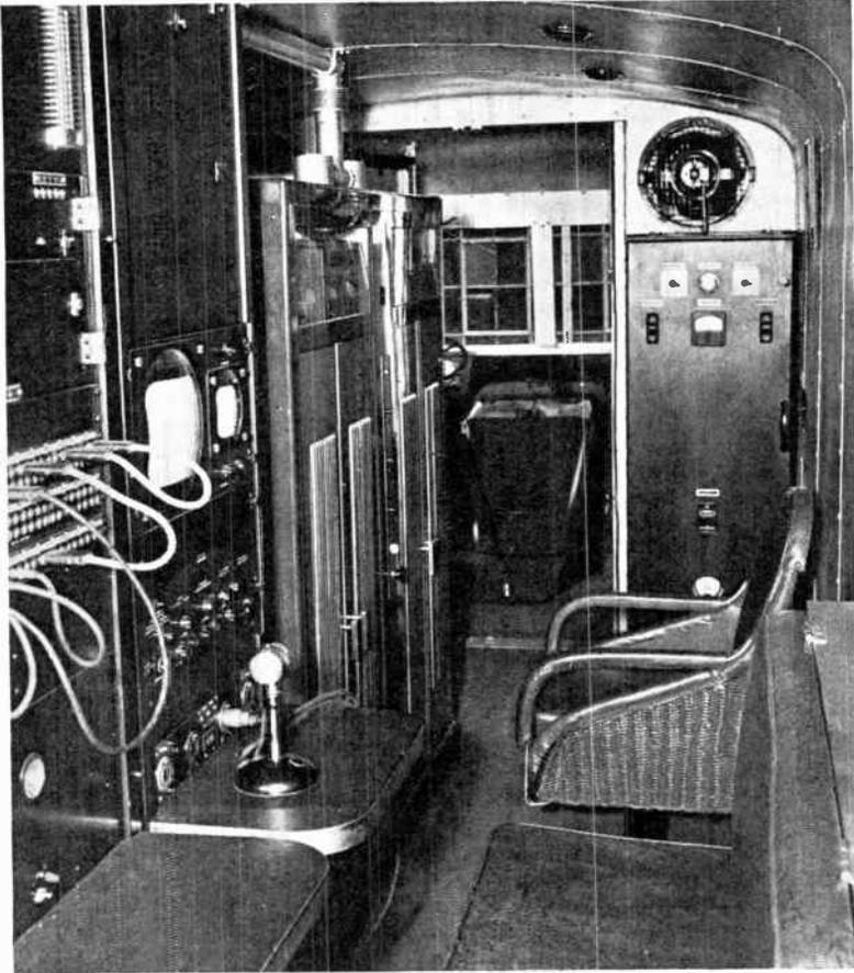
FIG. 46.—The control position in the radio transmitter truck.
