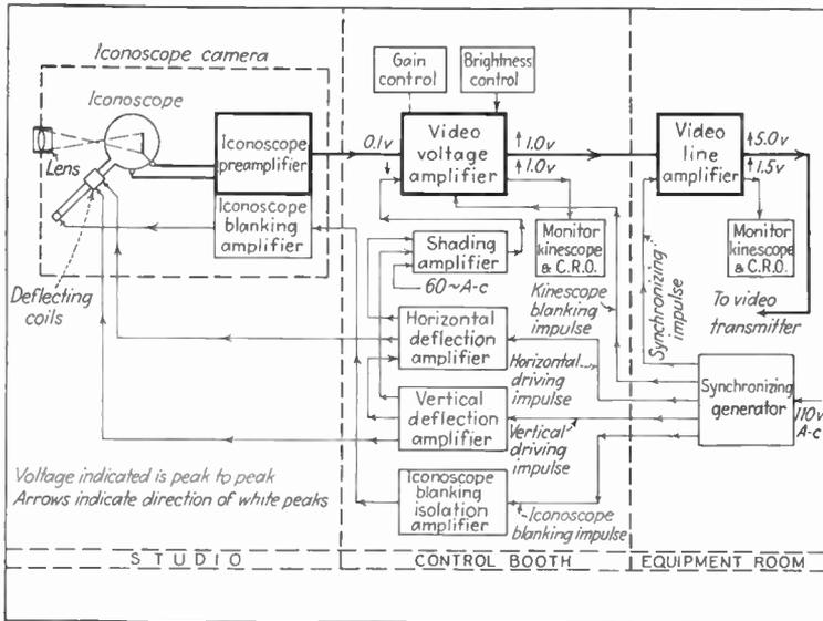
FIG. 67.—A typical one-channel television system.
