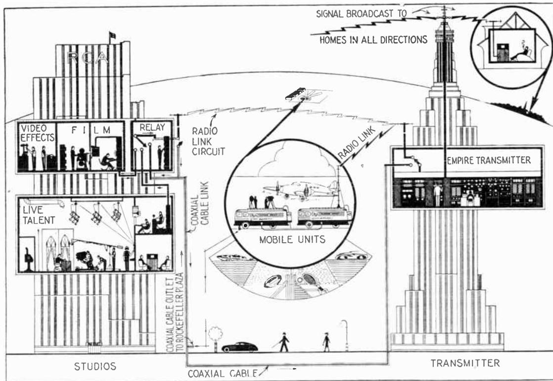
FIG. 20.—The three sources of program origination; live talent, film, and outside pickups; and the methods used to relay the television signal to the main transmitter at the Empire State tower for rebroadcast to viewers in the New York area.
