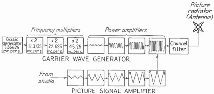
FIG. 69.—Diagram of frequency generation at the transmitter.
