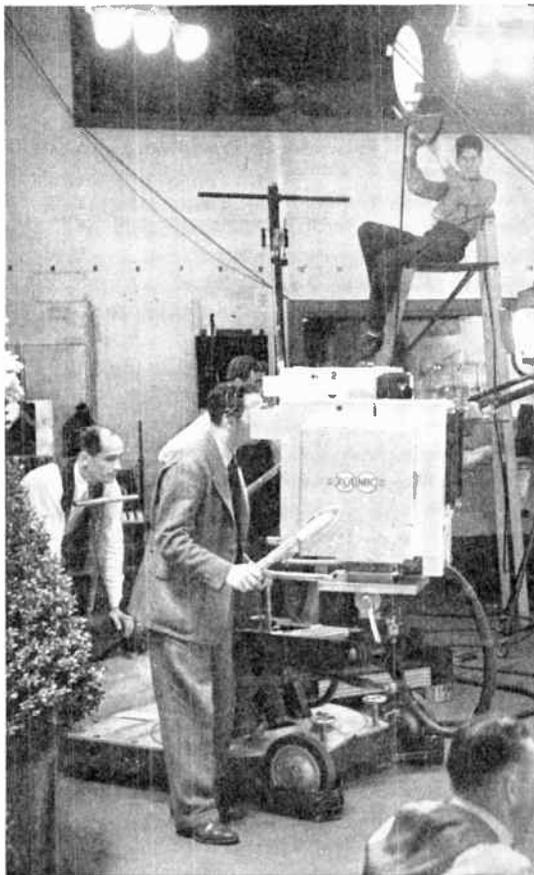
FIG. 26.—A “dolly” television camera. This camera is used for “moving shots”—such as moving in from a “long shot” of a person to a head-and-shoulders close-up. The camera operator can ride along with the camera, concentrating all his attention on the composition and focus of the picture, while being pushed by a second person.
