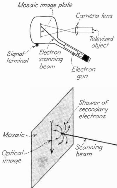
FIG. 63.—The essentials of the Iconoscope. Also, the existence of secondary electrons is shown diagrammatically.
