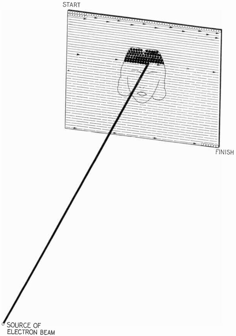
FIG. 6.—Process of scanning: Picture is analyzed point by point in a definite sequence, the amount of light associated with each point registering a corresponding influence on the transmitted radio signal. At the receiver, the process is virtually reversed.
