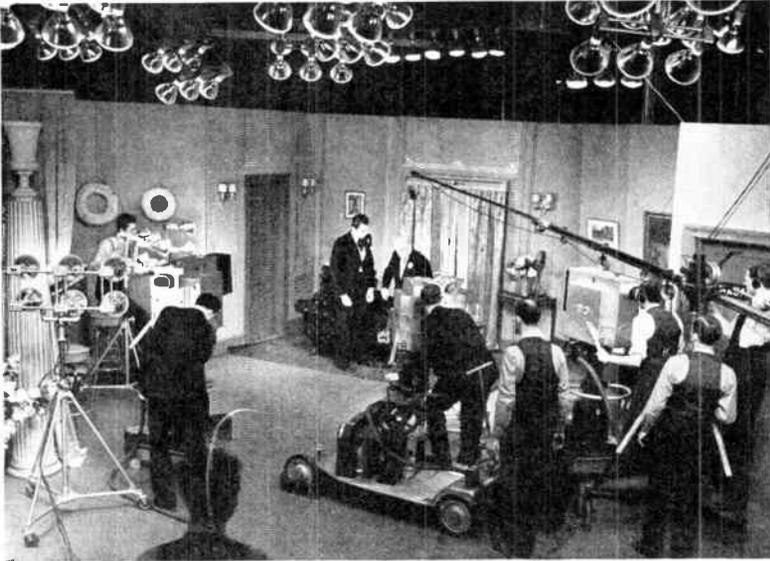
FIG. 15.—The live-talent studio during an actual broadcast showing the cameras, microphone boom, and technical personnel in action.
