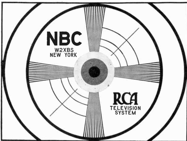
FIG. 68a.—The NBC-RCA standard test chart.
