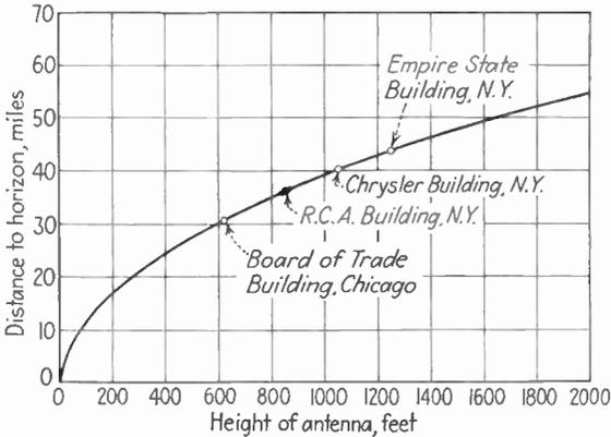
FIG. 71.—Horizon distances for given antenna heights.
