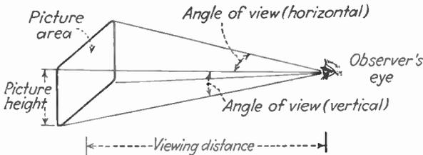
FIG. 62.—The factors considered in connection with viewing angles.
