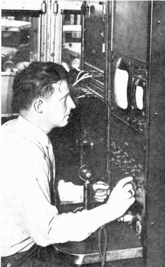
FIG. 49.—A monitoring position in the picture-bus truck. This is a piece of equipment similar to that described previously in connection with the live-talent studio equipment.
