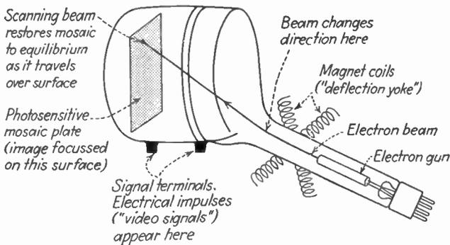
FIG. 5.—The essential parts of an Iconoscope.
