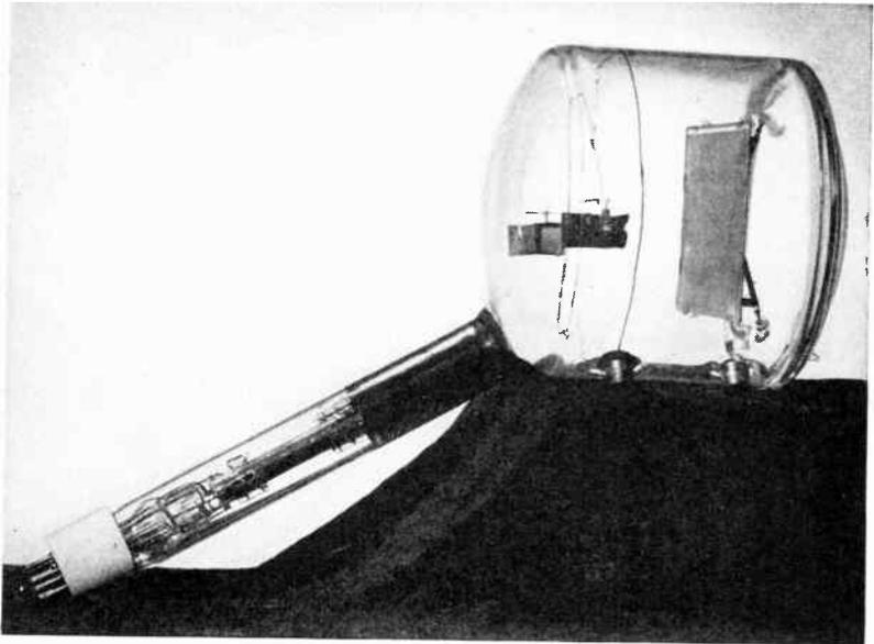
FIG. 4.—An Iconoscope of the type used in television cameras during 1938.
