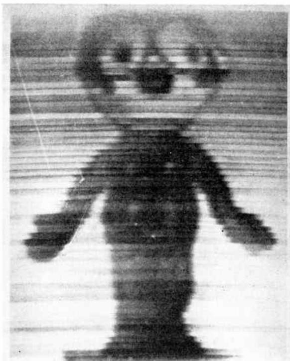
FIG. 3a.—Comparison between 60-line mechanical scanning on the left and modern 441-line scanning on the right. See Fig. 3b opposite.
