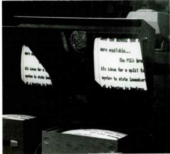
the TelePrompter consist of a mirror that is angled over the camera lens. A special camera takes an image of the news copy, and that image is projected onto the mirror. The newscaster or other performer can see the script, but it does not interfere with the camera's view.
