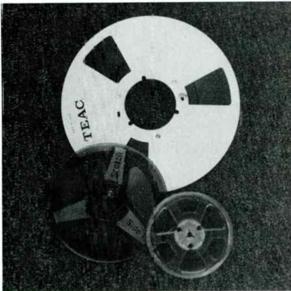
Figure 5.7. (above left) Tape reels come in various sizes; the most common are 5 inch, 7 inch, and 10<sup>1</sup>/<sub>2</sub> inch.
