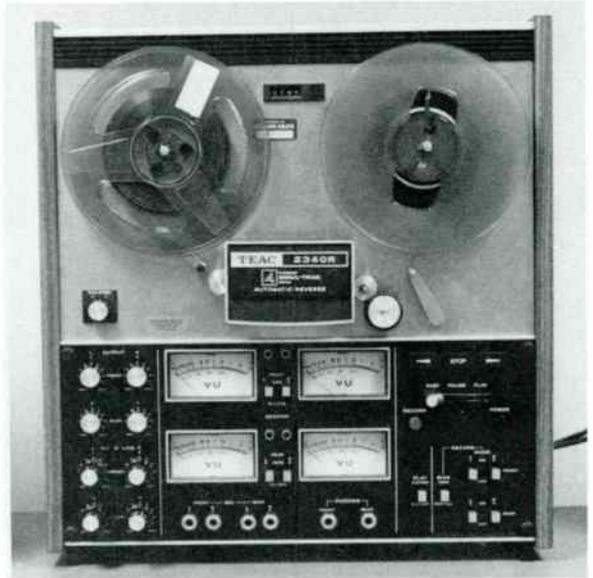
Figure 5.8. (above right) A broadcast-quality tape recorder.
