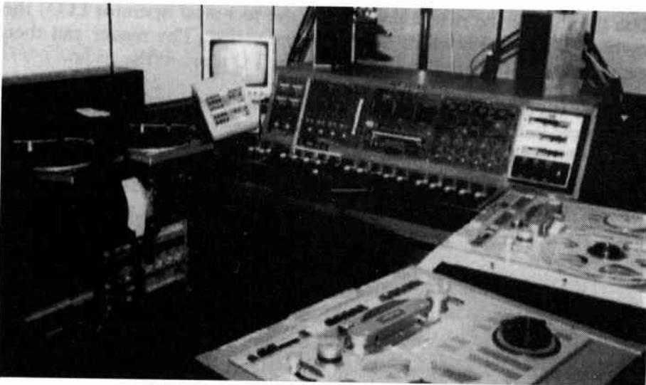
**Figure 57** (above) BBC Mark 3 control desk with grams and tape decks at BBC Radio Bedfordshire. (right) The on-air studio at Chiltern Radio, a British station in the independent radio network. The control desk is simpler and less cluttered than that used by the BBC. Commercials are kept on scores of cartridges – six are lined up in the machine (left) ready to go (Andrew Boyd)
