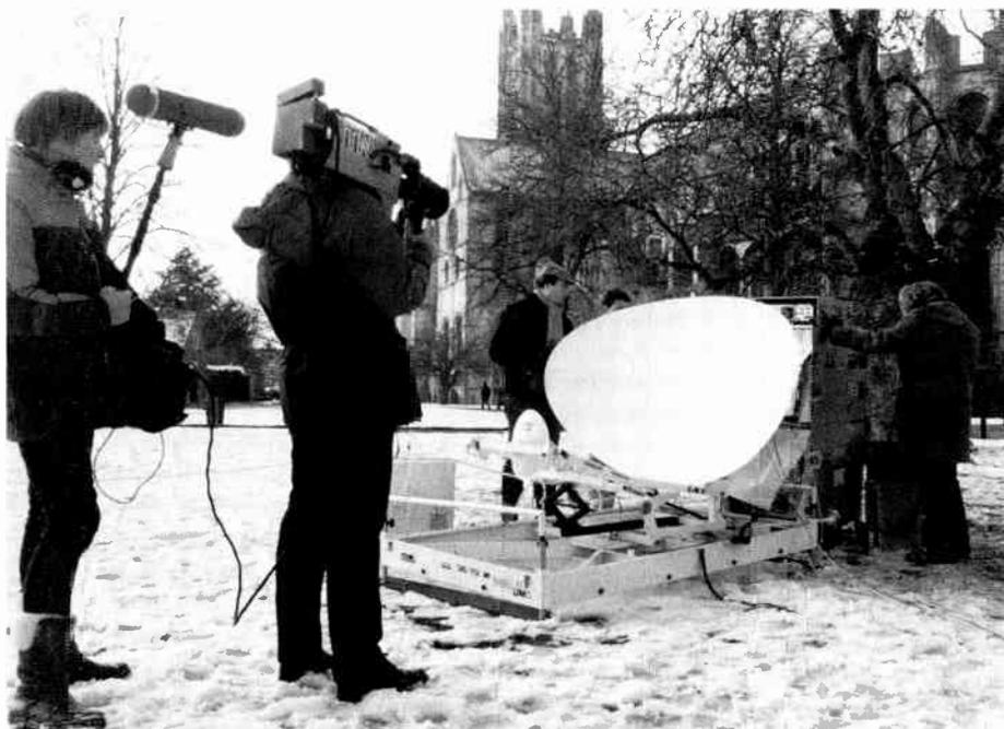
**Figure 82** Portable ground-stations are used to beam news reports into space, where they are bounced off satellites and relayed to transmitters the other side of the world (courtesy ITN)
