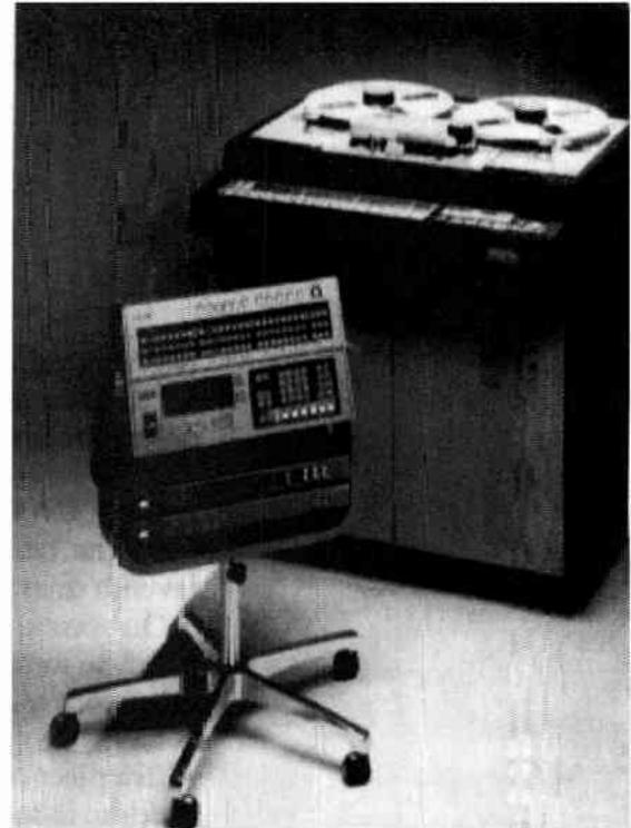
**Figure 53** (left) The Studer tape deck is the standard workhorse in many British radio stations. It features a counter for timing tapes and a built-in editing block for manual cutting and splicing. This machine is stereo (courtesy FWO Bauch Ltd, Studer Agents) (right) Digital technology is fast taking over in the studio, offering superior reproduction, computerized tape-handling and a sound quality that will not deteriorate over generations of recording (courtesy of Sony Broadcast Ltd)
