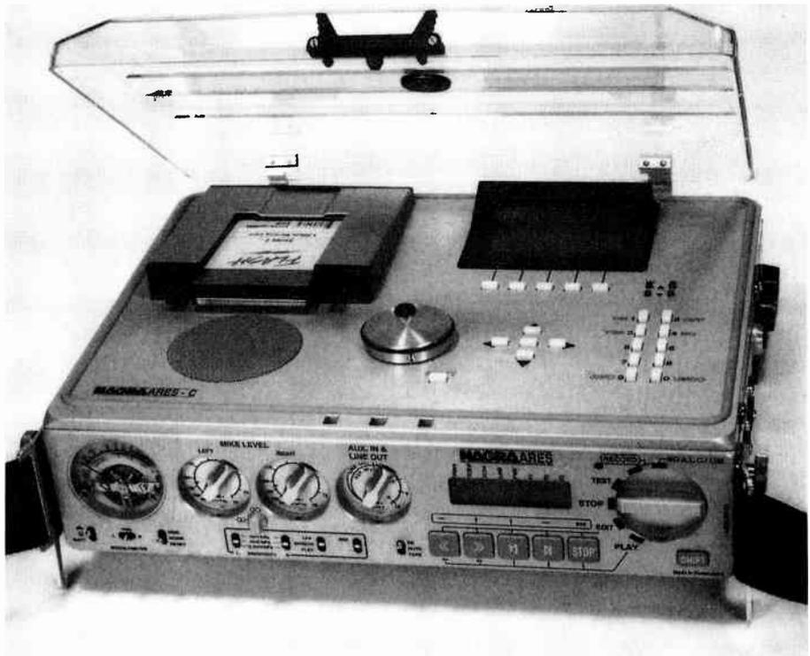
**Figure 54** Recording goes solid-state. The *Nagra ARES-C* uses credit card sized PCMCI cards to store up to 40 minutes of sound. Recordings can be edited on the machine and downloaded directly on to a computer (courtesy Kudelski)
