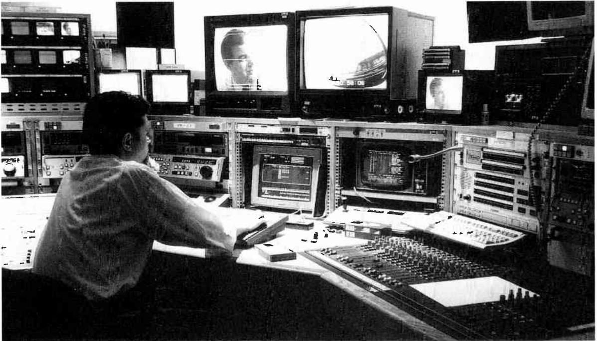
**Figure 74** Inside the production suite at ITN. Computer-controlled editing lays down pictures, soundtrack and graphics directly on to the Betacam cassette (Andrew Boyd)
