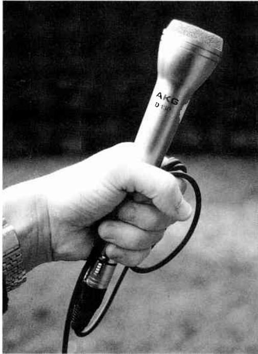
**Figure 55** Mike handling. Take up the slack on the cable, being careful not to pull at either of the connections, and grip the mike lightly (Andrew Boyd)
