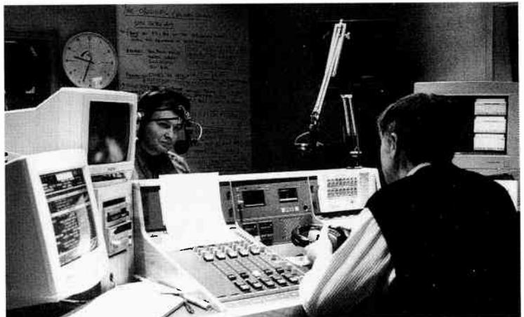
Standard equipment will include a control desk; two or more compact disc players (or record decks); cassette and DAT machines; large monitor loudspeakers; telephone and mini-switchboard system; talkback (a form of intercom); presenter and guest mikes; studio clock with on-air lights and some device for playing audio clips and jingles.
