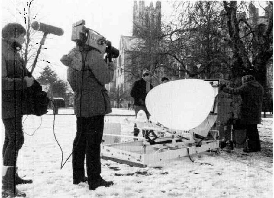
**Figure 83** Portable ground-stations are used to beam news reports into space, where they are bounced off satellites and relayed to transmitters the other side of the world (courtesy ITN)
