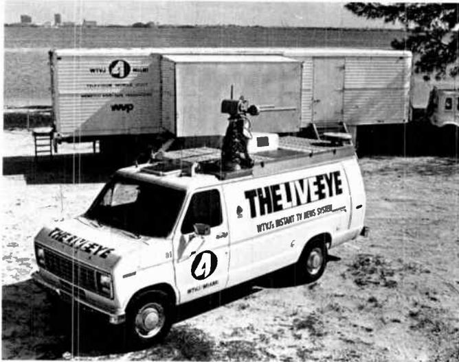
*A. The unwieldy remote vehicle in the background contrasts with the compact, lightweight ENG (electronic news-gathering) van in the foreground. The machine-gun-like object on top of the van is an antenna for relaying pictures to the studio by means of microwaves.*
