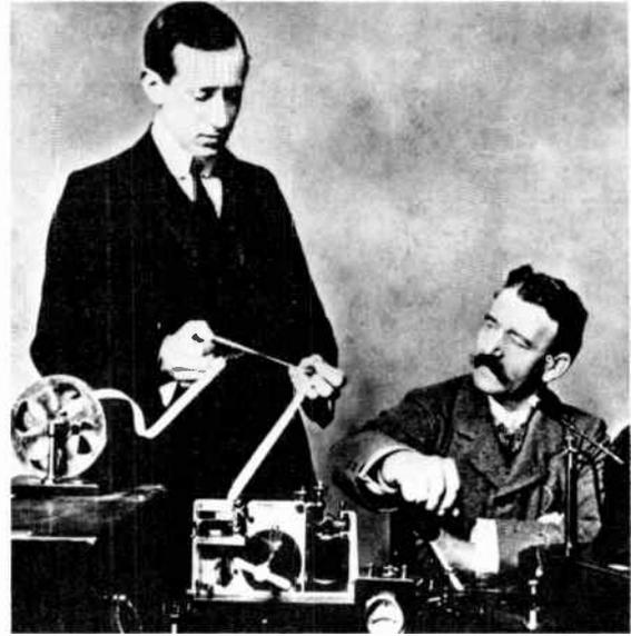
*In a 1902 photo, the inventor examines the paper tape on which a radiotelegraphic message is inscribed in Morse code. At that time radio equipment was still very crude, but the already well-developed equipment of wire telegraphy was readily adaptable to the task of recording wireless messages. Seated: George Kemp, Marconi's most trusted engineering assistant.*
