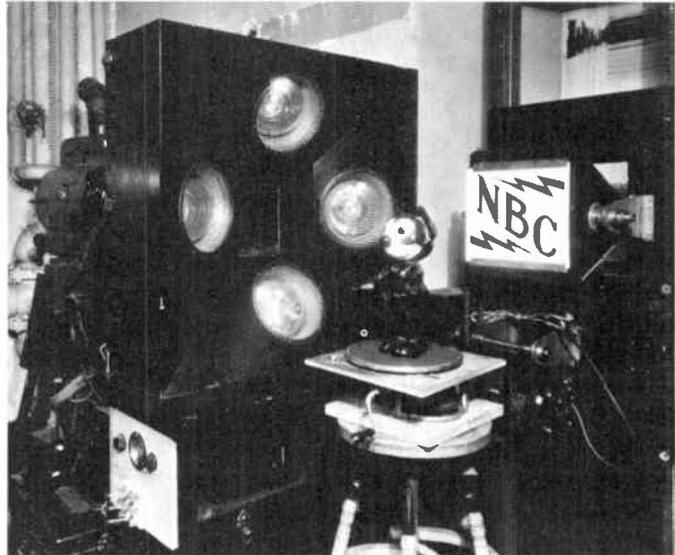
*A 12-inch model of Felix the Cat (a popular cartoon movie character of the 1920s), posed on a revolving turntable, was used at the RCA laboratories as a moving subject to televise during the development of electronic television. The image at left shows how Felix looked on television in 1929 when picture definition was still only 60 lines per frame.*
