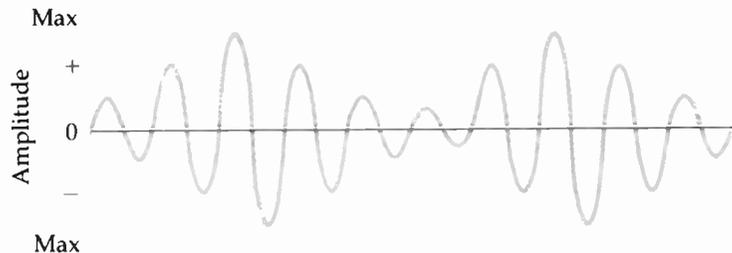
But a frequency-modulated carrier has constant amplitude, with frequency changes conveying the signal pattern:
