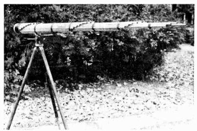
Fig. 11.—Machine-gun attachment for dynamic microphone (very directional).
