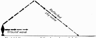
At night the coverage of the clear channel stations is extended by the reflected sky-wave
