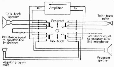
Fig. 45.—Diagram of talk-back wiring.
