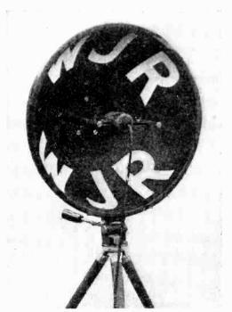
Fig. 12.—Improvised parabolic microphone.
