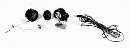
Fig. 46.—Inexpensively constructed talk-back microphone.
