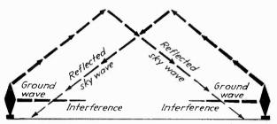
At night the coverage of local and regional channel stations is reduced because their reflected sky-waves produce interference with each others ground-waves
