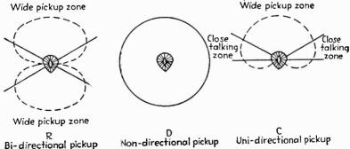
Fig. 9.—Cardioid directional microphone.
