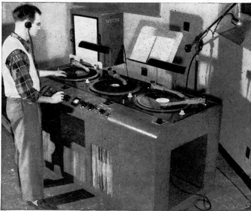
FIG. 39. Sound table. Four pickup heads, three turntables, mixers, record racks in the front, speaker set into recess at the end of the sound table. (*University of Michigan.*)
