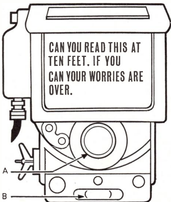
Announcer's view of the autocue, positioned just above the camera lens. As he reads, the announcer can give the impression of looking straight into the camera lens. A, camera lens. B, camera cue light.
