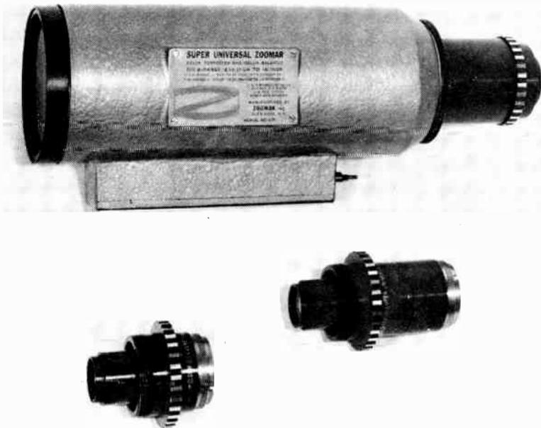
Fig. 5-12. Super Universal Zoomar with converters. Focal length of lens as shown above:  $2\frac{1}{2}$  to 16 inches ( $f/3.9$ ). With converter at lower left: 4 to 25 inches ( $f/5.6$ ). With converter at lower right:  $6\frac{1}{2}$  to 40 inches ( $f/8$ ).
