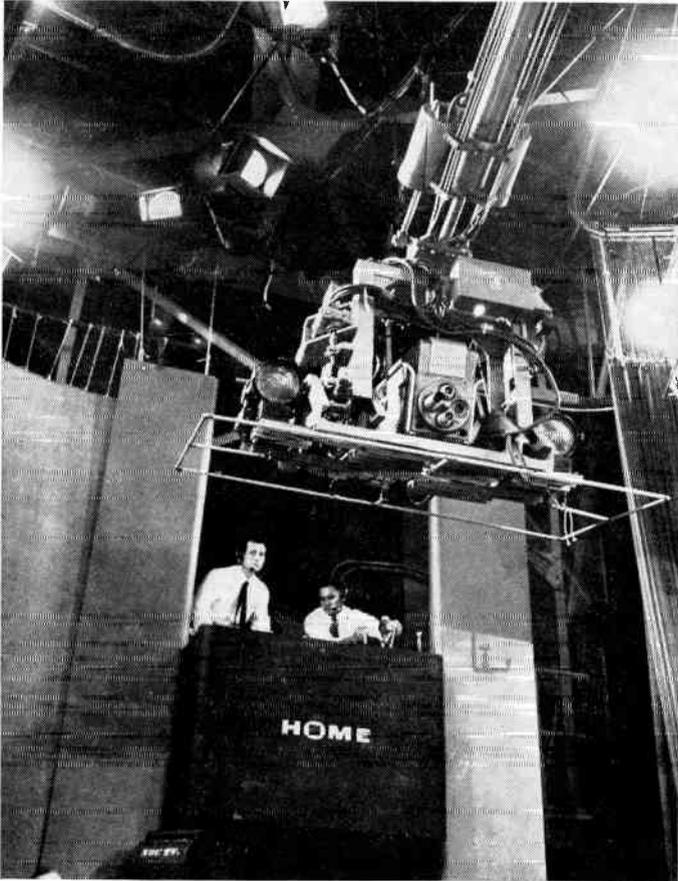
Fig. 4-26. Special remotely controlled pan, tilt, and crane apparatus used by NBC on the daily "Home" program. Camera operators watch view finder in control point overlooking the studio.
