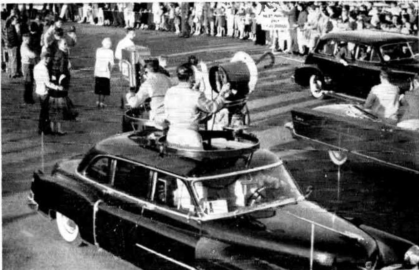
Fig. 20-37. Cadillac self-contained mobile unit used by NBC to cover a presidential arrival. Both camera and microwave transmitter are mounted on circular track and may be rolled around the periphery of each operating well to point in any direction.
