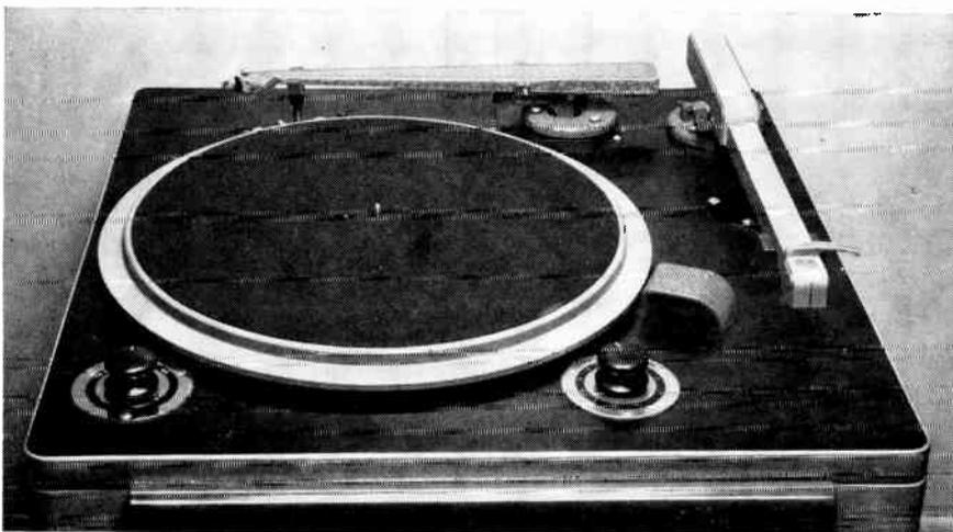
**Fig. 19-20.** Typical control-room turntable. Two pickup arms are included. The one at the back is a special lightweight arm for long-playing microgroove records. Left knob, speed selector; right knob, lateral or vertical cut selector.
