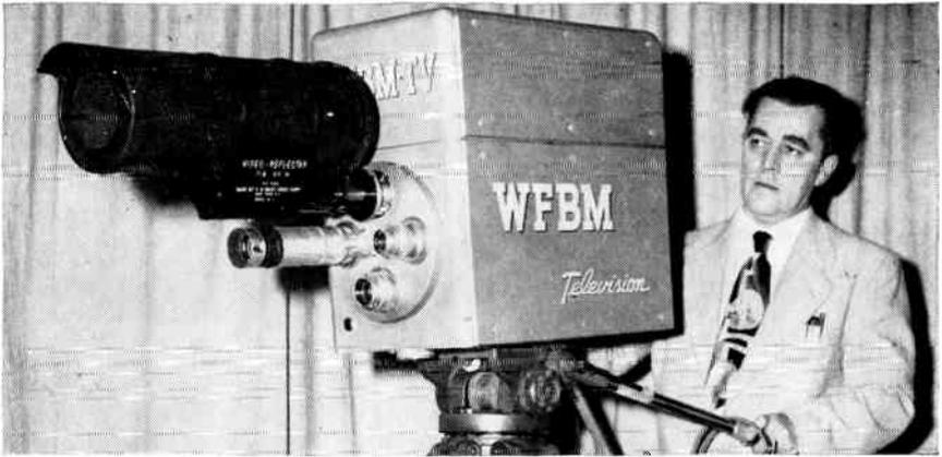
Fig. 5-4. Video Reflector lens in use.
