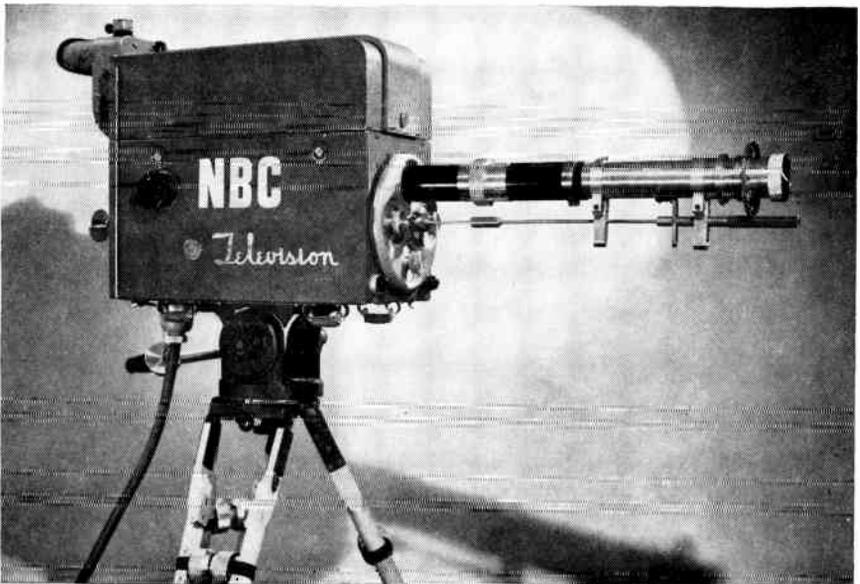
Fig. 5-9. The first model television Zoomar. Control handle is visible at rear of camera.
