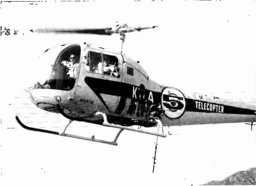
Fig. 20-20. KTLA Telecopter over Los Angeles. GE vidicon camera with Pan Cinor zoom lens and open frame view finder protrudes from cockpit window. Transmitter antenna, below, must be raised before landing.
