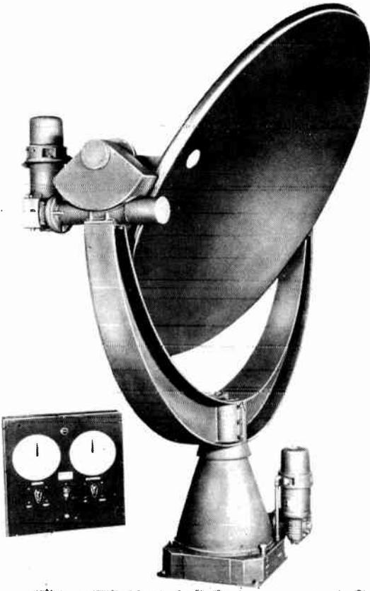
Fig. 20-6. Houston-Fearless remote control for microwave receiver. Controls at left include direction and tilt indicators.
