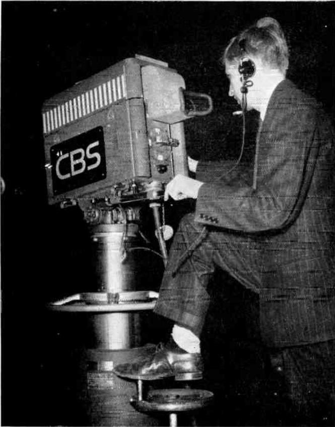
Fig. 4-11. Pat McBride adjusts pedestal height while his camera is on the air. (Courtesy of Popular Science.)
