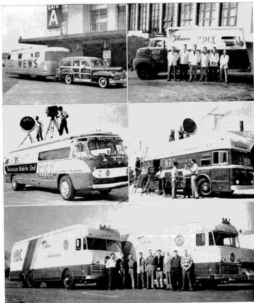
Fig. 20-15. Six representative mobile units. Top left, WEWS, Cleveland, adapted Spartan House trailer. Top right, KPIX, San Francisco, adapted Ford truck. Center left, WKY-TV, Oklahoma City, adapted Flexible bus. Center right, NBC "crash" unit includes audio and video transmitters and gas-driven generator. Bottom, NBC, Hollywood, color TV mobile vans.
