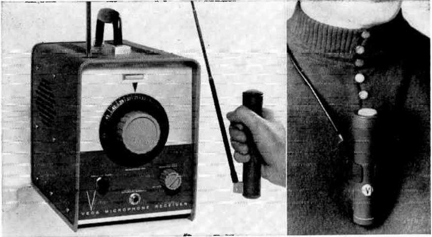
Fig. 19-15. Vega wireless microphone. Receiving unit on left. Mike may be used in the hand with telescoping antenna or may be worn as a lavalier, in which case the neck strap acts as an antenna element. Several Vega microphones may be used with one receiving unit, either on the same frequency (in which case they all operate together without individual adjustment) or on different frequencies (in which case they can only be used separately, since the receiving unit must be retuned between them).
