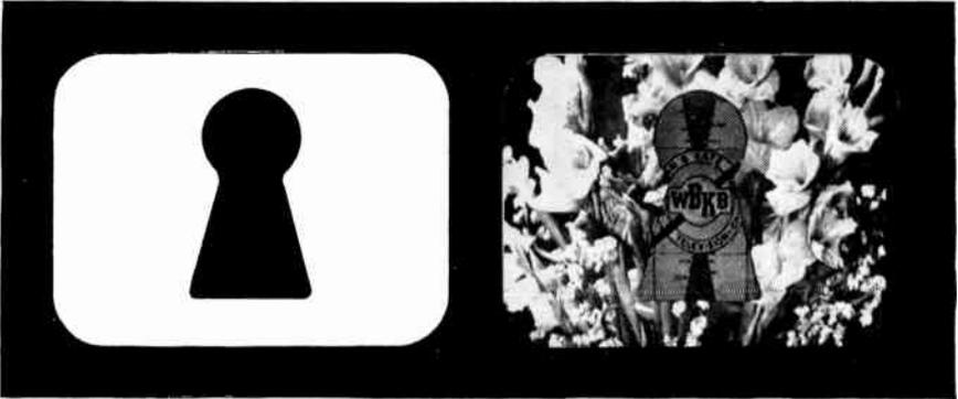
Fig. 15-9. Keyhole area used as control signal to make composite of two pictures.
