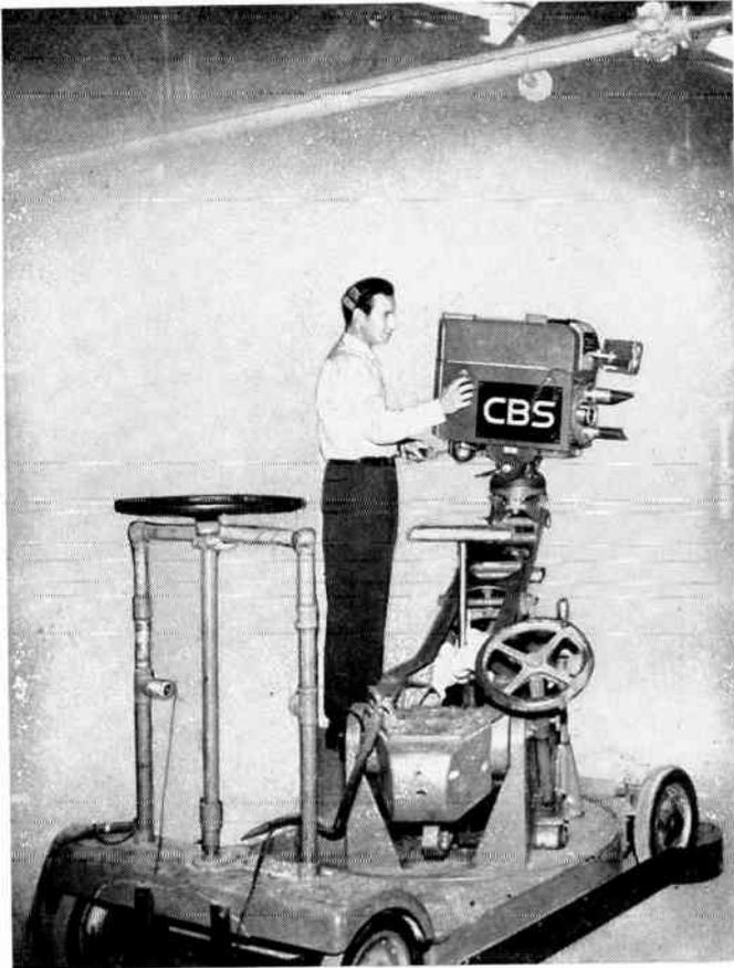
Fig. 4-16. Fearless dolly adapted by CBS with 3-foot extension on boom counterbalanced by large weight (foreground). Note that auto steering wheel replaces standard handle.
