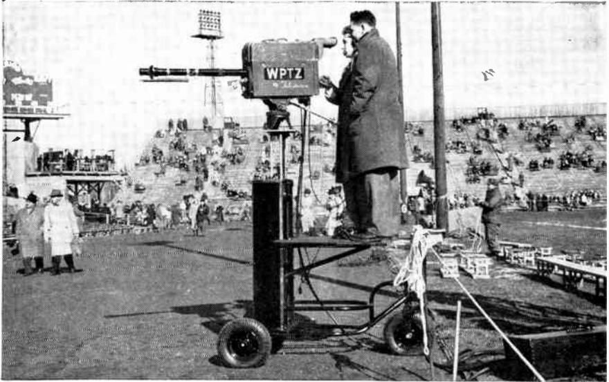
Fig. 20-27. WPTZ camera on field mounted on studio mike-boom base.
