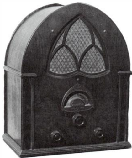
1931 Atwater Kent (superheterodyne) "cathedral" model table receiver.
