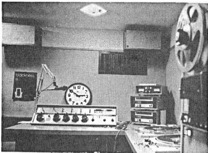
Fig. 4-2. No matter how small or financially deficient a station is, it has to have at least one small production studio. A studio like this can be used to cut commercials or promotional announcements or even tape programs where one person is both engineer and announcer (photo courtesy Thirk Holland).
