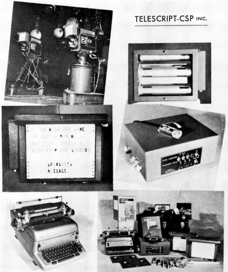
Figure 42. Telescript. Lower right, complete unit for two cameras; lower left, special typewriter with large print; middle right, speed control; upper right, scrolls of copy as they appear from rear; middle left, copy as seen from front; upper left, Telescript mounted on cameras.
