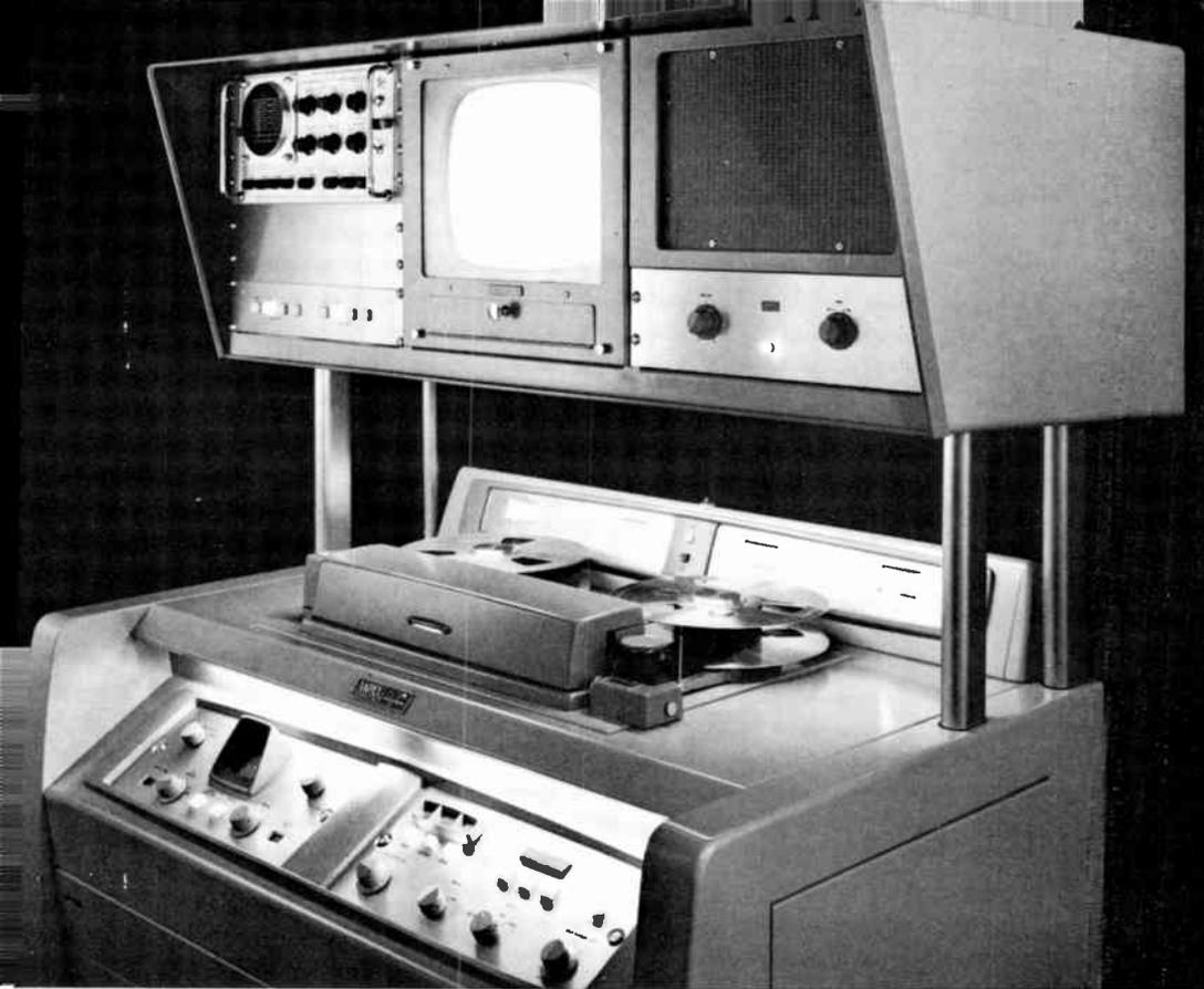
Figure 59. Videotape, Ampex VR-1000 Magnetic Recorder.
