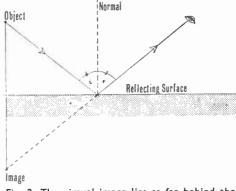
Fig. 2. The virtual image lies as far behind the mirror as the object does in front.
