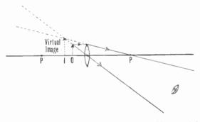
Fig. 9. When the object is between the principal focus and the lens, the image is erect, magnified and virtual.
