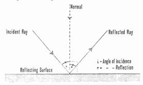
Fig. I. Behaviour of light wave striking a reflecting surface—such as a mirror. Note: Angle i = angle r.
