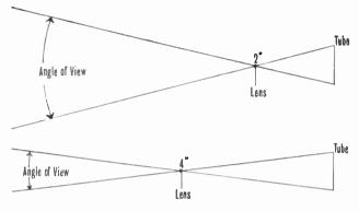
Fig. 14. A simple method of remembering the relationship between focal length and angle of view of a lens. Short focal length = wide angle of view. Long focal length = narrow angle of view.
