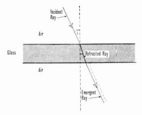
Fig. 4. Behaviour of light wave passing through glass. Note that the refracted ray is bent towards the normal and the emergent ray is parallel to the incident ray.
