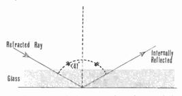
Fig. 7. When angle between refracted ray and the normal is greater than the "critical angle", there is no emergent ray.
