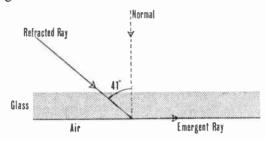
Fig. 6. When the refracted ray makes the "critical angle" with the normal, the emergent ray travels along the surface of the glass.
