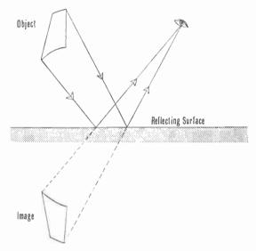
Fig. 3. If the image is studied from the position of the eye in the diagram, it will be seen that this image is vertically erect, laterally inverted and of unity magnification.
