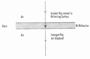
Fig. 5. A ray of light entering glass along the normal is not refracted.
