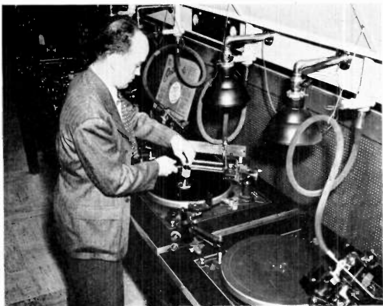
A transcription engineer adjusts the cutting device which makes a transcription out of a "blank", the ungrooved wax disc.
