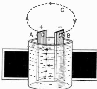
Fig. 1-A. A simple primary or electrolytic cell.
