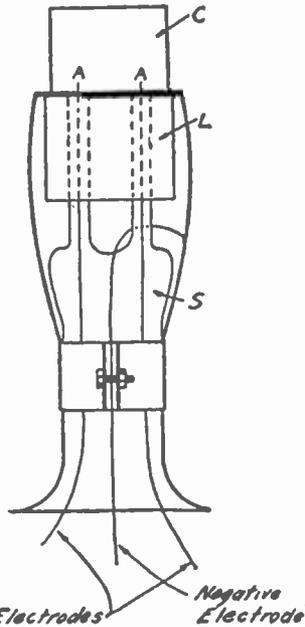
Fig. 2. Construction of the Raytheon tube.
