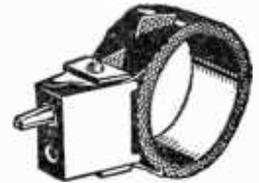
Honeycomb coil used in radio reception.
