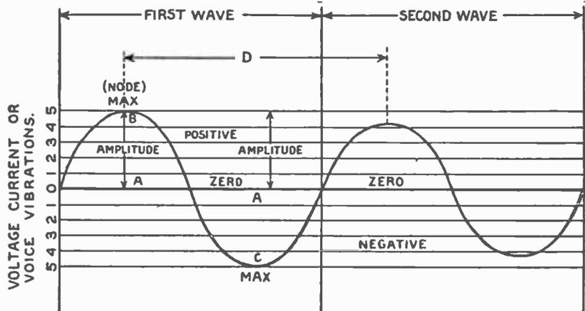
Line wave showing two cycles of an alternating current, indicating the amplitude and damping
