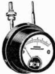
A plug-in type of voltmeter.
