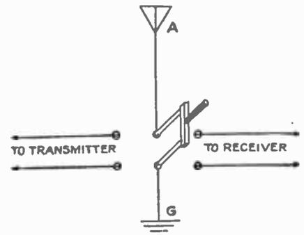
Fig. 2. Circuit for a simple Aerial Switch
