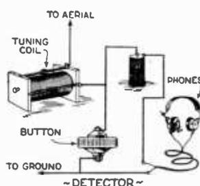
Fig. 15. Transmitter button used as radio detector.
