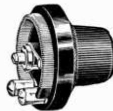
A rheostat constructed of resistance wire.
