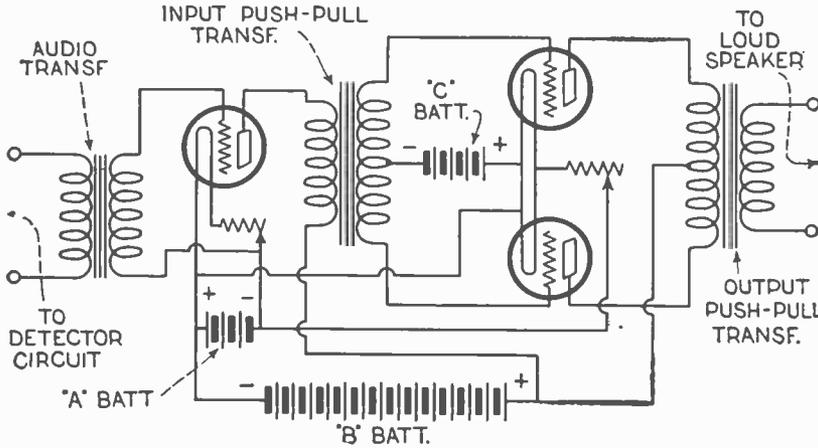
Fig. 1. Diagram of a push-pull amplification circuit.
