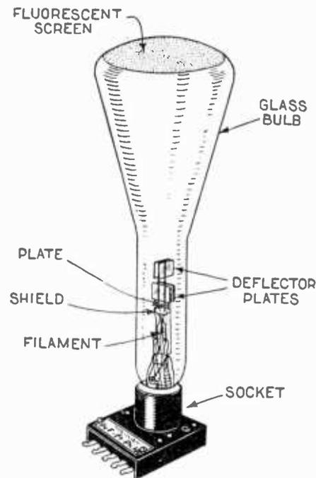
measurement of hysteresis and dielectric loss in various materials, study of phenomena in arcs and sparks, together with numerous other associated effects. The development of this tube is one of the marvels of science, enabling the research engineer to virtually see the electric wave, and to study exhaustively, electric phenomena otherwise invisible.
