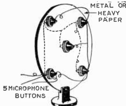
Fig. 5. Combining buttons to form sensitive microphone.
