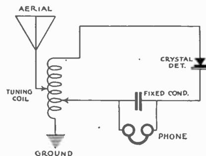
Fig. 2. Crystal receiver using double slide tuner.
