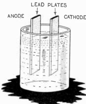
Fig. 2.—Storage or secondary cell.
