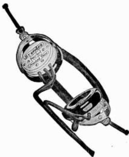
Illustration by courtesy of C. Brandes, Inc. A type of headphone used extensively in radio reception.
