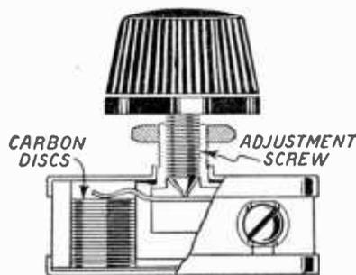
Fig. 2.—A carbon pressure type rheostat.
