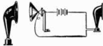
Fig. 2. Retransmitting radio programs.
