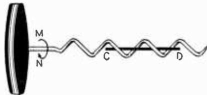
Illustration of Maxwell's corkscrew rule. When current flows from C to D, magnetic lines encircle the wire in the direction of the curved arrow MN.
