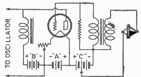
Fig. 17. Use of button in Heising modulation system.
