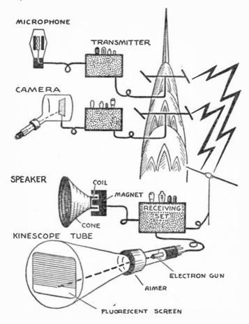
The procession of impulses, which is the electrical record of all the tiny sections of the picture, is fed into the electron gun. It is the gun's supply of ammunition —just as a machine gun is fed a steady procession of bullets. As each impulse enters the "firing chamber" of
