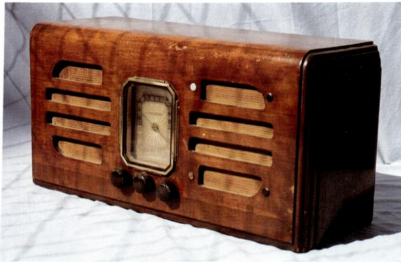
Unusual model 38-15 table model, which despite the two speaker openings, uses only one speaker. Photo by Michael Prosis.
