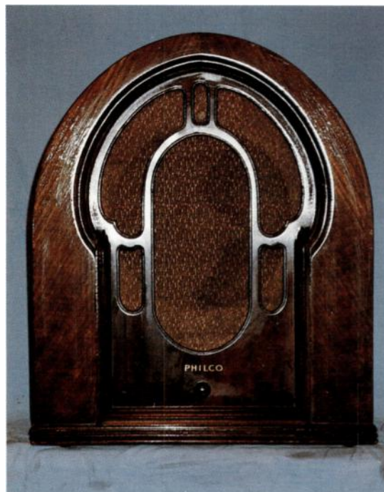
Extension speaker for use with Philco receivers, from 1932. Photo by Michael Prosis.
