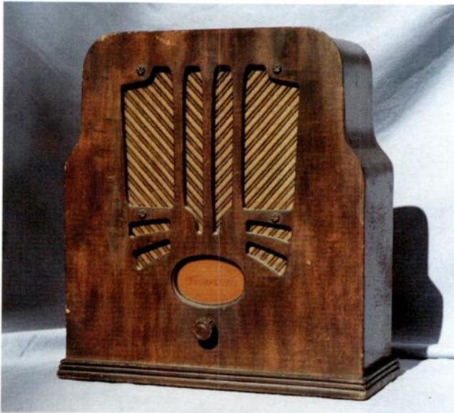
Philco "Teleflash" from the mid thirties. Not actually a radio; the cabinet contains an audio amplifier and a speaker. It was wired to telephone lines and may have been used for news reports or horse racing play-by-play. Photo by Michael Prosisie.
