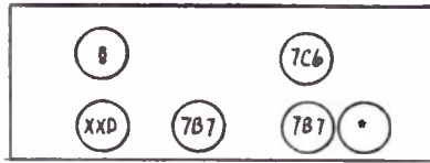
15-14. Model 42-358. * - 50L6GT in Code 121, 35L6GT in Code 122. # - 35Z3 in Code 121, 50Y6GT in Code 122.
