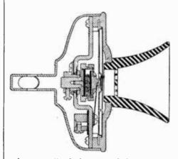
A cross sectional view of a telephone transmitter showing details of construction.
