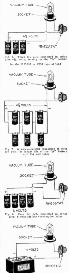
Fig. 9. Showing method of tapping at 4-volt terminal of a 6-volt storage battery for type U.V.199 or C299 tubes or other 4-volt tubes
