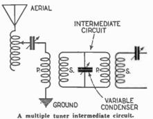
coils shunted by a variable condenser. One coil acts as primary to the secondary coil of the detector circuit and the other coil acts as secondary to the primary of the aerial circuit. A circuit such as this is sometimes referred to as a *multiple tuner intermediate* circuit and may be used as an interference eliminator.
