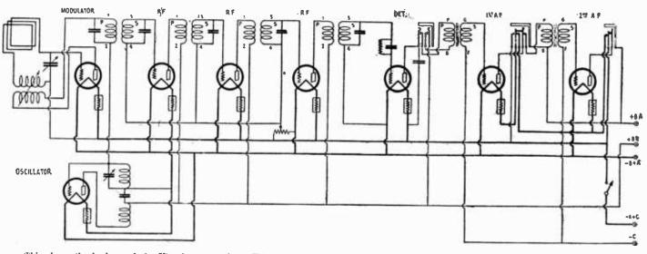
This shows the hook-up of the Ultradyne super-het. This set is not radically different from the average super-heterodyne. The heteroformers are of the tuned air core type and the filter is shown at the input side of the circuit. Aerial and ground as well as loop may be used with this set and instead of the first detector the inventor uses a tube known as the "modulator."
