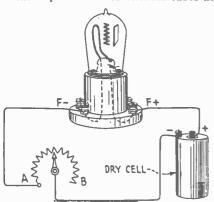
The current produced hy the dry cell battery, flowing through the rheostat and filament, is consumed by the filament, at a rate depending upon the type of tube.
