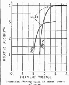
the curve indicating relation between voltage and signal strength in two types of vacuum tubes. The points marked "Peak" in each curve represent the critical points of the curves at which maximum audibility is obtained, any further increase in voltage not increasing the audibility. (See Charac-teristic Curve, also Curve.)
