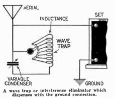
ceiving set. The inductance is usually tuned by means of a variable condenser which allows it to be tuned to the wave-length of the interfering signal. The interference can thus be by-passed to the ground. Interference eliminators of the kind described are generally known as wave traps (q.v.). A special form of interference due to atmospheric and electrical disturbances is known as static (q.v.). (See Static Eliminator.)
