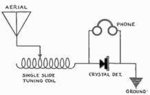
Fig. 1. Simple crystal set with single slide tuner.
