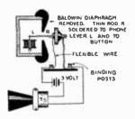
Fig. 9. Button attached to Baldwin 'phone.
