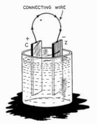
Fig. 1.-Common form of electric cell.
