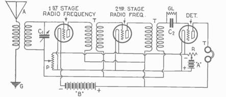
Fig. 1.-Circuit diagram showing two stages of cascade radio frequency amplification and detector.
