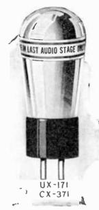
A new storagebattery type power amplifier tube, for use in the last stage audio amplifier only. This tube takes the same filament voltage and filament current as the No. 112 tube but employs a "B" voltage of 180 and 40½volt "C" babtery. Special means should be provided for handling its .eavy output.
