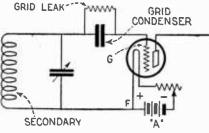
Showing how grid condenser is connected in a detector circuit.
