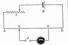
GALVANOMETER A simple form of potentiometer used for electrical measurements.
