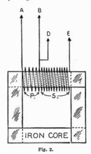
coming crossed or shorted. (See Short.) For this reason they are used mainly for comparatively low voltages. One of the most common forms is the step-down type, known as a "bell-ringing transformer." These are used to cut down the voltage of an electric light line to suitable value for use with small toys or bells. If the transformer is used to increase the voltage, it is known as a "step-up" transformer. (See Transformer—Radio, Audio.)
