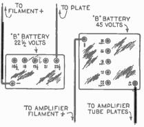
Fig. 5. Method of employing separate "B" Batteries for the detector and amplifier.
