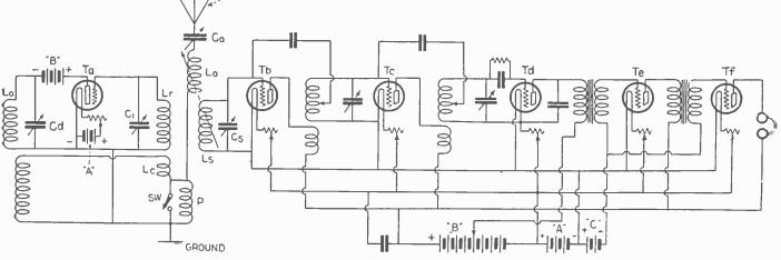
Arrangements of a static reducing device employing repeater circuits.
