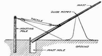
A method of erecting a tall mast using tackle and hoisting pole.
