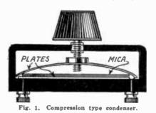
rotation of the dial of a variable condenser. Three types of condensers are shown here, the *compression*, Fig. 1, the *straight line capacity*, Fig. 2, and the square law, Fig. 3. In Fig. 1A is shown the relation of capacity and wavelength changes when the dial of a sample compression condenser was rotated. The condenser was shunted
