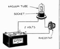
Fig. 10. How a single cell of a 6-volt storage battery may be employed to furnish "A" bat-tery current for 1½ volt tubes
