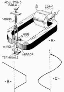
Fig. 1. The principle of operation of the oscillograph is shown at A. At B are shown diagonal and straight paths traced by the beam of light falling on a moving photographic plate. The type of curve which an oscillograph traces for alternating currents is shown at C.
