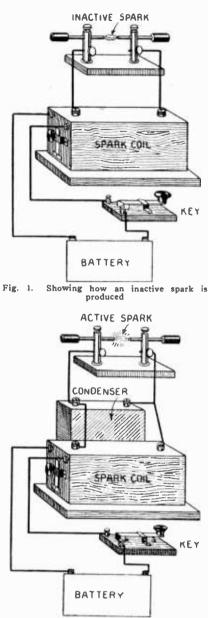
Fig. 2. The active spark is produced by means of a condenser in the circuit as shown
