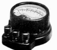
Photo by Courtesy of Weston Electrical Instrument Co. Double range meter, one range to 7½ volts, higher range to 140 volts maximum.
