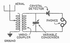
Fig. 1. Schematic diagram of a simple crystal receiver.
