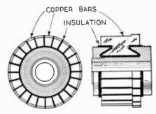
Front and side view of Commutator.
