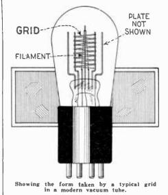
flow. That is to say, at the instant the grid is positive it will attract more electrons, but when it is momentarily negative the like charges will repel each other and less electrons will flow, some of them being held back to the filament. (See Grid Battery, Grid Bias, also Vacuum Tube, Theory of Operation of.)
