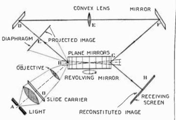
cover the picture, the latter six. It is obvious that to reproduce the picture at the other end the process must be reversed, the lines being replaced side by side by means of a pair of prismatic
