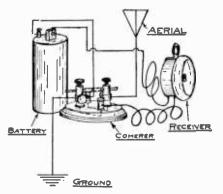
Coherer used in radio receiving circuit.
