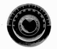
Fig. 3. A dial as used on radio receiving sets may be Calibrated according to different wavelengths.
