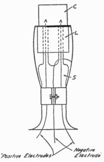
Fig. 2. Construction of the Raytheon tube.
