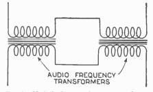
Fig. 2. Method of connecting two transformers where a tapped wound tranformer is not available.
