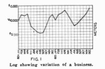
and horizontally, as in Figure 1, the months and years are marked at the bottom horizontally. The vertical lines then represent the months and the bottom horizontal line is called the *axis* of *time*. These vertical lines are known technically as *ordinates*. The vertical line to the extreme left is called the axis of ordinates and after it has been marked as shown in Figure 1, to represent dollars, it may be
