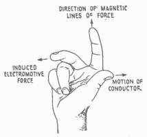
Method of using the right hand in determining the direction of the induced current.
