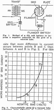
Fig. 2. Characteristic curve of a vacuum tube indicating more difference in current occurs between "B" and "C." than between "A" and "B."
