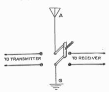
Fig. 2. Circuit for a simple Aerial Switch
