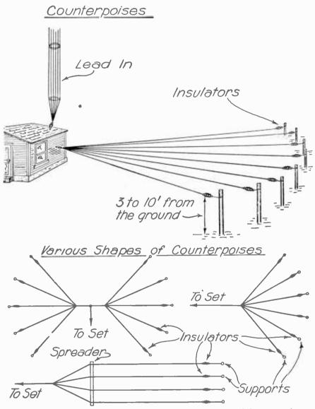
Fig. 11. Different methods of arranging counterpoises for either transmission or reception
