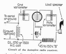
along the lines of the Super-regenerative principle and designed to operate a Loud-speaker. The circuit comprises two standard variometers, a 1500 turn duo-lateral coil, and the usual vacuum tube, socket, batteries, etc. It is extremely critical in operation, but if carefully assembled will give excellent volume under good conditions. Illustration shows the circuit diagram of the Autoplex receiver.
