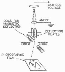
Fig. 2. A diagrammatic representation of the Dufour oscillograph.
