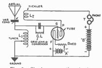
Fig. 2. Simple regenerative circuit.
