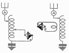
Fig. 19. Method of modulating output current.
