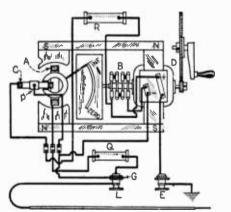
A diagrammatic illustration of a megger.
