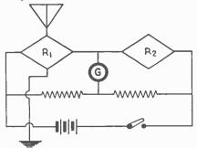
A thermal detector. By means of the change of resistance of a conductor, due to heating, electro-magnetic waves are detected.  $R_1$  and  $R_2$  are two rectangles of very fine iron wire.
