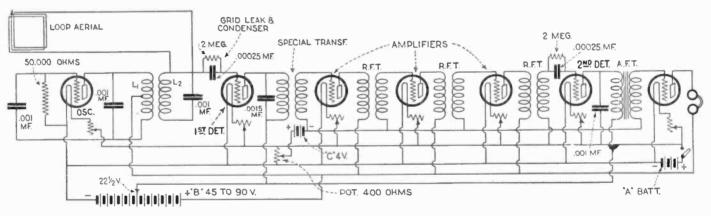
Fig. 2.-Wiring diagram of a standard 7-tube super-heterodyne.
