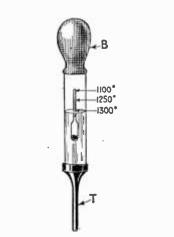
Hydrometer used to test the specific gravity of liquids.
