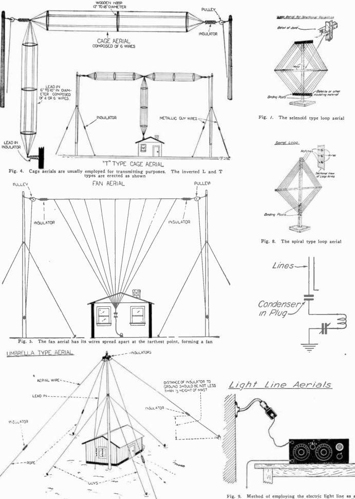
Fig. 6. The umbrella type of aerial derived its name from the arrangement of its wires in the form of an umbrella 8
