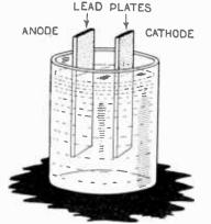
Fig. 2.-Storage or secondary cell.
