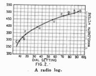
sufficiently satisfactory. In Figure 2, the dial setting is marked along the bottom of the chart. The scale is here chosen at one division on the chart equal to 5 divisions of the dial. If preferred the scale could be chosen so that one division on the chart would equal one division on the dial as shown on chart on the following page, which is a typical log of an actual set. Proceeding, it is first necessary to find
