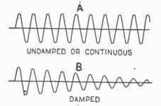
Series of undamped and damped waves.
