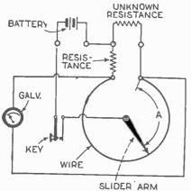
Diagram of connections of a slide wire ohmmeter.
