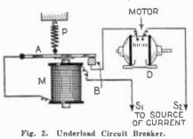
a switch, in which "A" has attached to it a piece of soft iron. Now if the current required for the motor is ten amperes, the magnet can be so designed
