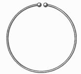
Fig. 1. Early type of cymoscope used to indicate resonance in a circuit.
