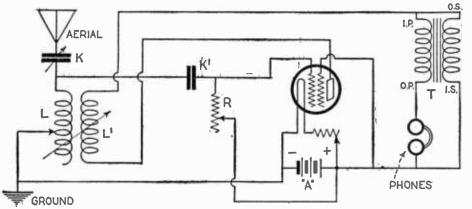
A Solodyne circuit. L and L<sup>1</sup> may be honeycomb coils or a vario-coupler.
