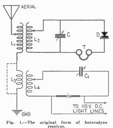
In its original conception by Fessenden, before the widespread use of vacuum tubes, it was used in conjunction with crystal receivers for the reception of *undamped waves* (q.v.). The heterodyne principle involves production of a local series of oscillations which are tuned to a frequency differing from the frequency of the incoming oscillations from the antenna. The difference between the two is known as the beat frequency. (See Beats, also Heterodyne Receiver.)
