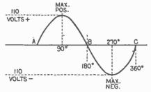
Curve showing action of 110 volts alternating current during one cycle.
