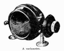
VARIOMETER—A tuner, similar to the vario-coupler, except that the primary and secondary coils are electrically connected.
