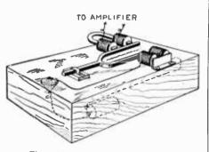
Fig. 14. A tuning fork oscillator.
