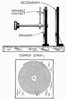
Front and side view of a pancake coil. **PANCAKE** COIL—A flat inductance Coils of this type are used in coil. radio receiving sets as radio frequency 122
