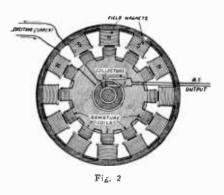
S, the poles of the magnets. As the conductor moves across the flux lines of the magnet, an *electro-motive force* (q.v.) or *electric* current is set up or induced in the conductor, this force being in such a direction that the current produced will create a flux or magnetic field, in the same direction as the flux on the side of the conductor. In this case E.M.F. (electromotive force) is in the direction B to C in the conductor. In order to establish a circuit and utilize the current pro-
