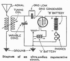
tion which uses a form of regeneration, without calling for the introduction of auxiliary equipment in the circuit. A typical ultra-audion circuit is illustrated. It will be noticed that
