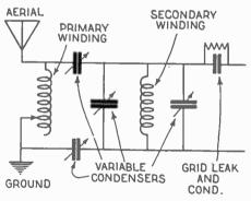
Fig. 3.—Electrostatic coupling between primary and secondary by means of variable condensers.
