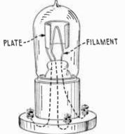
Fig. 1. The Fleming valve, which contained but two elements; i. e., filament and plate. It was the forerunner of the modern vacuum tube.
