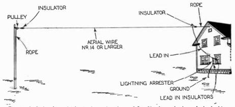
Fig. 1. A single wire aerial in the form of an inverted L. If a long wire is used, the lead-is may be connected in the center, forming a T type
