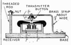
Fig. 7. Method of fastening a button to ear 'phone.
