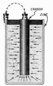
Fig. 1. Illustration showing the assumed direction of current flow in a dry battery.
