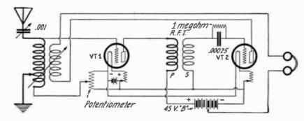
A single stage radio frequency amplifier as used in conjunction with a tuner and detector
