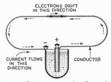
Fig. 2. Showing reverse action of current and electrons.
