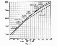
A three-dial radio log using only one chart.
