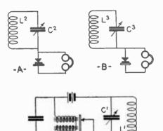
Diagram showing three-way method of wave-meter calibration.
