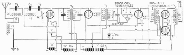
Fig. 2. Cockaday Circuit with push-pull amplifier.
