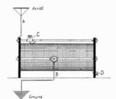
Fig. 1. Double slide tuner which affords direct coupling between the primary and secondary circuits.
