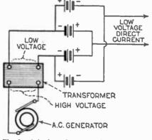
2. A hook-up for connecting four Noden cells to obtain full wave rectification. Fig. 2
