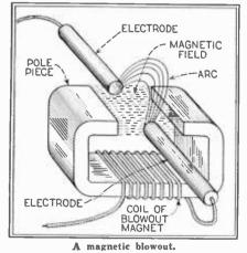
blow-out action is stronger, the larger the current to be interrupted. For small shunted arcs, permanent magnets are often used. The operating principle of the blowout coil depends upon the fact that in a magnetic field,
