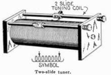
The illustration shows a common type of two slide tuner. (See Coupling Crystal Receiver, also Tuning.)
