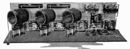
Fig. 2. A typical neutrodyne set.
