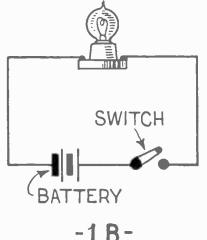
Circuit open by means of switch.
