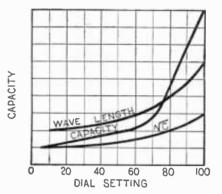
Fig. 1A. Curve for compression type condenser.
