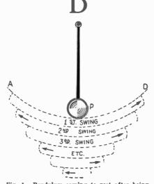
Fig. 1. Pendulum coming to rest after being given a momentary impulse.
