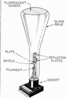
A cathode ray tube with socket.
