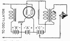
Fig. 17. Use of button in Heising modulation system.
