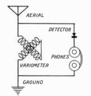
Fig. 4. A variometer is used as the tuning element in this crystal set.
