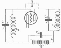
Fig. 1. A portion of a receiving circuit. Dotted line shows tube capacity represented by an equivalent condenser. represented
