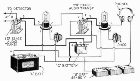
Fig. 2.--A diagram showing how the "C" battery is connected in the audio frequency amplifier.
