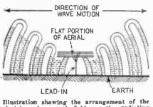
Illustration showing the arrangement of the electric and magnetic field around a radiating antenna.
