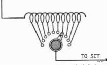
A tapped inductance which permits inductance to be added or taken out of the circuit by rotating the lever switch.
