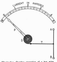
Illustration showing operation of a hot wire ammeter.
