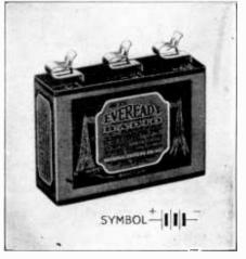
Fig. 1.—A 41/2 volt "C" battery. This type of battery has a common positive terminal and is tapped at negative terminals for 3 and 41/2 volts.
