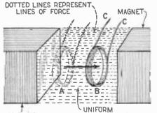
MAGNET MAGNETIC FIELD Fig. 1. Coil of wire in a uniform field moving parallel to direction of the field.
