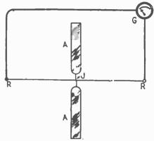
Schematic diagram showing Klemencic thermal iunction
