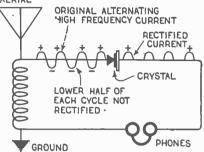
Disgram showing how crystal detector converts alternating high frequency current into pulsating direct current.
