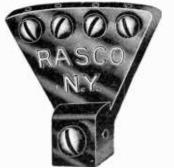
Illustration by Courtesy of Radio Specialty Co., Inc. Fan Connector—The leads from each wire of a multi-wire aerial go to the wide portion and are held by the set screws: the lead to the set goes to the small end.
