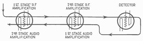
Diagram showing method of reflexing in an inverse duplex circuit,
