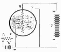
Showing how a standard vacuum tube can be connected to act as a dynatron.
