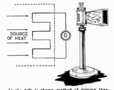
At the left is shown method of joining thermopile junctions to multiply the effect. At the right is a sensitive thermopile.
