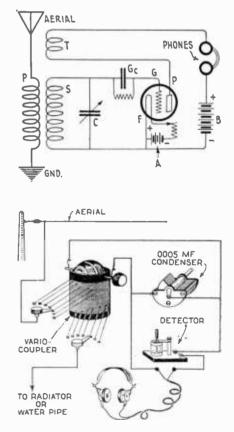
The upper diagram is in schematic form and shows a single tuhe regenerative receiver, and the lower diagram is in perspective form and shows a crystal receiving set.
