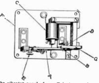
The vibrator panel of an efficient type of mechanical charger.
