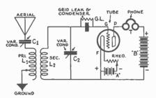
Fig 1. Non-regenerative vacuum tube circuit.
