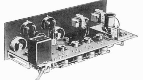
This is the rear view of the Callies Super. Note particularly the long wave transformers at the rear of the set and how they support the sub-panel.
