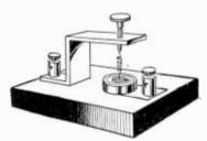
Fig. 1. Crystal detector using contact wire, or "cat-whisker."
