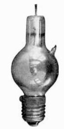
A typical rectifier tube of the Tungar type. The screw-base allows it to be inserted in a standard lamp socket from which current is obtained for the filament. Connection is made to the graphite disc by means of a Fahnestock connector which clips on to the wire post projecting from the other end of the tube.
