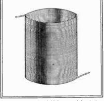
Air core coil made rigid by use of insulating compound.
