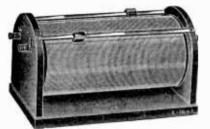
A sliding contact tuner formerly used in radio receiving sets.
