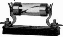
Grid leak and condenser.
