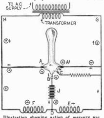
Illustration showing action of mercury arc rectifier.
