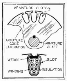
Details of armature slot.
