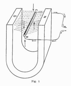
simplest form-merely a conductor, B C moved across a magnetic flux (q.v.) (Note: For a complete explanation of the production of alternating currents, see "Alternating Current, Theory of Production of.") Here the conductor B C is moved to the right across the magnetic flux shown as dotted lines between N and
