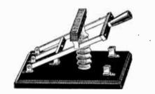
Fig. 4. An Aerial Switch with an extra blade
