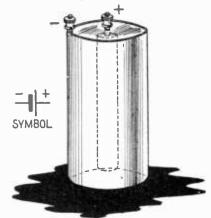
Dry cell showing positive and negative electrodes.
