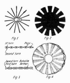
Details of spider web coil construction.
