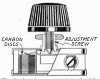
Fig. 2.---A carbon pressure type rheostat.
