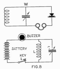
Circuit for the measurement of wavelength of coil and condenser.
