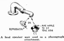
LOUDSPEAKER UNIT—The sound reproducing unit attached to the tone arm of the horn type speaker or to the diaphragm of the cone type speaker. Various types of units are described under the heading *Loudspeakers*.
