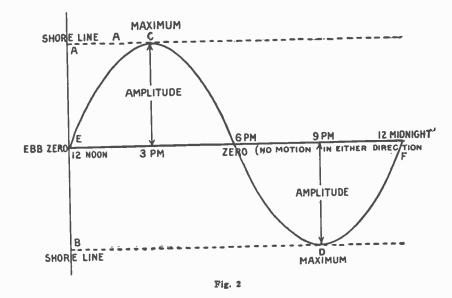
will move to B which will be the maximum positive *amplitude* (q.v.). It will then fall back to zero again, and with the power behind it, the momentum in this case, will rise on the other side to C, which is the maximum *negative*  ually rises toward that side until at 3 P. M. it has reached its maximum height. In the case of an alternating current, we may consider that at 3 P. M. the current has reached maximum value on the positive side or in
