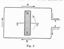
such manner as to make A act as a North pole. As the North pole of the magnet is toward this point A, the similar poles will oppose each other according to the simple law of magnetic attraction and repulsion. Now if we attempt to withdraw the magnet, the change will alter the linkages again, this time creating an induced current that makes A act as a South pole, thus *attracting* the magnetic North pole and opposing in the op-
