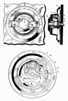
This dial utilizes the slip tooth principle. 5 is the main dial. 6 turns the slip gears (3) and (4), which cause 2 to turn. 2 is mounted on the shaft (1A) fastened in the main dial (1). 5 is the scale, fastened to the condemser shaft.
