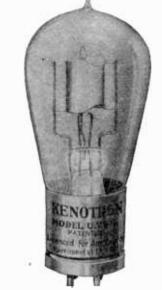
Illustration by courtesy of Radio Corp. of America A kenotron tube.
