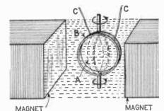
Fig. 2. Same coil, showing cutting of field due to the rotation of the coil.
