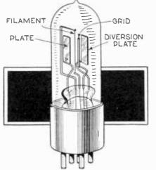
A negatron tube, showing the two plate con-struction.
