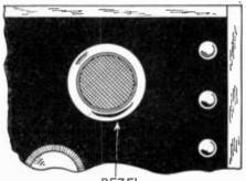
BEZEL A Bezel on the panel of a radio receiving set.
