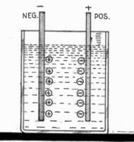
Illustration showing the action of ions in a primary cell.
