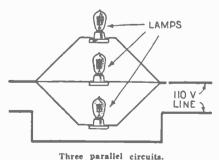
shows three parallel circuits. Actually each one is a part of the whole circuit. (See Parallel Resistances.)
