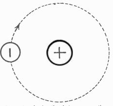
Illustration showing the electron, or negative particle, revolving around the proton or posi-tive nucleus.
