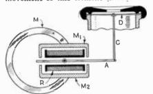
Principle plan of the Baldwin Receiver unit.
