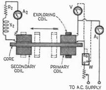
Diagram illustrating mutual inductance. The reactance of the coil  $A_1$  is reduced by the proximity of coil  $A_{22}$  since the circuit of  $A_2$  contains no source of electromotive force. The effect of the secondary coil depends not only upon its distance from the primary coil but also upon  $R_2$  and  $X_2$ . The presence of the iron core greatly increases the action.
