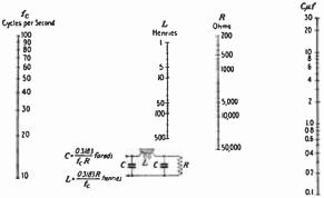
FIG. 30.—Low-pass filter design chart,  $\pi$  section.
