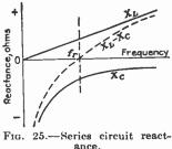
14. Impedance of Series Resonant Circuits. At resonance, the impedance is R, the total series resistance of the circuit. At any other frequency,  $f_1$ , there is also a reactance component
