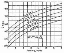
FIG. 59.-Characteristic impedance of open-wire r-f transmission line.
