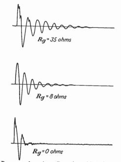
FIG. 40.—Response of moving-coil speaker with 8-ohm voice coil to an electrical pulse as source resistance is varied. Minor irregularities in curves are due to h-f modes of vibration of diaphragm.
