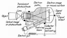
FIG. 16.-Structure of the image iconoscope.
