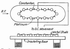
FIG. 7.-Galvanometer or bridge-type couple.
