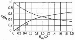
FIG. 6.-Linearity in absorption modulation.
