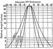
FIG. 7.—Selectivity characteristics of coupled tuned-circuit t-r-f transformer. circuit t-r-f transformer is approximately one-half that which ean be obtained from a transformer using a single tuned circuit.
