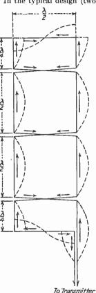
FIG. 45.—Current distribution in barrage antenna panel.
