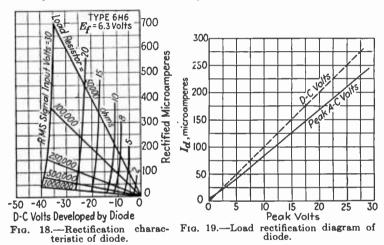
Figure 18 shows the rectification characteristic of a typical diode. Rectified current is given for several steps of r-m-s input voltage in terms of d-c load voltage. These characteristics may be determined by test at 60 cycles according to the method of Art. 9.
