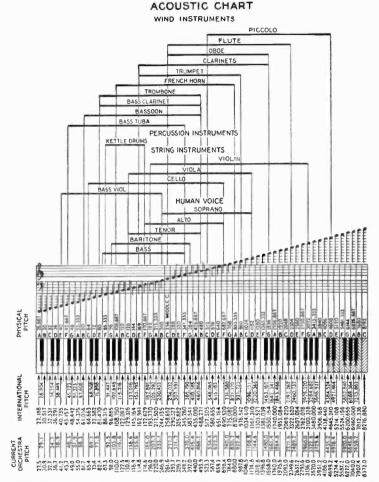
Fig. 2.—Correlated acoustic chart showing the scientific or philosophical scale generally used by physicists, the international equally tempered scale based on A = 435 complete vibrations per second. This scale was formerly used by musicians. The current orchestra or symphony scale based on A = 440 complete vibrations per second is at present generally used by musicians.
