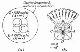
FIG. 8.—(a) Space radiation pattern of simultaneous radio range-beacon and weather-broadcast station; (b) range-beacon signals produced.
