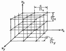
FIG. 34.—Distribution of resonant frequencies for a rectangular room with side lengths  $l_x$ ,  $l_y$ , and  $l_z$ . The length of a vector from the origin to each lattice point indicates the frequency and the direction of the vector indicates the direction of the corresponding standing wave. The velocity of the sound wave c is given by Eq. (1).
