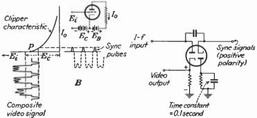
FIG. 48.—Clipper circuit and characteristic, used to separate composite sync signals from camera signals. Fig. 49.—Combined second detector and sync amplitude separator (clipper).
