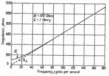
FIG. 6.—Impedance of inductive circuit with frequency.
