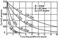
FIG. 2.—Fall of current in inductive circuit.
