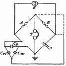
FIG. 46.—Three-terminal capacitance.
