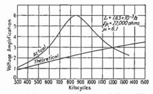
FIG. 6.—Amplification of a choke-coupled amplifier tube.
