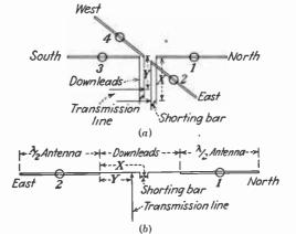
FIG. 14.—Details of antenna system for cone-type marker: (a) method of feeding; (b) detail of 10-deg. phasing.
