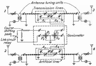
FIG. 9.--Schematic diagram of radio range-beacon antenna-coupling system.
