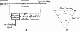
F10. 43.—Armstrong modulation system. A, the circuit arrangement, (Armstrong, Proc. I.R.E., 24, 689, May, 1936); B, a vector representation of manner in which side-band voltage is added to carrier to generate p-m wave.
