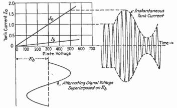
Fig. 28.-Modulation of class C amplifier by superimposing a-f signal voltage on plate-supply voltage
