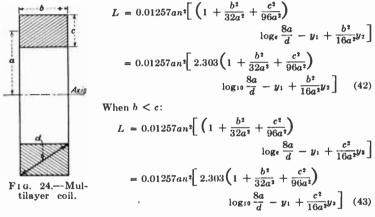
$y_1$ ,  $y_2$ , and  $y_3$  may be obtained from the table shown below. These formulas are quite accurate as long as the diagonal of the cross section (*d* Fig. 24) does not exceed the mean radius. The accuracy decreases considerably as *b* becomes large in comparison with *a*.
