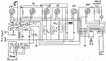
FIG. 51.-Schematic diagram of RCA 66A modulation monitor.
