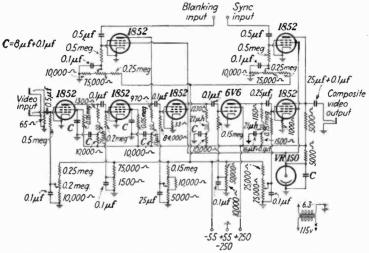
35. Shading-correction Generator. The shading-correction generator is a device for producing wave shapes of saw-tooth, sine, and parabolic
