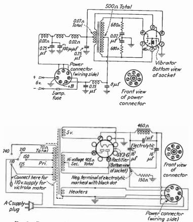
Fig. 8.-Power supplies from 6 volts d.c. and 110 to 240 volts a.c.
