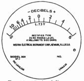
Fig. 14e.-Scale of db meter.
