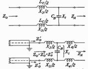
FIG. 91.—Matching circuits for balanced transmission lines.
