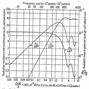
FIG. 11.—Radiation resistance, reactance, and mass per square centimeter of a flat, rigid piston vibrating in an infinite, rigid non-absorbing baffle. Piston radiates into a solid angle,  $\Omega = 2\pi$  steradians (hemisphere).
