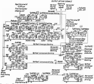
FIG. 21.—Typical vertical shaping unit of a synchronization signal generator (441-line image). (After Deal.)
