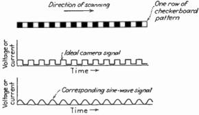
$F_{10}$ . 6.—Wave forms resulting from scanning a checkerboard image. The ideal square wave becomes a sine wave when only the fundamental frequency is transmitted.
