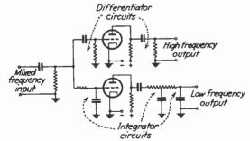
F13. 52.—Combined differentiator and integrator circuits for wave-form separation.
