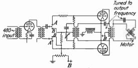
FIG. 14.—Schematic diagram of controlled thyratron inverter for driving synchronous motors.
