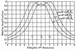
FIG. 14.—Response curves of doubly-tuned r-f stage.
