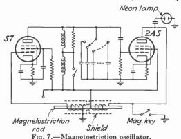
effect in crystals. There is an expansion or contraction of magnetic materials as a result of magnetization and, conversely, a change of magnetic permeability as a result of mechanical stress.
