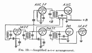
control potential is applied to the signal amplifier tube subsequent to the point to which the separate a-v-c amplifier tube is connected.
