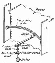
FIG. 12.—One type of startstop recorder used for home reception.
