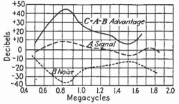
Fig. 64.—A, signal as received with ordinary antenna equipment; C, advantage secured by noise-reducing equipment.
