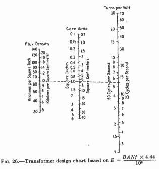
increase the core area and allow a smaller number of turns per volt, thus decreasing the cross section of the winding.
