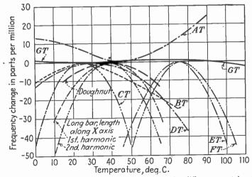
FIG. 6.-The temperature coefficient of frequency for different crystal cuts. (Courtesy of Bell System Tech. Jour.)
