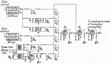
FIG. 24.-Typical shading-correction signal generator. (After Bedford.)
