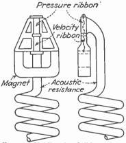
Fig. 10.— Unidirectional ribbon microphone elements.
