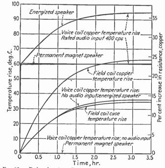
FIG. 25a.—Reduced voice-coil temperature rise in permanent-magnet speakers compared to energized types. Abnormal voice-coil temperature rise when rated "complex-wave" input is applied at 400 cycles also shown.
