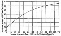
FIG. 12.—Flash-over voltage (60 cycles) of 2,000-kva. capacitor.
