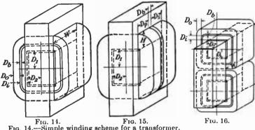
FIG. 14.-Simple winding scheme for a transformer. FIG. 15 .- Winding scheme for low effective capacitance. FIG. 16.—Simple winding scheme for a core-type transformer.
