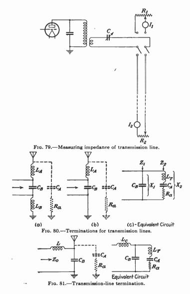
circuits used for terminating transmission lines are shown in Figs. 80 to 82 together with their equivalent circuits.
