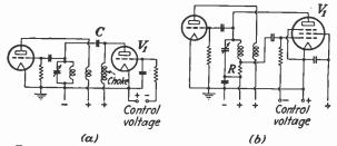
FIG. 33.-Oscillators having automatic-frequency control.
