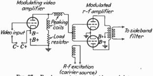
FIG. 37.-Fundamental circuit of video modulator.
