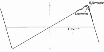
FIG. 8.—Ideal saw-tooth wave  $(k_k = 6.66)$  and approximations resulting from inclusion of 5 and 15 harmonics.
