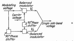
FIG. 42.—Phase-shift system for generation of single-side-band signal.
