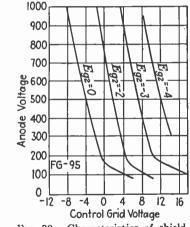
Fig. 38.—Characteristics of shieldgrid thyratron.
