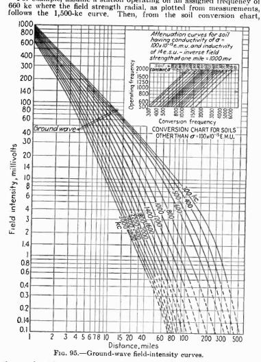
the conductivity is very nearly  $20 \times 10^{-15}$  e.m.u. On the other hand, if the soil conductivity is known, the signal attenuation can be determined from the conversion chart and the attenuation curves
