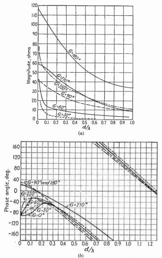
F10. 11a and b.—Magnitude and phase angle of mutual impedance vector for identical vertical radiators.
