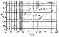
F10. 35.—Length of line to resonate with condenser. X = reactance of condenser;  $Z_0 =$  characteristic impedance of transmission line.
