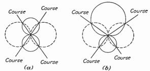
FIG. 10.—Alignment of range-beacon courses with the airways: (a) course squeezing; (b) course bending.
