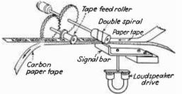
FIG. 19.-Elements of facsimile tape recorder with double spiral.
