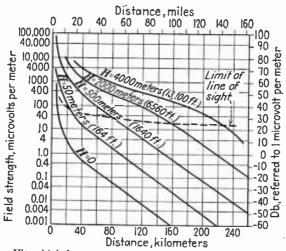
FIG. 8.—Ultra-high-frequency propagation over average land ( $\epsilon = 5, \sigma = 10^{-13}$  e.m.u.) at 50 Mc. Antenna current equals that produced by 1 kw in antenna at surface of earth. (Report of Committee on Radio Wave Propagation, Proc. I.R.E., 26, 1193, October, 1938.)
