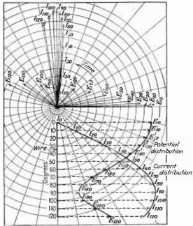
FIG. 3.—Currents and voltages in a wire of 120 deg. when appreciable power loss occurs.
