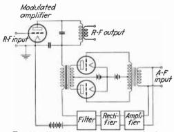
FIG. 36.—Variable carrier transmitter circuit.
