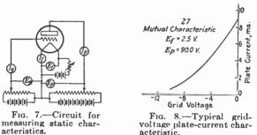
When the grid is connected to a source of voltage, the electrons are attracted if the grid is positive with respect to the cathode and repelled if it is negative. The close proximity of the grid to the space charge surrounding the cathode increases its effectiveness in controlling the electron flow.
