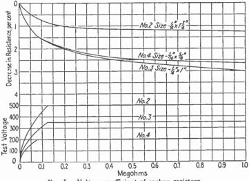
FIG. 5.-Voltage coefficient of carbon resistors.
