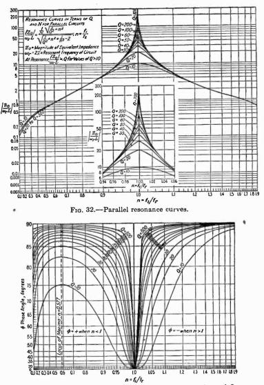
Fig. 33.—Phase angle of parallel LC circuit in terms of n and Q.
