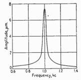
FIG. 23.—Resonance curve of Western Electric telephone.
