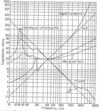
FIG. 23.—Magnitude of normal input impedance of various speakers all adjusted to same value at 400 cycles to simplify comparison. Magnitude of reactance of pure capacitance and inductance shown for comparison.
