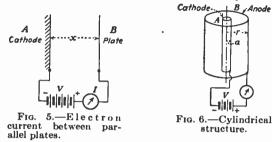
the value necessary to give the full current emitted at A. When the anode potential is great enough to draw over all of the electrons emitted at A, the current (saturation current)  $I_*$  is given by the Richardson-Dushman equation.
