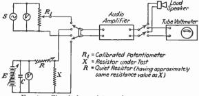
Fig. 9.—Circuit for resistor-noise measurement.
