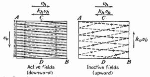
FIG. 2.-Scanning pattern for two-to-one odd-line interlaced scanning.
