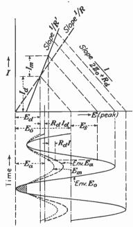
FIG. 22 .- Diode detection with resistive load.
