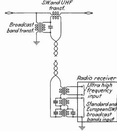
FIG. 63.-System for operating several broadcast receivers.
