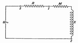
FIG. 12.-Circuit for determining inductance of iron-core coil.
