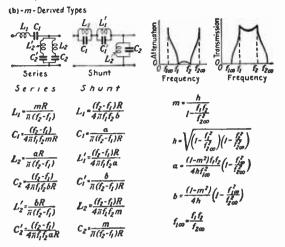
**Examples of Filter Design:** 1. Single-section Filter. Required: High-pass single-section filter to be connected between resistance terminations of R = 1,000 ohms, with a cutoff frequency of 1,000 cycles and maximum attenuation occurring at 800 cycles.
