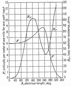
FIG. 7.—Radiation resistance and field intensity from simple vertical antenna over perfect earth.<sup>1</sup>
