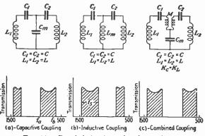
FIG. 44.-Coupled circuits as band-pass filters.
