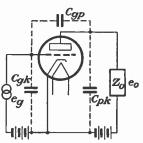
FIG. 3.—Triode amplifier showing interelectrode capacitances.
