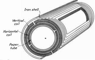
FIG. 63.—Construction of a typical scanning yoke (magnetic-deflection eoil system).
