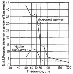
FIG. 30.—Total distortion of open-back cabinet and of the same cabinet enclosed as shown in Fig. 28, same speaker and electrical input in both cases. L-f distortion much reduced because diaphragm sees high antiresonant impedance of enclosure and therefore has only small displacement whereas air in port (which lacks the non-linear edge stiffness and non-uniform flux of the speaker) moves with large displacement.
