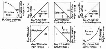
FIG. 65.—Transfer of object brightness to image brightness through subsidiary transfer characteristics of the elements of a television system.
