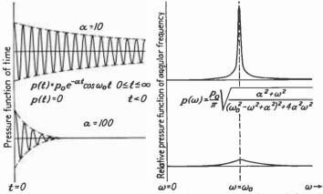
FIG. 7.—Pressure variation with frequency for two isolated damped sinusoids with different rates of decay, values of  $\alpha$  the same in the two sets of curves.
