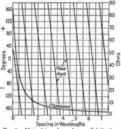
Fig. 9.-Mutual impedance for parallel dipoles.
