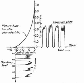
FIG. 57.-Dynamic action of video signal in picture-tube control circuit.
