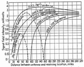
FIG. 96.—Sky-wave propagation curves for antennas of various heights. Layer height = 100 km, reflection coefficient = 1.
