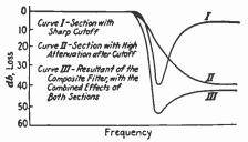
FIG. 64.—Transmission curves for composite low-pass filter.
