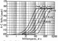
FIG. 15 .- Full-wave rectifier characteristics.
