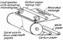
F10. 17.-Elements of bar-and-spiral type recorder with carbon recording.
