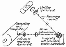
FIG. 16.—Elements of optical system with mirror galvanometer and linear penumbra mask.
