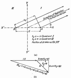
FIG. 20a and b.-Data used in calculating directivity diagrams.
