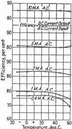
Fig. 13.—Ambient tempera-ture-efficiency relation.
