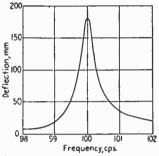
FIG. 3.—Resonance curve of vibration galvanometer.
