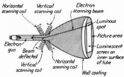
Fig. 53.—Structure of a typical picture tube.
