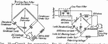
FIG. 10.—Circuit for measuring electrolytic condenser capacitance.
