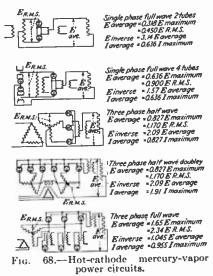
is only 4.5 per cent greater than the average output voltage; the wave form is that of a six-phase rectifier.
