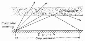
FIG. 5.—Probable paths traversed by sky wave at h.f. A single ionized layer is shown.
