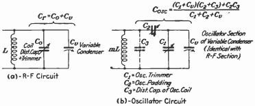
Fig. 34.—Oscillator circuits for superheterodyne.
