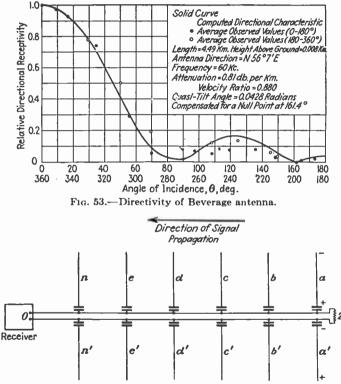
FIG. 54.—High-frequency Beverage antenna.
