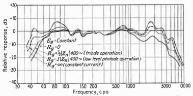
FIG. 39.—Variation in total sound power radiated by a bass reflex enclosure into a room as source impedance (impedance match) is varied. Generator or source voltage constant for each curve but arbitrarily raised as the source resistance was raised to maintain constant acoustic output at 400 cycles.
