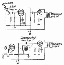
FIG. 6.—Typical scanner amplifier circuits: (above) a-c amplifier for use with light chopper in the optical system; (below) modulator amplifier for use with d-c output of phototube.
