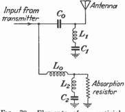
FIG. 39.—Elements of a vestigial side-band filter.
