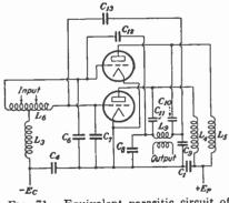
FIG. 71.—Equivalent parasitic circuit of Fig. 69.
