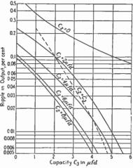
FIG. 36.—Percentage ripple as a function of C<sub>2</sub> and C<sub>3</sub>.
