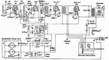
Fig. 29.—Superregenerator receiver for police cars.
