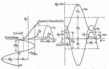
FIG. 26.-Instantaneous values of current and voltage in class C amplifier.
