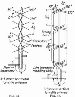
FIG. 47. FIG. 47. FIG. 48. FIG. 47.—Arrangement of the horizontal turnstile antenna for ultra-high frequencies.
