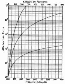
FIG. 26.—Attenuation of one, two, and three t-r-f circuits.
