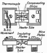
FIG. 6.—Compensated highfrequency thermocouple and heating element. the lugs themselves or temperature rise due to the total heat generated. The thermoelectric voltage is, therefore, strictly proportional to the temperature difference between the center and ends of the heated member which in turn is proportional to the square of the current causing this temperature rise, and a d-c instrument connected to the couple may be calibrated in terms of this current.
