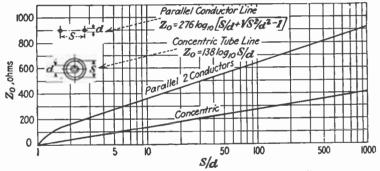
FIG. 78.--Impedance of parallel and concentric-tube lines.
