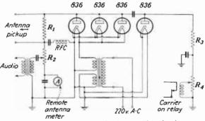
F1G. 47.—Antenna monitoring rectifier circuit.
