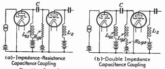
Fig. 11.-Impedance-capacitance coupled amplifier.
