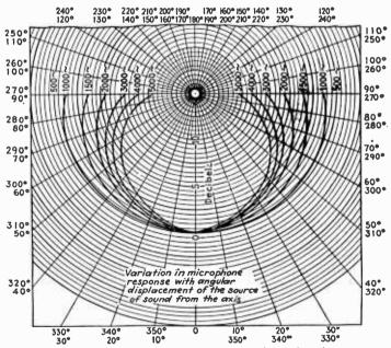
FIG. 17.—Directional characteristic of carbon microphone.
