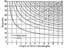
Fig. 14.—Angles at which nulls and maxima occur for the various patterns of Fig. 13.1
