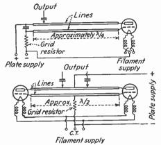
FIG. 27.—Ultra-high-frequency oscillators employing parallel lines as circuit elements.
