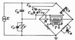
FIG. 48.-Schering bridge with guard circuit.
