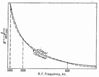
FIG. 35.-Closeness of tracking secured by formulas.
