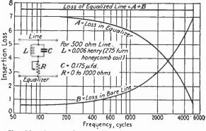
FIG. 55.—Attenuation equalizer for short cable circuits.
