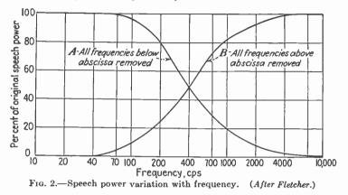
Articulation and naturalness are not to be confused. By successively raising the cutoff of high-pass filters and lowering the cutoff frequencies of low-pass filters, each by a barely perceptible amount, Schäfer has shown
