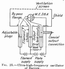
Special triodes in which the plate and grid leads provide support for the electrodes and extend through the bulb are especially useful for u-h-f work. A tube of this type having a rated output of 1.5 watts at 1,500 Me is available commercially.
