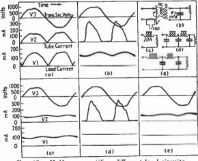
FIG. 18.-Half-wave rectifier, different load circuits.
