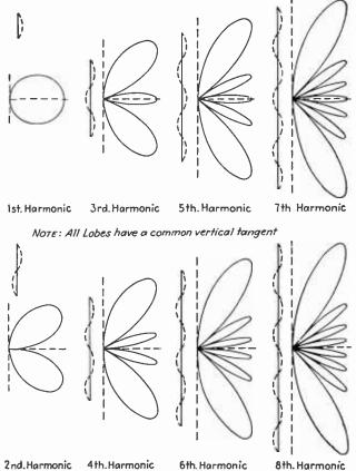
FIG. 13.—Polar diagrams of relative field strength distribution for straight wire antennas in free space with standing waves of current as shown, corresponding to the operation at various harmonics of the fundamental frequency of the antenna.
