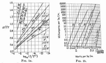
FIG. 1a.—Emission of coated filament compared to that from pure metals. (A.I.E.E. reprint.)
