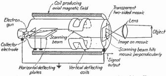
FIG. 15.—Structure of the orthiconoscope ("orthicon").
