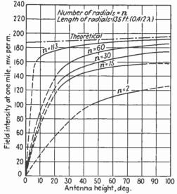
FIG. 23.--Variation of field intensity with antenna height and number of 0.412 wave length radials.
