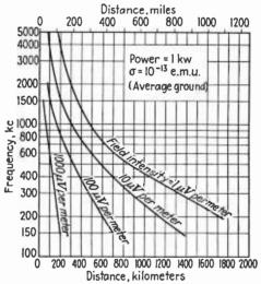
FIG. 1.—Ground-wave propagation over average ground; 1 kw, vertical 4 antenna. (Report of Committee on Radio Wave Propagation, Proc. I.R.E.,  $\lambda/4$  antenna. 26, 1193, October, 1938.)
