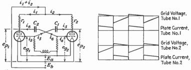
Fig. 18.—Fundamental circuit of the multivibrator and the voltage and current relations of the various branches.
