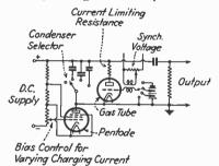
FIG. 22.—Relaxation oscillator employing a pentode to maintain a constant charging current.
