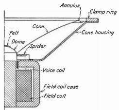
FIG. 24.—Sectional view of small moving-coil speaker showing structural simplicity.
