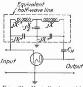
Fig. 24.—Neutralization with half-wave line.
