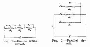
The equivalent resistance of a number of resistors connected in series is equal to the sum of the individual resistances. Referring to Fig. 1,  $E = iR_{\text{equiv.}} = e_1 + e_2 + \cdots + e_n = R_1 i + R_2 i + \cdots + R_n i = i(R_1 + R_2 + \cdots + R_n)$   $\frac{E}{i} = R_{\text{equiv.}} = (R_1 + R_2 + \cdots + R_n)$   $R_{\text{equiv.}} = \sum_{1}^{n} R$
