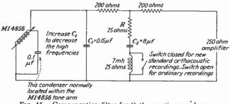
FIG. 45.-Compensation filter for Orthacoustic reproducer.
