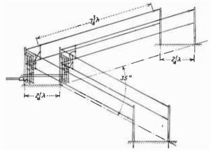
Fig. 38.—RCA model D antenna.
