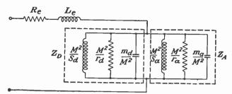
FIG. 25.—Equivalent 1-f electrical circuit of moving-coil or magneticarmature speaker in a total enclosure or in an infinite baffle. In the latter case the enclosure stiffness  $S_{a}$  is zero and its equivalent electrical inductance infinite.
