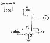
FIG. 17.—Circuit for measuring properties of insulators.
