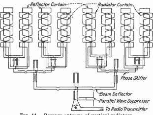
FIG. 44.-Barrage antenna of vertical radiators.
