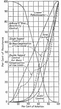
FIG. 11.—Taper curves of variable resistors.
