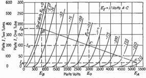
Fig. 60.-Method of determining modulator characteristics.
