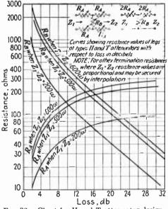
FIG. 32.—Chart for H and T attenuator design.
