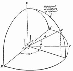
FIG. 21.-Geometry for calculating space characteristic of two-element array.
