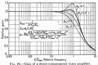
of  $C_t$ , at  $f_{\text{max}}$ . This is equivalent to making the resonant frequency between  $L_0$  and  $C_t$  equal to 1.41 times  $f_{\text{max}}$ .
