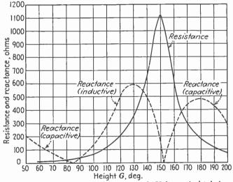
FIG. 28.—Measured resistance and reactance of 150-ft. vertical tubular mast antenna having a base insulator capacitance of 85  $\mu\mu f$ .
