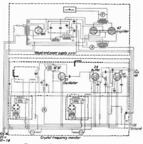
Fig. 50.—Circuit of frequency monitor.
