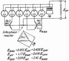
FIG. 9.—High-voltage supply for transmitter.
