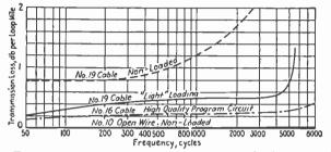
FIG. 53.—Transmission-loss characteristics of various audio-frequency circuits.
