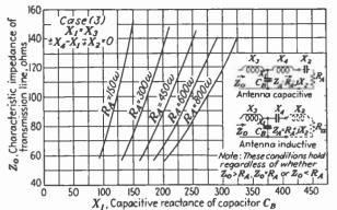
F10. 88.-Values of terminating reactors for case 3 when antenna reactance is compensated.
