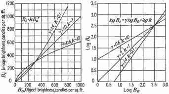
FIG. 64.-Brightness transfer characteristics of a television system.
