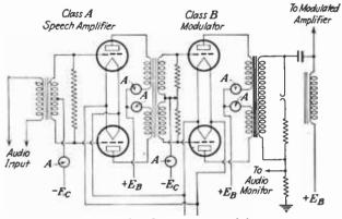
Fig. 62.—Class B push-pull modulator.
