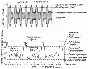
FIG. 9.—Top, modulated television carrier signal. Bottom, details of modulation envelope, according to R.M.A. recommended standard. According to the N.T.S.C. recommendations the black level is  $75 \pm 2.5$  per cent and the maximum white level 15 per cent or less.
