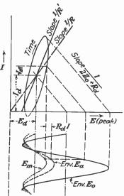
FIG. 23.—Diode detection with reactive load.
