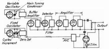
FIG. 15.-Block diagram of beat-frequency oscillator.
