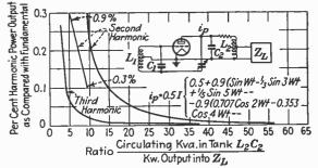
FIG. 76.—Effectiveness of high kilovolt-ampere to kilowatt ratio in reducing harmonic output with constant power output at fundamental.
