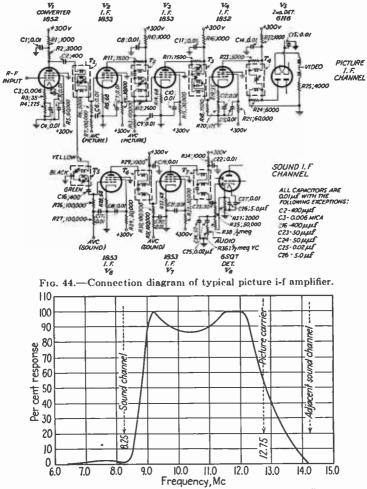
stage. A total i-f gain of 10,000 is usually considered sufficient. The effective tube and circuit noise at the input to the first i-f stage is usually 100  $\mu$ v
