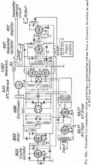
carrier or under full modulation. It also provides full frequency control over sufficient range to prevent the oscillator from drifting out of the control range.
