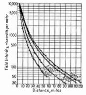
FIG. 3.—Average strength of daytime signals received in an airplane from 500-watt station on 1,510 kc. (Airplane at altitudes designated on graphs.)
