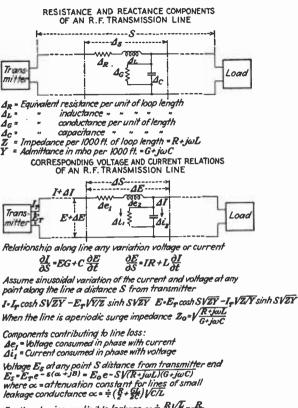
For lines having negligible leakage  $\alpha \doteqdot \frac{R}{2} \sqrt{\frac{L}{C}} = \frac{R}{2Z_{c}}$  $A = 4.343 \frac{R}{Z_0}$  decibels per unit length
