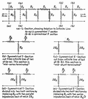
Fig. 61.—Equivalence of T and # networks.
