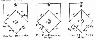
49. The resonance bridge shown in Fig. 53 is the simplest bridge in which inductance, capacitance, and frequency enter. At balance the arm containing the reactances is resonated to the applied frequency and becomes a pure resistance. The bridge is then an all-resistance equal-arm bridge. For this reason it may be used at high frequencies to measure the resistance and inductance of a reactor.
