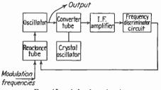
FIG. 45.—A-f-c f-m circuit.
