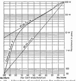
FIG. 12.—Advantage of special taper for volume control.
