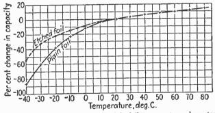
FIG. 8.-Comparison of etched- and plain-foil temperature characteristics.
