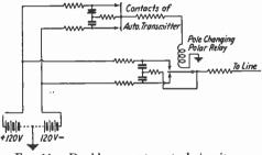
FIG. 11.—Double-current control circuits.
