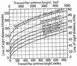
FIG. 10.-Length of line-of-sight path for various antenna heights.
