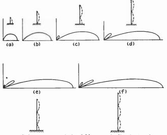
FIG. 16.—Polar patterns of the field strength distribution for vertical antenna over perfect earth when the currents in successive dipole sections are cophased. Note that minor lobes never exceed the horizontal tangent to the major lobe.
