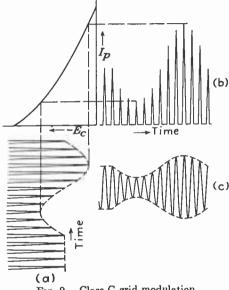
FIG. 9.-Class C grid modulation.
