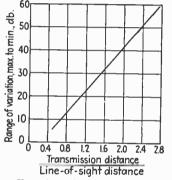
Fig. 18.—Ultra-high-frequency fading. Probable error in curve is  $\pm 10$  db.
