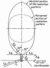
FIG. 50.-CAA cone-of-silence marker antenna system.
