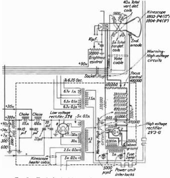
FIG. 3.-Typical television receiver power supply system.
