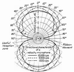
FIG. 7.-Directional characteristics of RCA velocity microphone.
