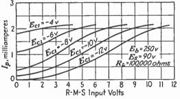
FIG. 28.-Load-rectification diagram of pentode.
