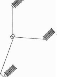
interconnected at the common gap (Fig. 58). Each pair of arms is made approximately of one-half wave length for the mean frequency of the band intended to be covered, although with a transmission line that matches the impedance of the doublet, either directly or through a matching device, the resonance is not critical.
