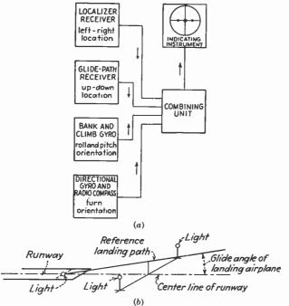
FIG. 23.—CAA-MIT microwave landing system: (a) combination of radio and airplane instrument indications; (b) three-light system on airport which gives equivalent visual indications.
