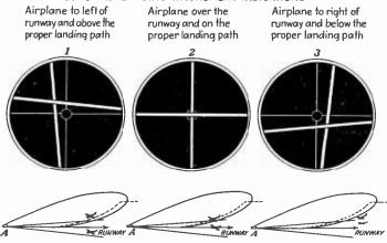
A=Landing beam and runway localizer beacon Fig. 20.—Combined-instrument indications for radio landing system.
