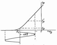
FIG. 25.—Vacuum-tube voltmeter characteristic.
