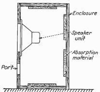
Fig. 28.—Bass reflex type of vented anclosure in which port area is large and placed near diaphragm to obtain maximum aid from mutual radiation resistance between diaphragm and port. Phase shift of back-side radiation obtained by choice of circuit constants.
