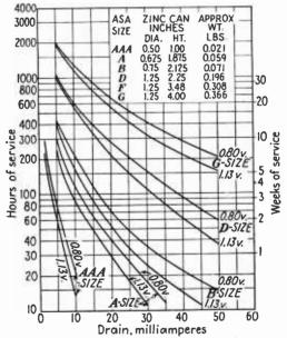
FIG. 10.—Radio-type dry cells; discharge versus time. Constant current, 6 hr. per day, 5 days per week to 1.13 volts and 0.80 volt per cell at 70°F.
