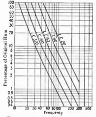
Fig. 31.—Smoothing effected by various products of inductance (henrys) and capacity (microfarads).
