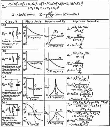
Equivalent impedances of parallel combinations of L, C, and R.
