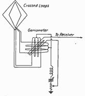
FIG. 9.—Loop-vertical antenna for directive reception.
