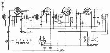
FIG. 33.-A-c-d-c receiver circuit.
