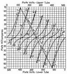
Fig. 23.—The composite characteristics of a push-pull amplifier.
