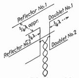
Fig. 59.—Television receiving antenna and reflection.
