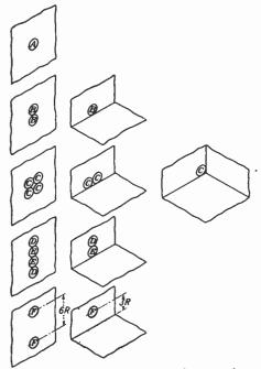
FIG. 14.—Effect of adding pistons and reflecting planes on radiation impedance. All pistons marked with the same letter see the same radiation impedance.
