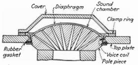
FIG. 19.—Cross section of a diaphragm and sound chamber in which concentric annular slots are used to reduce destructive sound chamber interference at high frequencies.
