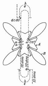
FIG. 49.-Schematic arrangement of wide-band television antenna developed for the Empire State Building.
