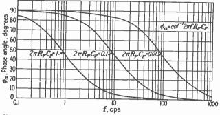
FIG. 32.—Phase response of low-frequency compensation system.
