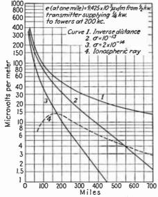
Fig. 1.—Field-intensity attenuation of 500-watt radio range-beacon station at 200 kc, 125-ft. towers.
