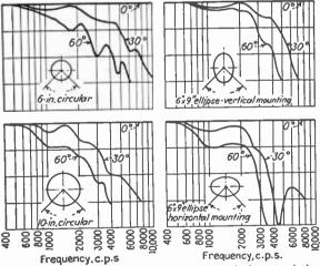
F10. 17b.—Experimentally determined directional characteristics for two circular and one elliptical diaphragms. The elliptical diaphragm has the broadest characteristic in the horizontal plane when its major (long) axis is vertical.
