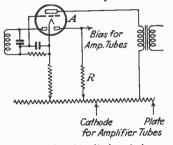
FIG. 18.—Double-diode triode as a-v-c. tube.
