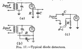
Diode current flows only for an instant at the peak of the carrier voltage in the forward direction. The pulses of current charge the load by-pass condenser to nearly the same voltage as the carrier envelope and bias the diode beyond cutoff except during the short pulses. Neglecting the slight h-f variation between pulses, the voltage across the load resistance is proportional to the carrier envelope.
