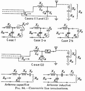
Case 2a. Antenna Impedance with Capacitive Reactance. Refer again to Fig. 84. It will be noted that the equivalent diagram for case 2a is the same as for case 1, except that the antenna impedance is now  $Z_A = R_A - jX_2$ . Then
