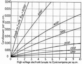
FIG. 55.—Phosphor light-output characteristic (type P4 phosphor).
