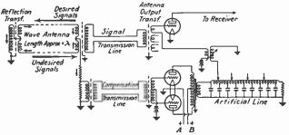
Fig. 8.—Wave antenna and output circuits.
