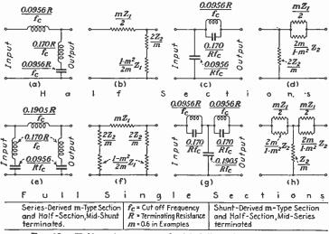
FIG. 63.—Half-section compared with full-section structures.
