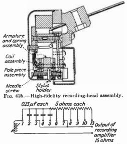
FIG. 43.—Circuit for correcting characteristic of recording head.
