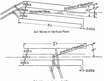
(b)-Wires in Horizonfal Plane F1G. 37.—RCA model B and C harmonic wire antennas.
