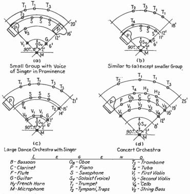
Fig. 22.—Orchestra arrangements for use with a single type 50A inductor microphone.
