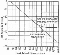
FIG. 44.—Frequency characteristics of audio system to convert phase modulation transmitter into f.m., and into pre-emphasized f.m.
