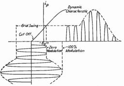
FIG. 23.—Characteristics of class B amplification.
