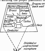
Figure 22 shows various arrangements of instruments and voices before the inductor or diaphragm type of microphone. The characteristic of this type permits the placement of the musical instruments within an area contained by an angle of 45 deg. on either side of the microphone axis. In using this type of instrument the source of sound, speaker, announcer, or
