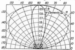
FIG. 15.—Vertical-plane radiation patterns of fan-ty<sub>b</sub>: marker: (a) in plane transverse to range-beacon course; (b) in plane parallel to range-beacon course.
