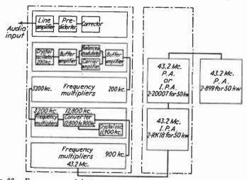
FIG. 66.—Frequency-modulation transmitter utilizing phase-shifting network.
