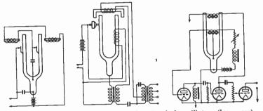
Fig. 32.—Circuits for various types of tuning-fork oscillators (hummers).
