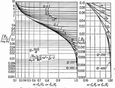
FIG. 26.-Design chart for series resonant circuit.
