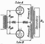
Fig. 22.—Schematic of a pushpull power amplifier.
