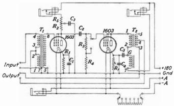
FIG. 34.-Microphone or preamplifier circuit.
