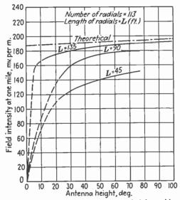
Fig. 24.—Variation of field intensity with antenna height and length of radials in a 113-wire ground system.
