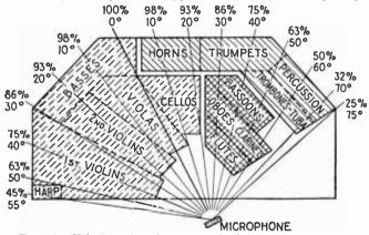
FIG. 24.-Velocity-microphone setup for large orchestra group.
