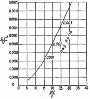
FIG. 46.—Typical reactor design curve; V in cubic centimeters and l in centimeters. Armco Radio 4.
