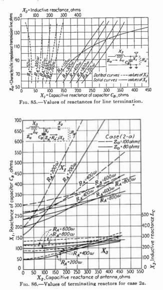
$$X_{1} = \frac{Z_{0}}{R_{A} - Z_{0}} \left[ -X_{2} \pm \sqrt{\frac{R_{A}}{Z_{0}}(R_{A}^{2} + X_{2}^{2} - Z_{0}R_{A}} \right]$$
