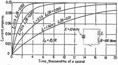
FIG. 1.-Rise of current in inductive circuit.
