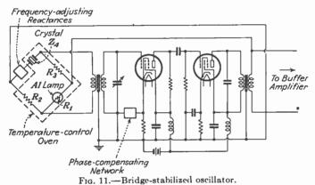
**13. Bridge Stabilization.** The bridge-stabilized oscillator was developed by L. A. Meacham<sup>1</sup> and is a constant-frequency oscillator of extremely high selectivity. Short-time frequency variations no greater
