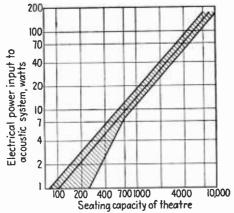
FIG. 37.—Recommended amplifier output for motion-picture reproduction. Speaker system efficiency assumed to be 25 per cent so acoustic input to theater is one quarter indicated electrical input. Trend is toward higher values.
