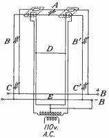
Fig. 26.—Ultra-high-frequency oscillator of King.
