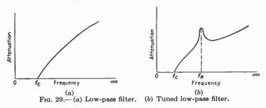
classes, tuned and untuned filters. The tuned filter offers a maximum impedance or attenuation to the frequency of the supply, but the impedance at near-by higher or lower frequencies is not quite so great (see
