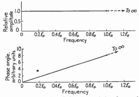
FIG. 11.-Ideal amplitude and phase transmission characteristics.
