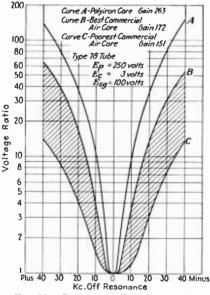
FIG. 22.-Iron-core coil characteristics.
