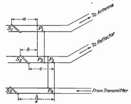
FIG. 46.-Transformer made up of transmission-line section.
