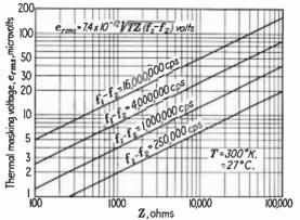
44. Noise Limitations to Video Amplification. One of the principal limitations to proper video amplification is inadequate signal/noise
