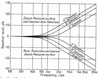
FIG. 17.—Effect of concentration of radiation on piston axis at high frequencies for the case of pistons radiating constant *total* power (top curves) and the case of constant pressure response on the axis (lower curves). Because of cone flexing the concentration is less marked in actual diaphragms where the equivalent piston diameter at high frequencies approaches about sixtenths the actual cone diameter.
