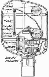
FIG. 12.—Simplified cross-sectional view of the cardiod directional microphone.
