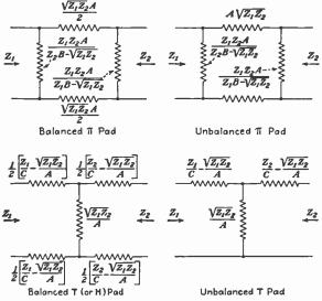
FIG. 58b.-Pads to be used between unequal impedances.
