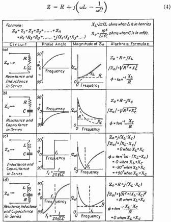
Equivalent impedances of series combinations of L, C, and R.
