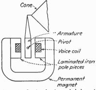
FIG. 26.—Sectional view of balanced armature magnetic speaker.
