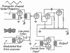
FIG. 8.—Schematic diagram of transmitting converter for CFVD.
