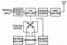
FIG. 66b.-Frequency stabilizing system of Western Electric.
