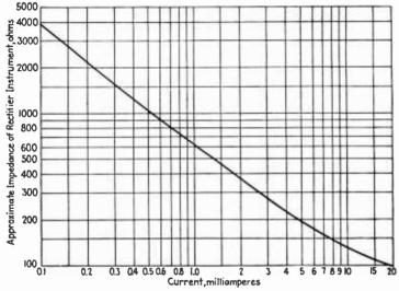
Fig. 11.-Impedance characteristic.
