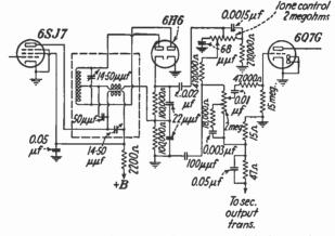
FIG. 34 .- Balanced detector for frequency modulation receiver.
