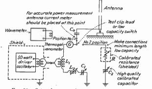
FIG. 90.—Setup for measuring antenna characteristics.
