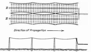
FIG. 55.—Double broadside Beverage antenna.
