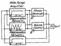
FIG. 17.—Block diagram of resistancecapacity audio oscillator. ously impractical.
