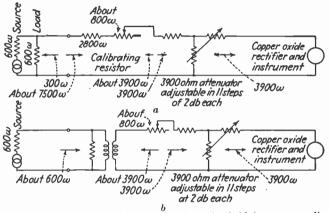
FIG. 33.—Standard volume-indicator circuit, a, for bridging across a line; b, low-impedance arrangement such as line termination.
