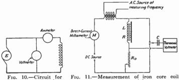
rig. 10.—Circuit for rig. 11.—Measurement of fion cor measurement of inductance.
