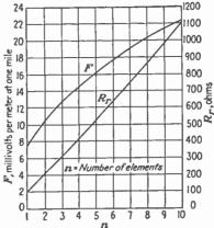
FIG. 6.—Radiation resistance at current antinode and field intensity at 1 mile radiated for a vertical array of colinear cophased dipoles.<sup>1</sup>
