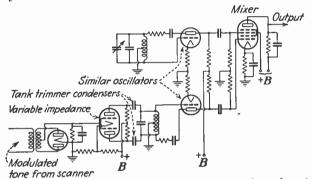
FIG. 9.—Schematic diagram of transmitting converter for subcarrier f-m method.
