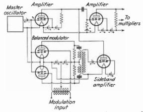
FIG. 65.—Schematic diagram of Armstrong frequency modulator.
