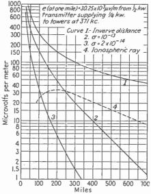
Fig. 2.—Field-intensity attenuation of 500-watt radio range-beacon station at 371 ke, 125-ft. towers.
