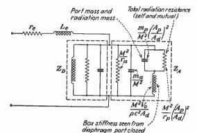
FIG. 29.—Equivalent l-f electrical circuit of moving-coil or magnetic-armature speaker in vented enclosure.
