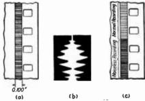
F1G. 35.—(a) Variable-density sound track produced by light-valve ribbons or glow lamp; (b) variable-area noiseless track produced by vibrating mirror; (c) noiseless recording showing greater density during periods of low modulation.
