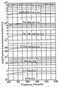
Fig. 23.—Voltage gain in superheterodyne receiver.
