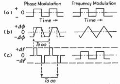
FIG. 4.-Comparison of phase and frequency modulation.
