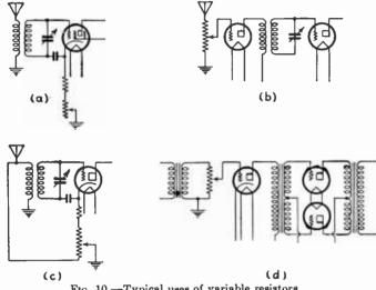
FIG. 10.-Typical uses of variable resistors.
