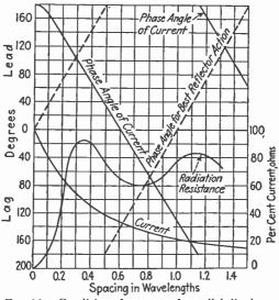
FIG. 12.-Conditions for array of parallel dipoles.
