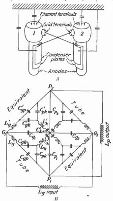
FIG. 28.-Wide-band, "complete," neutralizing. A shows the mechanical arrangement; B, the equivalent circuit. The condenser plates are adjustable.
