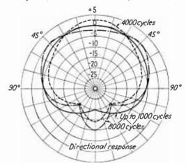
FIG. 11.-RCA 77B unidirectional microphone characteristics.
