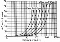
FIG. 17.---Voltage-doubler characteristics for receiver circuits.
