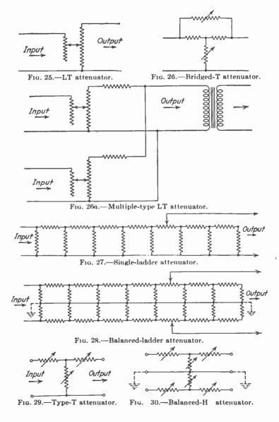
as in Fig. 26a, sufficient resistance is inserted in one output lead from each attenuator to maintain correct circuit matching. The bridged-T structure shown in Fig. 26 is used extensively for the same purposes.
