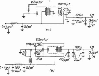
FIG. 31.—B-supply systems for automobile receivers.
