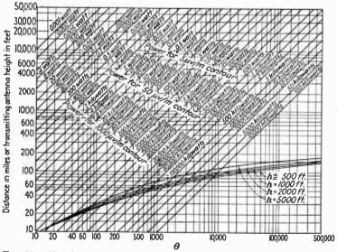
FIG. 98.—Signal range for high-frequency broadcast stations. (f = 46 Mc;  $\sigma = 5 \times 10^{-14}$  e.m.u.; dielectric constant  $\epsilon = 15$ .)
