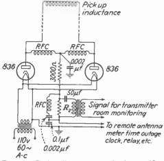
FIG. 48.—Push-pull antenna monitoring rectifier.
