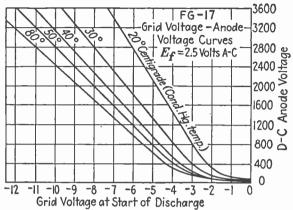
Fig. 36.—Typical mercury-vapor grid-controlled rectifier characteristics.
