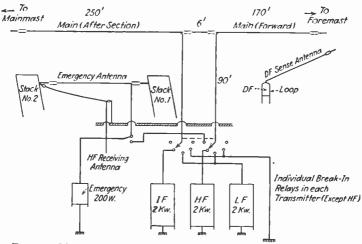
FIG. 31.-Marine antennas (SS. "Washington" and SS. "Manhattan").
