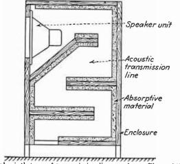
FIG. 32.—Labyrinth type of transmission-line speaker. Phase shift of backside radiation obtained by time of transmission delay in line.
