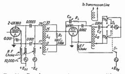
FIG. 21.—Broadcast transmitter power amplifier.
