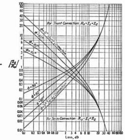
Fig. 23.—Transmission loss due to insertion of shunt or series impedance. The series impedance can usually be inserted at a point in the circuit where the impedances  $Z_1$  and  $Z_2$  are matched and where each is substantially a pure
