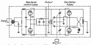
FIG. 66a .- Essential circuits of Western Electric f-m transmitter.
