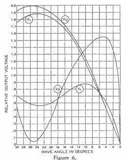
VERTICAL - PLANE DIRECTIONAL CHARACTERISTICS OF HORIZONTAL AND VERTICAL DOUBLETS ELEVATED 0.6 WAVE-LENGTH AND ABOVE TWO TYPES OF GROUND.
