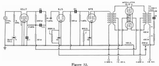
45-WATT BEAM-TUBE MODULATOR WITH DEGENERATIVE FEEDBACK.
