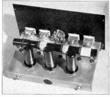
possibly for the incorporation of fixed battery bias. A standard duty 45-volt bias battery costs no more than cathode resistors and bypass condensers for the three stages, will last for at least 2 years, and permits better oscillator keying.
