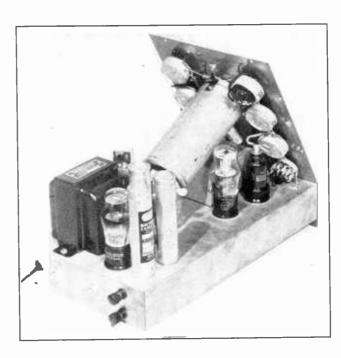
Construction. The galvanized iron pipe seen in Figure 53 acts as a shield over the c.r. tube, greatly reducing both inductive and electrostatic pickup of a.c. ripple. The pipe is just sufficiently large to take the tube. Further
