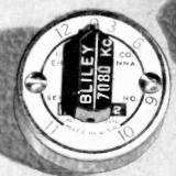
40-80 METERS VARIABLE FREQUENCY TYPE VF1
