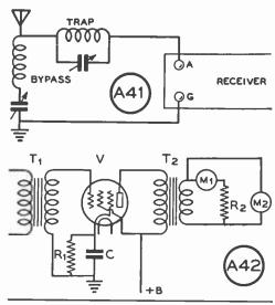
cast reception consisting of a series-tuned circuit connected in shunt with the b.c. receiver input to bypass the interfering signal and a parallel-tuned (trap) circuit in series with the receiver input to reject the interfering signal.
