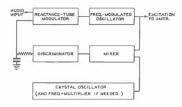
Figure 11. DISCRIMINATOR STABILIZING ARRANGEMENT.
