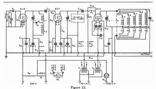
WIRING DIAGRAM OF BANDSWITCHING 814 EXCITER.
