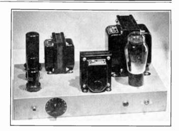
so as to present a plate-to-plate load of 4000 ohms to the T-21 tubes, with the value of secondary load into which the tubes are working. Maximum output and maximum modulating ability, with minimum harmonic distortion, will be obtained from the amplifier under these operating conditions.
