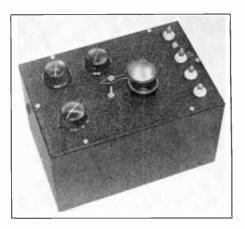
Figure 49. CATHODE RAY MODULATION CHECKER.
