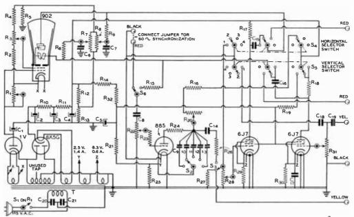
R<sub>1</sub>-25,000 - o h m potentiometer with a.c. line switch R<sub>2</sub>-25,000 ohms, 1/2 watt R<sub>3</sub>-50,000 - o h m potentiometer R<sub>4</sub>, R<sub>5</sub> — 100,000 ohms, 1 watt R<sub>1</sub>-2 megohms, ½ watt R<sub>7</sub>, R<sub>8</sub> — 100,000ohm potentiometers R<sub>0</sub>-4 megohms, ½ watt R<sub>10</sub>, R<sub>11</sub> — 2500 ohms, 1 watt R<sub>12</sub>-250,000 ohms, 1 watt R<sub>13</sub>—50,000 ohms,
