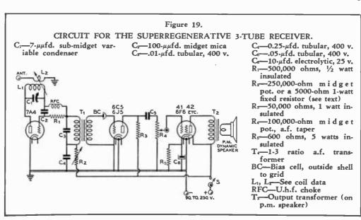
condenser goes to the grid and the stator to the plate. A bakelite or hard rubber shaft extension must be used with the tuning condenser in order to prevent body capacity detuning effects. As an alternative, an insulated coupler may be used in conjunction with a short piece of metal shafting and a panel bearing. Both r.f. choke and grid leak should be connected with the shortest possible leads to the r.f. circuit.
