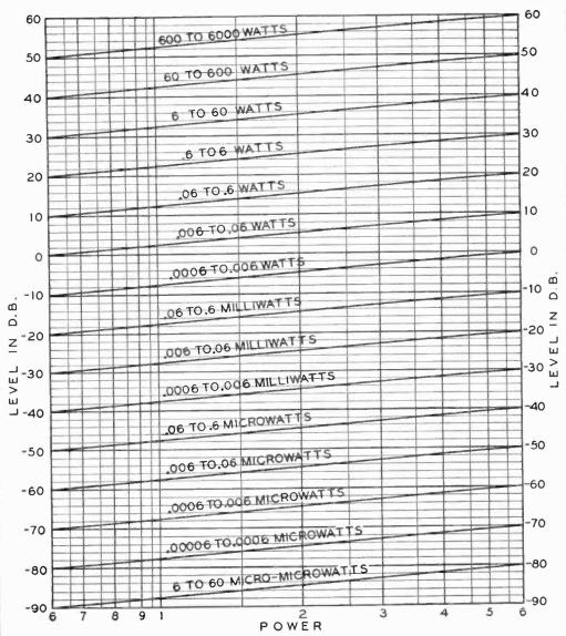
Based on .006 walls at zero level.
