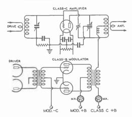
Figure 13. CLASS B PLATE MODULATION.
