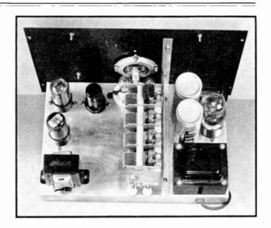
quite noticeable on the lowest frequency scale, where the oscillator and its harmonics will tend to lock in with the various harmonics of the a.c. line frequency. For this reason, it is important that the oscillator be operated only when it is thoroughly enclosed in its shielding cabinet.
