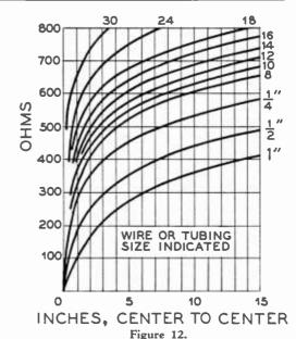
CONDUCTOR SIZE AND SPACING VERSUS SURGE IMPEDANCE FOR TWO-WIRE OPEN LINE OR MATCHING TRANSFORMER.
