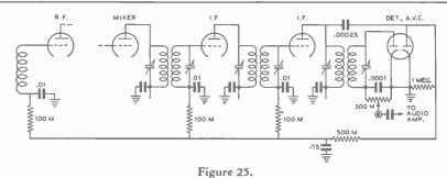
DOUBLE-DIODE DETECTOR-A. V. C. CIRCUIT.
