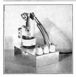
Figure 9. 8-WATT HY-75 224-MC. OSCILLATOR.
