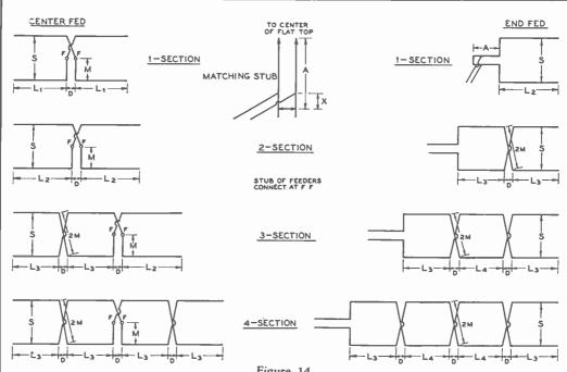
Figure 14. FLAT-TOP BEAM DESIGN DATA.
