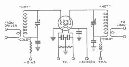
Figure 36. LINK COUPLED CIRCUIT.
