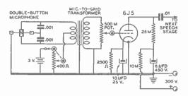
Figure 21. SPEECH AMPLIFIER CIRCUIT FOR WITH A DOUBLE-BUTTON USE MICROPHONE.
