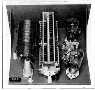
To eliminate the need for a more bulky, higher capacity plate tank condenser for 160-meter operation, which would not be advisable for 10-meter operation due to the high minimum capacity, the following expedient is resorted to: the 75-meter amplifier plate coil is made slightly lower Q than optimum. The same coil is then used on 160 meters by shanting a fixed vacuum padding condenser of 50- $\mu\mu$ fd. capacity across the tank tuning con-
