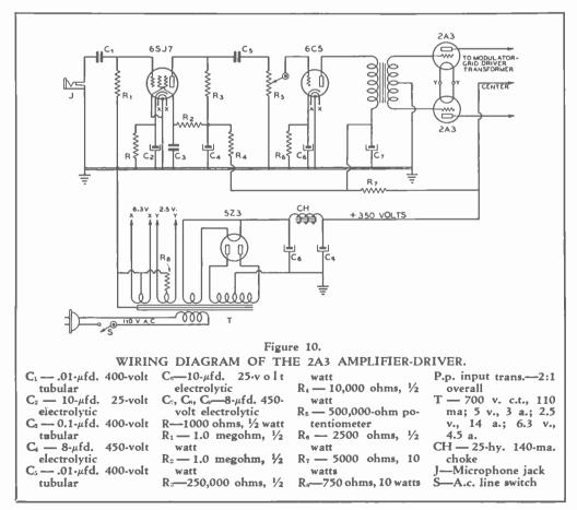
tubes are a pair of 2A3's, operating with a self-bias resistor in their common filament return. Operating in this manner, the 2A3's have an undistorted output of approximately 10 watts.
