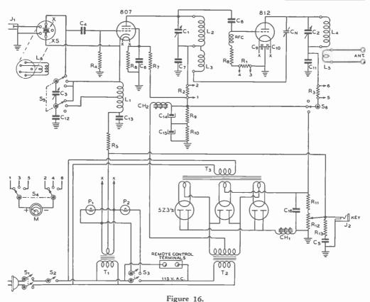
SCHEMATIC DIAGRAM OF 150-WATT C.W. TRANSMITTER.
