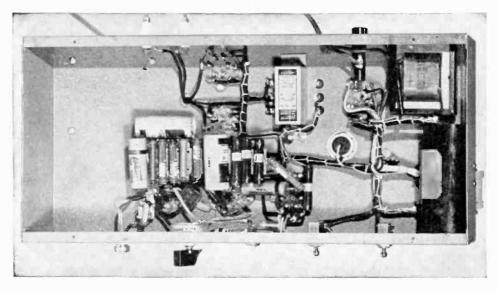
3. This modulator is simple and inexpensive to construct, and will plate modulate inputs of 40 to 60 watts on voice with excellent quality; the maximum output of the modulator, with voice frequency input and tolerable harmonic distortion, is about 25 watts.
