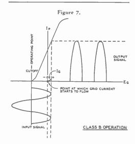
the voltage drop across this load will constantly change because the plate current is constantly changing. The actual value of voltage on the plate will vary in accordance with the IZ drop across the load, even though a steady value of direct current may be applied to the load impedance; hence, for an alternating voltage on the grid of the tube, there will be a constant change in the voltage at the anode.
