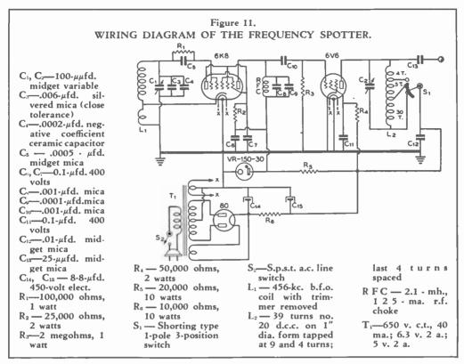
zero beat. If the second b.c. station is not at zero beat or within a few cycles of it, the oscillator definitely isn't on 50 kc. and the frequency will have to be rechecked by the procedure given in the preceding paragraphs, fixed condensers being added or subtracted, depending on whether the frequency is high or low.
