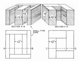
Figure 39. TYPES OF TRANSFORMER CORES.
