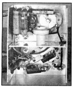
Figure 20. UNDER THE CRYSTAL FILTER CHASSIS. Note the shield between the input and output sections of the filter. The input section is at the bottom, the output circuits at the top, in this view. The bypass condensers for the 6SK7 are placed across the tube socket to help prevent oscillation from capacity coupling between the grid and plate.
