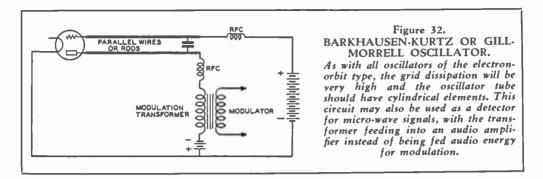
1.4 v. series. They are satisfactory for low-power transmitters and superregenerative receivers. The regenerative circuits are quite similar to those for longer wavelengths, except for the physical size of condensers and coils. The tube element spacing in these acorn tubes is made so small that electron transit time becomes a negligible factor for wavelengths above 0.6 meter.
