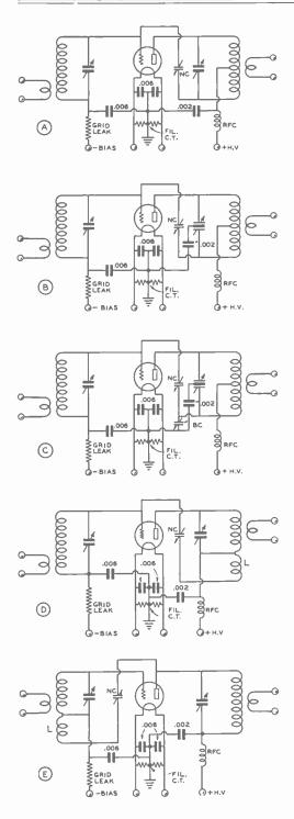
feedback may be eliminated: the first, and the most common method, is through the use of a capacity bridge, and the second method is through the use of a parallel reactance of equal and opposite polarity to the grid-to-plate capacity, to nullify the effect of this capacity.
