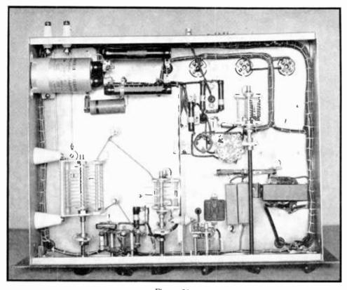
Figure 21. UNDER-CHASSIS VIEW OF 150-WATT C.W. TRANSMITTER.
