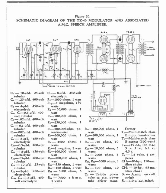
oughly shielded to prevent grid hum, and to reduce the possibility of either r.f. or audio feedback.
