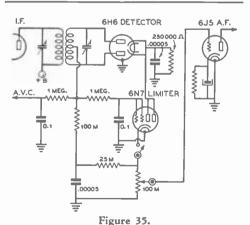
DICKERT AUTOMATIC LIMITER. This limiter will automatically adjust itself to various amounts of carrier strength.
