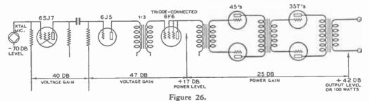
CALCULATION OF THE GAIN OF THE AUDIO CHANNEL OF A RADIOPHONE TRANSMITTER.
