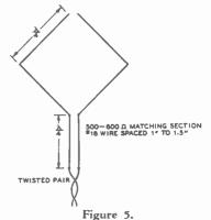
D.F. ANTENNA SYSTEM FOR U.H.F. In effect the antenna compares to two vertical close-spaced dipoles 180 degrees out of phase.
