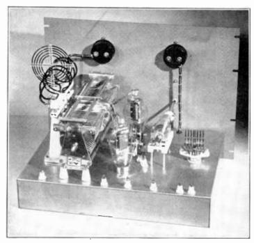
the excitation is removed. This arrangement allows the exciter to be keyed in the crystal oscillator stage without danger of damaging the final amplifier tubes. It also obviates the necessity for lowering the final amplifier plate voltage when the transmitter is being tuned, since there will always be sufficient bias on the 812's regardless of whether they are receiving grid excitation or not.
