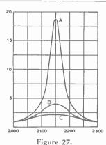
Resonance curve showing the effect of resistance upon the selectivity of a tuned circuit.
