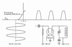
CLASS C AMPLIFIER PLATE CURRENT WAVEFORM
