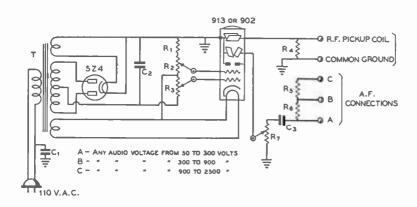
Ci-.01-µfd. tubular C2 - 1-µfd. 1000 volts w.v. C.—.01-µfd. mica. 5000 volts R<sub>1</sub>-150,000 ohms. 1 watt R2-50,000 - o h m potentiometer R -- 25,000 - o h m potentiometer R-5 meg., 1 watt Ro-6 meg., 6 watts (see text) R<sub>6</sub>-2 meg., 2 watts (see text) R-1-meg. pot. T-350 v. each side c.t., 40 ma.
