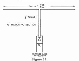
METHOD OF FEEDING A HALF-WAVE RADIATOR BY MEANS OF Q BARS. REFER TO TABLES FOR DIMENSIONS.
