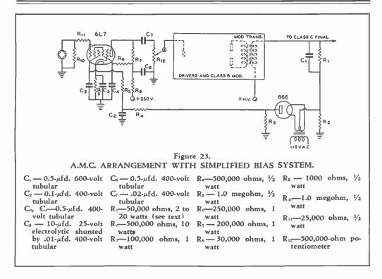
18. All this speech amplifier requires is a half-wave rectifier. The same voltage ratings apply for this rectifier as for the one just described, with the c.t. of its filament connected directly to the plate voltage lead to the plate modulated stage, and the plate connected to the input terminal on the amplifier.
