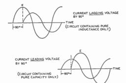
Figure 24. The above two illustrations show the manner in which a pure inductance or a pure capacitance (no resistance component in either) will cause the current in the cir-
