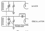
Figure 16. OSCILLATOR SERIES TRACKING CONDENSER ARRANGEMENT. The series condenser allows the oscillator to have a slower rate of capacity change than the mixer.
