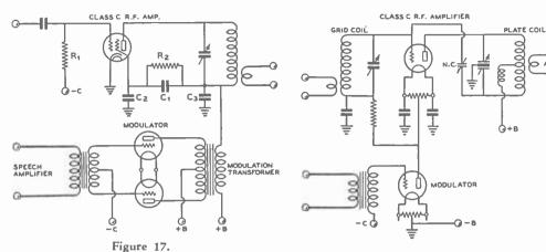
PLATE AND **SCREEN** MODULA-TION OF AN R.F. STAGE.
