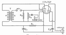
Figure 34. A.C. OPERATED AUDIO OSCILLATOR.
