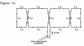
HORIZONTALLY POLARIZED BROADSIDE BARRAGE ANTENNAS
