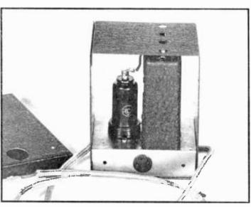
heater type tube is used to minimize the additional drain placed on the power transformer. As the plate current drawn by the tube is only a few ma., there is no need to fear there being an unduly heavy load placed on the power pack. The unit is quite compact, and will even fit inside the cabinet of some receivers. Where it will not, it may be attached to the outside rear of the receiver cabinet by means of brackets.
