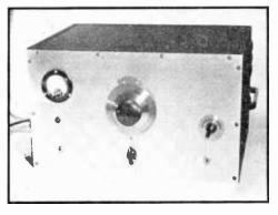
Figure 9. 20-25 WATT V.F.O. FOR 20, 40, AND 80 METERS.
