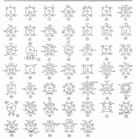
TRANSMITTING TUBE SOCKET CONNECTIONS—BOTTOM VIEWS.
