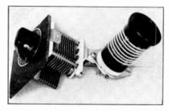
Figure 4. SIMPLE ABSORPTION TYPE WAVEMETER. The meter is merely a calibrated tank cir-
