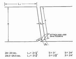
SL= 12" OR 2" FOR 112 MC. 2" OR 4" FOR 36 MC. 4" FOR 28 MC. 4" OR 8" FOR 14 MC. THIS ARRAY MAY BE USED ON HALF (NOT TWICE) FREQUENCY WITH GOOD RESULTS. NO CHANGES ARE REQUIRED.
