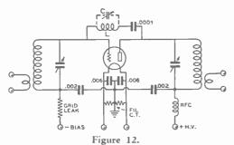
SHUNT OR "COIL" NEUTRALIZATION.
