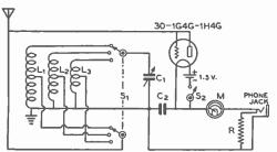
Figure 31. WIRING DIAGRAM OF THE 'PHONE TEST SET.
