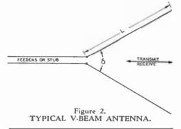
the lobes of radiation from the two long-wire antennas aid each other to form a bidirectional beam. Each wire by itself would have a radiation pattern similar to that for antennas operated on harmonics. The reaction of one upon the other removes two of the four main lobes, and increases the other two in such a way as to form two lobes of still greater magnitude.
