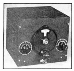
Figure 12. THE 6K8-6J5 CONVERTER IN ITS CABINET.
