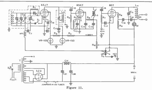
SCHEMATIC DIAGRAM OF 25-WATT V.F.O. UNIT.
