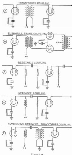
Figure 8. COMMON FIVE **METHODS** AUDIO-FREQUENCY INTERSTAGE COUPLING.
