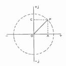
Figure 18. ROTATING VECTOR DIAGRAM.
