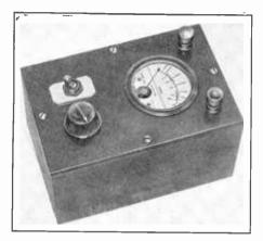
Figure 2. LOW RANGE OHMMETER. This ohmmeter is particularly useful for measuring resistances too low to be read accurately on an ohmmeter of the type illustrated in Figure 1.
