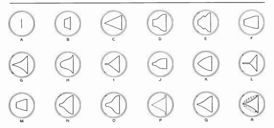
Figure 51. TYPICAL OSCILLOGRAPHIC MODULATION PATTERNS.
