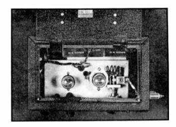
the coil are all placed as close together as possible to provide the shortest possible leads. The coil is soldered directly to the condenser term:nals. The "hot" lead wire on each r.f.
