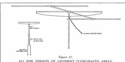
ALL PIPE VERSION OF 3-ELEMENT CLOSE-SPACED ARRAY.
