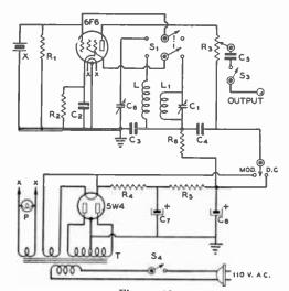
Figure 13. WIRING DIAGRAM OF CRYSTAL CALIBRATOR.
