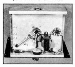
3500- to 4100-kc. range is covered in two jumps (two settings of the bandset condenser). This spreads out the frequency divisions and makes closer readings possible.
