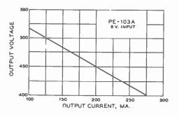
Figure 5. OUTPUT VOLTAGE VS. LOAD CUR-RENT FOR A PE-103A DYNAMOTOR POWER UNIT (APPROXIMATE).
