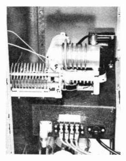
Figure 6. SHOWING THE 4-65A AMPLIFIER INSTALLED IN THE TRANSMITTER.
