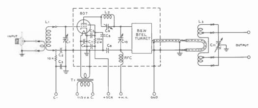
Figure 4. SCHEMATIC OF THE SHIELDED 807 AMPLIFIER.
