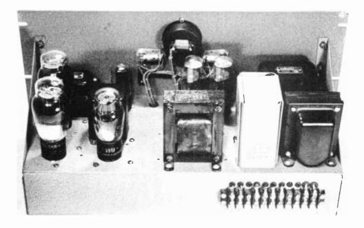
Figure 16. REAR VIEW OF THE VARIABLE-VOLTAGE POWER SUPPLY.
