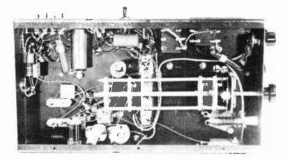
Figure 20. 807 MOBILE TRANSMITTER UNDERCHASSIS. The band-selector switch can be seen along the center of the chassis. The second section from the front of the bandswitch is not in use, but could be connected into the antenna circuit so that a single coaxial output connector could be used.
