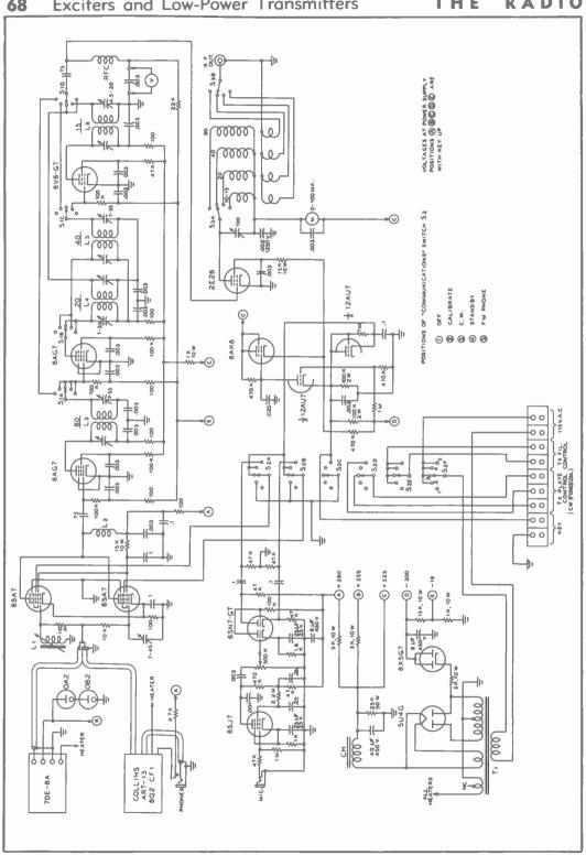
Le-Two coils 8 turns no. 18 engm. closewound on XR-2, separated 1/2" S--Assemble from Centralab Switchkit, with four
