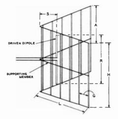
Figure 14. CORNER-REFLECTOR ANTENNA CONSTRUCTION.
