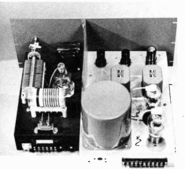
Figure 4. LOOKING DOWN ON THE MODULATOR AND FINAL AMPLIFIER.
