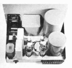
Figure 7. TOP OF THE TRANSMITTER MAIN POWER SUPPLY.
