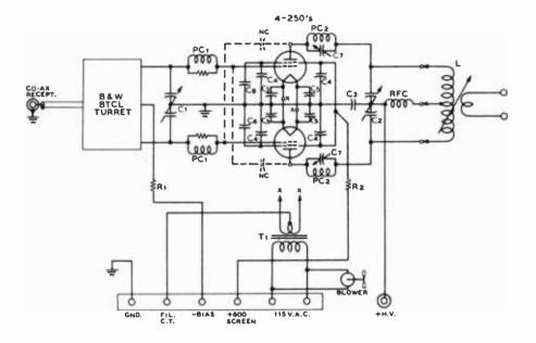
Figure 28. SCHEMATIC OF THE 4-250A AMPLIFIER.
