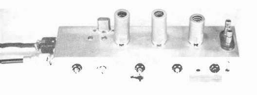
Figure 12. TOP VIEW OF THE CRYSTAL-CONTROLLED CONVERTER.
