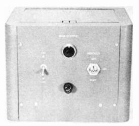
Figure 33. CONTROL BOX FOR THE ROTARY ANTENNA SYSTEM. antenna control system. The installation uses the common propeller pitch-change motor as the driving motor and reduction gear. A pair of 115-volt synchros (Selsyns) repeat back antenna position information to the operating position.
