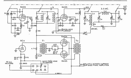
Figure 16. SCHEMATIC DIAGRAM OF THE 10/75 METER MOBILE TRANSMITTER.
