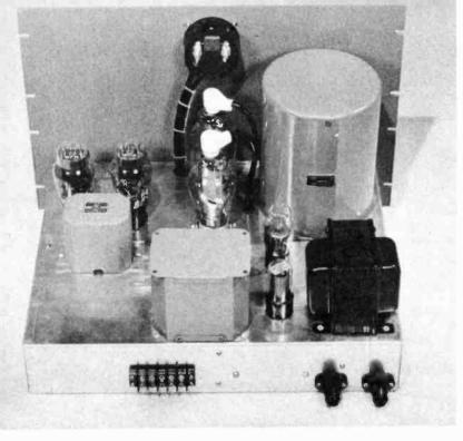
Figure 21. REAR VIEW OF THE MODULATOR CHASSIS.
