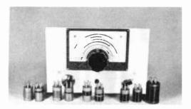
,Figure 5. FRONT OF THE SUPERHET CONVERTER, SHOWING ALL COILS.
