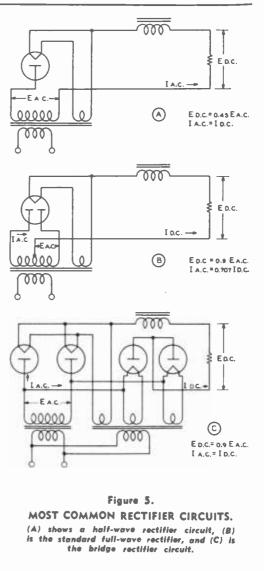
rating of the rectifier tube seldom will be exceeded.
