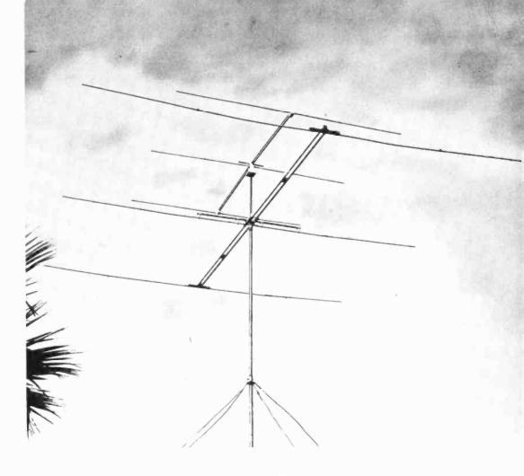
Figure 20. LIGHTWEIGHT STACKED 28-MC. AND 50-MC. ANTENNA ARRAY. Both antennas are supported by a lightweight rotating mast structure. The twa coaxial feed lines for the antennas pass down the rotating support pipe to the operating position.
