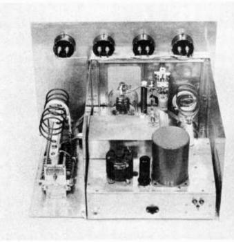
Figure 31. REAR OF THE SHIELDED KILOWATT WITH COVER REMOVED. The various components which go to make up the amplifier may be seen clearly in this photograph.
