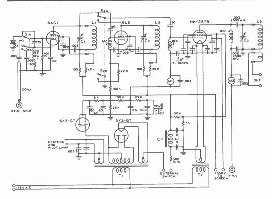
Figure 31. SCHEMATIC OF THE 4E27/257B TRANSMITTER.
