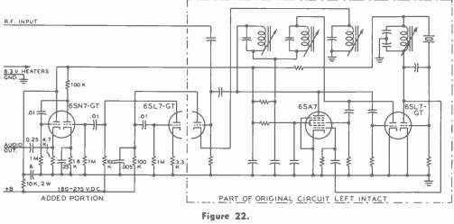
SCHEMATIC OF THE MODIFIED 8Q2 CRYSTAL CALIBRATOR UNIT.
