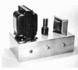
Figure 12. TOP VIEW OF THE 350-VOLT 110-MA. POWER SUPPLY.
