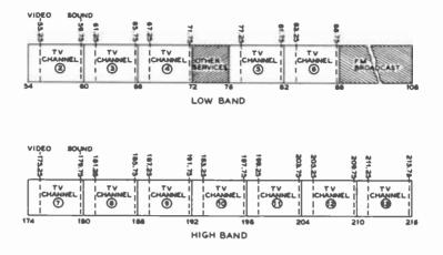
Figure 5. FREQUENCIES OF THE TV CHANNELS. Indicated are the frequencies of TV channels 2 through 13, with both the video and sound carrier frequencies shown.
