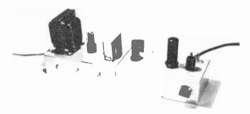
Figure 1. FRONT OF THE SIMPLE TWO-TUBE TRANSMITTER. The associated power supply unit from Chapter Eight is shown alongside the transmitter r-f unit.
