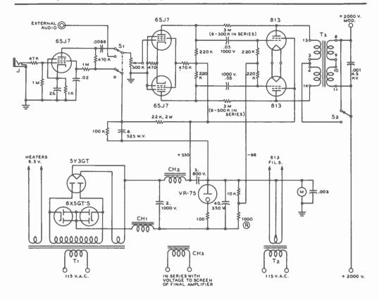
Figure 26. SCHEMATIC OF THE 200-WATT 813 MODULATOR.
