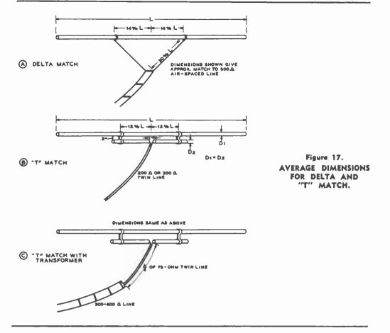
folded-element or yoke matching system with different sizes of conductors or different spacings than those shown on figure 16. Note, then, that the impedance transformation ratio of these types of matching systems is dependent both upon the ratio of conductor diameters and upon their spacing. The following equation has been given by Roberts (RCA Review, June, 1947) for the determination of the impedance transformation when using different diameters in the two sections of a folded element:
