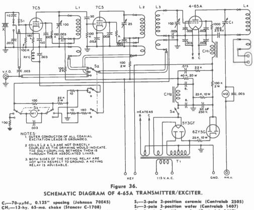
C<sub>1</sub>—70-µµfd., 0.125" spacing (Johnson 70145) CH<sub>1</sub>—13-hy. 65-ma. choke (Stancor C-1708) CH<sub>2</sub>—10.5-hy. 110-ma. choke (Stancor C-1001) L1, L2, L3, L4, L4 M1,—0-10 d.c. milliammeter (Marion 535N) M2—0-250 d.c. milliammeter (Marion 535N) S1--2-pole 2-position ceramic (Centralab 2505) S2--3-pole 3-position wafer (Centralab 1407) S3--3-pole 3-position wafer (Centralab 1407) S---S.p.s.t. toggle switch (H&H) T1--700 c.t. 120 ma., 5 v. 3 a., 6.3 v. 4.7 c. (Stancor P-6013)
