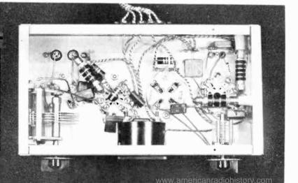
Figure 5. UNDERCHASSIS OF THE ALL-BAND R-F UNIT.
