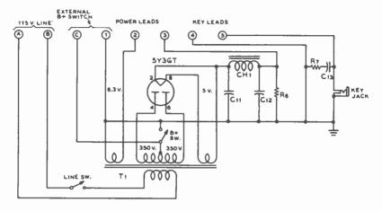
Figure 14. SCHEMATIC OF THE 350-VOLT SUPPLY.
