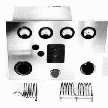
Figure 29. FRONT VIEW OF THE SHIELDED KILOWATT AMPLIFIER. The 14-Mc. coils for L, and Ly can be seen in front of the amplifier.
