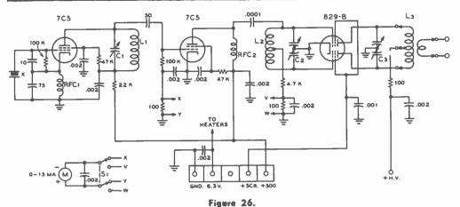
SCHEMATIC OF THE 8298 TRANSMITTER.
