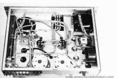
Figure 8. MAIN POWER SUPPLY UNDERCHASSIS.
