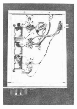
Figure 22. UNDERCHASSIS OF THE CONVERTER. The unit is connected for the 50 to 230 Mc. range in this photo.
