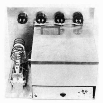
Figure 30. REAR OF THE SHIELDED KILOWATT WITH COVER IN PLACE.
