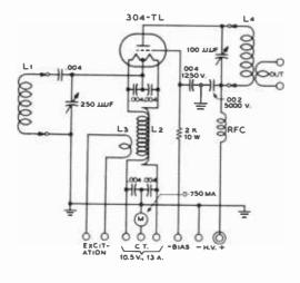
coil serves in itself to tune to resonance with the 250 µµfd. tuning capacitor. For operation on the higher frequency bands it is necessary to parallel the filament coil with additional inductors to reduce the effective inductance. However, it was found sufficient to couple the excitation link into the cathode coil only for all bands. This is illustrated on the schematic.
