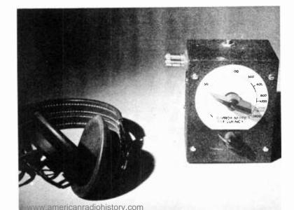
Figure 3. THE MINIATURE AUDIO OSCILLATOR A standard pair of hea phones is shown alongsi for size comparison.
