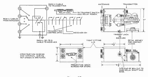
Figure 17. SCHEMATIC AND SKETCH OF THE CONTROL RELAY AND ANTENNA SELECTOR.
