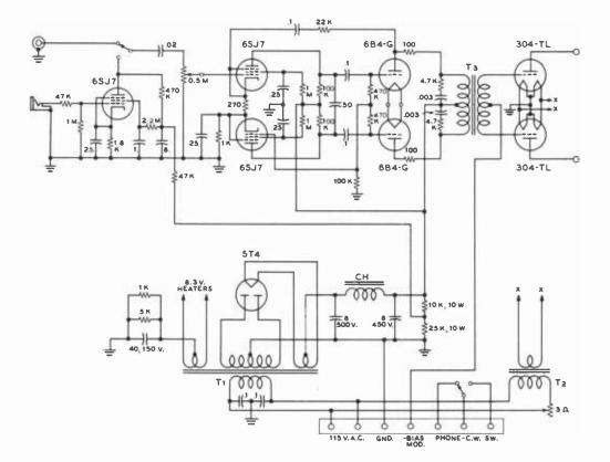
Figure 32. SCHEMATIC OF THE HIGH-POWER MODULATOR.
