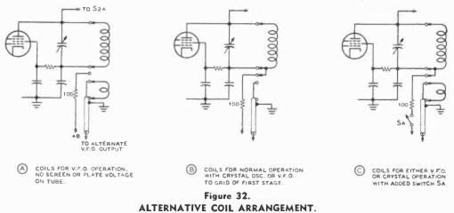
The use of this coil arrangement in place of that shown in figure 31 permits the feeding of an external v.f.o. directly into the grid of the 4E27/257B final stage. The circuit requires changes in the plate and screen returns of both the 6AG7 and 6L6 stages, plus the substitution of five-prong coil forms. The additional arrangement shown at (C) permits the use of links on all coils but requires the addition of a switch in series with the plate voltage supply for the 6AG7 stage.
