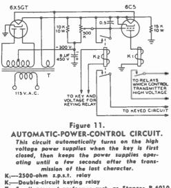
T—Small power transformer such as Stancor P-6010 furnishing 650 v. c.t. at 40 ma., 6.3 v. at 2 a., and a 5-volt winding which is not used.
