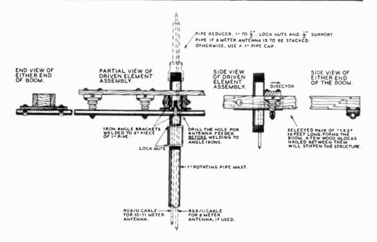
Figure 21. CONSTRUCTIONAL DETAILS OF THE LIGHTWEIGHT ARRAY.
