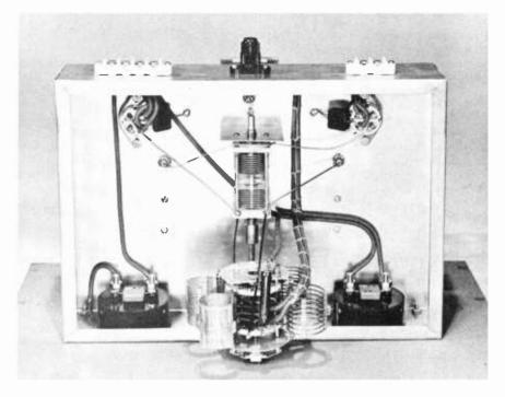
Figure 13. PUSH-PULL GENERAL-PURPOSE AMPLIFIER, UNDERCHASSIS.
