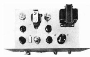
Figure 12. LOOKING DOWN UPON THE 3.9-MC. FM EXCITER. The operating frequency of the crystal is obtained by dividing the marked frequency of the channel (26.2 Mc. in this case) by 54.
