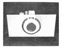
Figure 21. FRONT VIEW, SHOWING TEN-TURN DIAL.
