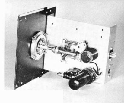
Figure 8. TOP CHASSIS OF THE ONE-TUBE V.F.O.
