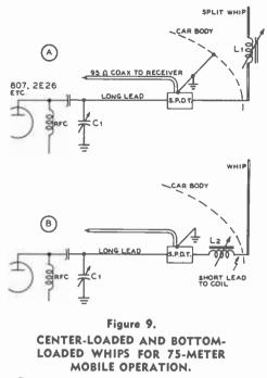
The center-loaded arrangement has a more favorable current distribution, but because of mechanical considerations a higher coil Q is possible with the bottom-loaded arrangement. The performance of the two arrangements is about equal. The whip should be at least 8 feet long, preferably longer.
