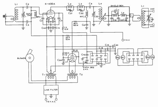
Figure 33. SCHEMATIC OF THE SHIELDED KILOWATT AMPLIFIER.
