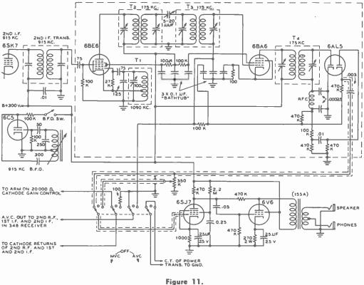
SCHEMATIC OF THE CIRCUITS ADDED TO THE BC-348.
