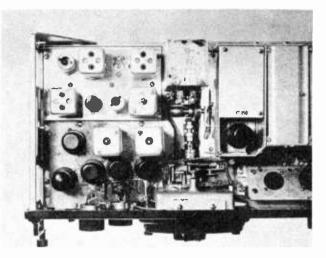
Figure 9. TOP VIEW OF THE BC-348 WITH THE 175-KC. I-F
