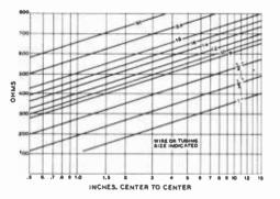
Figure 19. CHARACTERISTIC IMPEDANCE OF TWO-WIRE OPEN LINES.
