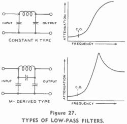
Filters such as these may be used in the circuit between the antenna and the input of the receiver.
