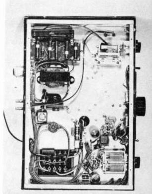
link switching. A 90-degree index is used with the switch sections, and the appropriate sections of the wafer switches are picked up at the 90-degree indexing points.
