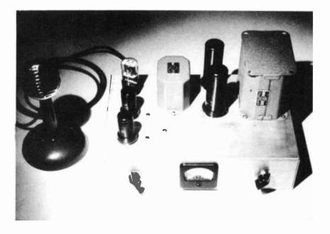
Figure 5. TOP VIEW OF THE 6L6 MODULATOR.
