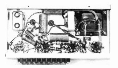
Figure 7. UNDERCHASSIS PHOTO OF THE KEYER UNIT.
