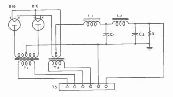
Figure 20. SCHEMATIC OF THE 400-VOLT 250-MA. SUPPLY.
