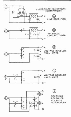
Figure 6. LINE-RECTIFIER CIRCUITS.
