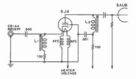
Figure 15. ALTERNATIVE INPUT CIRCUIT FOR USE WITH COAXIAL LINE. L, and L, are the same as described in figure 14. The r-f chokes in the heater leads of the 6J4 may be Ohmite type Z-28 chokes. One-half of a type 6J6 tube may be used in place of the 6J4 with slightly reduced performance.
