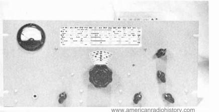
Figure 15. FRONT-PANEL VIEW OF THE EXCITER UNIT. is available to drive a pair of beam tetrodes to 1 kw. input.
