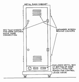
Figure 8. ISOLATING MEASURES FOR THE RACK-ENCLOSED TRANSMITTER.
