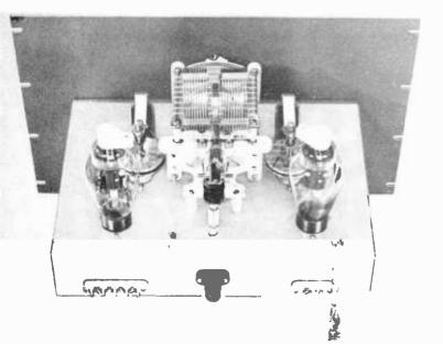
Figure 12. PUSH-PULL GENERAL-PURPOSE AMPLIFIER, REAR VIEW.
