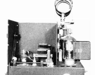
A parasitic suppressor consisting of 9 turns of solid hookup wire wound around a 10-ohm 2-watt resistor is included in series with the grid lead of the HK-57 tube. This parasitic suppressor may be seen in figure 12 between the grid r-f choke and the potentiometer mounted on the front panel. The potentiometer serves as a variable grid leak for the HK-57 stage.
