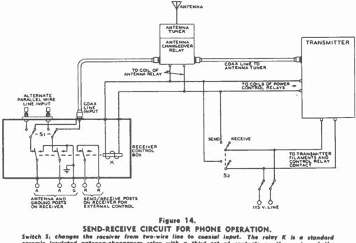
ceramic insulated antenna-changeover relay with a third set of contacts on the center of the relay structure for receiver control.
