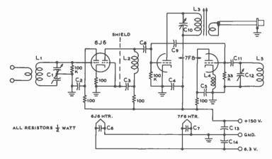
Figure 19. SCHEMATIC OF THE 144-MC. CONVERTER.
