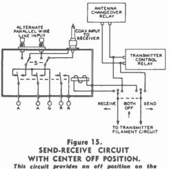
transmit-receive switch for disabling both the transmitter and the receiver. The balance of the circuit is the same as that of figure 14.
