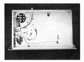
Figure 17. 35TG AMPLIFIER UNDERCHASSIS. Note that all r-f components are mounted a bove the chassis.
