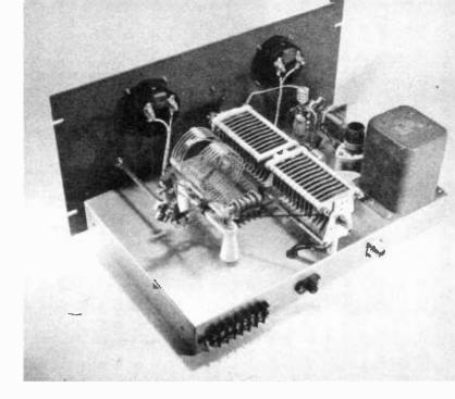
Figure 16. REAR OF THE 35TG AMPLIFIER. The 14-Mc. coils are in place in this photograph.
