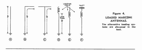
ever, the efficiency with a counterpoise will be quite good, regardless. It is when the radials are buried, or laid on the ground, that a large number should be used for best efficiency. Brodacast stations use as many as 120 radials of from 0.3 to 0.5 wavelength long.
