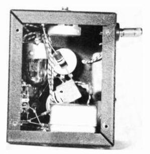
Figure 4. INSIDE THE MINIATURE AUDIO OSCILLATOR. The 12AU7 tube and its sock-
