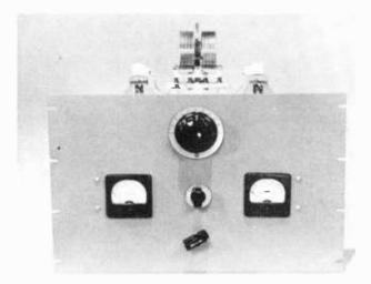
Figure 11. PANEL VIEW OF THE GENERAL-PURPOSE AMPLIFIER.
