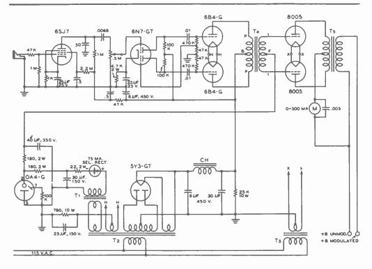
Figure 23. SCHEMATIC OF THE 300-WATT CLASS B MODULATOR.
