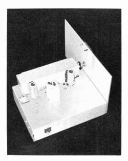
Figure 20. SIDE VIEW, SHOWING PLACEMENT OF THE INDUCTUNER.
