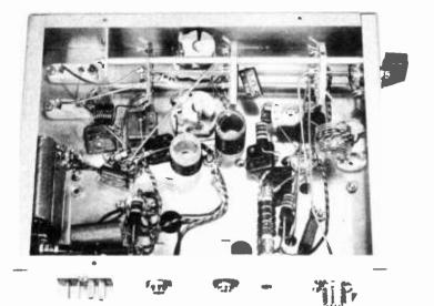
Figure 15. UNDERCHASSIS OF THE 12-WATT MOBILE TRANSMITTER.
