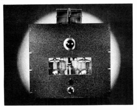
Figure 25. FRONT OF THE PUSH-PULL 4-250A AMPLIFIER.
