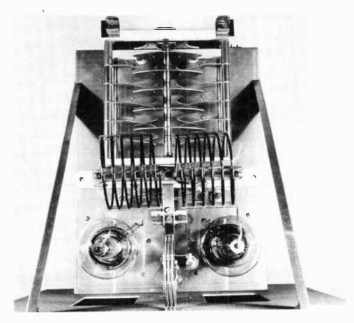
Figure 23. LOOKING DIRECTLY DOWN ON THE 250TH AMPLIFIER. It was necessary to dis-assemble and re-assemble the main tuning capacitor to place the neutralizing plates next to the tubes at the front. Procedure is given in the text.
