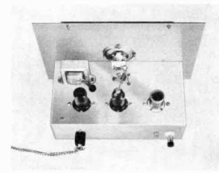
Figure 2. TOP PHOTO OF THE REGENERATIVE RECEIVER.
