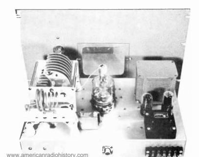
Figure 8. REAR VIEW OF THE 4-125A AMPLIFIER. In this photograph the plate tank circuit is on the left side and the screen, blas and filament voltage supplies are on the right.
