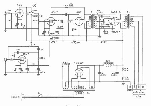
Figure 14. SCHEMATIC OF THE 6AS7-G AMPLIFIER.
