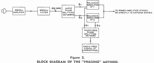
The phasing method of obtaining a single-sideband signal is simpler than the filter system in regard to the number of tubes and circuits required. The system is also less expensive in regard to the components required, but is more critical in regard to adjustments for the transmission of a pure single-sideband signal.
