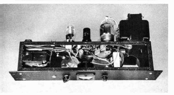
Figure 9. LOOKING INSIDE THE MODULATOR CHASSIS. The chassis has been removed from the cabinet and inverted for this photograph. Note the heavy-duty filament transformer for all tubes mounted inside the chassis and attached to the left end in this view.
