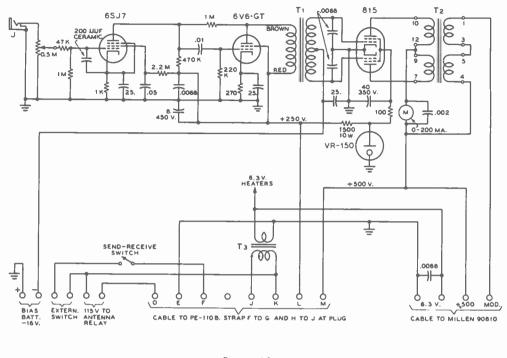
Figure 10. SCHEMATIC OF THE 815 MODULATOR.
