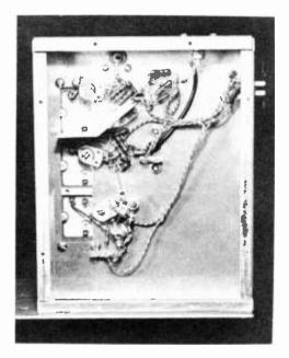
Figure 24. UNDERCHASSIS OF THE CONVERTER FOR 26 TO 135 MC. COVERAGE.
