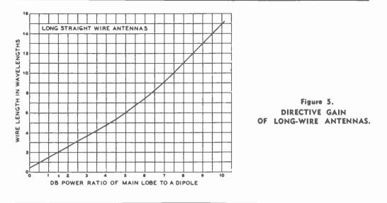
ing stations in nearly all directions, though the power radiated broadside to the radiator will not be great if the radiator is more than a few half wavelengths long. The directive gain of long-wire antennas, in terms of the wire length in wavelengths is given in figure 5.
