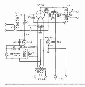
liammeter at ground potential, yet the grid current of the stage does not pass through the milliammeter in the cathode.
