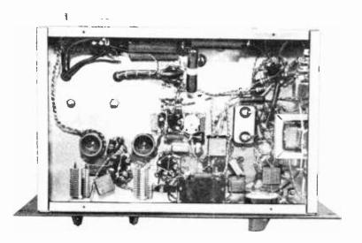
Figure 13. UNDERCHASSIS OF THE 3.9-MC. FM EXCITER.
