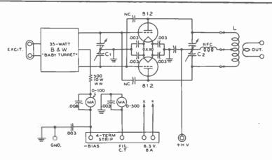
Figure 14. PUSH-PULL GENERAL-PURPOSE AMPLIFIER, SCHEMATIC.
