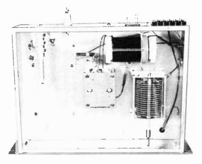
Figure 20. UNDERCHASSIS OF THE 304TL G-G AMPLIFIER.
