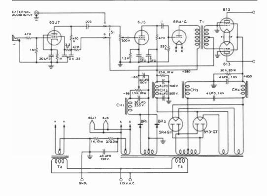
Figure 29. SCHEMATIC OF THE 500-WATT 813 MODULATOR.
