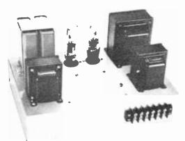
Figure 19. VIEW OF THE 750/600 VOLT 200-MA. SUPPLY.
