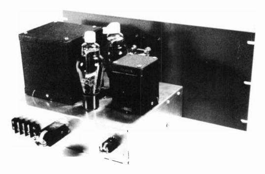
Figure 16. REAR VIEW OF THE 809 MODULATOR.
