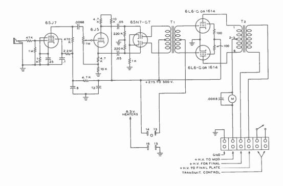
Figure 7. SCHEMATIC OF THE 6L6 MODULATOR. M—0-250 d-c milliammeter (Simpson model 127) T1—Driver transformer to 6L6 grids (UTC S-10) T2—60-wott modulation transformer (UTC S-20)
