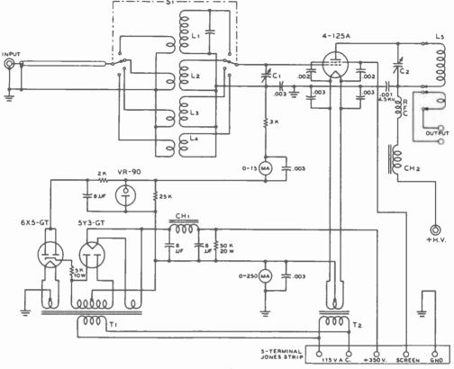
Figure 10. SCHEMATIC OF THE 4-125A AMPLIFIER.
