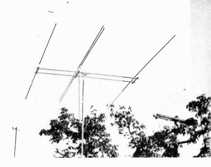
Figure 36. MANUFACTURED 3-ELEMENT 28-MC. ROTARY. This antenna is used in conjunction with the control and indicator systems of figures 33, 34, and 35 at W6DGN.
