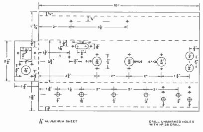
Figure 16. CHASSIS LAYOUT DRAWING FOR THE BROAD-BAND CONVERTER.
