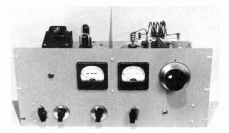
Figure 27. PANEL VIEW OF THE 4E27/257B TRANSMITTER. The dial lamp to the left of the two d-c instruments is connected in parallel with the 6.3-volt filoments to serve as a pilot light.
