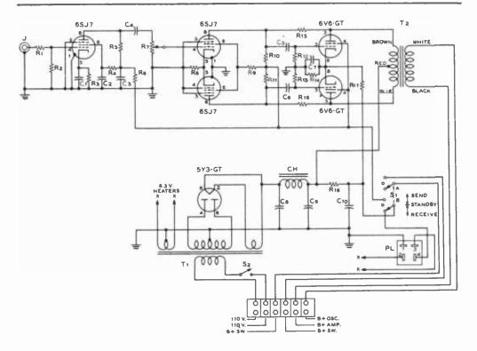
Figure 4. SCHEMATIC OF THE 10-WATT 6V6-GT MODULATOR.
