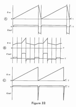
Differentiator outputs of short-time-constant RC circuits for various input voltage waveshapes. The output voltage is proportional to the rate of change of the input voltage.
