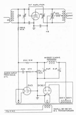
Figure 3 GRID-BIAS MODULATOR CIRCUIT
