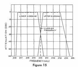
PASSBAND OF LOWER- AND UPPER-SIDEBAND MECHANICAL FILTER
