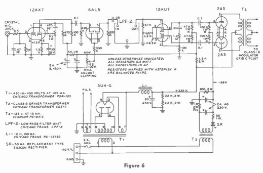
SCHEMATIC, 15-WATT CLIPPER-AMPLIFIER
