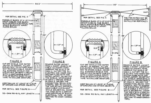
DIMENSIONS SMOWN HERE ARE FOR THE 40-METER BAND. THIS ANT-ENNA MAY BE BUILT FOR OTHER BANDS BY USING DIMENSIONS THAT ARE MULTIPLES OR SUBMULTIPLES OF THE DIMENSIONS SHOWN. BALUN SPACING IS 1.5" ON ALL BANDS.
