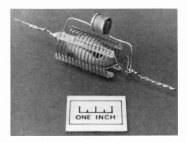
Figure 31 TRAP CONSTRUCTION
