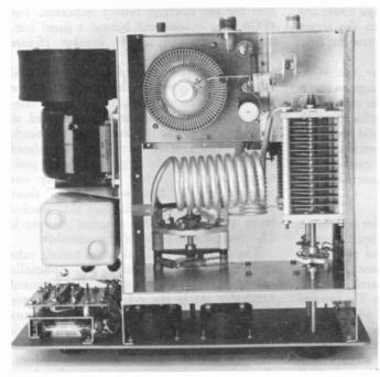
The 4CX1500B is mounted at the rear of the main amplifier inclosure on a separate subchassis. To the right of the tube are the plate r-f chokes and bypass capacitors. The ALC coupling capacitor is directly behind the main plate tuning capacitor.
