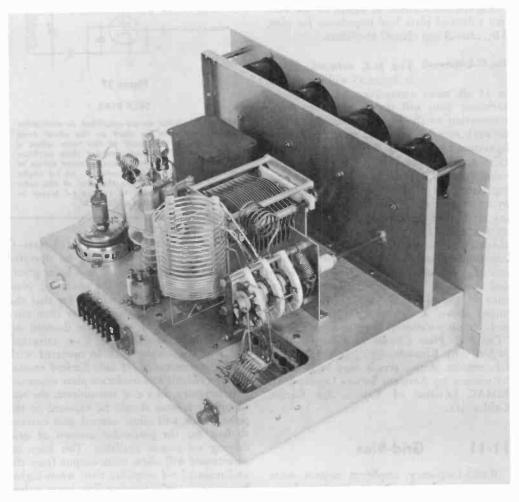
Figure 36 PI-L NETWORK PROVIDES EXTRA HARMONIC ATTENUATION
