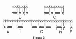
Diagram liliustrating relative lengths of dashes and spaces referred to the duration of a dot. A dash is exactly equal in duration to three dots; spaces between parts of a letter equal one dot; those between letters, three dots; space between words, five dots. Note that a slight increase between two parts of a letter will make it sound like two letters,
