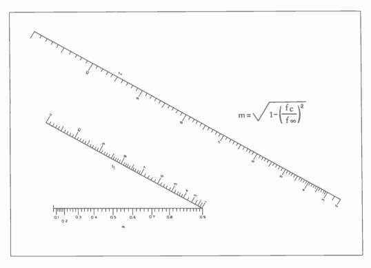
Figure 44 NOMOGRAPH #2. FILTER CONSTANT  $\it m$  IS DETERMINED FROM  $\it f_{\infty}$  and  $\it f_{c}$
