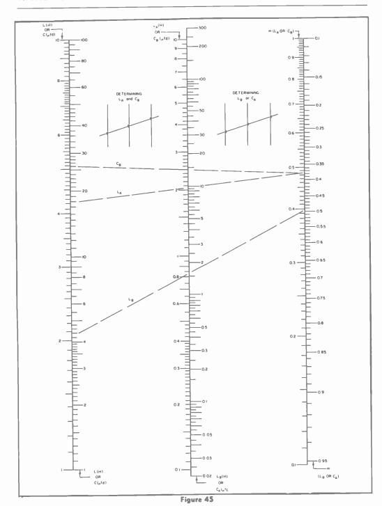
NOMOGRAPH #3. L, AND  $C_B$  ARE DETERMINED USING L AND C (NOMOGRAPH #1) AND m (NOMOGRAPH #2.) ALL NUMBERS ARE FOUND WITH LEFT SIDE OF SCALES. L, AND  $C_A$  ARE DETERMINED IN THE SAME MANNER, USING RIGHT SIDE OF SCALES.
