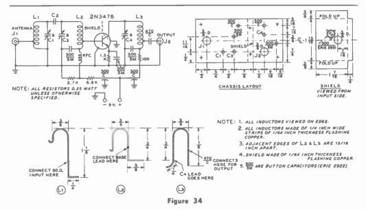
SCHEMATIC AND LAYOUT FOR 432-MHz R-F AMPLIFIER
