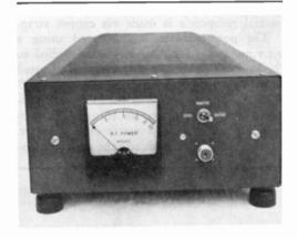
Figure 14 2-KILOWATT DUMMY LOAD FOR 3-30 MHz
