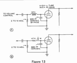
CIRCUITS FOR ELIMINATING AUDIO-STAGE RECTIFICATION
