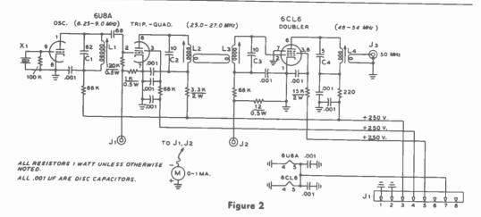
SCHEMATIC OF SIX-METER EXCITER
