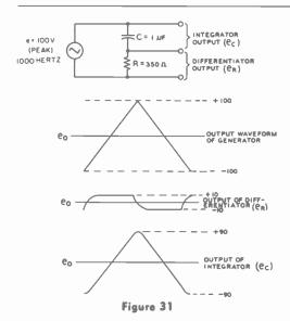
RC DIFFERENTIATOR AND INTEGRATOR ACTION ON A SAWTOOTH WAVE
