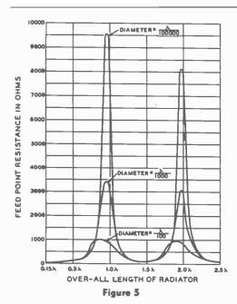
FEED-POINT RESISTANCE OF A CENTER-DRIVEN RADIATOR AS A FUNCTION OF PHYSICAL LENGTH IN TERMS OF FREE SPACE WAVELENGTH
