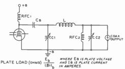
CB - .00025 UF. MICA GAPACITOR RATED AT TWICE THE D.C. PLATE VOLTAGE.
