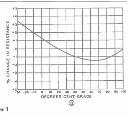
HEAT CYCLE OF UNCONDITIONED COMPOSITION RESISTORS
