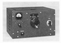
Inductance switch S, and sensitivity control are at left with counter dial for L, at center. Output tuning capacitor C, is at right. SWR meter is mounted above S.
