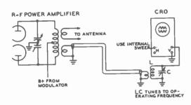
Figure 24 MONITORING CIRCUIT FOR **MODULATED-WAVE PATTERN**
