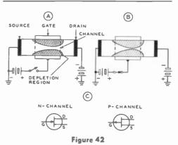
Depletion control is exercised by a "gate" of opposite intrinsic material across the conducting path.
