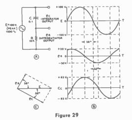
RC DIFFERENTIATOR AND INTEGRATOR ACTION ON A SINE WAVE
