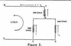
In this simple network the current divides through the 2000-ohm and 3000-ohm resistors. The current through each may be found by using two simultaneous linear equations. Note that the arrows indicate the direction of electron flow as explained on page 18.
