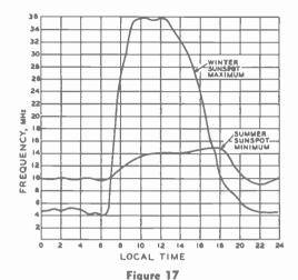
TYPICAL CURVES SHOWING CHANGE IN M.U.F. AT MAXIMUM AND MINIMUM POINTS IN SUNSPOT CYCLE
