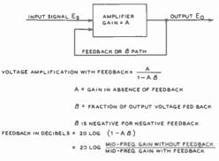
DISTORTION WITH FEEDBACK = DISTORTION WITHOUT FEEDBACK
