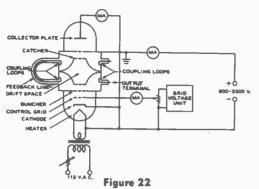
TWO-CAVITY KLYSTRON OSCILLATOR
