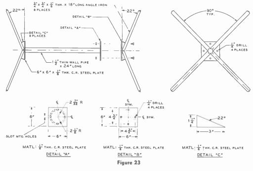
SPIDER CENTER STRUCTURE FOR QUAD ANTENNA
