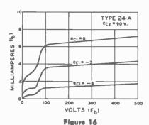
TYPICAL Ib vs. Eb TETRODE CHARACTERISTIC CURVES
