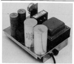
Figure 40 **300-WATT IVS POWER SUPPLY** FOR SSB TRANSCEIVERS
