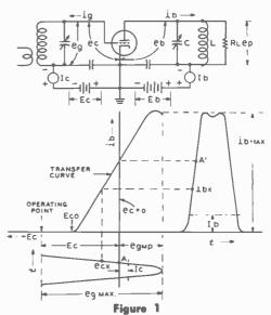
TRANSFER CURVE FOR OPERATING CYCLE OF CLASS-C AMPLIFIER
