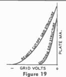
ACTION OF A REMOTE-CUTOFF GRID STRUCTURE
