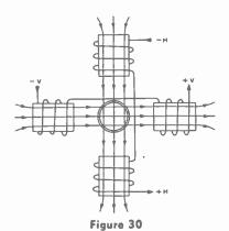
Two pairs of coils arranged for electromagnetic deflection in two directions.
