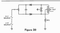
SERIES DIODE MODULATOR CIRCUIT
