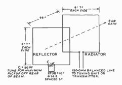
NOTE: \$10E LENGTH\* 11'8" FOR 21 MHI 17'7" FOR 14 MHI ELEMENT SPACING 98" FOR EACH BAND. STUB LENGTH APPROX. 13" FOR 21 MHI 20" FOR 14 MHI
