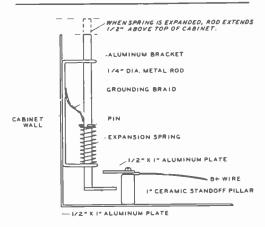
Figure 32 HOME-MADE HIGH-VOLTAGE SAFETY SHORTING SWITCH
