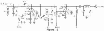
TWO-STAGE AMPLIFIER WITH FEEDBACK CIRCUIT
