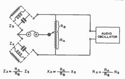
$Z_X=$  impedance being measured,  $R_S=$  resistance component of  $Z_S$   $z_S=$  impedance of standard,  $X_X=$  reactance component of  $Z_X$   $R_X=$  resistance component of  $Z_X$ ,  $X_S=$  reactance component of  $Z_X$
