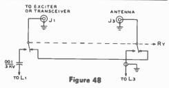
SUGGESTED ANTENNA-RELAY CIRCUIT FOR USING AMPLIFIER WITH **TRANSCEIVER**
