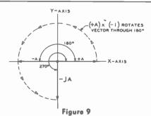
Operation on the vector (+A) by the quantity (-1) causes vector to rotate through 180 degrees.
