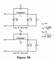
SHUNT m-DERIVED FILTER PI SECTIONS
