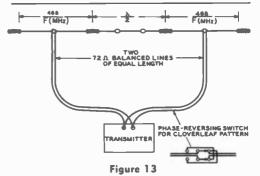
TWO COLLINEAR HALF-WAVE ANTENNAS IN PHASE PRODUCE A 3 DB GAIN WHEN SEPARATED ONE-HALF WAVELENGTH
