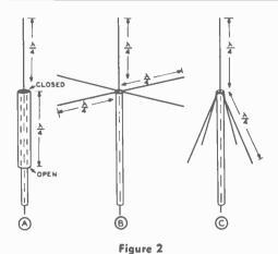
THREE VERTICALLY POLARIZED LOW-ANGLE RADIATORS
