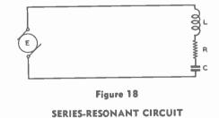
If the values of inductance and capacitance both are fixed, there will be only one resonant frequency.
