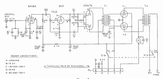
SCHEMATIC OF MEDIUM-POWER MODULATOR
