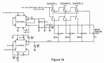
FREQUENCY-CONTROL SYSTEM AND REGULATED SUPPLY
