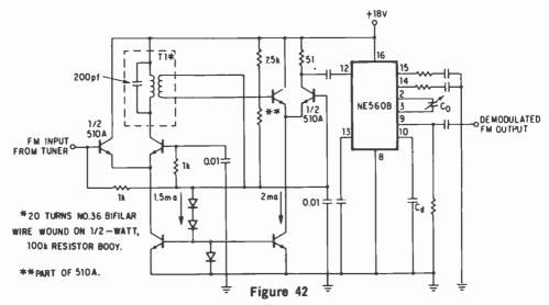
SIGNETICS NE-560B PHASE-LOCKED LOOP AS AN F-M DETECTOR
