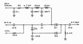
Figure 11 PIN DIODE USED AS R-F ATTENUATOR OR SWITCH
