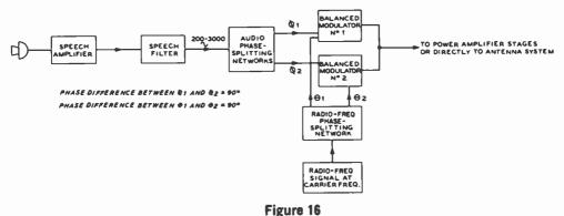
BLOCK DIAGRAM OF A PHASING TYPE EXCITER
