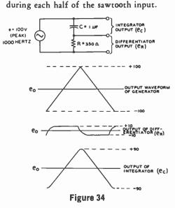
RC DIFFERENTIATOR AND INTEGRATOR ACTION ON A SAWTOOTH WAVE
