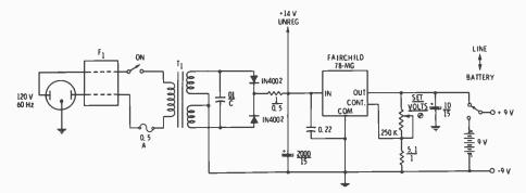
Figure 20 SCHEMATIC OF KEYER POWER SUPPLY
