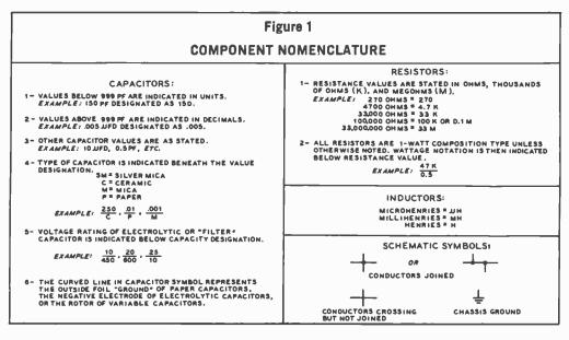
Circuitry and It is the practice of the edi-Components tors of this Handbook to place as much usable information in the schematic illustration as possible. In order to simplify the drawing, the component nomenclature of figure 1 is used in all the following construction chapters.
