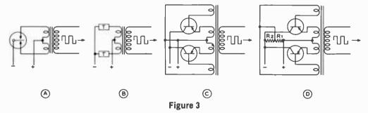
TRANSISTORS CAN REPLACE VIBRATOR IN MOBILE POWER SUPPLY SYSTEM
