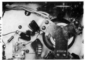
All other grid circuit components are within the inclosure, and the various auxiliary components are mounted on the outside, left wall of the inclosure. All leads passing from the inside to the outside are bypassed by means of a 1500-pF ceramic feedthrough capacitor in parallel with a  $.01-\mu F$ , 1-kV disc capacitor.
