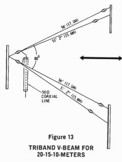
A compact design provides good gain for 3-band operation. Two V-beams are connected in parallel at the apex. The 56' legs are cut for operation on 10 and 15 meters, while the 51-foot legs provide 20-meter operation. The included angle is 80°. The shorter legs run under the longer ones, and are separated by about 10' (3 meters) distance at the tips. A 1-to-1 balun may be used with the antenna, if desired.
