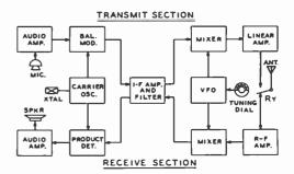
Figure 38 THE SSB TRANSCEIVER
