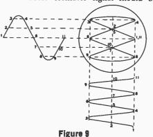
PROJECTION DRAWING SHOWING THE RESULTANT LISSAJOUS PATTERN WHEN A SINE WAVE APPLIED TO THE HORIZONTAL AXIS IS THREE TIMES THAT APPLIED TO THE VERTICAL AXIS
