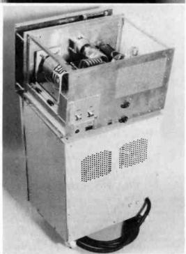
zero when the amplifier is switched out of the line. Shorting the *in/out* control terminals (figure 24) engages the antenna relay. In this mode, grid current with no drive should be zero. Plate current should read appoximately 120 milliamperes (the exact value varying from tube to tube). If grid current is observed, it is probably a sign of parasitic oscillation, and the circuit should be examined for parasitic resonances and the plate parasitic choke checked before additional tests are run.
