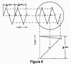
PROJECTION DRAWING SHOWING THE RESULTANT PATTERN WHEN THE FREQUENCY OF THE SAWTOOTH IS ONE-HALF OF THAT EMPLOYED IN FIGURE 7
