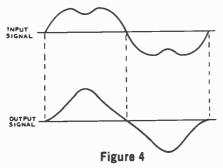
Illustration of the effect of phase distortion on input wave containing a third-harmonic signal.
