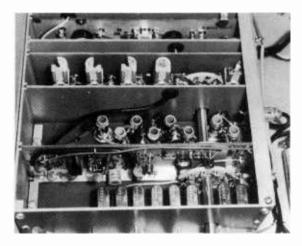
locating all of the tuned circuits close to the bandswitch while at the same time avoiding unwanted interstage coupling. In this design all of the bandswitched circuits were constructed on 214" × 534" circuit boards. A representative board is shown in figure 44.
