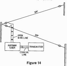
This V-beam performs well on the lower DX bands. The included angle should be 80° for 80 meters, 60° for 40 meters and 45° for 20 meters. Gain varies from 3 dB at 80 meters to about 7.5 dB at 20 meters. The beam is fed with a two-wire transmission line and an antenna tuner, such as described in Chapter 26.
