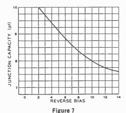
JUNCTION CAPACITANCE VARIATION WITH RESPECT TO REVERSE VOLTAGE
