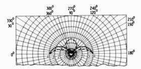
(A) 0, 25 (SOLID) AND 0, 375 (BROKEN) WAVELENGTH ABOVE GROUND.
