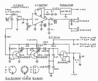
applied to the gate of a P-channel JFET  $(Q_{14})$ , across which there is a long-time-constant circuit. The FET is operating in depletion mode; the more positive gate voltage it receives, the more negative the output voltage becomes. The FET output, tied to the bottom of the R-F Gain control, establishes the most negative bias level on the r-f and i-f amplifier stages in the receiver.
