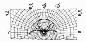
(B) 0, 5 (SOLID) AND 0, 75 (BROKEN) WAVELENGTH ABOVE GROUND.
