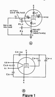
LEAD INDUCTANCE AND INTERNAL CAPACITANCE
