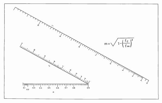
Figure 49 NOMOGRAPH #2. FILTER CONSTANT  $\it{m}$  IS DETERMINED FROM f $_{\it{c}}$  and f $_{\it{c}}$
