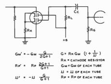
EQUIVALENT FACTORS INDICATED ABOVE 8Y (') ARE THOSE OBTAINED BY USING AN AMPLIFIER WITH A PAIR OF SIMILAR TUBE TYPES IN CIRCUIT SHOWN ABOVE.
