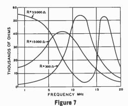
CURVES OF THE IMPEDANCE OF WIRE WOUND RESISTORS AT RADIO FREQUENCIES
