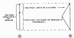
Figure 10 VECTOR RELATIONSHIP OF FEEDBACK VOLTAGE
