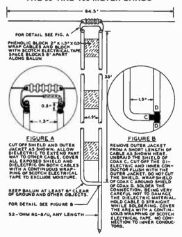
DIMENSIONS SMOWN MERE ARE FOR THE 40-METER BAND. THIS ANT-ENNA MAY BE BUILT FOR OTHER BANDS BY USING DIMENSIONS THAT ARE MULTIPLES OR SUBMULTIPLES OF THE DIMENSIONS SMOWN, BALUN SPACING IS 1.5° ON ALL BANDS.
