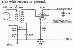
Figure 5 **CATHODE-FOLLOWER** SCREEN-MODULATION CIRCUIT
