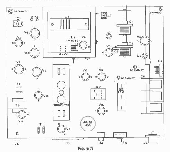
UNDER-CHASSIS LAYOUT OF TRANSCEIVER
