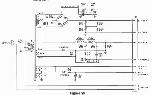
SCHEMATIC, 600-WATT TRANSCEIVER SUPPLY
