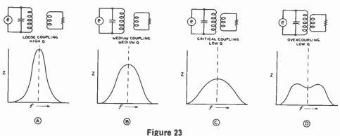
EFFECT OF COUPLING ON CIRCUIT IMPEDANCE AND Q
