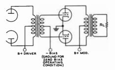
Figure 22 **CLASS-B AUDIO-FREQUENCY**
