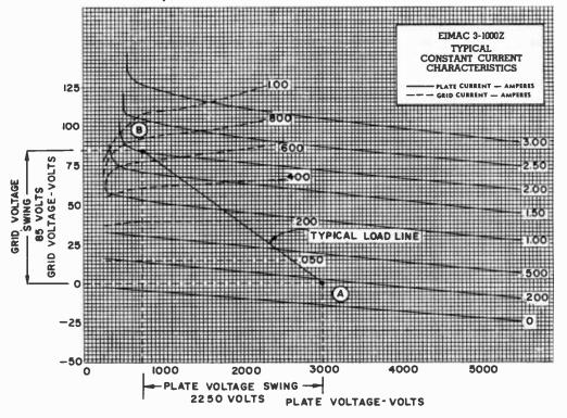
Figure 4 CONSTANT-CURRENT CHART FOR 3-1000Z HIGH- $\mu$  TRIODE
