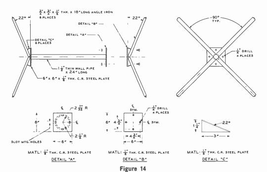
SPIDER CENTER STRUCTURE FOR QUAD ANTENNA
