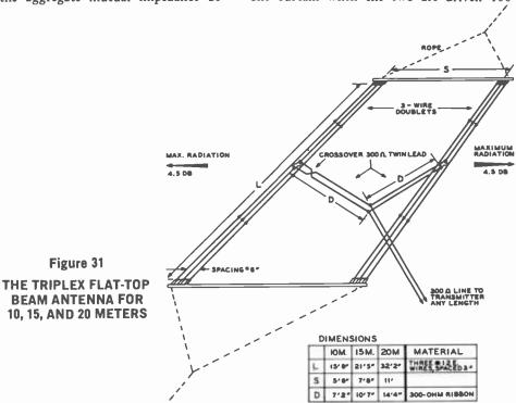
degrees out of phase to give a bidirectional pattern (the type of pattern obtained with a single curtain). However, if they are driven in phase quadrature (and with equal currents) the gain is approximately 3 dB.
