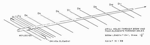
ELEMENT DIMENSIONS, 2-METER BAND SPACING LENGTH DIPOLE (DIAM. 1/8-) 144 MHz 145 MH 146 MHz 147 MHz 40 7 REFLECTOR 41" 40 3 40 3 19 " 36 } 36 -36 3 36 🖟 D1= 7" DIRECTORS D2= 14.5\* DRIVEN ELEMENT D3= 22" D4= 36" D5= 70" CLEARANCE HOLE Da= 102\* D7= 134\* D6= 166\* # 6 WIRE FOR 300 0 INSULATING PLATE MATCH. #10 WIRE FOR 450 Q MATCH Do= 1984 TUBING AT ENDS D10= 230" D11=242\*
