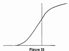
A TYPICAL GRID-VOLTAGE PLATE-CURRENT CHARACTERISTIC CURVE
