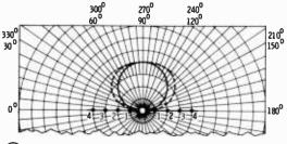
(A) 0.1 (SOLID) AND 0.25 (BROKEN) WAVELENGTH ABOVE GROUND.
