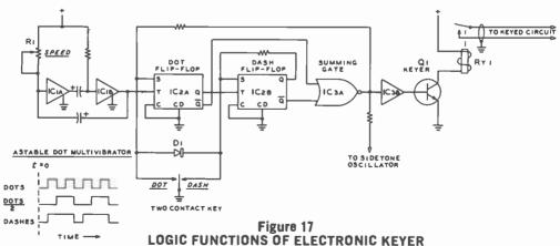
Astable multivibrator (IC,) generates string of pulses (dots) with speed controlled by potentiometer R,. Dot flip-flop sends precise square-wave dots when key contact is closed. Dash flip-flop adds long pulse to dot, forming 3-baud dash at output of summing gate. Amplifier and keying transistor drive a reed relay which controls the transmitter circuit. Dot memory, sidetone monitor, and iambic characteristic may be added to the basic keyer, if desired.
