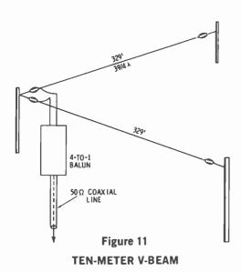
This antenna provides about 11.5 decibels gain over a dipole on the 10-meter band. The included angle between the wires is 32°. The beam is fed at the apex with a 4-to-1 balun and a coaxial transmission line. See Chapter 26, figures 6 and 7 for balun design.
