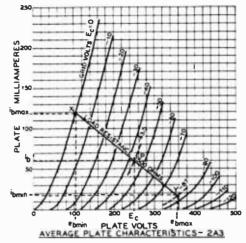
H=4.2 Rp = 800 OHMS PLATE DISSIPATION = 15 WATTS
