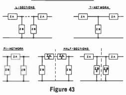
Complex filters may be made up from these basic filter sections.
