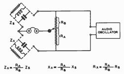
$Z_X$  = impedance being measured,  $R_S$  = resistance component of  $Z_S$   $Z_S$  = impedance op standard,  $X_X$  = reactance component of  $Z_X$   $R_X$  = resistance component of  $Z_X$ ,  $X_S$  = reactance component of  $Z_S$
