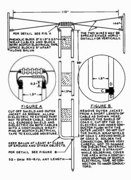
DIMENSIONS SHOWN HERE ARE POR THESO-METER BAND, THIS ANT-ENNA MAY BE SUILT POR OTHER BANDS BY USING DIMENSIONS THAT ARE MULTIPLES OR SUBMULTIPLES OF THE DIMENSIONS SHOWN. BALUN SPACING IS 1.5" ON ALL BANDS.
