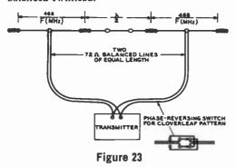
TWO COLLINEAR HALF-WAVE ANTENNAS IN PHASE PRODUCE A 3 DB GAIN WHEN SEPARATED ONE-HALF WAVELENGTH
