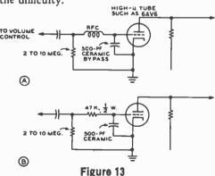
CIRCUITS FOR ELIMINATING AUDIO-STAGE RECTIFICATION
