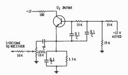
Figure 16 SIDETONE GENERATOR FOR BREAK-IN KEYING
