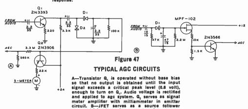
driving the gain control transistor.
