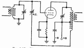
FIG. 2-17.—Plate neutralization system.
