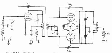
FIG. 2-16.—Radio-frequency amplifier with capacity neutralization.
