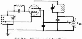
Fig. 2-9.-Electron-coupled oscillator.
