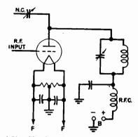
Fig. 4-21.-Simple series-fed plate arrangement.
