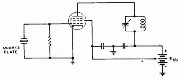
FIG. 2-10.—Pentode-type crystal-controlled oscillator.
