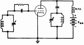
FIG. 2-5.—Tuned-plate tuned-grid shunt-fed oscillator.
