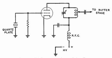
FIG. 2-6.—Triode-type crystal-controlled oscillator.
