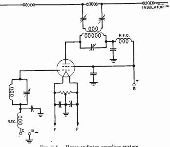
FIG. 3-8.—Hertz-radiator coupling system.
