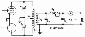
FIG. 4-11.—Transmission-line coupling system.
