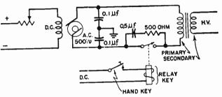
FIG. 5-3.-Transformer-primary keying system.
