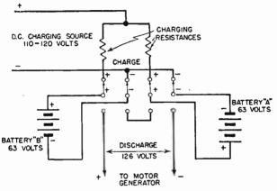
FIG. 2-29.-Battery charging arrangement.
