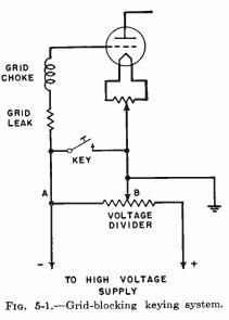
Ans. The most satisfactory means of keying a high-power radiotelegraph transmitter is by the so-called grid-blocking system. With this system a grid bias sufficient to block the power amplifier is applied when the key is up. The key is connected to shunt the bias resistor, thus removing the bias when the key is down. When the bias is removed, the signal wave is emitted by the transmitter.
