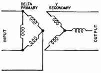
FIG. 4-2.—Delta-star or Y transformer.
