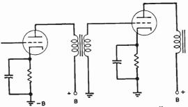
FIG. 2-14.-Inductive or transformer coupling.
