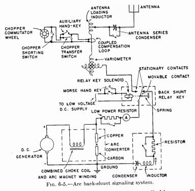
excited from the ship's direct current and controlled by a small Morse hand key in series with the solenoid. When the key is open, the back-shunt relay arm is connected to a closed absorption circuit into which the arc oscillates. When the key is closed, the arc is transferred to the antenna oscillatory system. This results in a uniwave signal emission, enables the operator to adjust the arc for maximum stability when the key is open, and eliminates unnecessary adjustment interference.
