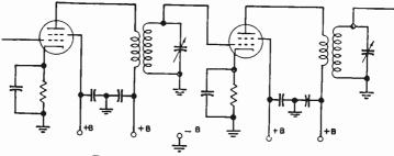
FIG. 2-20.-Interstage coupling system.
