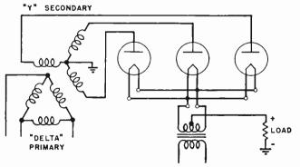
FIG. 2-38.—Half-wave three-phase rectifier.
