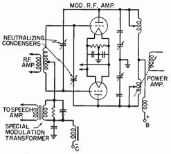
FIG. 3-7 .- Grid-modulation system.
