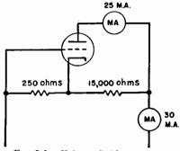
FIG. 3-2.--Voltage divider network.
