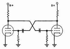
FIG. 4-19.-Multivibrator oscillator.
