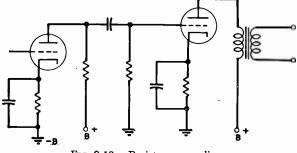
FIG. 2-13.—Resistance coupling.
