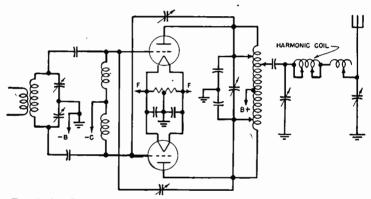
FIG. 4-10.-Capacitive coupling and harmonic suppression arrangement.
