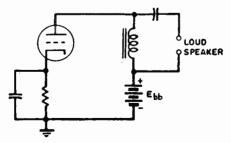
FIG. 2-11.-Loud-speaker coupling arrangement.
