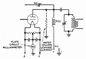
Fig. 4-15.—Correct ammeter connection in water-cooled system.
