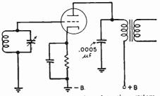
FIG. 2-23.—Power or plate detection system.
