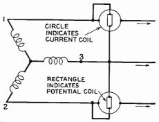
FIG. 4-1.—Three-phase wattmeter connections.
