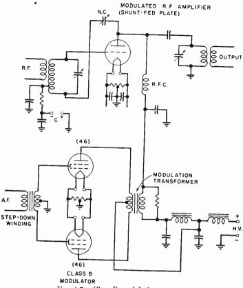
FIG. 4-7.-Class B modulation system.
