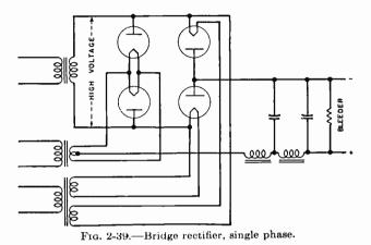
Ques. 2.246. Draw a diagram of a full-wave, single-phase rectifier employing thermionic vacuum tubes, connected to a condenser input, two-section filter system, and including a bleeder resistance.
