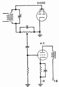
Fig. 2-22.-Diode detector and audio-frequency amplifier.
