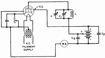
FIG. 3-12.-Dynatron oscillator.
