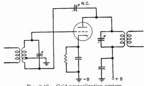
FIG. 2-18.—Grid neutralization system.
