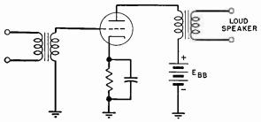
FIG. 2-12.-Loud-speaker coupling arrangement.
