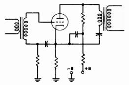
FIG. 4-4.-Parallel-fed amplifier system.
