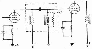
FIG. 2-15.—Impedance coupling.
