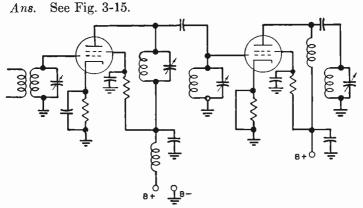
FIG. 3-15.—Capacitative coupling system.
