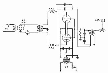
FIG. 6-6.-Marine self-rectifying transmitter circuit.
