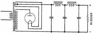
FIG. 2-41.—Half-wave rectifier.
