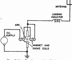
FIG. 3-14.—Fundamental oscillating arc.
