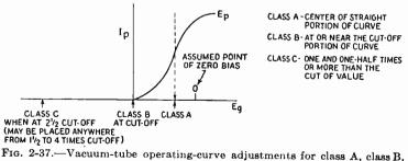
rig. 2-37.—vacuum-tube operating-curve adjustments for class A, class B, and class C amplification.
