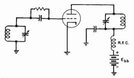
FIG. 2-2.-Tuned-plate tuned-grid series-fed oscillator.
