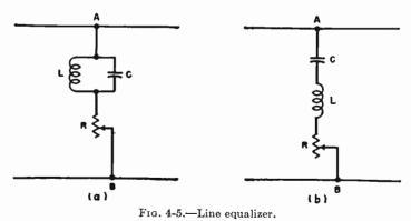
Ques. 4.45. Draw a diagram of an equalizer circuit most commonly used for equalizing wire-line circuits.
