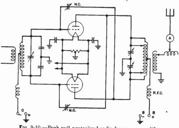
FIG. 3-10.—Push-pull neutralized radio-frequency amplifier.
