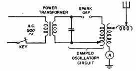
FIG. 3-13.—Fundamental spark transmitter.
