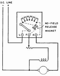
D.C. MOTOR FIG. 2-34.—Shunt-wound motor, speed regulator, and starter.
