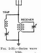
Ques. 2.115. Draw a diagram of a simple series wave-trap circuit, connected in shunt with the input terminals of a radio receiver, and designed to bypass an undesired signal.
