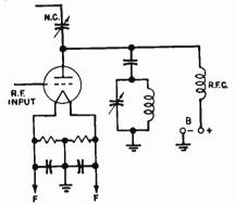
FIG. 4-20.—Simple shunt-fed plate arrangement.
