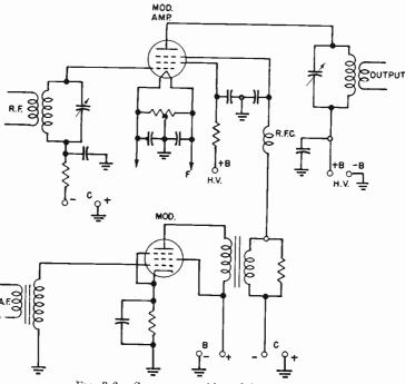
FIG. 3-6.—Suppressor-grid-modulation system.
