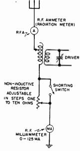
FIG. 4-12.—Circuit for measuring antenna resistance.
