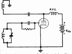
FIG. 2-4.—Armstrong tuned-grid shunt-fed oscillator.
