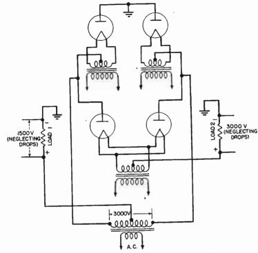
FIG. 4-16.—Balanced single-phase full-wave rectifier.
