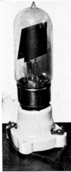
A special neon lamp with electrodes measuring 1\frac{1}{2} \times 1\frac{1}{2} . Such lamps are connected in the output circuits of television receivers.
