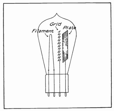
Figure 7: Sketch showing the elements in a radio vacuum tube.
