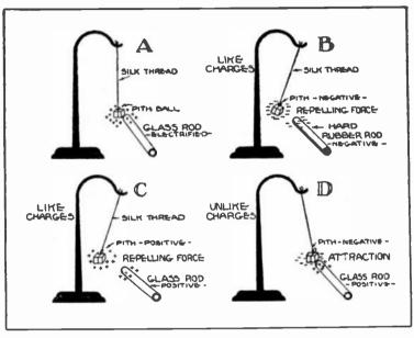
Figure 8: Sketches illustrating the basic laws of electrostatics.
