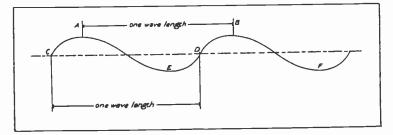
Figure 6: Diagram showing method of measurement of radio waves.
