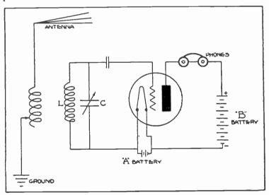
Figure 10: Sketch of circuit in which the grid receives its positive and negaive charges from the antenna, which is energized by passing electromagnetic waves.
