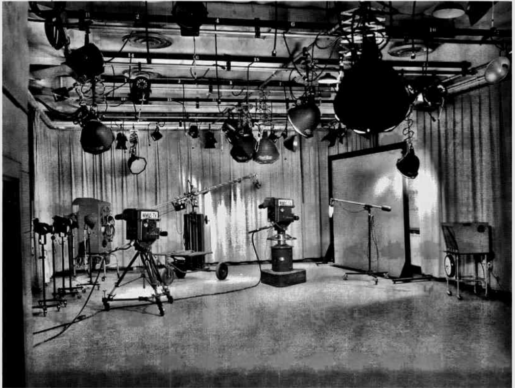
The original WMVS-TV studio on the 6th floor of The Milwaukee Vocational School. Seen in this photo are two RCA Image Orthicon monochrome cameras, a rear projection screen, boom microphone, and studio monitor. (MPTV photo)
