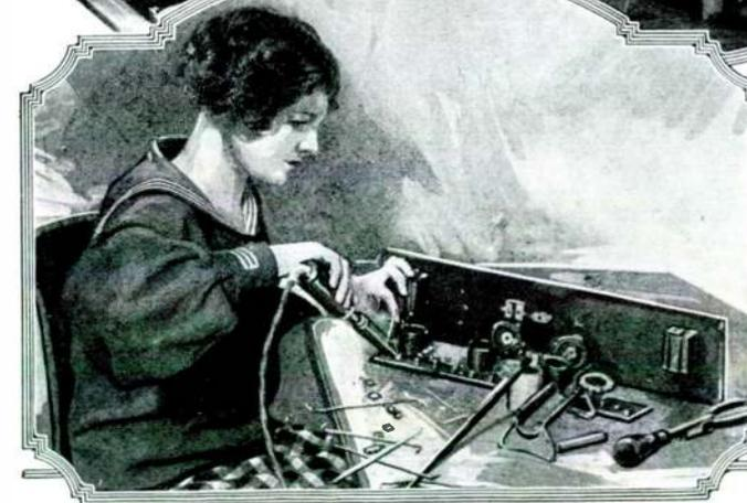
The Shipping End of One of the Long Assembly Tables, Each Side of Which Turns Out a Set Every Three Minutes, and (Below) a Soldering Job on One Subpanel Connection
