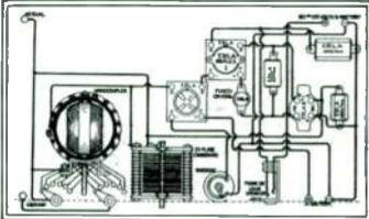
At the top of this page is the usual symbol diagram for the three-tube Erla hookup dealt with in this article. To the left is a pictorial diagram showing the hookups of the single-tube Erla reflex circuit.
