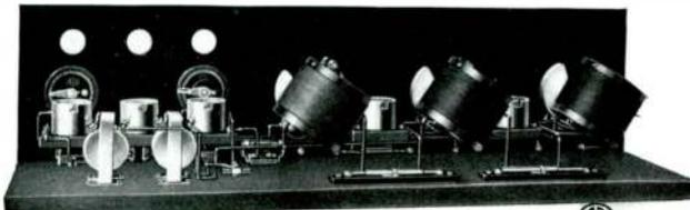
The rear view of the five tube home-made "Neutrodyne" receiving set. Audio frequency amplifying transformers on this set are both placed to the rear of the tube socket.
