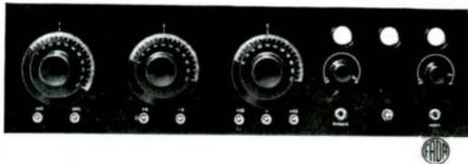
The front panel layout of the five tube "Neutrodyne" set is somewhat different, three of the vacuum tubes being placed at the right hand end of the panel.
