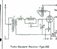
The above diagram shows the circuit of the Tuska Standard Receiver. This hookup gives excellent results. By adding two stages of audio frequency amplification you have a long distance receiver equal to the best.
