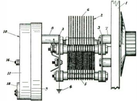
1. In combination with a radio transformer, a shield comprising two parts for supporting, prelocating and protecting said transformer, a condenser, and means for mounting the shield on the condenser.
