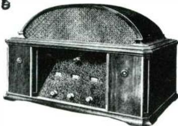
**C-40** Not illustrated. Seven tubes—199's or 201-A's. Balanced tuned radio frequency. In specially designed custom-built hand-carved cabinet. Every detail and feature is provided in this model to make it the last word, not only as a radio receiving set, but also as a beautiful furniture piece for the select home. Without accessories \$350
