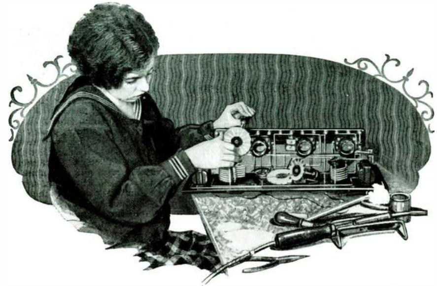
The Basket-Woven Inductance Coil Follows the Antenna and Ticker Coils into Place as the Growing Set Flits down the Long Assembly Table
