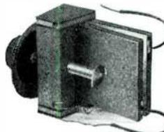
This Condenser works on an entirely new principle. The two plates are hinged and are opened and closed like a book by means of a specially designed cam. The plates are surfaced with copper. One copper sheet is covered with mica, so that when the two plates are clamped tightly together the maximum capacity is obtained. The maximum capacity of this Condenser will average about .0008. We rate it conservatively, however, at .0005.
