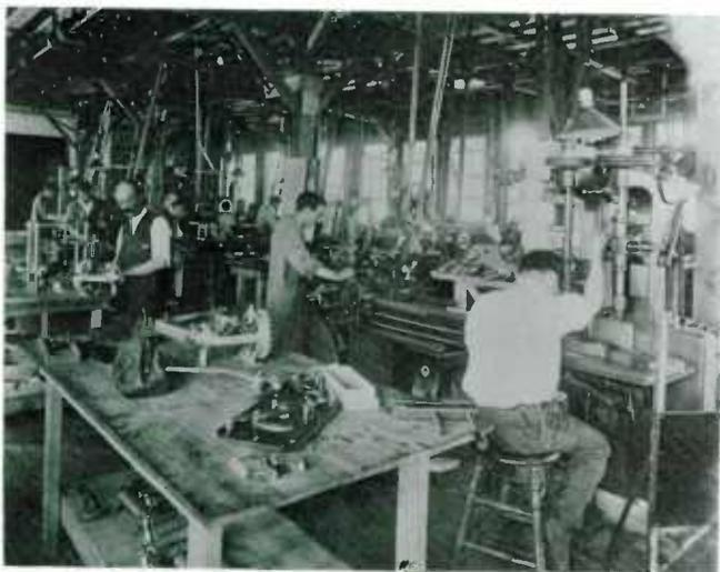
Machining rotary spark gaps, 1917.
