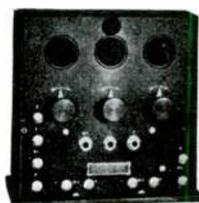
Detector and Two-Stage Audio Frequency Amplifier.
