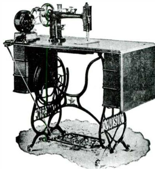
THE KENT ALTERNATING SEWING MACHINE MOTOR.
