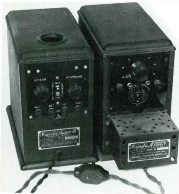
In the 1924-27 period, before AC sets were fully established, B-battery eliminators rang up more than \$30 million in sales, the most popular model being the Majestic Super-B. A-battery eliminators were less successful, as no really good rectifier was available for the high currents needed (1 1/2 amperes for a six-tube radio).
