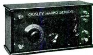
Complete tuner and audion detector assembled on a formica or other high grade dielectric panel, mounted complete in mahogany finish cabinet. Range, 150 to 600 meters, non-regenerative hook-up. Price without battery, tube or phones .....\$16.00
