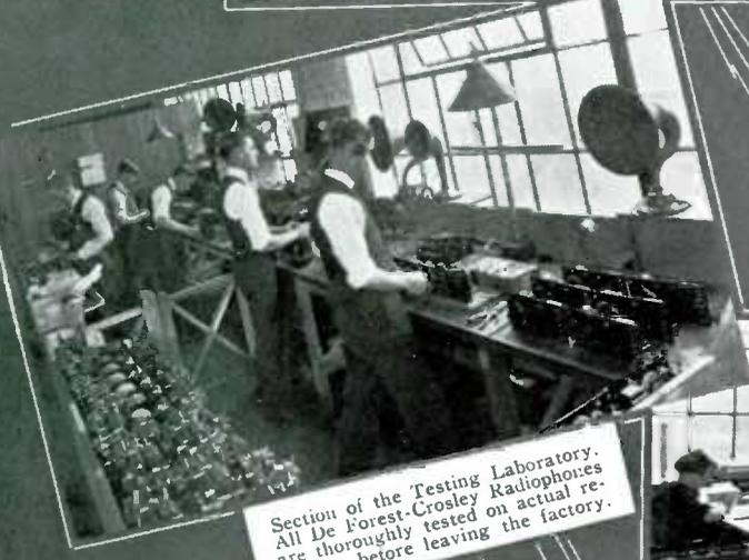
Section of the Testing Laboratory. All De Forest-Crosley Radiophones are thoroughly tested on actual reception before leaving the factory.
