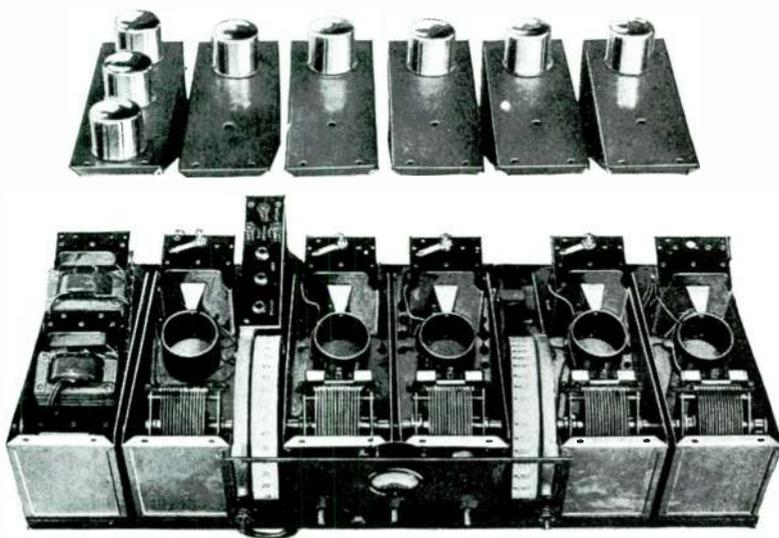
Fig. 4 An eight-tube tuned-radio-frequency receiver which is completely shielded, and is extremely easy to tune and control.
