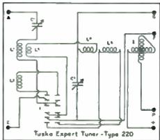
The above diagram shows the circuit of the Tuska Expert Tuner. This is a very effective circuit and the tuner may be constructed easily from the parts listed in this catalogue.
