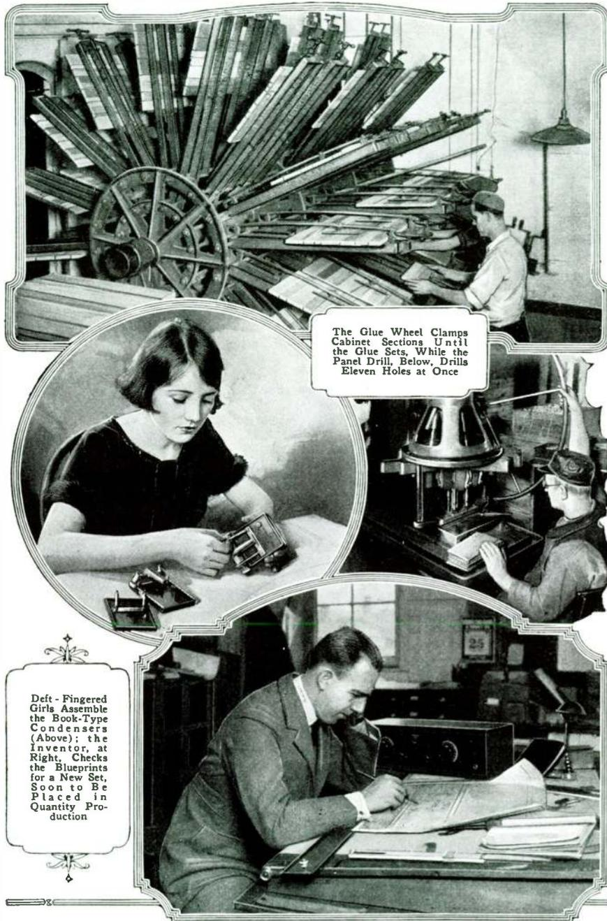
The Glue Wheel Clamps Cabinet Sections Until the Glue Sets, While the Panel Drill, Below, Drills Eleven Holes at Once
