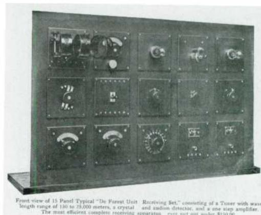
Front view of 15 Panel Typical "De Forest Unit Receiving Set," consisting of a Tuner with wave length range of 130 to 25,000 meters, a crystal and audion detector, and a one step amplifier. The most efficient complete receiving apparatus ever put out under \$100.00.
