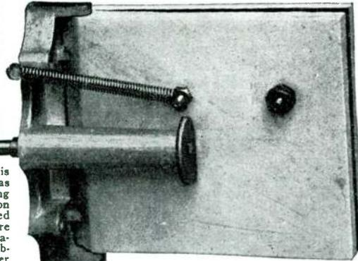
Model "A" with wood frame and laminated wood plates.
