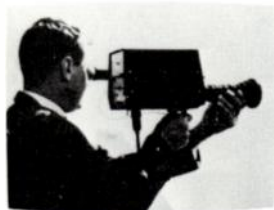
March 1966: the world's first battery-powered transistor television tape camera is displayed in California; it weighs just seven pounds and takes half-an-hour of broadcast-quality pictures without recharging.
