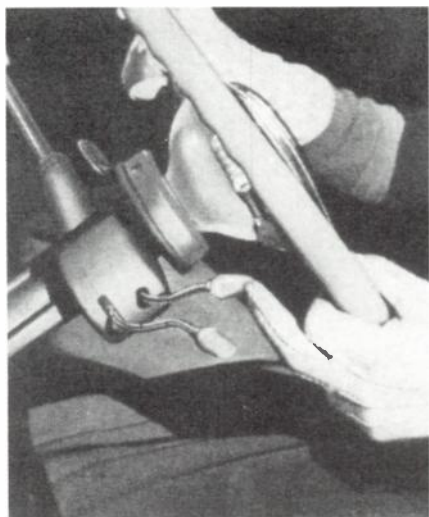
Studebaker's finger control tuning lever was located just above the turn signal lever.
