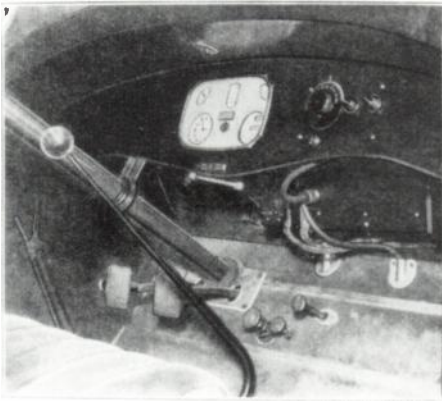
The "Voice of the Road" receiver installed on the firewall of an automobile. The instrument panel controls operate the set by means of the shielded cable.
