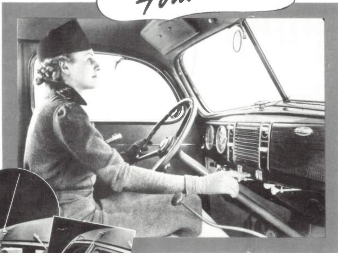
ANTENNA CONTROL HANDLE IS ABOVE REAR VIEW MIRROR, WITHIN EASY REACH OF DRIVER'S SEAT
