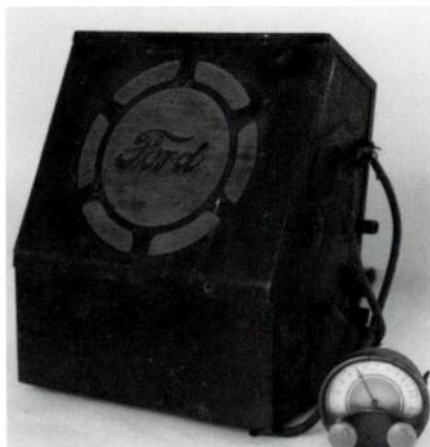
Ford Model FT-6 open car radio showing self-contained speaker.
