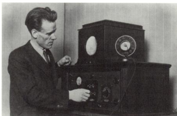
Farnsworth tunes his first prototype of a home TV receiver
