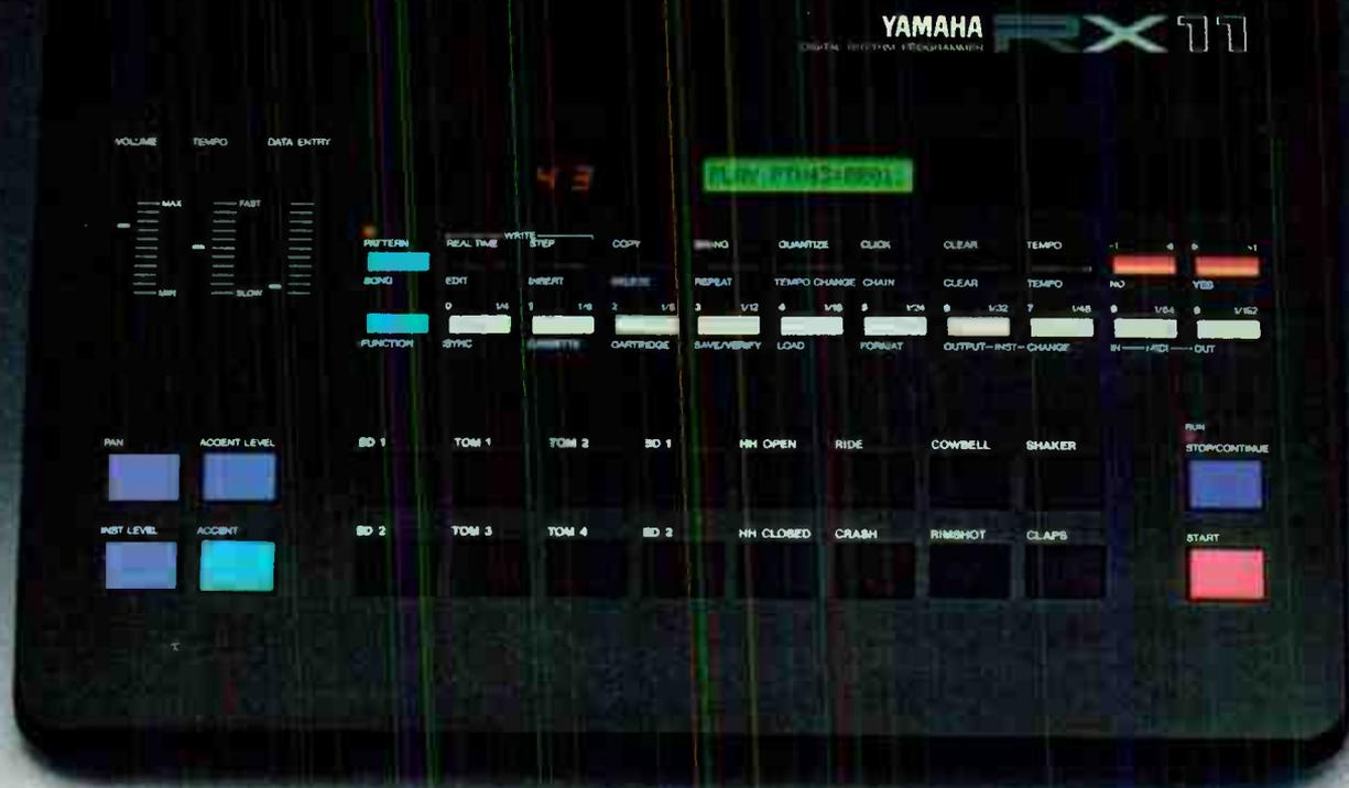
and rearrange any part of the composition. Its built-in disc drive can store up to 80,000 notes on a 5¼" floppy disc.
