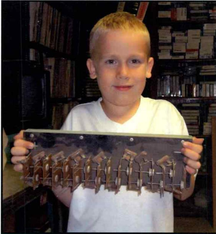
***Anthony Detwiler holding a power supply rectifier board for the Gates FM-5G FM transmitter.***
