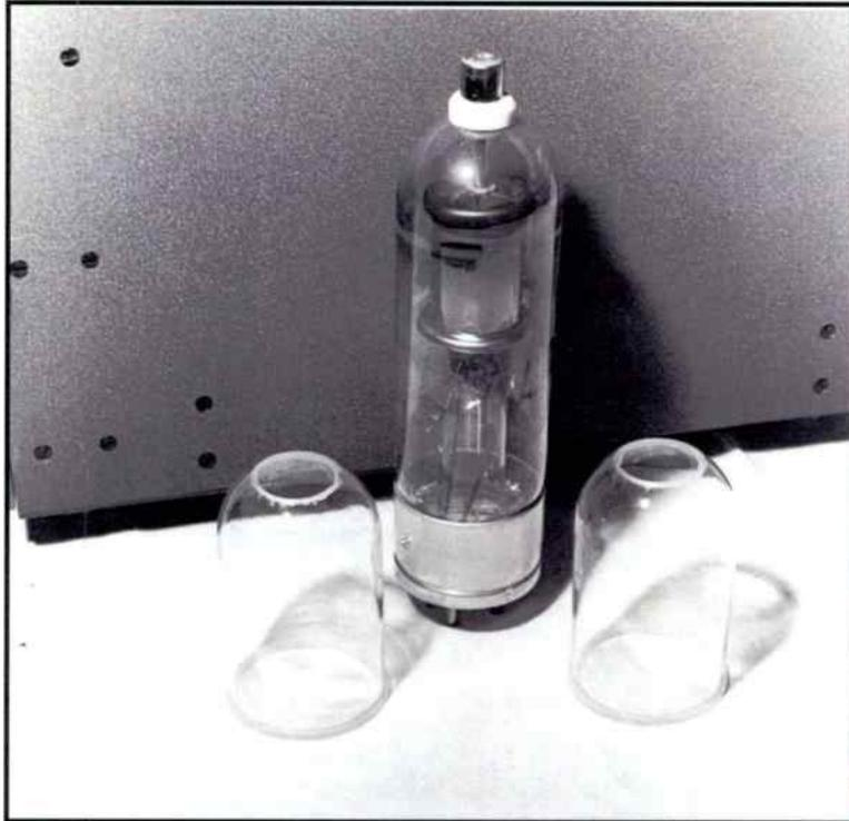
*Picture of a 8008 tube taken from the Gates AM transmitter, saved from the shotgun of Roger Harvey! Beside the tube are two finished glass tube chimneys for the authors' 1500 watt ham radio linear amplifier built in 1975. the homebrew amp. required four chimneys.*
