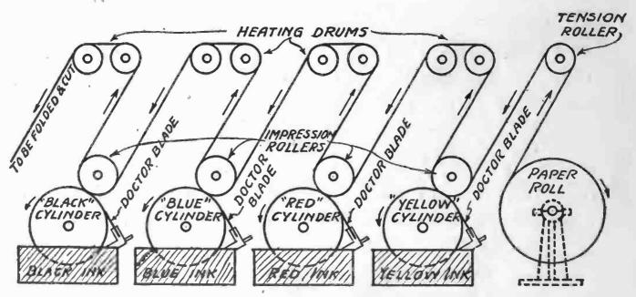
Diagram showing the passage of paper through the COLORoto press.
