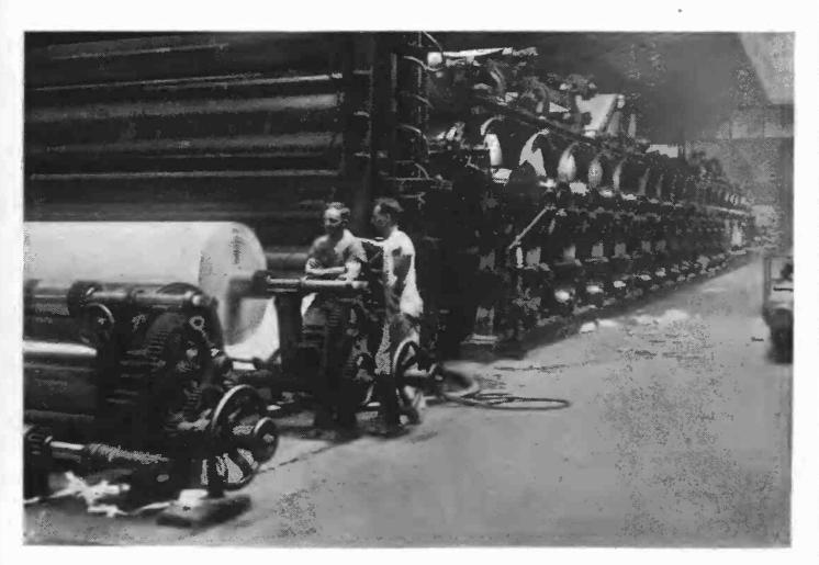
This picture shows, from right to left, the long row of dryers, the calendering stack, the winder, and the rewinder of one of The Tribune's paper machines. THIS picture shows, from right to left, the long row of dryers,
