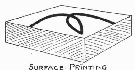
In this process the surface of the printing plate is flat all over. Some parts of the plate take up ink, while other parts, having been chemically treated to resist ink, do not. Lithography and offset printing come under this head.
