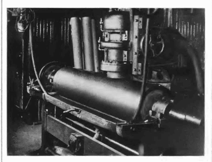
After the COLORoto Magazine is printed, the copper cylinders are re-surfaced so that another set of pages may be etched. The cylinder was made by depositing copper on a steel core in an electrolytic bath.
