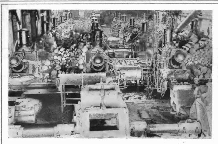
Wood grinding machines in Tribune's paper mill. each machine is a giant grindstone whirling at high speed. Logs are forced against each stone from these turrets. Logs are floated to the machines in tanks, which run from the left to the right of the above picture.
