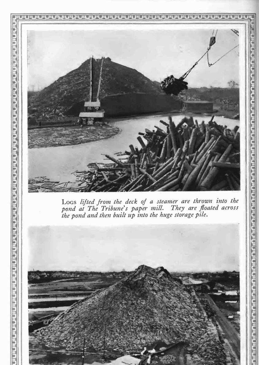
Logs lifted from the deck of a steamer are thrown into the pond at The Tribune's paper mill. They are floated across the pond and then built up into the huge storage pile.
