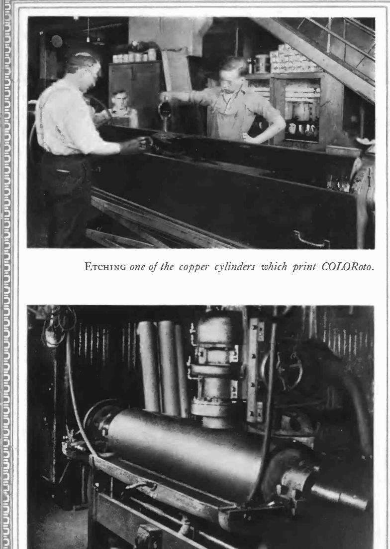
Etching one of the copper cylinders which print COLORoto.
