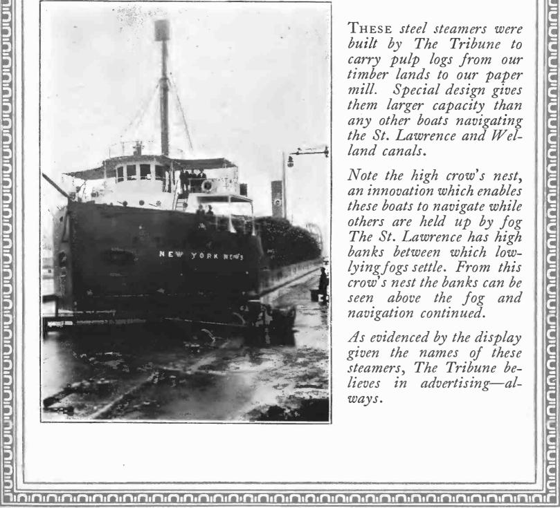
These steel steamers were built by The Tribune to carry pulp logs from our timber lands to our paper mill. Special design gives them larger capacity than any other boats navigating the St. Lawrence and Welland canals.
