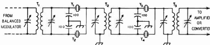
Fig. 11-5—A cascaded half-lattice crystal filter that can be used for sideband selection. The crystals are surplus type in FT-243A holders.  $Y_1$  and  $Y_3$  should be the same frequency and  $Y_2$  and  $Y_4$  should be 1.8 kc. higher.  $T_1, T_2, T_3$ —450-kc. i.f. transformers.
