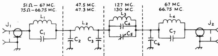
Fig. 23-25—Circuit of the 6-meter low-pass filter. See table for capacitance and inductance values.  $C_1, C_2, C_3, C_4, C_6, C_7$ —6000-volt disk ceramic (Centralab DD60, Sprague 60GA, Erie HD6 or similar).  $C_5$ —45- $\mu\text{f.}$  ceramic trimmer (Centralab 822BN).  $J_1, J_2$ —Chassis-mounting coax receptacle (SO-239). Resonant frequencies refer to the following independent combinations:  $L_1C_1, L_2C_2C_3, L_3C_3C_4$  and  $L_4C_7$ .
