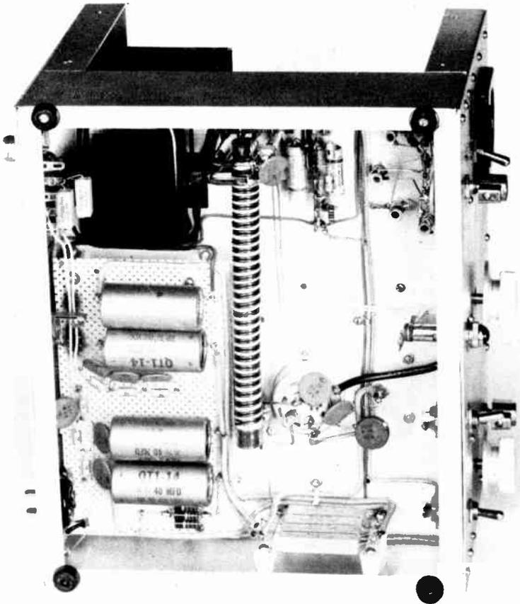
Fig. 6-56—The 811-A socket is mounted below the chassis in a recessed shell. One end of the homemode filament choke is supported near the socket, and the other end is mounted near the transformer. Four 25,000-ohm bleeder resistors (bottom) and two 50-ohm resistors (upper left) are mounted well away from the plate-supply diodes (left) and bias diodes (top center, to right of filament choke).
