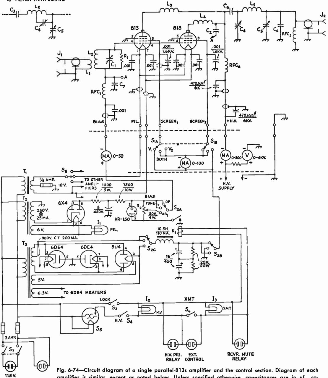
Fig. 6-74—Circuit diagram of a single parallel-813s amplifier and the control section. Diagram of each amplifier is similar, except as noted below. Unless specified otherwise, capacitances are in  $\mu\text{f.}$ , capacitors marked with polarity are electrolytic, fixed capacitors are ceramic, resistances are in ohms.
