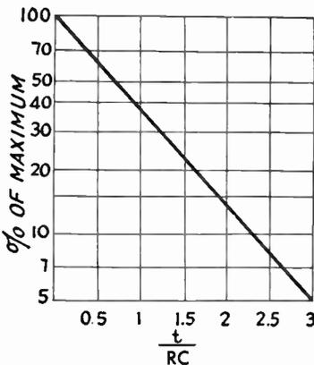
Fig. 2-22—Voltage across capacitor terminals in a discharging RC circuit, in terms of the initial charged voltage. To obtain time in seconds, multiply the factor  $t/RC$  by the time constant of the circuit.
