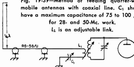
have a maximum capacitance of 75 to 100  $\mu\text{mf.}$  for 50 Mc., and should be adjusted for maximum loading with the least coupling to the transmitter. Some method of varying the coupling to the transmitter should be provided.
