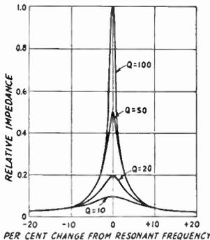
Fig. 2-42.—Relative impedance of parallel-resonant circuits with different  $Q$ s. These curves are similar to those in Fig. 2-42 for current in a series-resonant circuit. The effect of  $Q$  on impedance is most marked near the resonant frequency.
