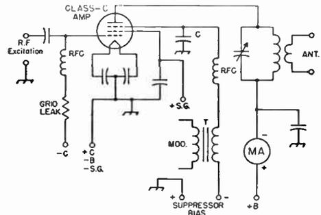
Fig. 10-13—Suppressor-grid modulation of an r.f. amplifier using a pentode-type tube. The suppressor-grid r.f. bypass capacitor,  $C$ , should be the same as the grid bypass capacitor in control-grid modulation.
