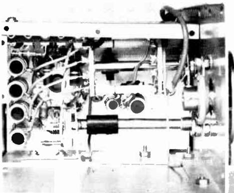
“x” is shown in Fig. 19-24 in each lead that is run through these plugs and sockets. The 11th lead is a ground lead, not necessary when everything is bolted together but useful during the testing stage.
