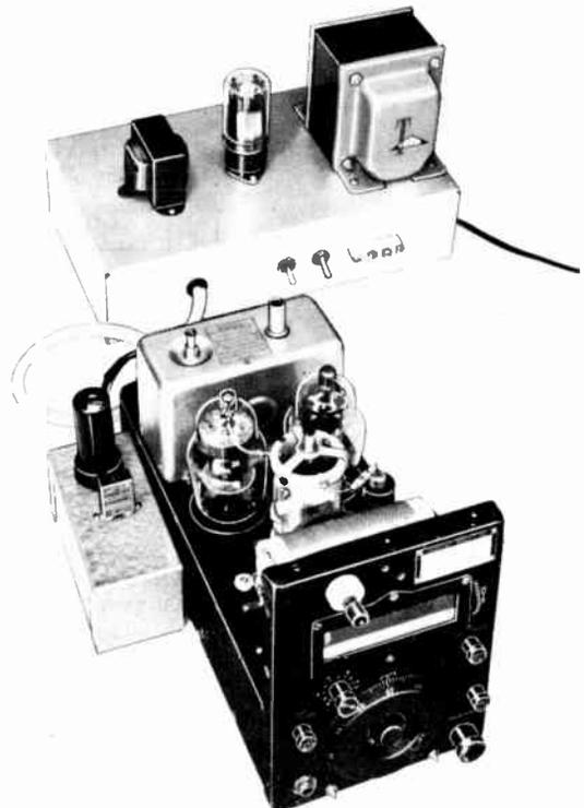
Fig. 6-90—The complete Novice setup, in this case using the 80-meter (BC-696) transmitter. Note the key jack at the lower-left corner of the transmitter panel. The crystal oscillator is connected to the transmitter oscillator-tube socket with a short length of cable terminating in an octal plug. A small notch should be cut in the transmitter cover to provide clearance for the cable when the cover is installed.
