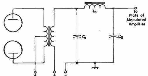
Fig. 9-13—Splatter-suppression filter for use at high level, shown here connected between a Class B modulator and plate-modulated r.f. amplifier. Values for  $L_1$ ,  $C_1$  and  $C_2$  are determined as described in the text.
