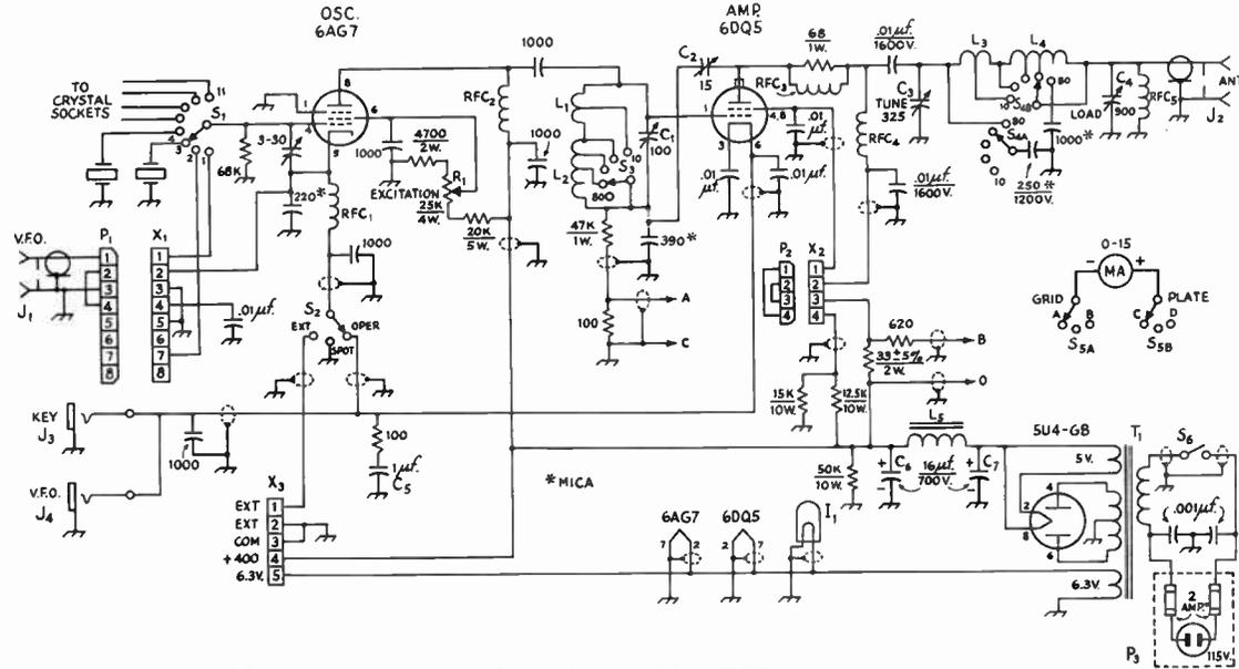
Fig. 6-44—Circuit diagram of the 75-watt 6DQ5 transmitter. Unless specified otherwise, capacitance is in picofarads (pf. or  $\mu\text{mf.}$ ), resistance is in ohms, resistors are  $\frac{1}{2}$  watt.
