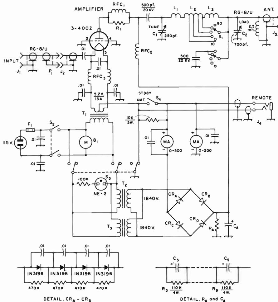
Fig. 6-64—Circuit diagram of the 900-watt p.e.p. grounded-grid amplifier. Unless specified otherwise, capacitances are in  $\mu$ f., resistances are in ohms, resistors are  $\frac{1}{2}$  watt.
