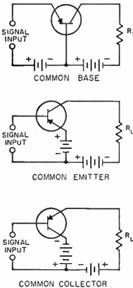
Fig. 4-10—Basic transistor amplifier circuits.  $R_L$ , the load resistance, may be an actual resistor or the primary of a transformer. The input signal may be supplied from a transformer secondary or by resistance-capacitance coupling. In any case it is to be understood that a d.c. path must exist between the base and emitter.
