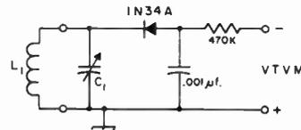
Fig. 21-11—Circuit diagram of the simple wavemeter.  $C_1$ —100- $\mu\text{f}$ . variable (Hammarlund MC-100-M).  $L_1$ —Made from 1-inch diameter, No. 24 wire, 32 t.p.i. coil stock (B&W 3016). See coil table.
