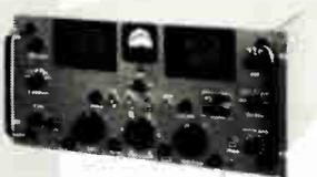
**GPR-92** This receiver is patterned after the field proven GPR-90RXD but incorporates a product detector for the reception of SSB signals and provides selectable IF bandpass up to 15 kc. A very low noise figure provides excellent reception capabilities in ISB, SSB, AM, CW, MCW, FSK and FAX modes of operation. An external oven crystal amplifier, TMC Model TRX-1, provides stable 10 channel HFO crystal selectivity... REQUEST TB 3006
