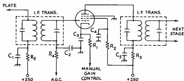
Fig. 5-15—Typical intermediate-frequency amplifier circuit for a superheterodyne receiver. Representative values for components are as follows:  $C_1, C_3, C_4, C_5$ —0.02  $\mu\text{f.}$  at 455 kc.; 0.01  $\mu\text{f.}$  at 1600 kc. and higher.
