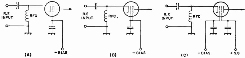
Fig. 6-27—A—Grounded-grid triode input circuit. B—Tetrade input circuit with grid and screen directly in parallel. C—Tetrade circuit with d.c. voltage applied to the screen. Plate circuits are conventional.
