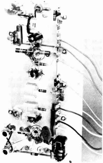
Fig. 17-3—Bottom view of the 50-Mc. transmitter. The oscillator/daubler circuitry is at the bottom of the aluminum plate. All power leads are terminated at the tie points along the right-hand side, and flexible leads run from the tie points to the 15-pin plug on the side of the chassis (not visible).
