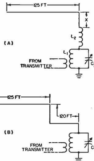
Fig. 14-28—Bent antenna for the 160-meter band. In the system at A, the vertical portion (length  $X$ ) should be made as long as possible. In either antenna system,  $L_1C_1$  should resonate at 1900 kc., roughly. To adjust  $L_2$  in antenna A, resonate  $L_1C_1$  alone to the operating frequency, then connect it to the antenna system and adjust  $L_2$  for maximum loading. Further loading can be obtained by increasing the coupling between  $L_1$  and the link.
