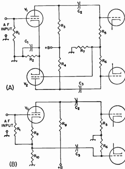
Fig. 9-4—Self-balancing phase-inverter circuits.  $V_1$  and  $V_2$  may be a double triode such as the 12AU7 or 12AX7.  $V_3$  may be any of the triodes listed in Table 9-1, or one section of a double triode.
