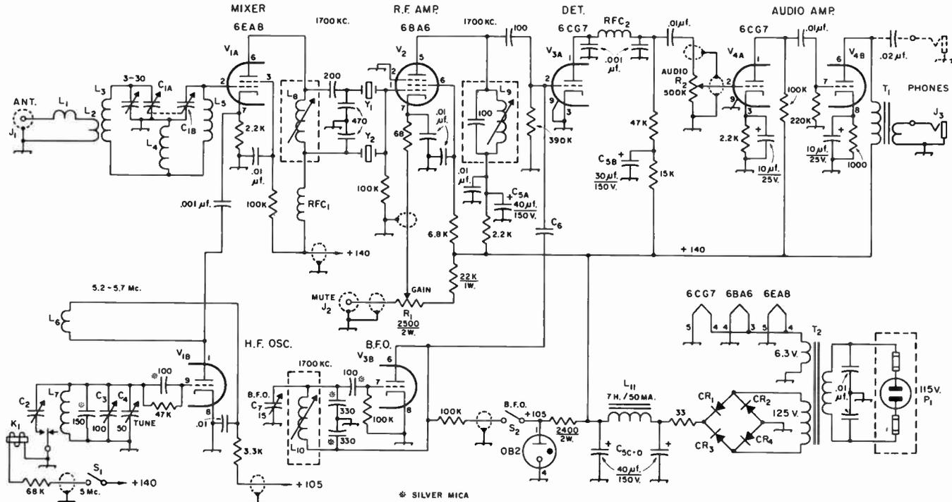
Fig. 5-37—Circuit diagram of the 2X4+ receiver. Unless otherwise indicated, capacitances are in pf. (picofarads or  $\mu\mu\text{f.}$ ), resistances are in ohms, resistors are  $\frac{1}{2}$ -watt. Capacitors marked with polarity are electrolytic; those marked with asterisk are silver mica.
