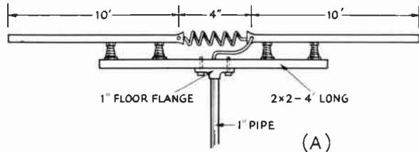
Fig. 14-59—(A) Diagram of the 21-Mc. antenna and mounting. The U-bolts that hold the 2 by 2 to the floor flange are standard 2-inch TV mast type bolts. (B) A more detailed drawing of the coil and coax-fitting mountings. The 1/4-inch spacing between turns is not critical, and they can vary as much as 1/16 inch without any apparent harm to the match.
