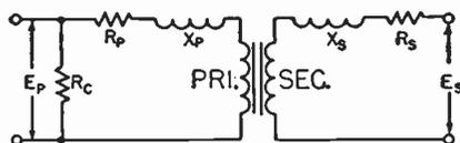
Fig. 2-33—The equivalent circuit of a transformer includes the effects of leakage inductance and resistance of both primary and secondary windings. The resistance  $R_c$  is an equivalent resistance representing the core losses, which are essentially constant for any given applied voltage and frequency. Since these are comparatively small, their effect may be neglected in many approximate calculations.
