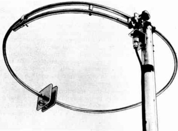
Tuning up at 145 Mc., for example, will give quite satisfactory operation from the low end to 146 Mc., the halo being much broader in frequency response when it is operated on its third harmonic. In this model the series capacitor in the gamma arm was at about the middle of its range for 50 Mc., and near minimum for 144 Mc. Slight differences in mechanical construction may change the value of capacitance required, so these settings should not be taken as important.
