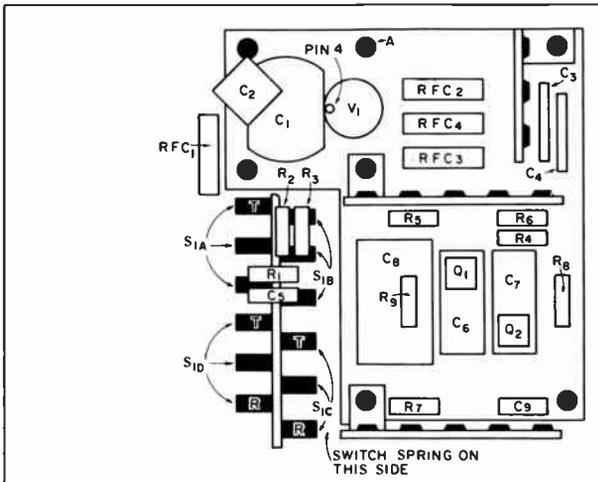
Fig. 16-21—Location of components on the clear plastic sheet. One 3-terminal and two 5-terminal tie-point strips are required.
