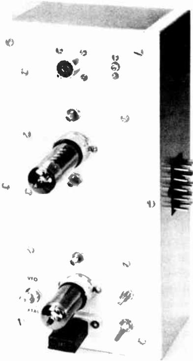
Fig. 17-2—Top view of the 50-Mc. transmitter. The toggle switch at the lower left changes the input circuit for crystal or v.f.o. operation; when used, the v.f.o. output is introduced at the crystal socket.
