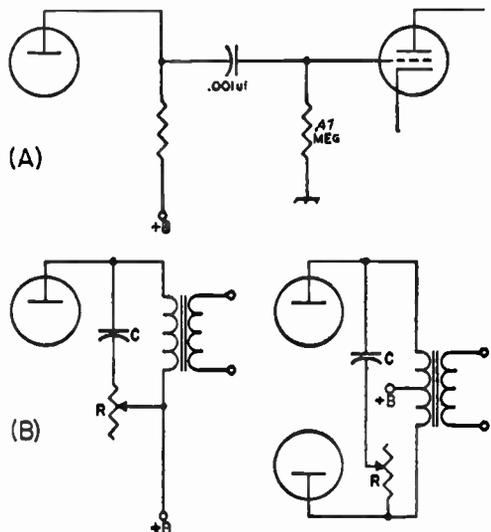
Fig. 9-10—A, use of a small coupling capacitor to reduce low-frequency response; B, tone-control circuits for reducing high-frequency response. Values for C and R are discussed in the text; 0.01  $\mu$ f. and 25,000 ohms are typical.
