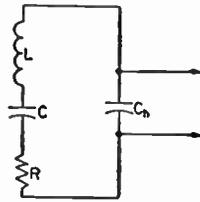
450 kc., where crystals are widely used as resonators, the equivalent  $L$  may be several henrys and the equivalent  $C$  only a few hundredths of a micromicrofarad. Although the equivalent  $R$  is of the order of a few thousand ohms, the reactance at resonance is so high that the  $Q$  of the crystal likewise is high.
