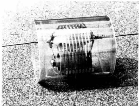
Fig. 14-25—Method of connecting the antenna wire to the strain insulator. The antenna wire is cut off close to the wrap before checking the resonant frequency of the trap.
