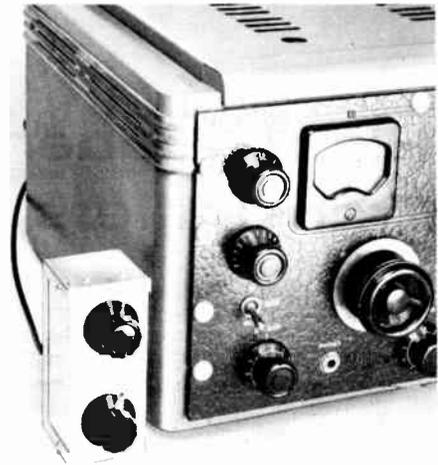
Fig. 5-60—View of the Q multiplier showing its single connecting cable to the receiver. The box can be placed in any convenient spot on or around the receiver.
