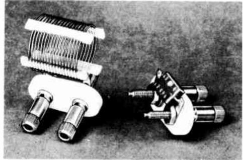
Fig. 21-37—A convenient mounting, using binding-post plates, for  $L$  and  $C$  standards made from commercially-available parts. The capacitor is a  $100\text{-}\mu\mu f.$  silver mica unit, mounted so the lead length is as nearly zero as possible. The inductance standard,  $5 \mu h.$ , is 17 turns of No. 3015 B & W Miniductor, 1-inch diameter, 16 turns per inch.
