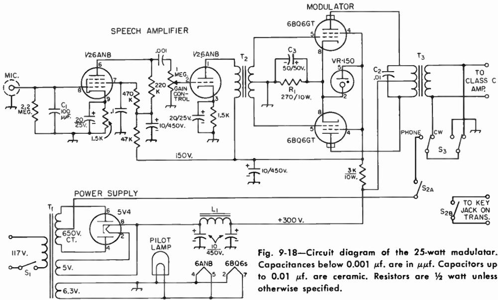
Fig. 9-18—Circuit diagram of the 25-watt modulator. Capacitances below 0.001  $\mu\text{f.}$  are in  $\mu\text{mfd.}$  Capacitors up to 0.01  $\mu\text{f.}$  are ceramic. Resistors are  $\frac{1}{2}$  watt unless otherwise specified.
