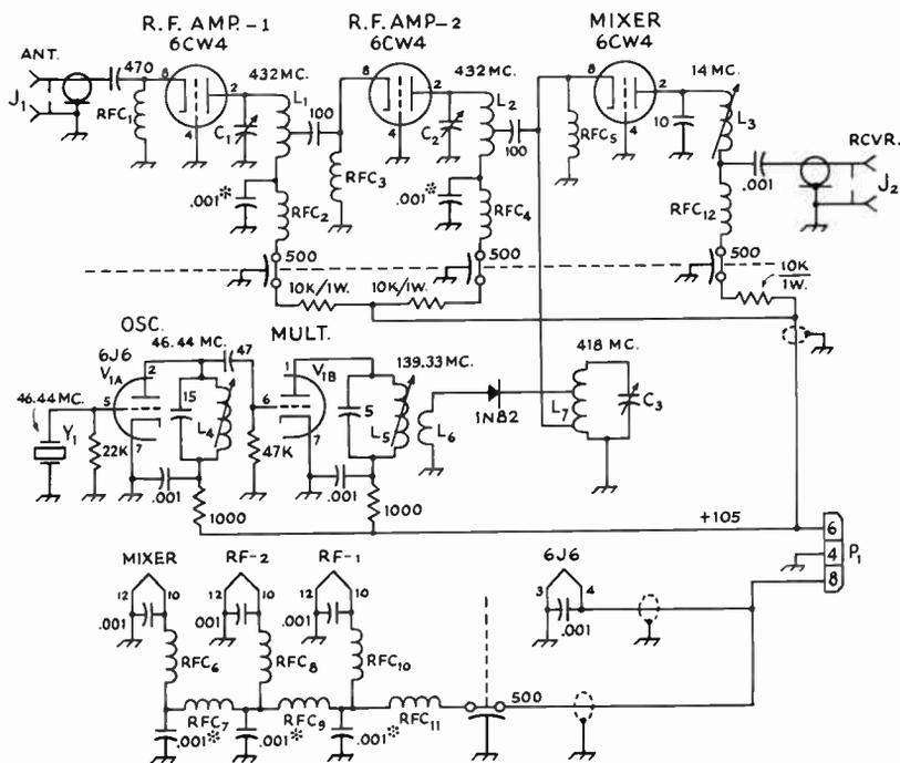
Fig. 16-24—Wiring diagram of the 432-Mc. converter. Capacitance values are in  $\mu\text{mf.}$ , except decimal values which are in  $\mu\text{f.}$  Resistors are  $\frac{1}{2}$  watt unless specified otherwise. All 0.001- $\mu\text{f.}$  capacitors marked \* are button-type (Centralab ZA-102); other 0.001- $\mu\text{f.}$  capacitors are disk ceramic. All 500- $\mu\text{mf.}$  feedthrough capacitors are Centralab FT-500.
