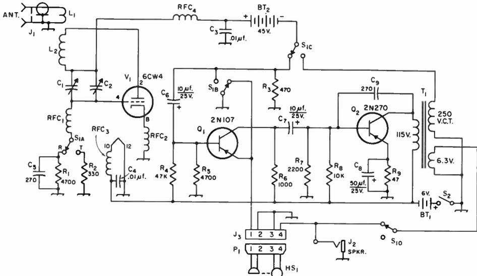
Fig. 16-18—Circuit diagram of the 420-Mc. transceiver. Unless specified otherwise, capacitances are in picofarads (pf. or  $\mu\text{mf.}$ ), resistances are in ohms, resistors are  $\frac{1}{2}$  watt. Capacitors marked with polarity are electrolytic.
