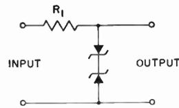
Fig. 4-5—Full-wave clipping action with two zener diodes in opposition. The output level would be at a peak-to-peak voltage of twice the zener rating of a single diode.  $R_1$  should have a resistance value sufficient to limit the current to the zener diode rating.
