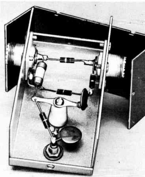
Fig. 21-43—An inexpensive bridge for matching adjustments using the circuit of Fig. 21-42. It is built in a  $1\frac{1}{2} \times 2\frac{1}{2} \times 4$ -inch "Channel-lock" box. The standard resistor,  $R_3$ , bridges the two coax connectors. A pin jack is provided for connection to the d.c. meter, 0-1 ma. or 0-500  $\mu$ a.; the meter negative can be connected to the case or to one of the coax fittings.
