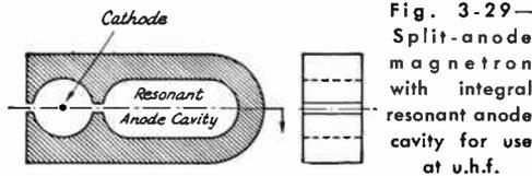
Fig. 3-29—Split-anode magnetron with integral resonant anode cavity for use at u.h.f.
