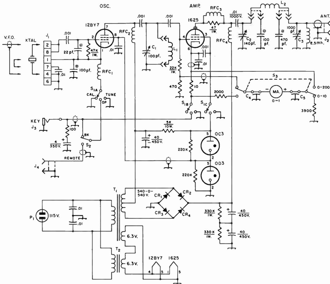
Fig. 6-40—Circuit diagram of the inexpensive 75-watt transmitter. Unless indicated otherwise, all resistors are 1/2-watt, all resistances are in ohms, all capacitances are in  $\mu\text{f}$ . Electrolytic capacitors are marked with polarity, mica capacitors are marked with \*, other fixed capacitors under 0.1  $\mu\text{f}$ . are ceramic.
