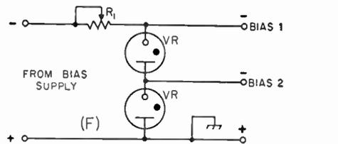
Fig. 7-29—Illustrating the use of VR tubes in stabilizing protective-bias supplies.  $R_1$  is a resistor whose value is adjusted to limit the current through each VR tube to 5 ma. before amplifier excitation is applied.  $R$  and  $R_2$  are current-equalizing resistors of 50 to 1000 ohms.
