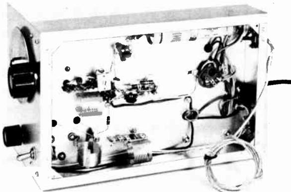
Fig. 5-41—Bottom view of the converter showing placement of parts. The coil at the lower left is  $L_3$ , and the input coil,  $L_1L_2$ , is just to the right of  $L_3$ . The oscillator coil  $L_4L_5$  is at the left near the center. The output coil,  $L_6$ , is near the top center.
