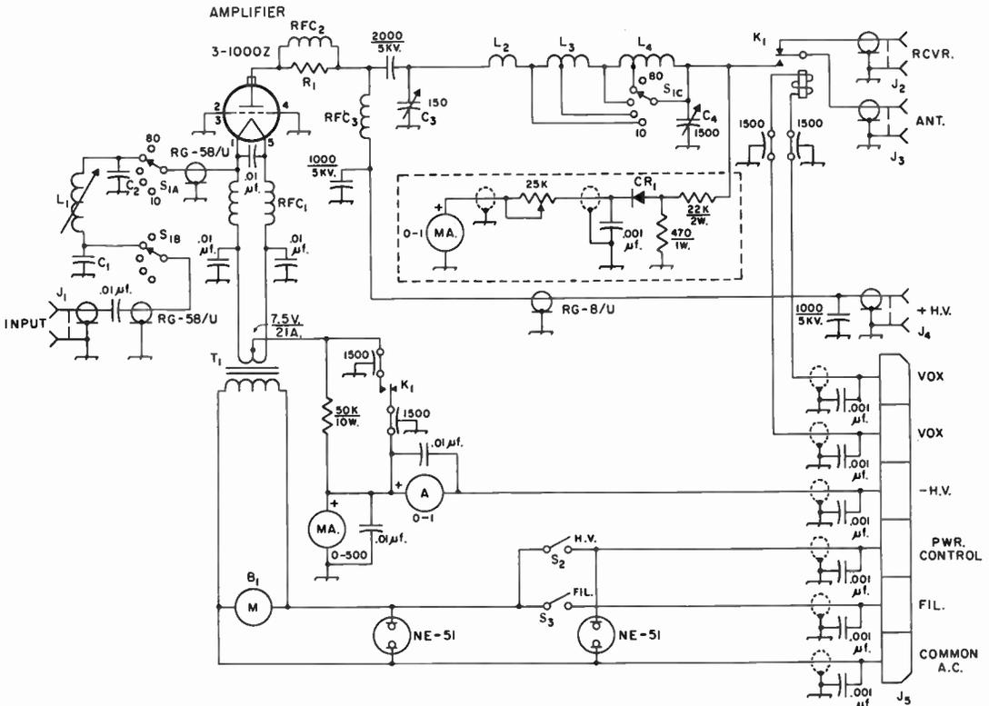
Fig. 6-79—Circuit diagram of the 3-1000Z amplifier. Unless specified otherwise, capacitances are in picotaras (pf. or  $\mu\text{mf.}$ ). For simplicity, only one set of components is shown at  $S_{1A-B}$ .
