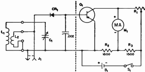
Fig. 21-39—Transistor d.c. amplifier applied to the wavemeter of Fig. 21-10 to increase sensitivity. Components not listed below are the same as in Fig. 21-10.  $B_1$ —Small flashlight cell.  $M_1$ —0-1 d.c. milliammeter (see text).  $Q_1$ —2N107, CK722, etc.  $R_1$ —10,000-ohm control.
