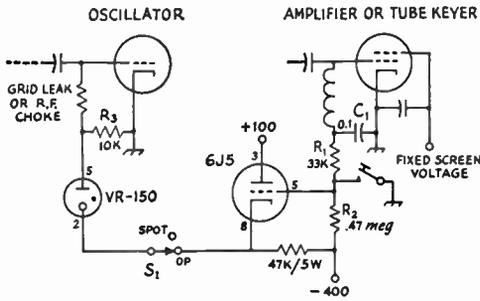
Fig. 8-7—When satisfactory blocked-grid or tube keying of an amplifier stage has been obtained, this VR-tube break-in circuit can be applied to the transmitter to furnish differential keying. The constants shown here are suitable for blocked-grid keying of a 6146 amplifier; with a tube keyer the 6J5 and VR tube circuitry would be the same.
