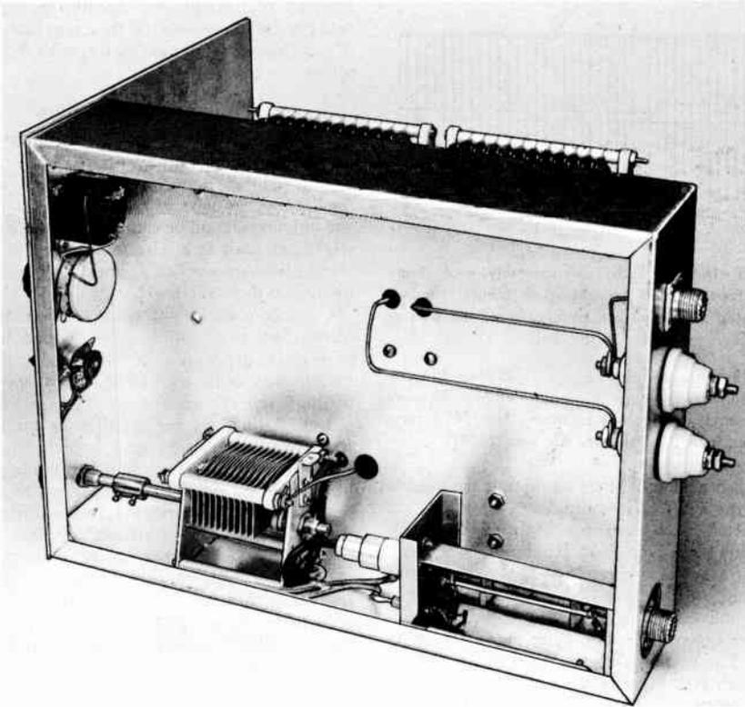
Fig. 13-18—The link capacitor and the Manimatch are mounted underneath the chassis.
