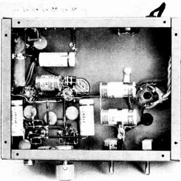
Fig. 9-16—Below-chassis view of the modulator. The rectifier tube socket and electrolytic filter capacitors are at the right in this view. The 12AX7 socket is at the lower left. Bleeder resistor R<sub>5</sub> is at the upper left, near the 6-terminal connection strip on the rear edge of the chassis. Placement of components is not critical, but the leads in the first two stages should be kept short and close to the chassis to minimize hum troubles.
