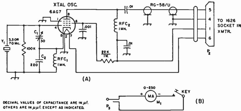
Fig. 6-92—(A) Circuit diagram of external crystal-controlled oscillator. Unless otherwise specified, resistances are in ohms, resistors are 1/2 watt. The 0.01- and 0.001-μf. capacitors are disk ceramic. (B) Method of connecting the milliammeter in series with the key.
