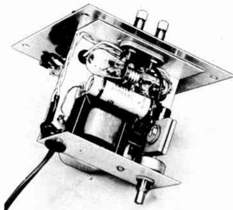
Fig. 21-20—Bottom view of the audio oscillator, showing the power-supply components and amplitude-control lamp, *I*<sub>1</sub>. The lamp is mounted by wires soldered to its base. The selenium rectifier is supported by a tie-point strip. Placement of resistors, which are hidden by the other components, is not critical. The unit fits in a 4 × 5 × 6 inch box.
