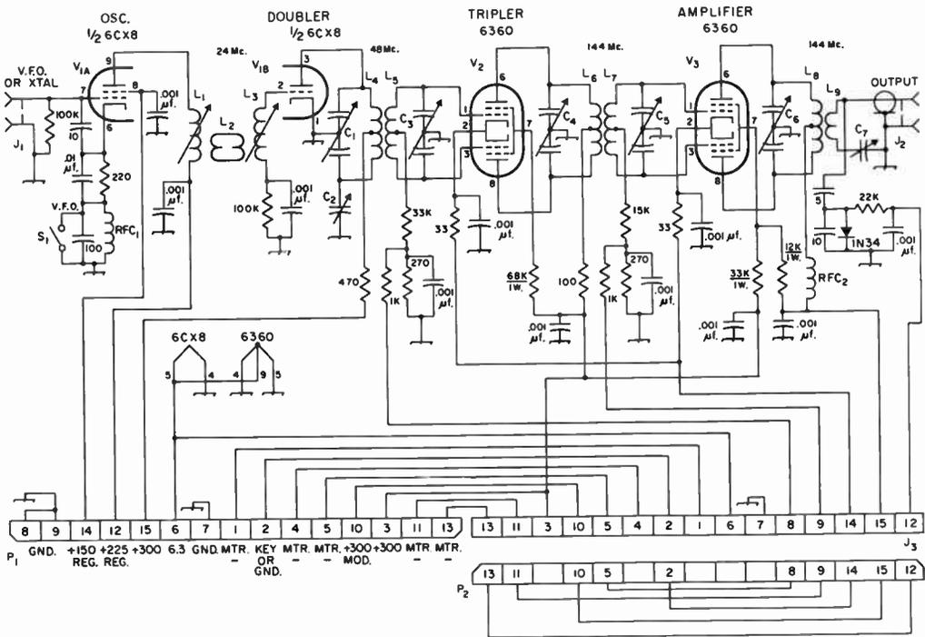
Fig. 17-7—Circuit diagram of the 144-Mc. transmitter. Unless specified otherwise, capacitances are in picofarads (pf. or  $\mu\text{mf.}$ ), resistances are in ohms, resistors are  $\frac{1}{2}$  watt.  $P_2$  plugs into  $J_3$  for 144-Mc. operation.
