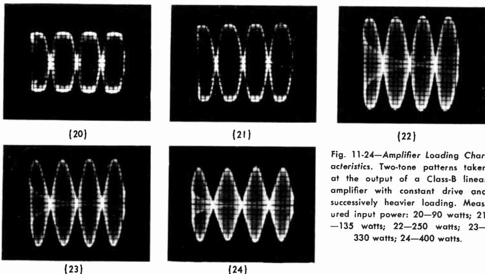
Fig. 11-24—Amplifier Loading Characteristics. Two-tone patterns taken at the output of a Class-B linear amplifier with constant drive and successively heavier loading. Measured input power: 20—90 watts; 21—135 watts; 22—250 watts; 23—330 watts; 24—400 watts.
