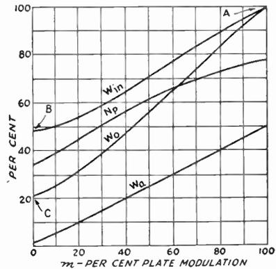
Fig. 10-16—Cathode-modulation performance curves, in terms of percentage of plate modulation plotted against percentage of Class C telephony tube ratings.  $W_{1a}$ —D.c. plate input watts in terms of percentage of plate-modulation rating.
