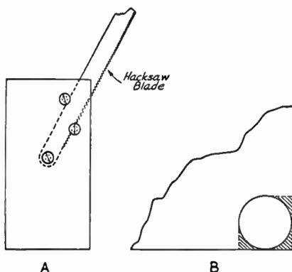
Fig. 20-2—To cut rectangular holes in a chassis corner, holes may be filed out as shown in the shaded portion of B, making it possible to start the hack-saw blade along the cutting line. A shows how a single-ended handle may be constructed for a hack-saw blade.
