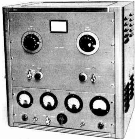
Fig. 6-67—The kilowatt 4-400A amplifier and its control unit are mounted in a 21-inch gray hammerstone rack cabinet (Bud CR-1727). Shelf brackets (Bud SA-1350) are mounted on both sides of the cabinet to hold the amplifier chassis. Below the meters, from left to right: filament pilot light, key-type a.c. switch, Class AB<sub>1</sub>/C bias switch, screen autotransformer, plate switch and plate pilot light.
