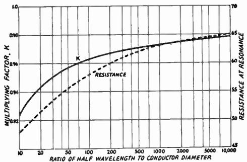
Fig. 14-3—Effect of antenna diameter on length for half-wave resonance, shown as a multiplying factor, *K*, to be applied to the free-space half wavelength (Equation 14-A). The effect of conductor diameter on the center impedance also is shown.
