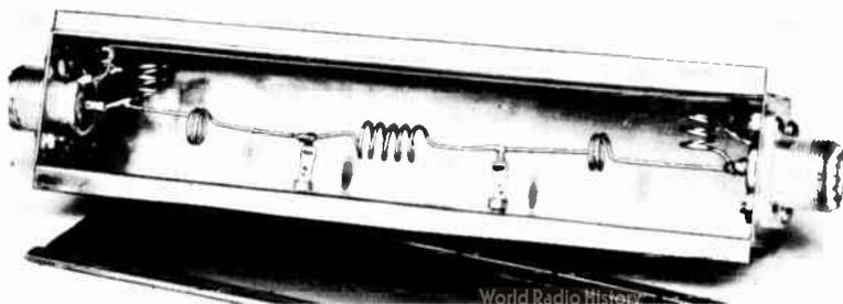
Fig. 23-26—A 52-ohm low-pass filter for 144-Mc. Transmitters. Case is made from flashing copper and is  $1\frac{1}{4}$  inches square by  $7\frac{1}{2}$  inches long. Cover slips on flanges folded out at the bottom; ends are folded down and soldered.
