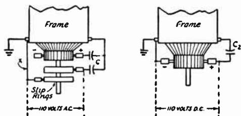
Fig. 19-50—Connections used for eliminating interference from gas-driven generator plants. C should be 1  $\mu$ f., 300 volts, paper, while C<sub>2</sub> may be 1  $\mu$ f. with a voltage rating of twice the d.c. output voltage delivered by the generator. X indicates an added connection between the slip ring on the grounded side of the line and the generator frame.
