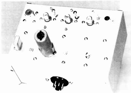
Fig. 16-23—The 432-Mc. converter is built in a 5 X 7 X 3-inch Minibox. At the top in this view, from left to right: input jack, r.f. amplifier, r.f. amplifier, mixer, output jack. The tube (shielded) is a 6J6, used as crystal oscillator and frequency multiplier.
