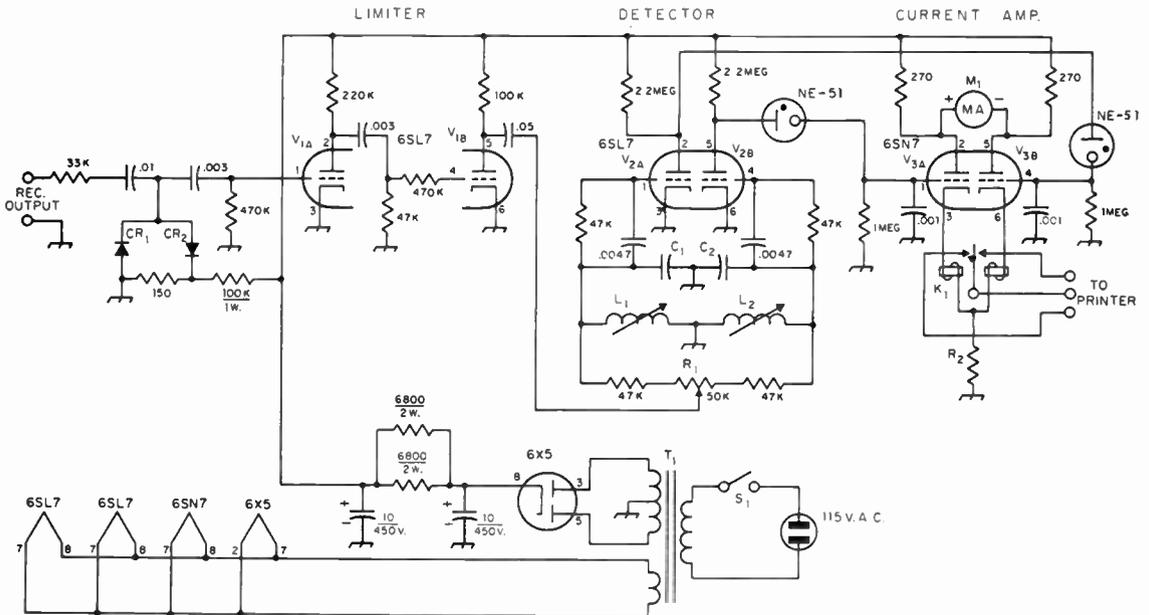
Fig. 12-12—Receiving converter for f.s.k. teletype signals (W2PAT). Unless otherwise indicated, capacitances are in  $\mu\text{f}$ . resistances are in ohms, resistors are  $\frac{1}{2}$  watt. Capacitors of 0.01  $\mu\text{f}$ . or less may be mica or ceramic; larger values may be paper. Capacitors with polarities indicated are electrolytic.
