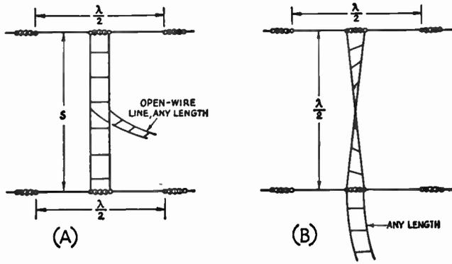
Broadside arrays may be fed either by tuned open-wire lines or through quarter-wave matching sections and flat lines. In Fig. 14-30B, note the "crossing over" of the phasing section, which is necessary to bring the elements into proper phase relationship.
