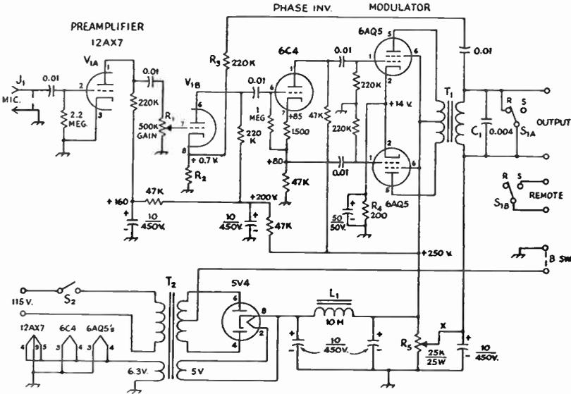
Fig. 9-15—Circuit of the speech amplifier and modulator. All capacitances are in  $\mu\text{f}$ .; capacitors with polarities marked are electrolytic, others are ceramic. Resistors are  $\frac{1}{2}$  watt except as noted below. Voltages measured to chassis with v.t. vultmeter.
