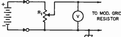
Fig. 12-4—D.c. method of checking frequency deviation of a reactance-tube-modulated oscillator. A 500- or 1000-ohm potentiometer may be used at R<sub>1</sub>.
