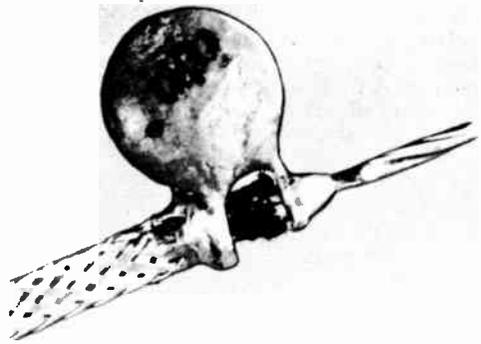
Fig. 23-9—Proper method of bypassing the end of a shielded lead using disk ceramic capacitor. The 0.001- $\mu$ f. size should be used for 1600 volts or less; 500  $\mu$ f. at higher voltages. The leads are wrapped around the inner and outer conductors and soldered, so that the lead length is negligible. This photograph is about four times actual size.
