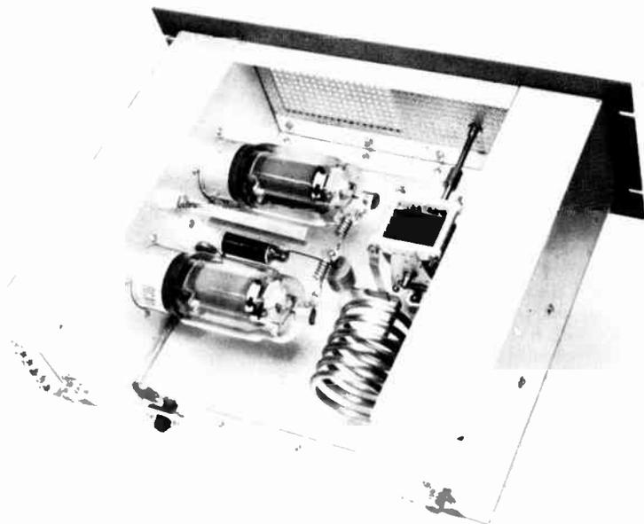
Fig. 6-76—Top view of the 15-meter amplifier. The neutralizing capacitor consists of two strips of aluminum, supported by the plate-blacking capacitor and a feedthrough insulator. It is mounted over the r.f. choke between the two 813 tubes.
