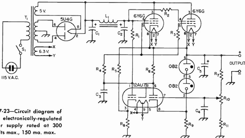
Fig. 7-23—Circuit diagram of an electronically-regulated power supply rated at 300 volts max., 150 ma. max.
