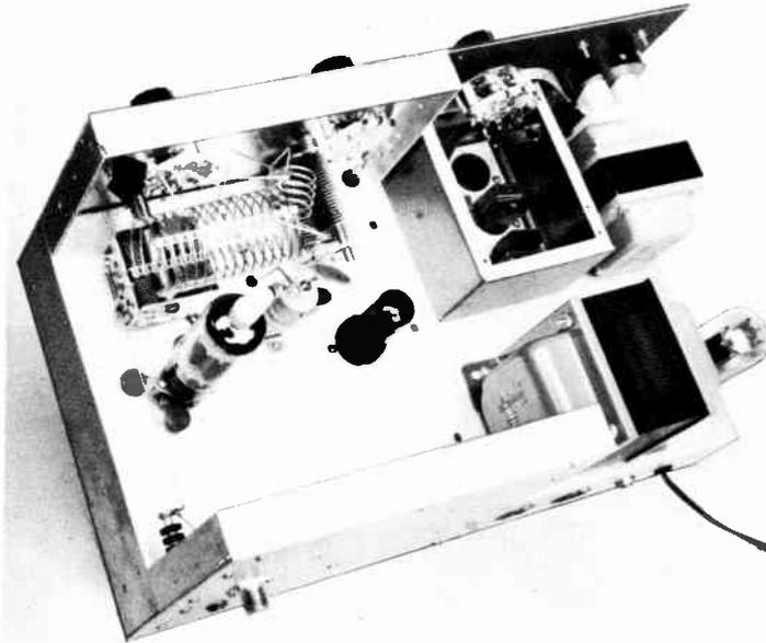
Fig. 6-45—Top view of the 6DQ5 transmitter with cone-metal cover removed. A  $3 \times 4 \times 5$ -inch utility box (upper right) serves as a shield for the crystals; the cane-metal protection for the meter switch is fastened to the box cover. Phono jack mounted on the meter-side of the box receives v.f.o. output; short length of Twin-Lead from this jack to octal plug brings v.f.o. output to crystal socket.
