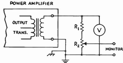
Fig. 9-31—Circuit for measuring power and making qualitative checks of the amplifier output. Values to be used for R<sub>1</sub> and R<sub>2</sub> are discussed in the text. The secondary winding of the output transformer in the amplifier should be disconnected from any d.c. source in the unit and one end connected to chassis as shown. An earth ground should be used on the system.
