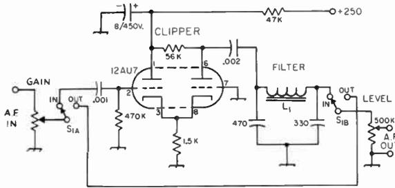
Fig. 9-12—Practical speech clipper circuit with low-pass filter. Capacitances below 0.001  $\mu\text{f.}$  are in  $\mu\text{m.f.}$  Resistors are  $\frac{1}{2}$  watt.  $L_1$ —20 henrys, 900 ohms (Stancor C-1515).  $S_1$ —D.-p.d.t. toggle or rotary.
