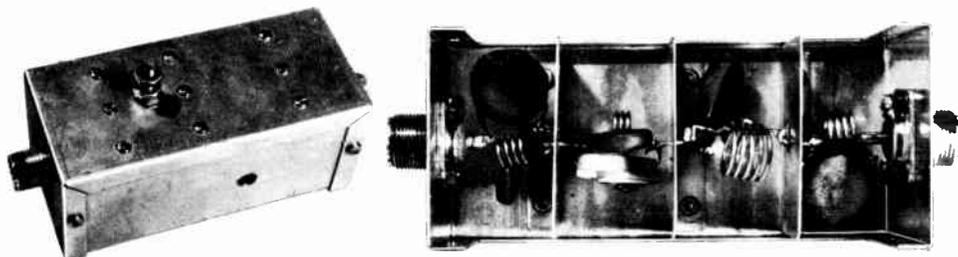
Fig. 23-24—Low-pass filter for use with 50-Mc. transmitters at powers up to about 300 watts. The housing is a 2¼-inch square by 5-inch long Minibox. Connections between the various sections of the filter are made through 5/16-inch clearance holes cut in the centers of the shielding partitions.
