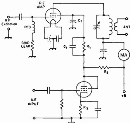
Fig. 10-11—Screen modulation by a "clamp" tube. The grid leak is the normal value for c.w. operation and  $C_2$  should be  $0.002 \mu\text{f.}$  or less. See text for discussion of  $C_1$ ,  $R_1$ ,  $R_2$  and  $R_3$ .  $R_3$  should have the proper value for Class A operation of the modulator tube, but cannot be calculated unless triode curves for the tube are available.
