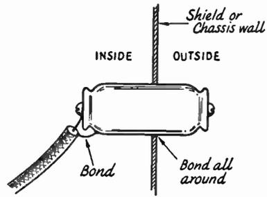
Fig. 23-13—The best method of using the "Hypass" type feed-through capacitor. Capacitances of 0.01 to 0.1  $\mu$ f. are satisfactory. Capacitors of this type are useful for high-current circuits, such as filament and 115-volt leads, as a substitute for the r.f. choke shown in Fig. 23-11, in cases where additional lead filtering is needed.
