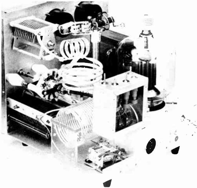
Fig. 6-80—Rear view of the 3-1000Z amplifier with the back wall and SK-516 chimney removed. The 4 × 4 × 2-inch box in the foreground houses the pi-network input circuits and band-switch sections. S<sub>1A-B</sub>. The antenna changeover relay is mounted directly below.
