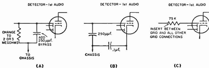
The cause is rectification of the signal in an audio circuit.
