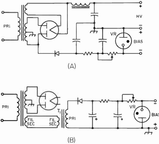
Fig. 7-31—Convenient means of obtaining biasing voltage. A—From a low-voltage plate supply. B—From spare filament winding.  $T_1$  is a filament transformer, of a voltage output similar to that of the spare filament winding, connected in reverse to give 115 volts r.m.s. output.
