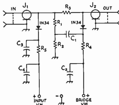
Fig. 21-41—Bridge circuit for s.w.r. measurements. This circuit is intended for use with a d.c. voltmeter, range 5 to 10 volts, having a resistance of 10,000 ohms per volt or greater.
