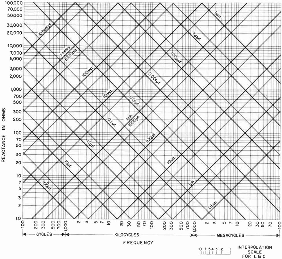
Fig. 2-28—Inductive and capacitive reactance vs. frequency. Heavy lines represent multiples of 5; e.g., the light line between 10  $\mu$ h. and 100  $\mu$ h. represents 50  $\mu$ h., the light line between 0.1  $\mu$ f. and 1  $\mu$ f. represents 0.5  $\mu$ f., etc. Intermediate values can be estimated with the help of the interpolation scale shown.
