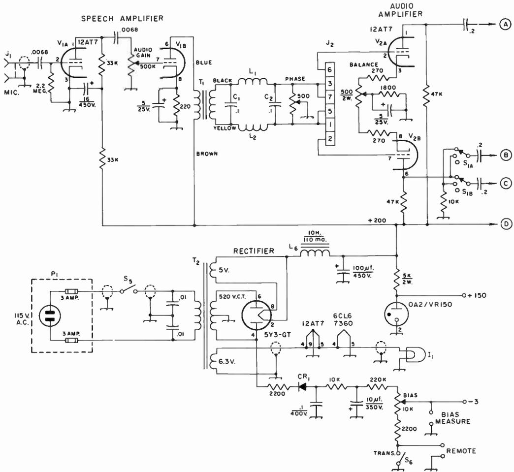
Fig. 11-12—Schematic diagram of the sideband generator. Unless specified otherwise, resistors are 1/2-watt, .01- and .002-μf. capacitors are disk ceramic, 600 volts; .1- and .2-μf. capacitors are tubular paper, 400 volts; capacitors marked with polarities are electrolytic.
