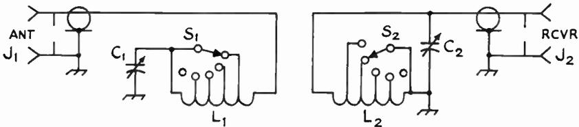
Fig. 5-46—Circuit diagram of the receiver antenna coupler.
