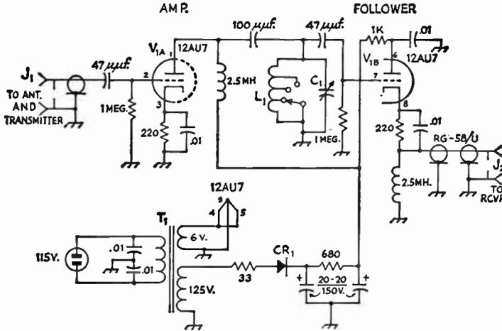
Fig. 8-17—Circuit diagram of the electronic t.r. switch.
