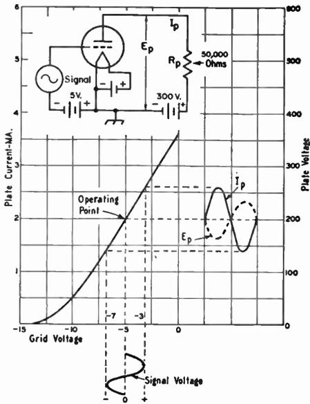
Fig. 3-8—Amplifier operation. When the plate current varies in response to the signal applied to the grid, a varying voltage drop appears across the load,  $R_p$ , as shown by the dashed curve,  $E_p$ .  $I_p$  is the plate current.
