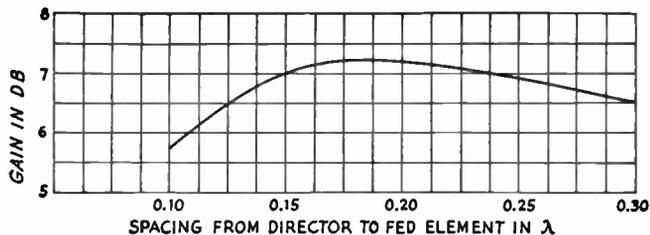
With 0.2 wavelength reflector spacing, Fig. 14-35 shows the gain variation with director spacing. It is obvious that the director spacing is not especially critical, and that the over-all length of the array (boom length in the case of a rotatable antenna) can be anywhere between 0.35 and 0.45 wavelength with no appreciable difference in gain.
