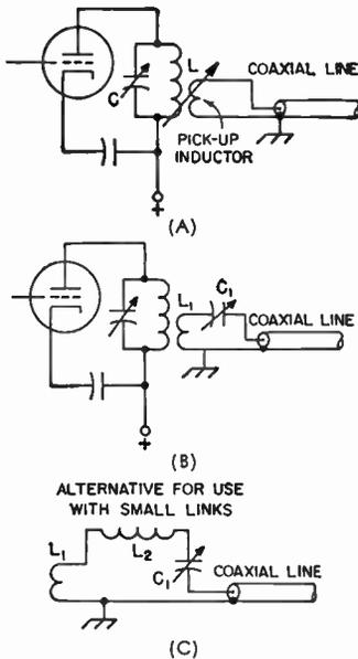
Fig. 6-11—With flat transmission lines, power transfer is obtained with looser coupling if the line input is tuned to resonance.  $C_1$  and  $L_1$  should resonate at the operating frequency. See table for maximum usable value of  $C_1$ . If circuit does not resonate with maximum  $C_1$  or less, inductance of  $L_1$  must be increased, or added in series at  $L_2$ .
