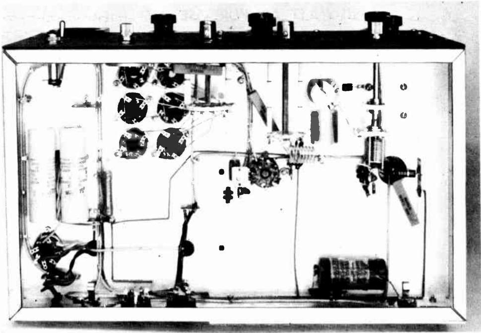
Fig. 6-46—Group of six octal sockets (upper left) serves as crystal sockets. Socket at center of chassis holds 6AG7 oscillator tube; the 3–30-pf. mica compression trimmer mounted alongside is excitation control for oscillator stage. Small midget capacitor above coil is neutralizing capacitor adjusted from above chassis; this capacitor and grid tuning capacitor to right must be insulated from chassis.
