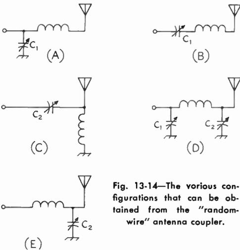
Fig. 13-14—The various configurations that can be obtained from the "random-wire" antenna coupler.
