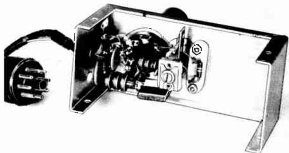
Fig. 6-93—This bottom view of the crystal oscillator shows the arrangement of components. Terminal strips are used for the cable connections and also as a support for  $C_1$ , the feedback capacitor.
