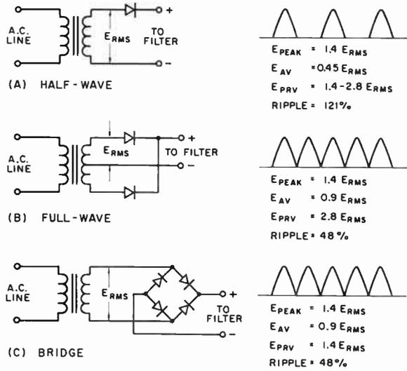
Fig. 7-1—Fundamental rectifier circuits. A—Half-wave ( $E_{PRV} = 1.4 E_{RMS}$  with resistive load,  $= 2.8 E_{RMS}$  with capacitor-input filter). B—Full-wave. C—Full-wave bridge. Output voltage values do not include rectifier voltage drops.
