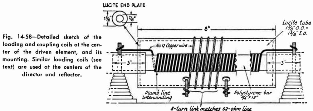
Fig. 14-58—Detailed sketch of the loading and coupling coils at the center of the driven element, and its mounting. Similar loading coils (see text) are used at the centers of the director and reflector.
