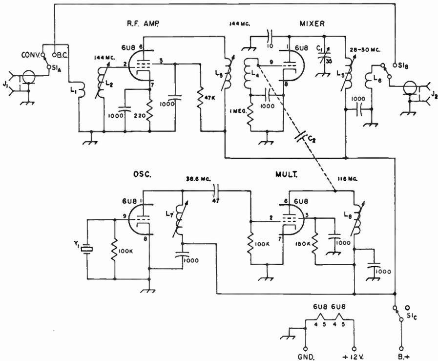
Fig. 19-13—Schematic diagram for the 144-Mc. converter. All resistors  $\frac{1}{2}$  watt unless otherwise specified. Capacitor values below  $0.001 \mu\text{f.}$  are in  $\mu\mu\text{f.}$  All  $1000\text{-}\mu\mu\text{f.}$  capacitors are disk ceramic. Other fixed capacitors are tubular ceramic.
