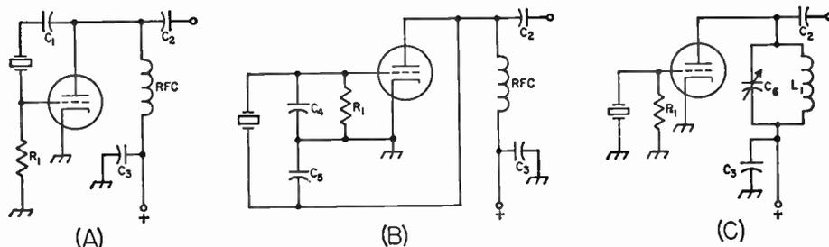
Fig. 6-2—Simple crystal oscillator circuits. A—Pierce. B—Equivalent of circuit A. C—Simple triode oscillator.  $C_1$  is a plate blocking capacitor,  $C_2$  an output coupling capacitor, and  $C_3$  a plate bypass.  $C_4$  and  $C_5$  are discussed in the text.  $C_6$  and  $L_1$  should tune to the crystal fundamental frequency.  $R_1$  is the grid leak.
