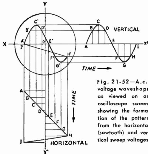
Fig. 21-52—A.c.-voltage waveshape as viewed on an oscilloscope screen, showing the formation of the pattern from the horizontal (sawtooth) and vertical sweep voltages.
