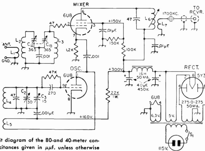
Fig. 5-40—Circuit diagram of the 80- and 40-meter converter. All capacitances given in  $\mu\text{f.}$  unless otherwise noted.
