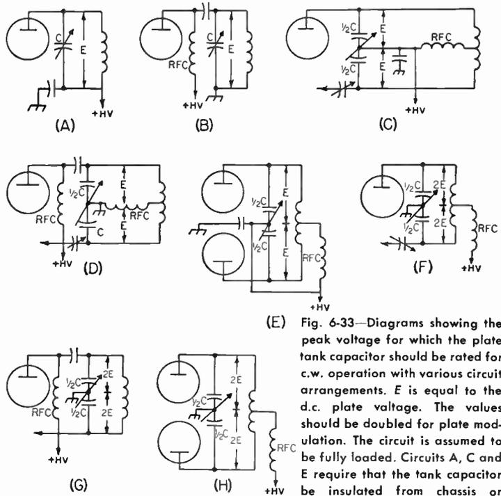
Fig. 6-33—Diagrams showing the peak voltage for which the plate tank capacitor should be rated for c.w. operation with various circuit arrangements. *E* is equal to the d.c. plate voltage. The values should be doubled for plate modulation. The circuit is assumed to be fully loaded. Circuits A, C and E require that the tank capacitor be insulated from chassis or ground, and from the control.
