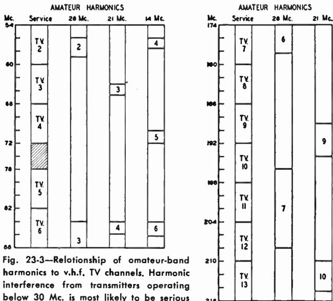
Fig. 23-3—Relationship of amateur-band harmonics to v.h.f. TV channels. Harmonic interference from transmitters operating below 30 Mc. is most likely to be serious in the low-channel group (54 to 88 Mc.).
