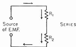
Fig. 2-4—Resistors connected in series and in parallel.
