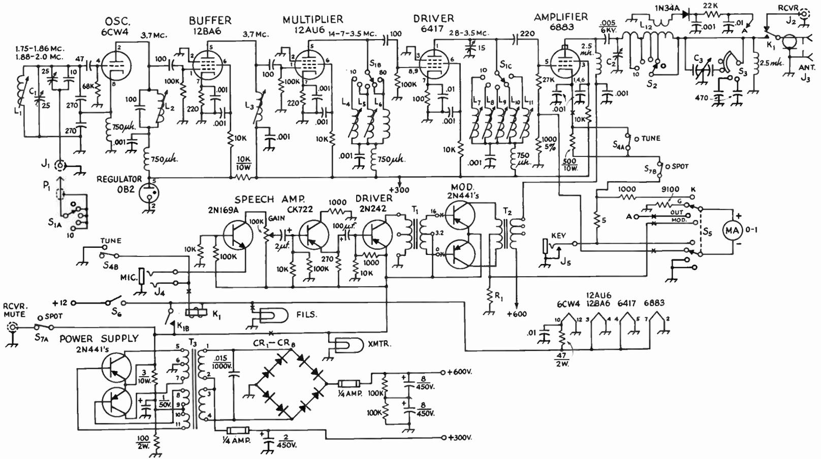
Fig. 19-26—Circuit diagram of the mobile transmitter. Unless specified otherwise, capacitances are in  $\mu\text{f.}$ , decimal values are in  $\mu\text{f.}$ , resistances are in ohms, resistors are  $\frac{1}{2}$  watt.
