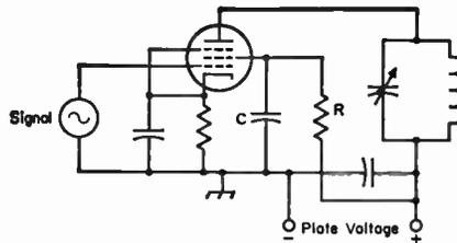
Fig. 3-20—Screen-voltage supply for a pentode tube through a dropping resistor,  $R$ . The screen bypass capacitor,  $C$ , must have low enough reactance to bring the screen to ground potential for the frequency or frequencies being amplified.
