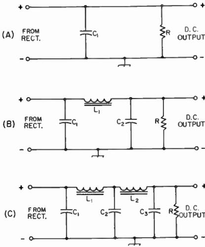
Fig. 7-5—Capacitive-input filter circuits. A—Simple capacitive. B—Single-section. C—Double-section.
