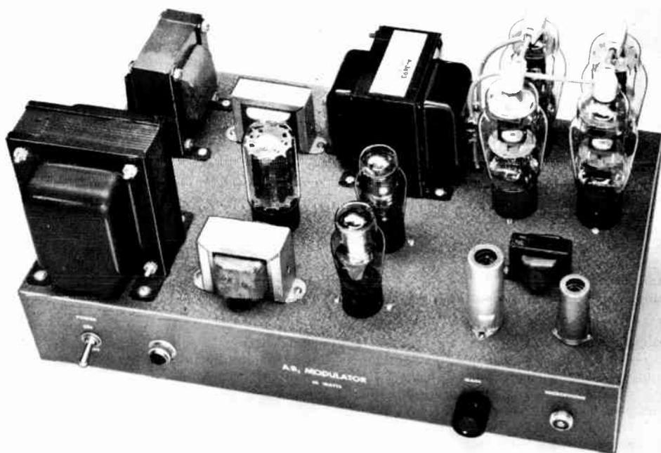
Fig. 9-20—A 50-watt modulator, using four 1625-type tubes in Class AB<sub>1</sub>. With higher plate voltage and a larger modulation transformer, the tubes can deliver up to 140 watts of audio power.
