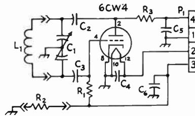
Fig. 21-16—Circuit diagram of the grid-dip meter.  $C_1$ —50  $\mu\text{mf.}$  per section (Johnson 167-11 with stator bars sawed between 6th and 7th plates).
