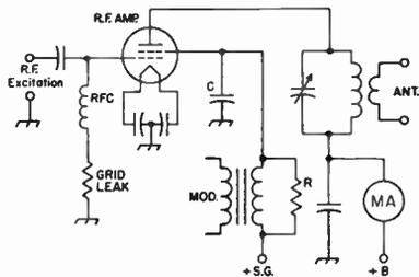
Fig. 10-10—Screen-grid modulation of beam tetrode. Capacitor C is an r.f. bypass capacitor and should have high reactance at audio frequencies. A value of 0.002  $\mu$ f. is satisfactory. The grid leak can have the same value that is used for c.w. operation of the tube.
