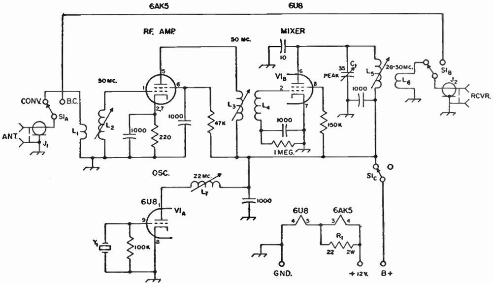
Fig. 19-11—Schematic diagram for the 50-Mc. mobile converter. All resistors 1/2 watt unless otherwise specified. Capacitor values below 0.001  $\mu$ f. are in  $\mu$  $\mu$ f. All 0.001  $\mu$ f. capacitors are disk ceramic.
