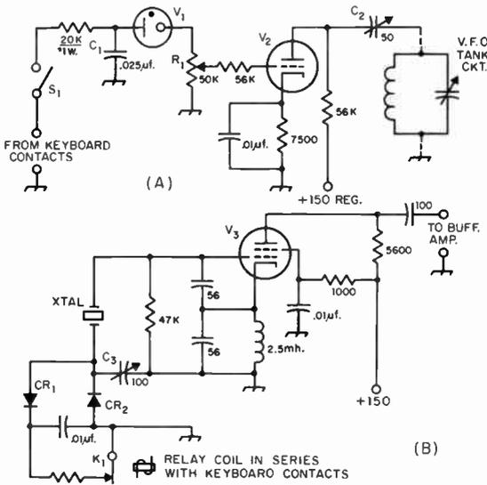
Fig. 12-14—Frequency-shift keyer circuits. Unless otherwise indicated, capacitances are in  $\mu\text{mf.}$ , resistances are in ohms, resistors are  $\frac{1}{2}$  watt. A—Reactance-tube keyer for use with variable-frequency oscillator (W6OWP). B—Crystal oscillator circuit (W2PAT). It is essential that all leads associated with the crystal portion of the circuit be held to a small fraction of an inch in length if maximum shift is desired.
