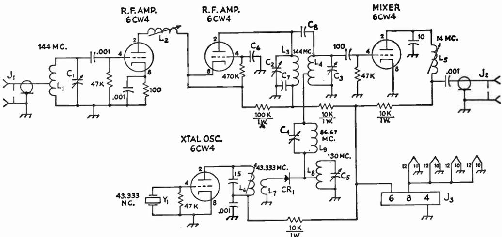
Fig. 16-11—Schematic diagram and parts information for the 144-Mc. converter. Resistors  $\frac{1}{2}$  watt unless specified. Fixed capacitors are ceramic unless specified. Decimal values in  $\mu$ f., others in  $\mu\mu$ f.
