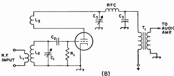
(B) Feeding some signal from the plate circuit back to the grid makes the circuit regenerative. When feedback is sufficient, the circuit will oscillate. Feedback is controlled here by varying reactance at  $C_5$ ; with fixed capacitor at that point regeneration could be controlled by varying plate voltage or coupling between  $L_2$  and  $L_3$ .
