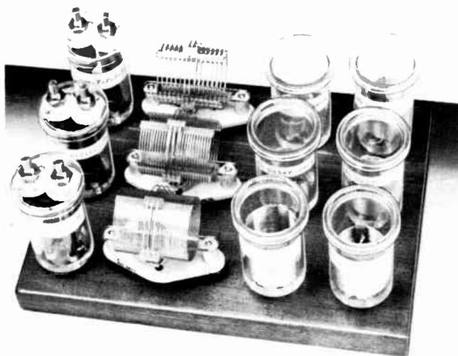
Fig. 11-13—Plug-in coils and r.f. phase-shift networks for the sideband generator. Output tank coils (right) include additional padding capacitor for  $C_7$ , as given in the coil table. Polystyrene coil forms are 4-pin (Allied Radio 24-4P) and 5-pin (Allied Radio 24-5P).
