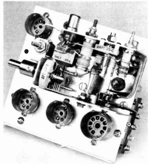
Fig. 19-22—The v.f.o. section is built in the U-shaped portion of a 3¼  $\times$  2½  $\times$  1½-inch Minibox (Bud CU-2101-A) mounted on a sheet of aluminum; the other half of the Minibox serves as the cover. The Nuvistor socket and the oscillator coils are mounted on one side of the Minibox and the oscillator coils are mounted on the other side of the Minibox and is visible between the two right-hand tube sockets.
