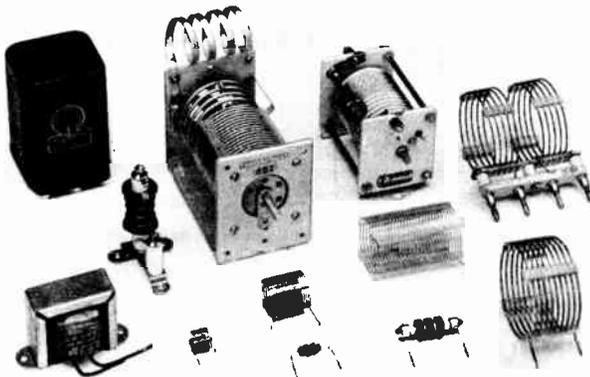
Inductors for power and radio frequencies. The two iron-core coils at the left are "chokes" for power-supply filters. The mounted air-core coils at the top center are adjustable inductors for transmitting tank circuits. The "pie-wound" coils at the left and in the foreground are radio-frequency choke coils. The remaining coils are typical of inductors used in r.f. tuned circuits, the larger sizes being used principally for transmitters.
