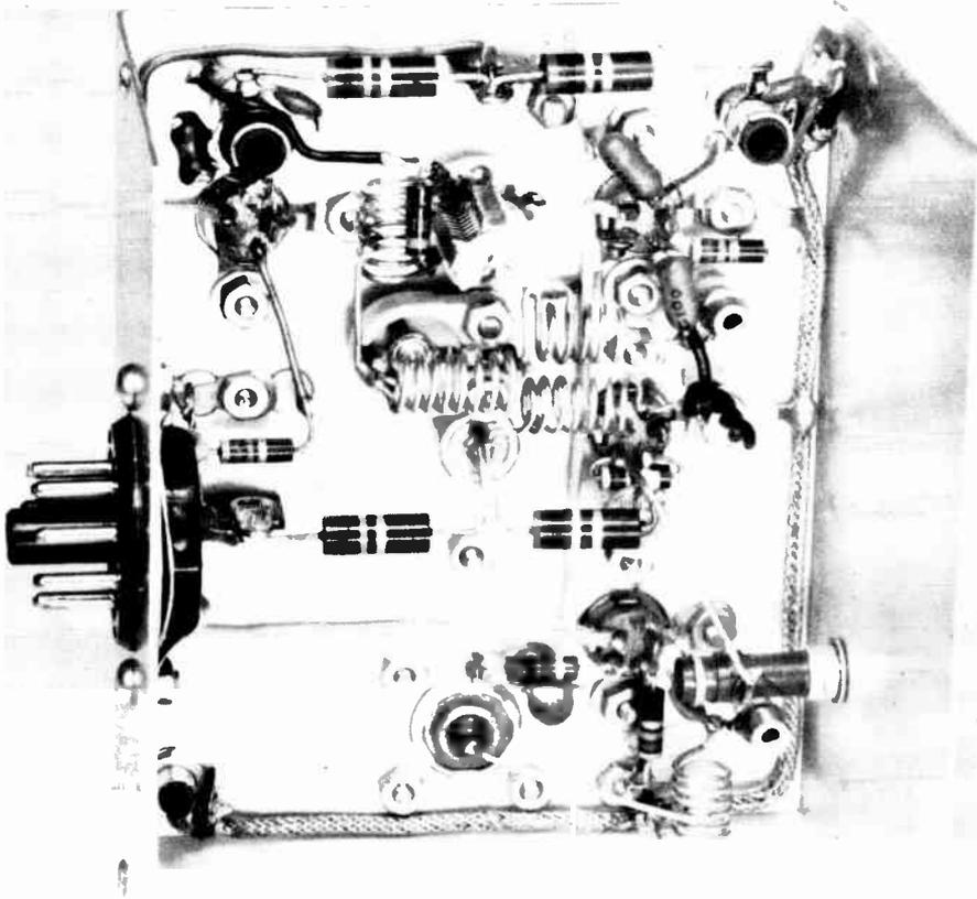
Fig. 16-12—Interior of the 144-Mc. converter. Details of parts arrangement are given in the text. The i.f. output from the mixer plate coil,  $L_5$ , (upper right) is brought through a shielded lead down the side and across the bottom to the output connector,  $J_2$ , at the lower left.
