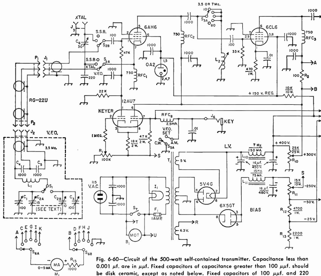
Fig. 6-60—Circuit of the 500-watt self-contained transmitter. Capacitance less than 0.001  $\mu\text{f.}$  are in  $\mu\text{m.}$  Fixed capacitors of capacitance greater than 100  $\mu\text{f.}$  should be disk ceramic, except as noted below. Fixed capacitors of 100  $\mu\text{f.}$  and 220  $\mu\text{f.}$  should be mica. Capacitors marked with polarity are electrolytic. Resistors not otherwise marked are  $\frac{1}{2}$  watt. R.f. chokes in  $\mu\text{h.}$  unless otherwise marked.
