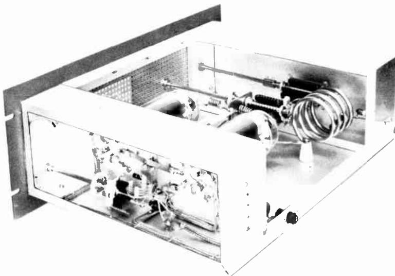
Fig. 6-77—As in the other amplifiers, the 10-meter final uses shielded wires in the filament, screen, and grid-return circuits. For tuning this amplifier uses a small variable capacitor connected across half of the plate coil, to maintain a favorable  $L/C$  ratio.
