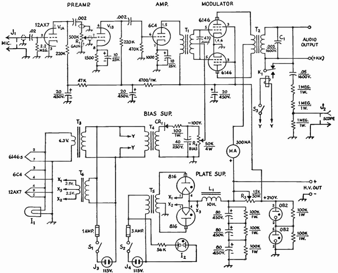
Fig. 9-24—Circuit diagram of the 6146 modulator and power supply. Capacitances are in  $\mu\text{f.}$  unless indicated otherwise; capacitors marked with polarity are electrolytic, others may be paper or ceramic as convenient. Resistances are in ohms; resistors are  $\frac{1}{2}$  watt except as indicated.
