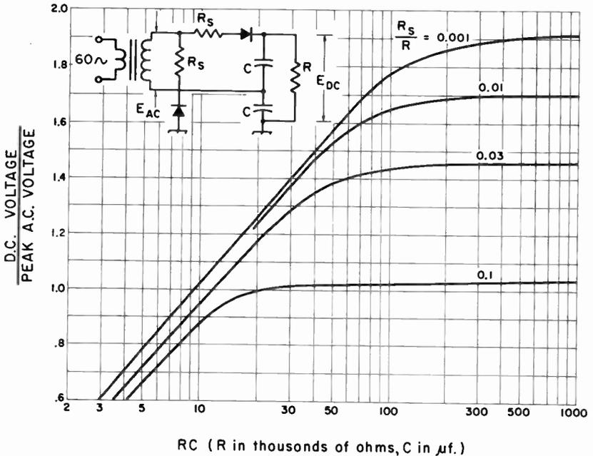
Fig. 7-19—D.c. output voltages from a full-wave voltage-doubling circuit as a function of the filter capacitances and load resistance. For the ratio  $R_s/R$ , both resistances are in ohms; for the RC product,  $R$  is in thousands of ohms.
