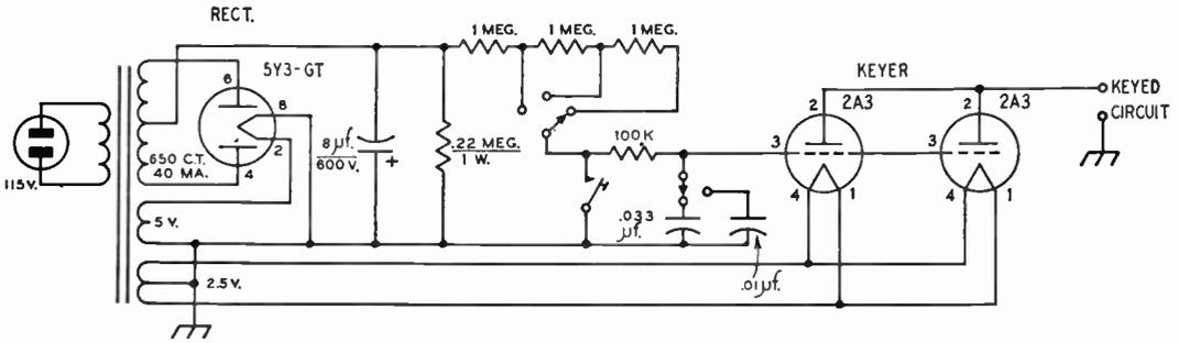
Fig. 8-6—Wiring diagram of a practical vacuum-tube keyer.
