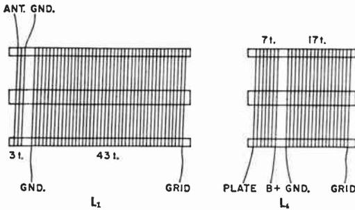
Fig. 5-32—Details of the coil construction. Each one is made from B & W 3012 Miniductor or Illumitronic 632 stock, which is wound 32 t.p.i. and  $\frac{3}{4}$ -inch diameter. The separation between coils in  $L_1$  is  $1\frac{1}{2}$  turns; the separation between coils in  $L_4$  is 1 turn.  $L_3$  is 43 turns of the same stock.
