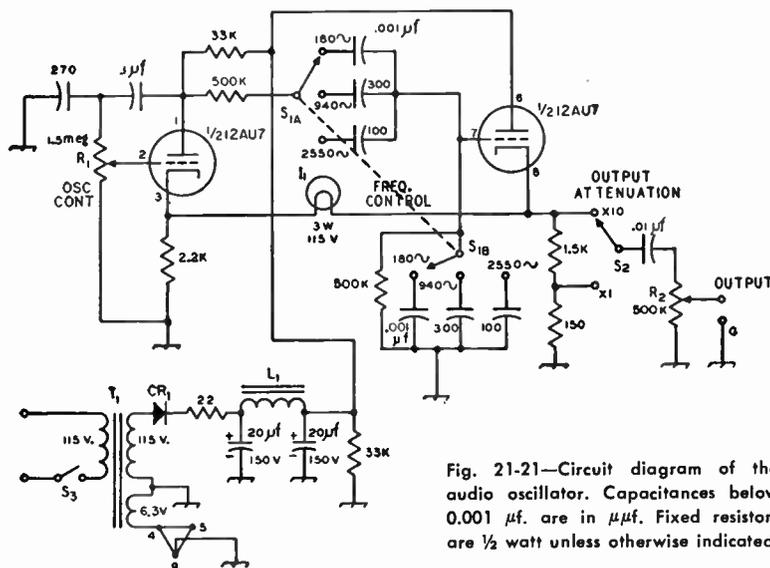
Fig. 21-21—Circuit diagram of the audio oscillator. Capacitances below 0.001 μf. are in μf. Fixed resistors are 1/2 watt unless otherwise indicated.
