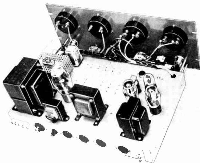
Fig. 6-70—Top view of the control unit. The voltmeter multiplier resistors are housed in a cane-metal protective shield (upper left). Resistors  $R_8$  and  $R_9$  are mounted under the sets of ventilation holes (center near panel).
