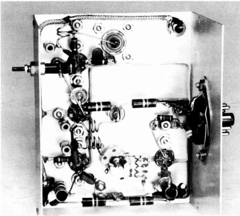
Fig. 16-15—View underneath the chassis of the 220-Mc. converter. The long shielded wire runs from  $L_5$  at the lower left to the output jack. Silver-button mica capacitors (Centralab ZA-102) that bypass the plate coil and the control grid of the second 6CW4 (center left) are also used to support several resistors. Coil  $L_5$  is supported by the terminals of  $C_6$  (bottom center). Chassis is part of  $3 \times 4 \times 5$ -inch Minibox.
