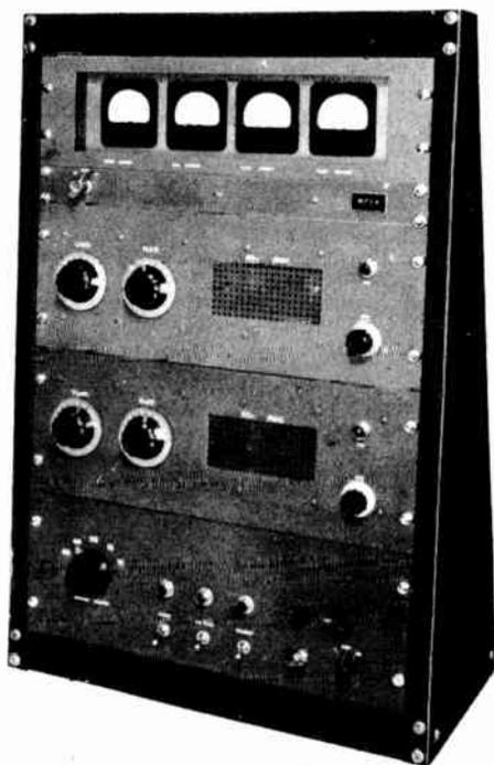
Fig. 6-73—Individual kilowatt amplifiers for two bands plus complete metering and all control circuits and power supplies (except plate) fit handily into a table rack. Amplifiers for five bands plus the plate supply will mount in floor rack. Band switch at lower left ( $S_8$  in Fig. 6-74) switches filament supply, excitation and output connections to all amplifiers in use; screen and plate supplies are connected to all amplifiers at all times.
