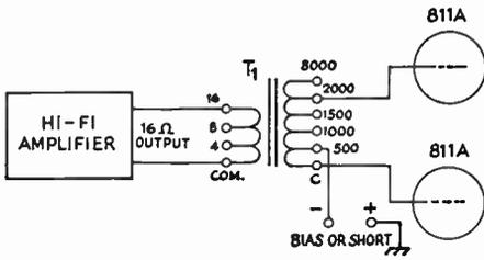
Fig. 9-29—A "hi-fi" audio amplifier will drive a Class-B modulator; a suitable coupling transformer is required. The connections shown here are for a pair of 811As. The amplifier should have an output rating of at least 10 watts.
