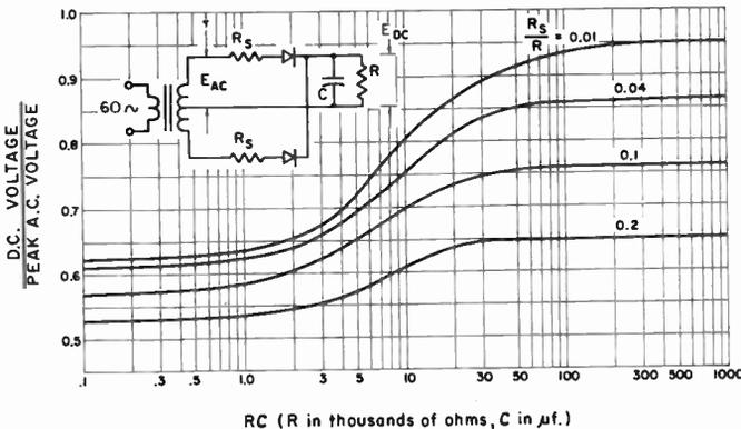
Fig. 7-6—D.c. output voltages from a full-wave rectifier circuit as a function of the filter capacitance and load resistance.  $R_s$  includes transformer winding resistance and rectifier forward resistance. For the ratio  $R_s/R$ , both resistances are in ohms; for the  $RC$  product,  $R$  is in thousands of ohms.
