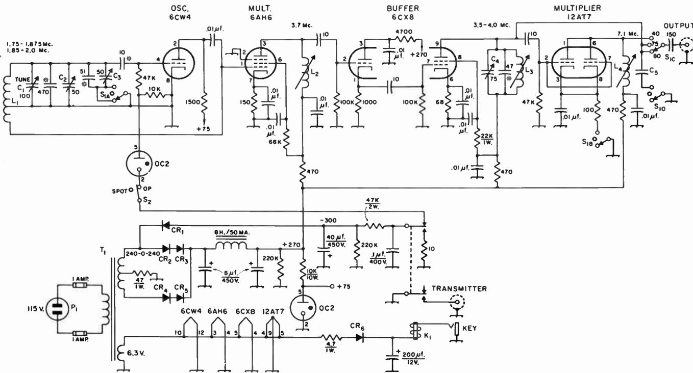
Fig. 6-89—Circuit diagram of the two-band v.f.o. Unless otherwise specified, all capacitances are in picofarads (pf. or  $\mu\text{mf.}$ ), resistances are in ohms, resistors are  $\frac{1}{2}$ -watt. Capacitors marked with polarity are electrolytic, those marked with asterisk are silver mica.
