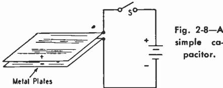
Fig. 2-8—A simple capacitor.
