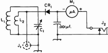
Fig. 21-10—Circuit of typical wavemeter with built-in indicator. The circuit responds to the frequency for which  $L_1C_1$  is resonant; a small amount of energy is coupled to  $L_2$ , rectified by CR1, and indicated by the meter. By plugging in a pair of headphones at  $J_1$ , any modulation on the signal will be heard.
