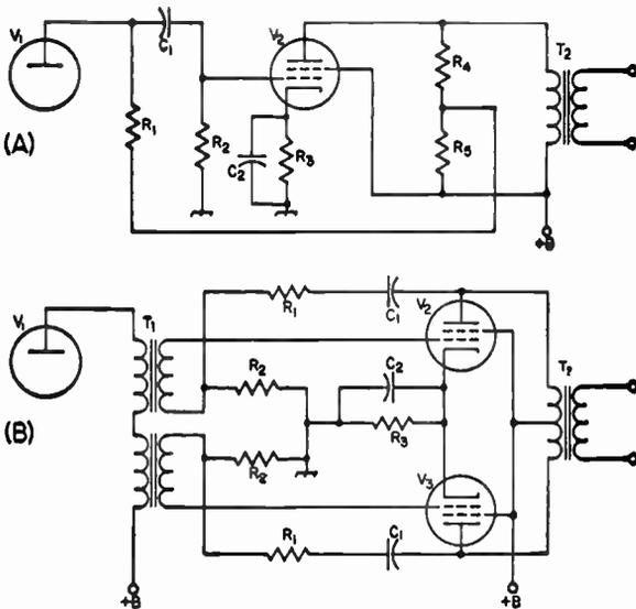
Fig. 9-9—Negative-feedback circuits for drivers for Class B modulators. A—Single-ended beam-tetrode driver. If V<sub>1</sub> and V<sub>2</sub> are a 6J5 and 6V6, respectively, or one section of a 6CG7 and a 6AQ5, the following values are suggested: R<sub>1</sub>, 47,000 ohms; R<sub>2</sub>, 0.47 megohm; R<sub>3</sub>, 250 ohms; R<sub>4</sub>, R<sub>5</sub>, 22,000 ohms; C<sub>1</sub>, 0.01  $\mu\text{f.}$ ; C<sub>2</sub>, 50  $\mu\text{f.}$
