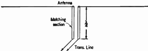
Fig. 14-41—"Q" matching section, a quarter-wave impedance transformer.
