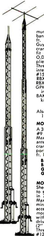
imum height 25 ft. Supports triband beams or equivalent at 60 ft. in winds up to 60 mph. No Guys! 140 mph winds when cranked down. CDR-Ham-M rotors fit in special head mount. 1.90 O.D. x 7 ft. galv. steel mast supplied.
