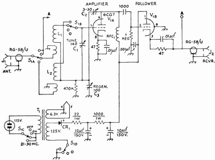
Fig. 5-50—Circuit diagram of the regenerative preselector. Unless otherwise specified, resistors are  $\frac{1}{2}$  watt, capacitors are in  $\mu\text{mf.}$ , capacitors marked in polarity are electrolytic.
