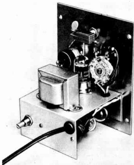
Fig. 21-22—Inside view of the audio oscillator. The a.c. switch,  $S_3$ , is mounted on the OUTPUT control at the left on the panel. The ceramic capacitors in the frequency-determining circuits are mounted on the rotary switch,  $S_1$ , at the right.  $S_2$  is above the tube, and  $T_1$  is on the near edge of the chassis, which is a U-shaped piece of aluminum  $3\frac{1}{2}$  inches deep with  $1\frac{1}{2}$ -inch lips.  $R_1$  is mounted on the near lip at the left.
