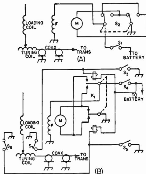
Fig. 19-37—Circuit of the remote mobile-whip tuning systems.
