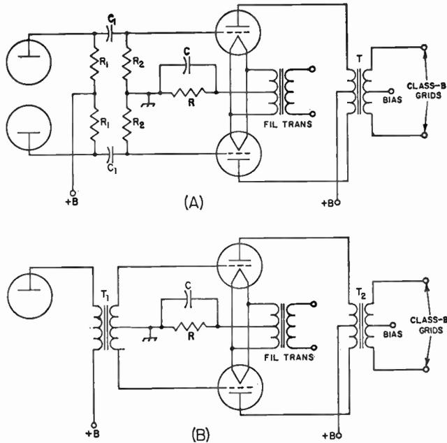
Fig. 9-7—Triode driver circuits for Class B modulators. A, resistance coupling to grids; B, transformer coupling. R<sub>1</sub> in A is the plate resistor for the preceding stage, value determined by the type of tube and operating conditions as given in Table 9-1. C and R<sub>2</sub> are the coupling capacitor and grid resistor, respectively; values also may be taken from Table 9-1.
