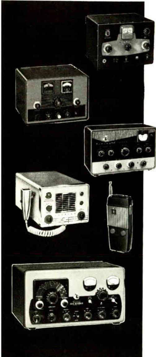
**ADVENTURER**—Self-contained . . . 50 watts CW input . . . rugged 807 transmitting tube . . . instant bandswitching 80 through 10 meters. Crystal or external VFO control—wide range pi-network output—timed sequence keying. With tubes, less crystals.
