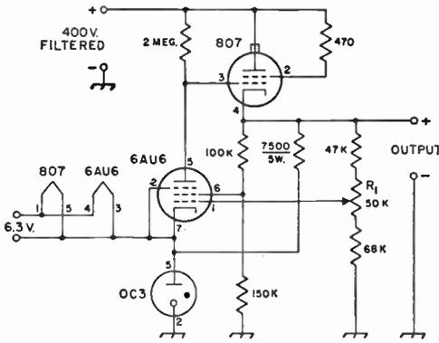
Fig. 7-22—Electronic voltage-regulator circuit. Resistors are 1/2 watt unless specified otherwise.
