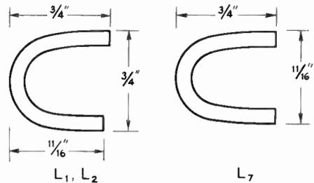
Fig. 16-26—Details of "coils"  $L_1$ ,  $L_2$  and  $L_7$ . Material is No. 10 tinned copper wire. Taps on  $L_1$  and  $L_2$  are  $\frac{1}{2}$  up from ground end; taps on  $L_7$  are  $\frac{1}{3}$  and  $\frac{1}{2}$  up from ground end.
