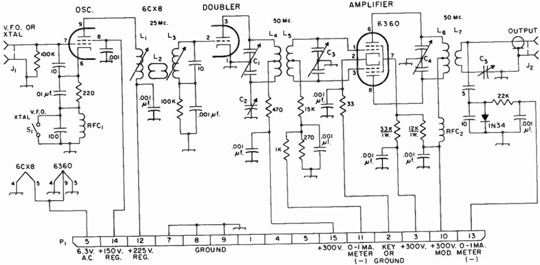
Fig. 17-4—Circuit diagram of the 50-Mc. transmitter. Unless specified otherwise, capacitances are in picofarads (pf. or  $\mu\text{f.}$ ), resistances, are in ohms, resistors are  $\frac{1}{2}$  watt. Fixed capacitors are ceramic.
