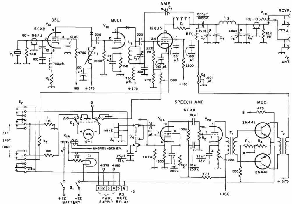
Fig. 19-16—Circuit diagram of the 40-watt "extended-band" mobile transmitter. Unless noted otherwise, resistances are in ohms, resistors are  $\frac{1}{2}$  watt, capacitances are in picofarads.
