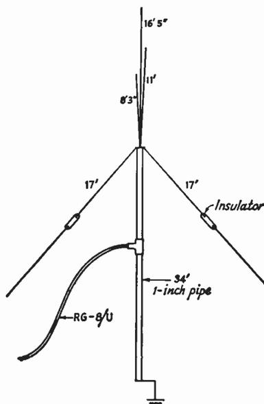
Fig. 14-27—The 14-, 21- and 28-Mc. ground-plane antenna uses wire elements. Vertical elements are taped to a cane pole; the four radials also serve as guy wires. The radials "droop" a little, making a 40-degree angle with the supporting 1-inch pipe.
