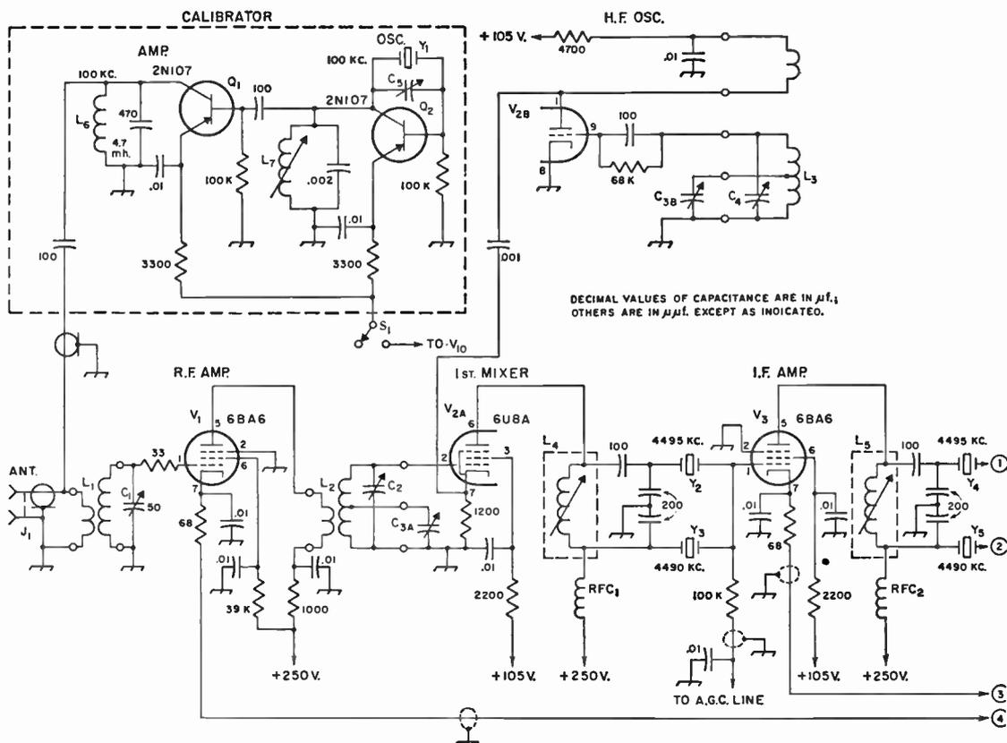
Fig. 5-52—Front-end circuit of the receiver. Unless otherwise specified, resistors are  $\frac{1}{2}$  watt; 0.01 and 0.02- $\mu$ f. capacitors are disk ceramic, 600 volts; 0.5 capacitors are tubular paper or Mylar; capacitors below 0.01  $\mu$ f. are mica; capacitors marked with polarities are electrolytic.
