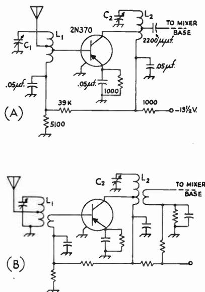
Fig. 5-27—Transistor r.f. amplifier circuit. The low-impedance connections to the base and collector can be (A) taps on the inductors or (B) low-impedance coupling links.  $L_1C_1$ ,  $L_2C_2$ —Resonant at signal frequency.
