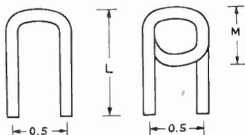
Fig. 21-19—Details of the coils used in the u.h.f. grid-dip meter. The material is No. 10 tinned-copper wire.
