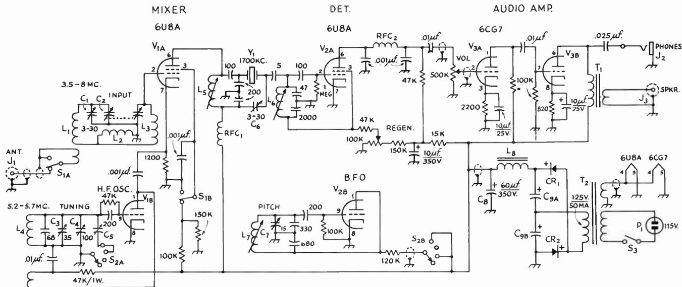
Fig. 5-31—Circuit diagram of the SimpleX Super receiver. Unless otherwise indicated, capacitances are in  $\mu\text{mf.}$ , resistances are in ohms, resistors are  $\frac{1}{2}$  watt. Polarity is shown on electrolytic capacitors, 680  $\mu\text{mf.}$  or less are silver mica or NPO ceramic, 2000- $\mu\text{mf.}$  fixed capacitor is mica. Capacitors specified in decimal- $\mu\text{f.}$  values are ceramic.
