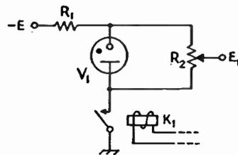
Fig. 11-26—Bias-switching circuit for use with a Class-AB<sub>1</sub> linear amplifier and an electronic t.r. switch.
