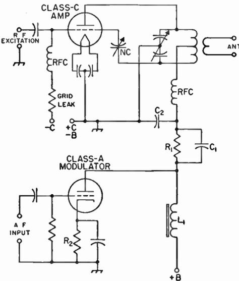
Fig. 10-8—Choke-coupled Class A modulator. The cathode resistor,  $R_2$ , should have the normal value for operation of the modulator tube as a Class A power amplifier. The modulation choke,  $L_1$ , should be 5 henrys or more. A value of 0.001 to 0.005  $\mu$ f. is satisfactory for  $C_2$ , the r.f. amplifier plate bypass capacitor. See text for discussion of  $C_1$  and  $R_1$ .
