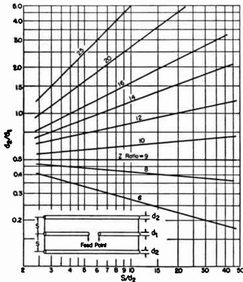
Fig. 14-44—Impedance transformation ratio, three-conductor folded dipole. The dimensions  $d_1$ ,  $d_2$  and  $s$  are shown on the inset drawing. Curves show the ratio of the impedance (resistive) seen by the transmission line to the radiation resistance of the resonant antenna system.
