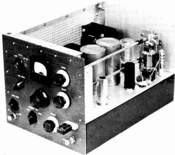
The photograph shows the front panel of the exciter unit. It features a large knob under a meter, a small knob at the lower left, and a switch to the left of the meter. The interior of the unit is visible, showing a 6DQ5 output tube, a 9-Mc. crystal filter, and other components. The top plate is partially removed, revealing the internal wiring and components.
