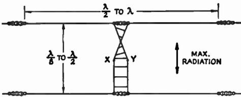
Fig. 14-31—Top view of a horizontal end-fire array. The system is fed with an open-wire line at  $x$  and  $y$ ; the line can be of any length. Feed points  $x$  and  $y$  are equidistant from the two insulators, and the feed line should drop down vertically from the antenna. The gain of the system will vary with the spacing, as shown in Fig. 14-32, and is a maximum at  $\frac{1}{2}$  wavelength. By using a length of 33 feet and a spacing of 8 feet, the antenna will work on 20, 15 and 10 meters.
