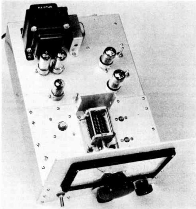
Fig. 6-87—The two-band v.f.o. uses a 6CW4 Nuovistor triode (left front) in the oscillator circuit. In this view the tube shields have been removed from the r.f. tubes (tubes in front of transformer are voltage regulators), and the Minibox cover has been lifted to show the tuning capacitor. The front half of the chassis is reinforced with a plate of  $\frac{1}{8}$ -inch thick aluminum, to eliminate microphonics.
