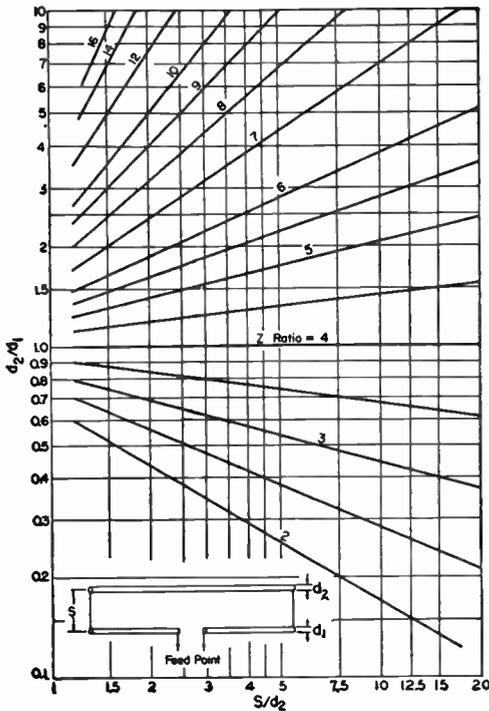
Fig. 14-43—Impedance transformation ratio, two-conductor folded dipole. The dimensions  $d_1$ ,  $d_2$  and  $s$  are shown on the inset drawing. Curves show the ratio of the impedance (resistive) seen by the transmission line to the radiation resistance of the resonant antenna system.
