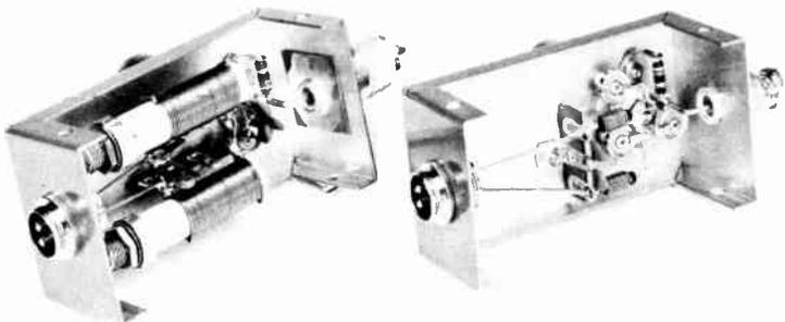
Fig. 21-26—Each diode noise generator is housed in a  $4 \times 2\frac{1}{2} \times 1\frac{1}{2}$ -inch "Minibox" (Bud CU-2102-A). Power connections are made through double-pin male receptacles (Amphenol 80 PC2M), and the r.f. connection is made to the receiver or converter by a suitable plug. The plug on the 7- to 90-Mc. generator (left) is a PL-259 held to the face of the "Minibox" by a small copper plate and a UG-176/U reducing adapter.
