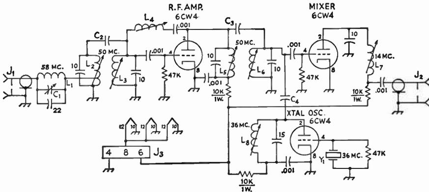
Fig. 16-9—Schematic diagram and parts information for the 50-Mc. converter. Resistors ½ watt unless specified. Fixed capacitors are ceramic; decimal values in  $\mu\text{f.}$ , others in  $\mu\mu\text{f.}$
