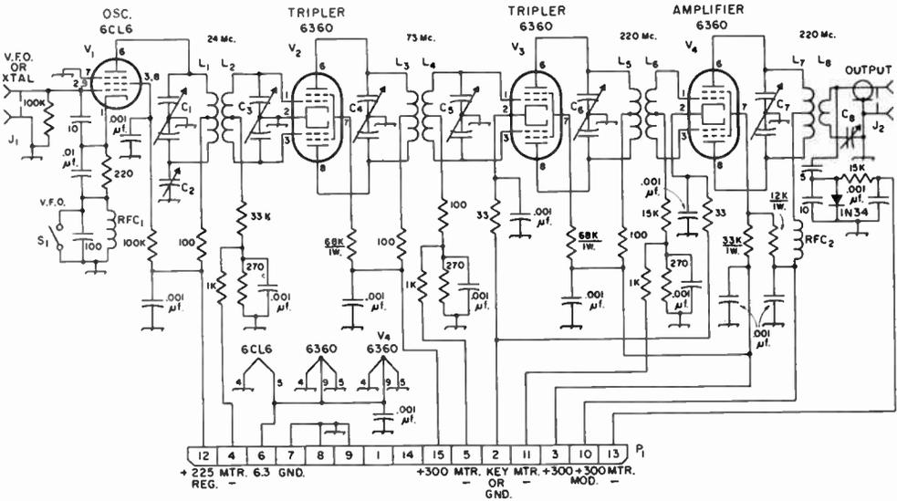
Fig. 17-10—Circuit diagram of the 220-Mc. transmitter. Unless specified otherwise, capacitances are in picofarads (pf. or  $\mu\text{mf.}$ ), resistances are in ohms, resistors are  $\frac{1}{2}$  watt.
