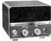
**HA-1 "T.O." KEYER.** Meets all requirements of the CW perfectionist. Employs digital techniques to produce constant ratio of dot-to-space-to-dash throughout entire speed range. Transformer operated. Speeds from 20-45 WPM. Monitor or sidetone may be heard through built-in speaker.
