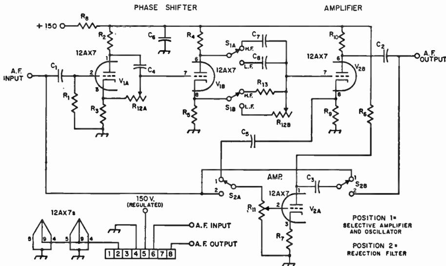
Fig. 5-45—Complete schematic of Selectoject using 12AX7 tubes.
