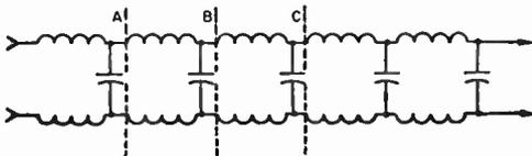
Fig. 13-1—Equivalent of a transmission line in lumped circuit constants.
