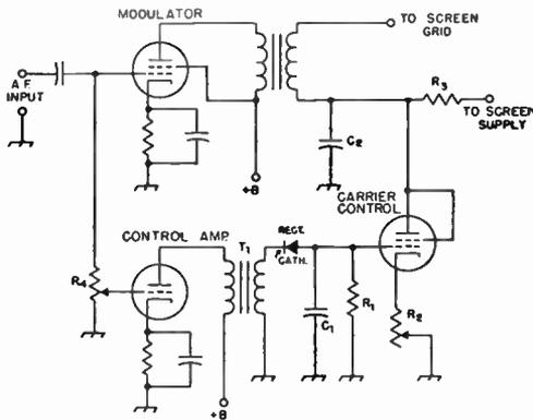
Fig. 10-12—Circuit for carrier control with screen modulation. A small triode such as the 6C4 can be used as the control amplifier and a 6Y6G is suitable as a carrier-control tube.  $T_1$  is an interstage audio transformer having a 1-to-1 or larger turns ratio.  $R_4$  is a 0.5-megohm volume control and also serves as the grid resistor for the modulator. A germanium crystal may be used as the rectifier. Other values are discussed in the text.
