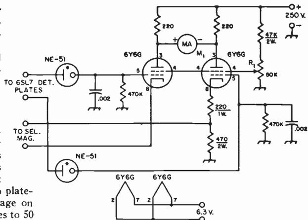
The zero-center meter,  $M_1$ , is not a necessity but is a convenience in making adjustments.  $R_1$  should be adjusted on receiver noise for zero reading. With a 2125-cycle tone the pointer will swing to the left and  $L_1$  should be adjusted for maximum deflection. With a 2975-cycle tone the pointer will swing to the right and  $L_2$  should be adjusted for maximum deflection. Equal deflections should be obtained from both channels.
