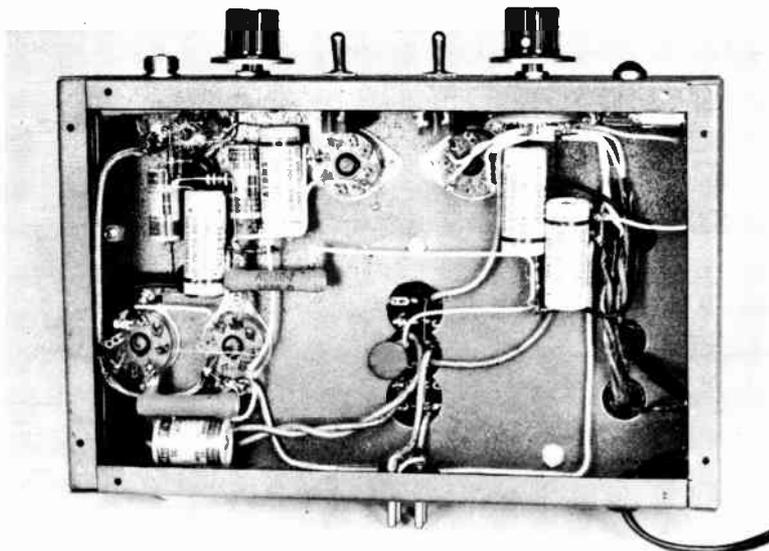
Fig. 9-19—Under-chassis view of the 6BQ6GT modulator. The two large capacitors at the right are the filter capacitors in the power supply. The modulator bias resistor and bypass capacitor (R<sub>1</sub>C<sub>3</sub>) are at lower left. Leads from the modulation transformer go through the three holes in the chassis. Shielded wire is used for heater, microphone input, and gain-control leads.
