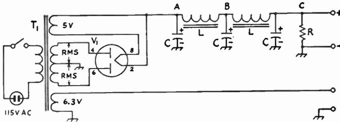
Fig. 7-14—Typical a.c. power-supply circuit for receivers, exciters, or low-power transmitters. Representative values will be found in Table 7-II. The 5-volt winding of  $T_1$  should have a current rating of at least 2 amp. for types 5Y3-GT and 5V4-GA, and 3 amp. for 5U4-GB.
