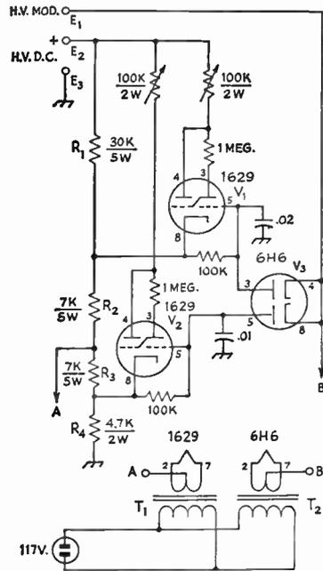
Fig. 10-24—Circuit diagram of the modulation monitor. Unless specified otherwise, resistors are  $\frac{1}{2}$  watt, resistances are in ohms, capacitances are in  $\mu\text{f}$ .
