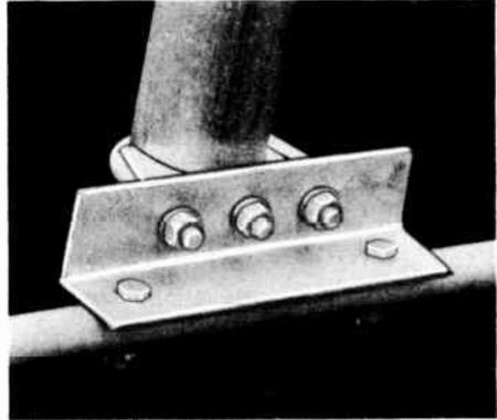
Fig. 14-54—Muller clamps can be used to hold beam elements to the boom. The angle can be aluminum angle or angle iron; if iron is used it should be cadmium plated. This example shows a ¼-inch-diameter element held to a 2-inch diameter boom.
