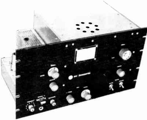
Fig. 17-16—The 50-Mc. r.f. unit. Exciter, left portion on the assembly, also serves on 144 Mc. Amplifier utilizes a 4-125A, 4-250A or 4-400A.
