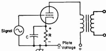
Fig. 3-19—Cathode biasing.  $R$  is the cathode resistor and  $C$  is the cathode bypass capacitor.
