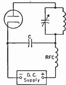
capacitor should not be more than one-tenth of the impedance of the bypassed part of the circuit. Very often the latter impedance is not known, in which case it is desirable to use the largest capacitance in the bypass that circumstances permit. To make doubly sure that r.f. current will not flow through a non-r.f. circuit such as a power supply, an r.f. choke may be connected in the lead to the latter, as shown in Fig. 2-58.
