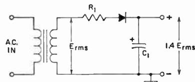
Fig. 7-17—If the current demand is low, a simple half-wave rectifier will deliver a voltage increase. Typical values, for  $E_{rms} = 117$  and a load current of 1 ma.:  $C_1 - 50\text{-}\mu\text{f.}$ , 250-v. electrolytic.
