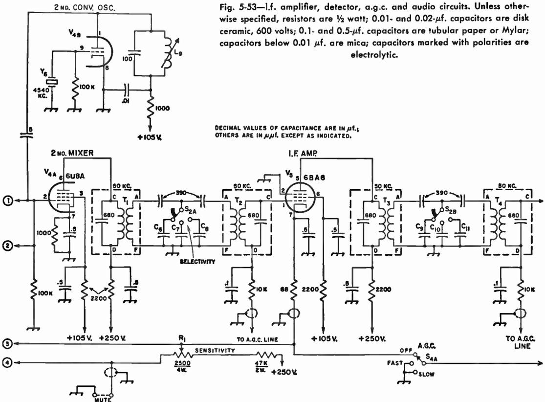
Fig. 5-53—i.f. amplifier, detector, a.g.c. and audio circuits. Unless otherwise specified, resistors are  $\frac{1}{2}$  watt; 0.01- and 0.02- $\mu\text{f.}$  capacitors are disk ceramic, 600 volts; 0.1- and 0.5- $\mu\text{f.}$  capacitors are tubular paper or Mylar; capacitors below 0.01  $\mu\text{f.}$  are mica; capacitors marked with polarities are electrolytic.
