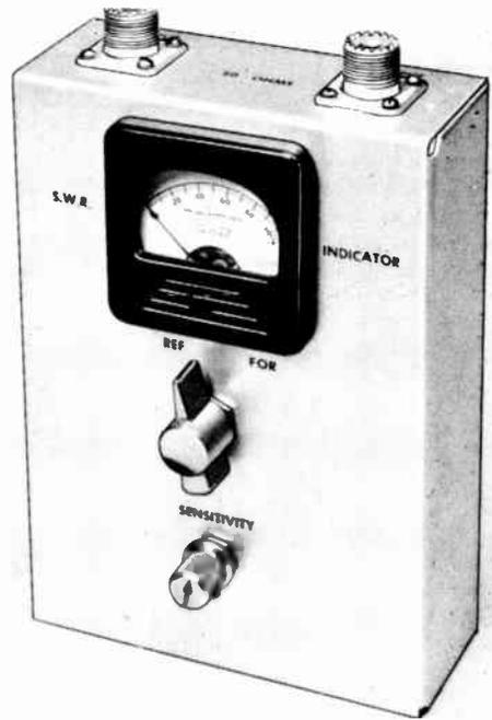
Fig. 13-21—The Monimatch, an s.w.r. monitor that can be left in the line at all times. The unit shown here will handle a kilowatt.
