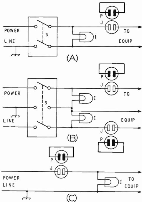
Fig. 7-35—Reliable arrangements for cutting off all power to the transmitter. *S* is an enclosed double-pole knife-type switch, *J* a standard a.c. outlet, *P* a shorted plug to fit the outlet and *I* a red lamp.
