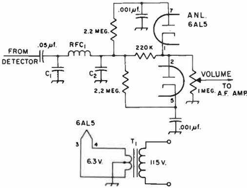
Fig. 5-19—Full-wave shunt limiter using contact-potential-biased diodes. A low-level limiter ( $\frac{1}{2}$  volt), this circuit finds greatest usefulness following a product detector.
