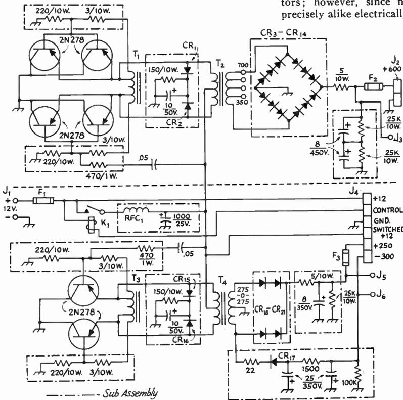
Fig. 19-48—Circuit diagram of the triple transistorized power supply. Capacitances are in  $\mu\text{f}$ ., resistors are  $\frac{1}{2}$  watt unless specified otherwise. Capacitors marked with polarity are electrolytic; others are paper.
