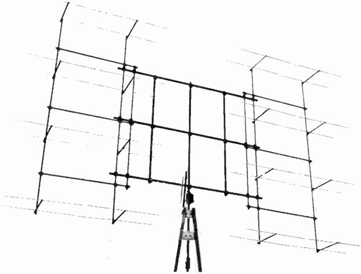
Fig. 18-18—Two 16-element arrays spaced  $\frac{1}{2}$  wavelength and fed in phase.
