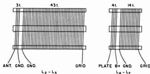
Fig. 5-38—Details of the coil construction. Each one is made from B & W 3012 Miniductor or Illumitronic 632 stock, which is wound 32 t.p.i. and  $\frac{3}{4}$ -inch diameter. The separation between  $L_2$  and  $L_3$  is 1 turn; the separation between  $L_6$  and  $L_7$  is 1 turn.  $L_6$  is 43 turns of the same stock.
