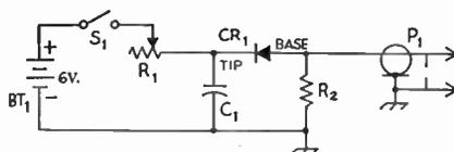
Fig. 21-23—Circuit of a simple crystal-diode noise generator.
