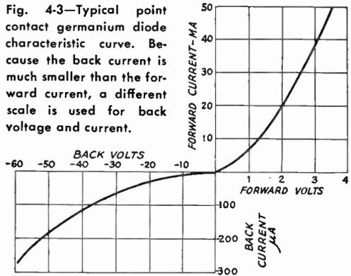
Fig. 4-3—Typical point contact germanium diode characteristic curve. Because the back current is much smaller than the forward current, a different scale is used for back voltage and current.
