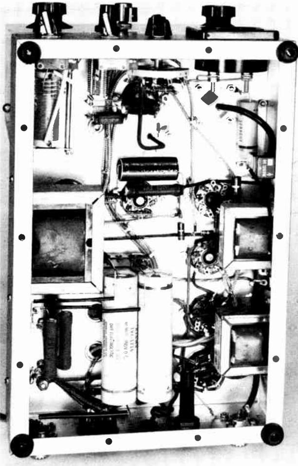
Fig. 6-50—Bottom view of the all-purpose amplifier. The 150-ma. filter choke is mounted on the left-hand wall; the smaller filter choke, the small filament transformer ( $T_1$  in Fig. 6-49) and the selenium rectifier are mounted on the right-hand wall. The strap of aluminum, visible below the meter at the top right, provides additional support for the length of RG-58/U cable that runs to the output coaxial connector. All power leads except the high voltage to the plate are run in shielded wire.
