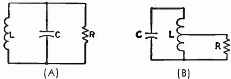
Fig. 2-43—The equivalent circuit of a resonant circuit delivering power to a load. The resistor  $R$  represents the load resistance. At B the load is tapped across part of  $L$ , which by transformer action is equivalent to using a higher load resistance across the whole circuit.
