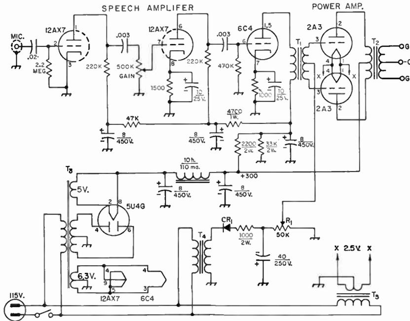
Fig. 9-8—Typical speech-amplifier driver for 10-15 watts output. Capacitances are in  $\mu$ f. Resistors are  $\frac{1}{2}$  watt unless specified otherwise. Capacitors with polarity indicated are electrolytic.
