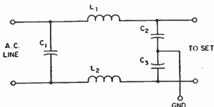
Fig. 23-1—"Brute-force" a.c. line filter for receivers. The values of  $C_1$ ,  $C_2$  and  $C_3$  are not generally critical; capacitances from 0.001 to 0.01  $\mu\text{f.}$  can be used.  $L_1$  and  $L_2$  can be a 2-inch winding of No. 18 enameled wire on a half-inch diameter form. In making up such a unit for use external to the receiver, make sure that there are no exposed conductors to offer a shock hazard.
