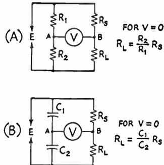
Fig. 21-40—Basic bridge circuits. (A) Resistance bridge; (B) resistance-capacitance bridge. The latter circuit is used in the "Micromatch," with  $R_3$  a very low resistance (1 ohm or less) and the ratio  $C_1/C_2$  adjusted accordingly for a desired line impedance.
