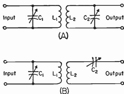
Fig. 2-48—Inductively-coupled resonant circuits. Circuit A is used for high-resistance loads (load resistance much higher than the reactance of either  $L_2$  or  $C_2$  at the resonant frequency). Circuit B is suitable for low resistance loads (load resistance much lower than the reactance of either  $L_2$  or  $C_2$  at the resonant frequency).
