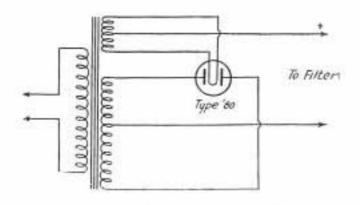
CONNECTIONS USED WITH A TYPE '80 TUBE
