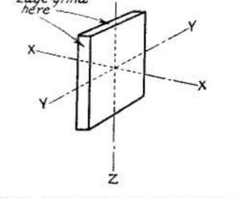
RELATION OF THE AXES OF AN X-CUT QUARTZ PLATE
