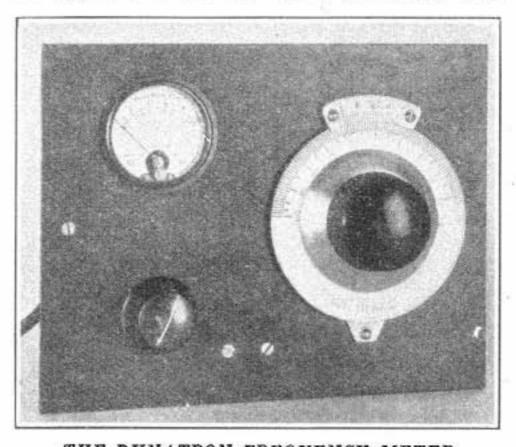
THE DYNATRON FREQUENCY METER The 0-10 milliammeter for reading space current is in the upper left-hand corner, the potentiometer being immediately below it. The vernier dial is used for precise reading.
