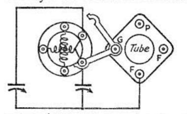
Wiring of coil which connects both sections of condenser in parallel for the 3,500 k.c.
