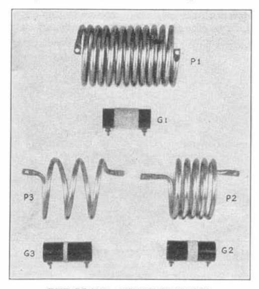
THE PLATE AND GRID COILS
