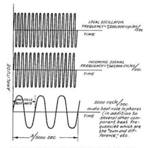
RECEPTION OF CONTINUOUS WAVE TELEGRAPH SIGNALS (By self-heterodyne or outodyne oscillator)
