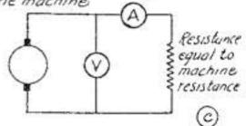
LOAD FOR MOST OUTPUT Half the generated voltage at mochine terminals, heavy
