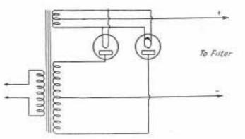
FULL-WAVE RECTIFICATION WITH THERMI-ONIC OR MERCURY-VAPOR TUBES
