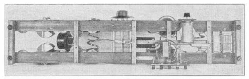
D.C. AND LOW-FREQUENCY A.C. WIRING IS RUN BENEATH THE FRAME The terminal strip, by-pass condenser for key, grid-leak and r.f. chokes are grouped beneath the tubes in the neutral area of the radio-frequency field.
