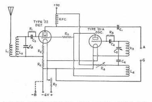
THESE CONNECTIONS ARE USED WITH D.C. TUBES
