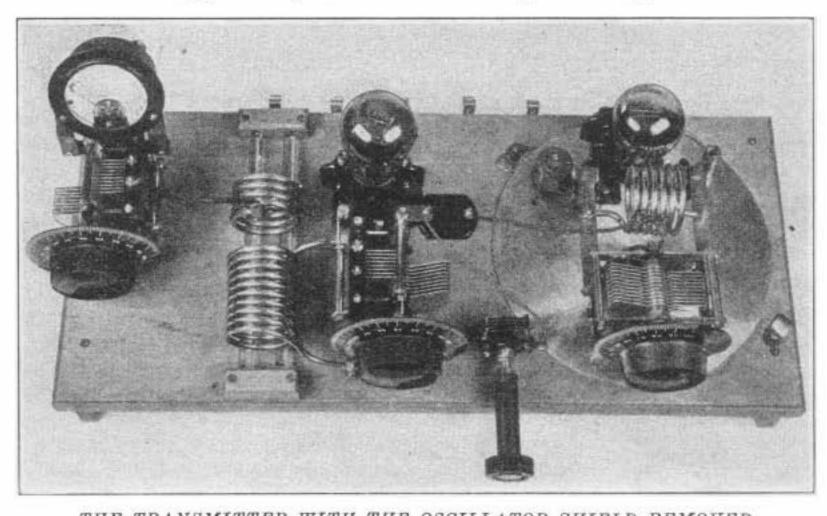
THE TRANSMITTER WITH THE OSCILLATOR SHIELD REMOVED The amplifier receives excitation through the lead tapped on the oscillator inductance. A connection is made by a clip at the center of the amplifier tank inductance. The neutralizing condenser is connected between the grid of the amplifier tube and the front terminal of the tank inductance.
