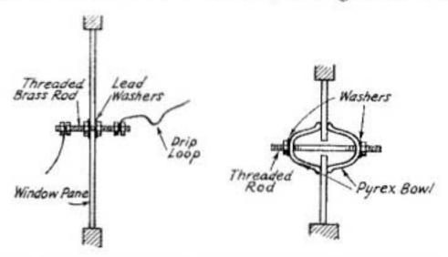
TWO GOOD METHODS OF BRINGING THE TRANS-MITTING ANTENNA LEAD-IN THROUGH A
