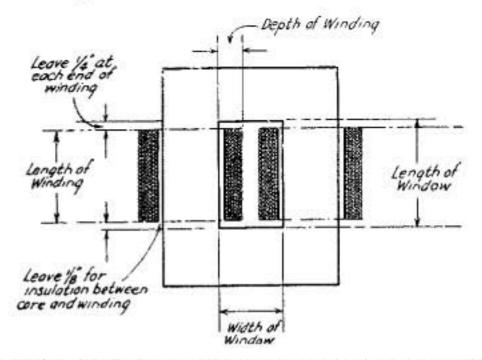
A FULL SIZE DRAWING OF THE TRANSFORMER should be made showing the space to be occupied by the wind-
