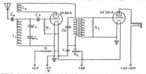
THE SIMPLE WIRING OF THE TWO-TUBE SET
