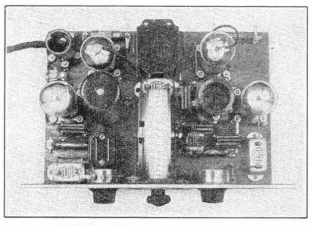
The coils for this receiver are wound on special coil forms which can be obtained at most radio stores. Tube bases could be used for the coil forms, or other types of coils could be substituted.
