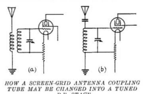
R.F. STAGE A tuned circuit (covering the same band of frequencies as the detector circuit) is substituted for the resistor or choke ordinarily employed in the antenna circuit. The antenna may be
