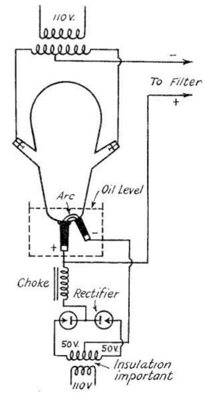
The transformer supplying the "keep-alive" circuit must be well insulated because, just as in the case of the filament-heating transformer for tube rectifiers, the filament circuit of the rectifier CIRCUIT FOR MERCURY-ARC RECTIFIER Connections for the keep-alive circuit are also shown.
