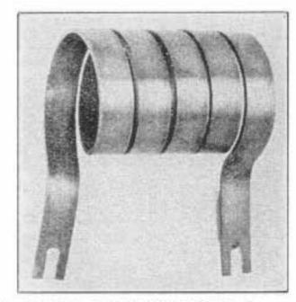
PLATE TANK INDUCTANCES for a high-power transmitter can be made in this fashion. The copper strip is  $\frac{1}{8}''$ thick and  $\frac{3}{4}''$  wide.
