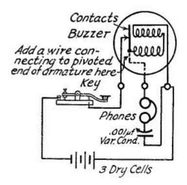
help by sending to you. A buzzer, a telegraph key and a dry cell connected as shown in the diagram make a buzzer practice set. Using a head-set will give more nearly the conditions that obtain in actual radio receiving. It will keep out outside noises. A variable condenser of about .001  $\mu$ fd. max. shunted by another small fixed capacity
