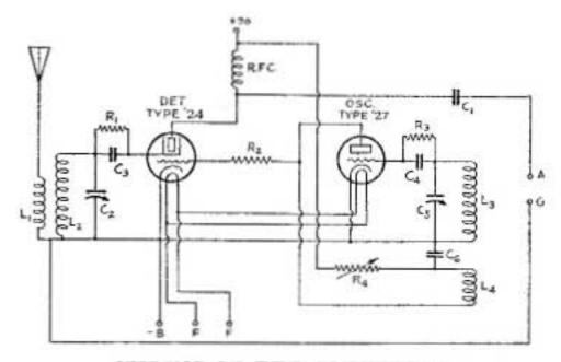
WIRING OF THE CONVERTER
