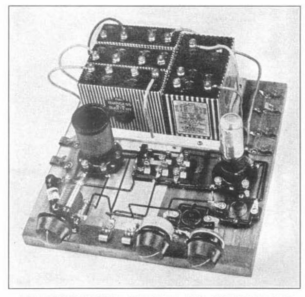
AN EXPERIMENTAL MODEL OF THE MODULOMETER The non-inductive resistor is to the left of the variable condenser. The d.p.d.t. switch in the center is for changing from "audio input" to r.f. input for the measurement of percentage of modulation.
