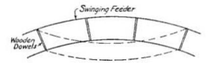
THE USE OF LIGHT WOODEN DOWELS IN THE FEEDER
