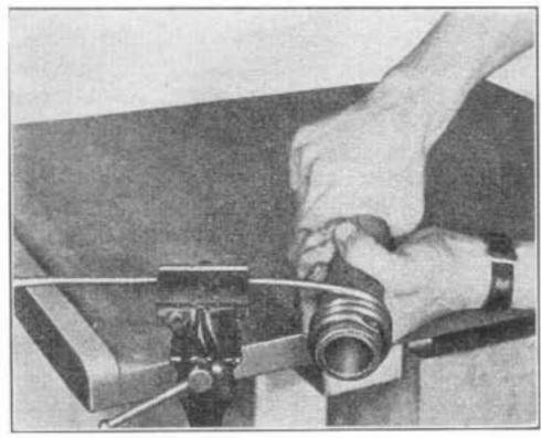
WINDING A COPPER-TUBING INDUCTANCE
