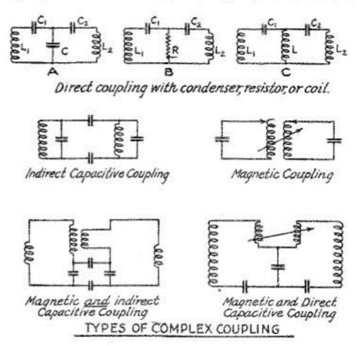
$L_2 C_2$  circuit. The  $L_1 C_1$  current and the value of C, R, or L determine what takes place in the  $C_2 L_2$  circuits.
