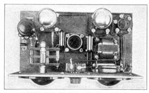
— so that the effective capacity range of the tuning condenser is progressively lower for the higher frequency bands. An understanding of the reason why a lower setting of the series midget condenser reduces the capacity range of the tuning condenser can be obtained by studying the explanation of the action of condensers in series in Chapter III. The methods of band spreading used in the other receivers described in the chapter could be incorporated in this two-tube set.
