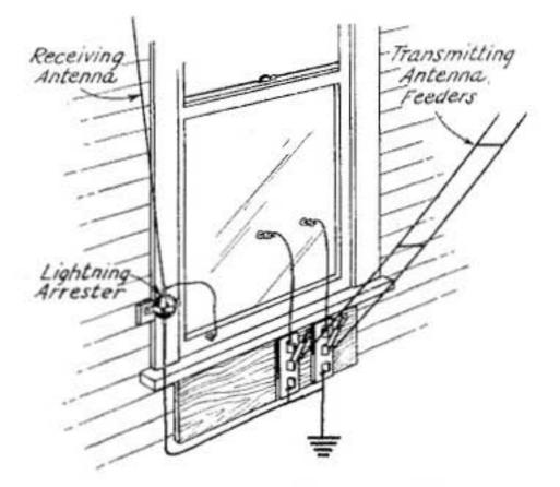
ANTENNA AND FEEDER GROUNDING METHODS FOR LIGHTNING PROTECTION
