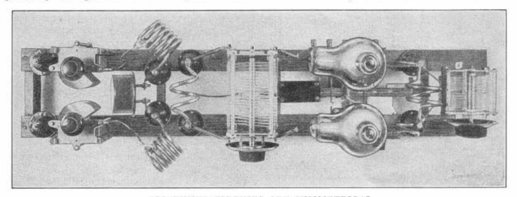
ALL TUNED CIRCUITS ARE SYMMETRICAL The air-dielectric blocking condenser is between the tubes and the plate-tank condenser. The inductances shown are for the 28,000-kc, band.
