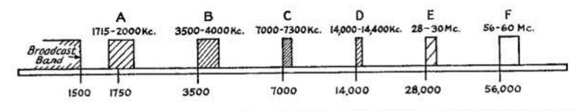
RELATIVE POSITION AND WIDTH OF THE AMATEUR BANDS IN THE HIGH FREQUENCY SPECTRUM (There is also a band from 400 to 401 Mc., not shown in this drawing)
