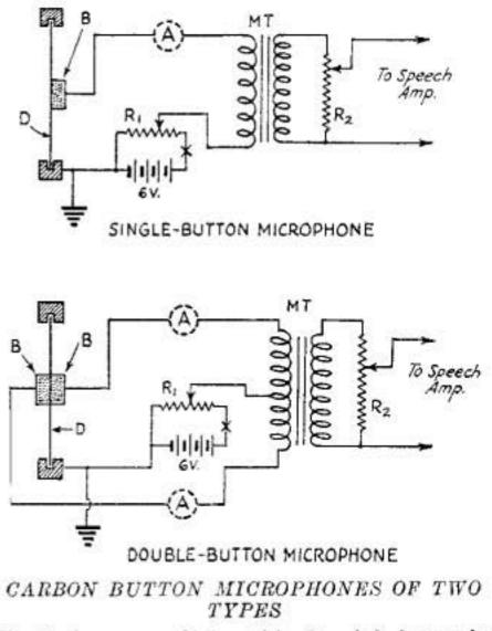
The diaphragms are designated by D and the buttons by B.  $R_1$  may be 400 ohms and the gain control  $R_2$  a 100,000-ohm potentiometer. The microphone frame should be grounded and the leads should be shielded to prevent r.f. pick-up.
