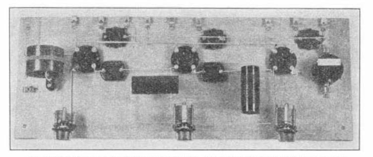
THE OSCILLATOR AND DOUBLER STAGES WITH THE TUBES REMOVED
