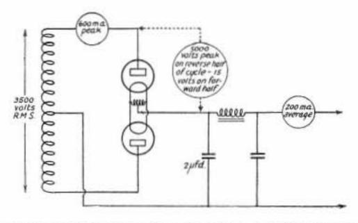
TWO MERCURY-VAPOR TUBES IN A FULL-WAVE CIRCUIT
