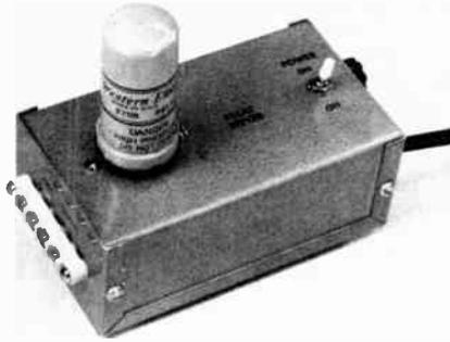
Fig. 11-17 — Relay driver as constructed by WA1CQW. The Western Electric 275B relay plugs into an octal socket.
