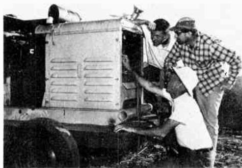
Fig. 10-5 — Gasoline-powered ac generators used for portable/emergency operation should be treated for ignition noise in the same manner as automobile engines are. The frame of the gas generator should be connected to an earth ground, and the entire unit should be situated as far from the operating position as possible. This will not only reduce ignition noise, but will minimize ambient noise from the power unit. (Shown here are WA6LXX, WA6HUB and W6PQH during portable operations.)
