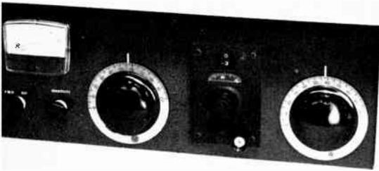
Fig. 20-16 – The universal Transmatch shown here will couple a transmitter to almost any antenna system. If the amateur already has a matching indicator, the Monimatch section of the circuit can be eliminated. The counter dial and knobs are James Millen & Co. components.
