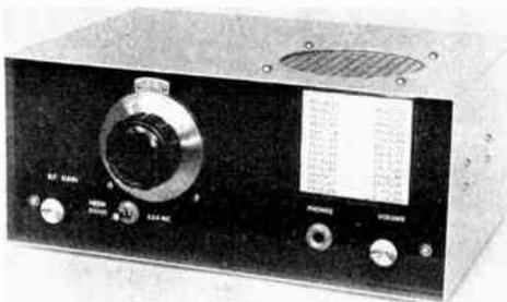
Fig. 8-52 — Front view of the direct-conversion receiver. The panel is finished in machine gray spray paint. The two controls are main tuning and audio gain.
