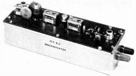
Fig. 14-23 — The solid-state fm adapter is constructed on a 6 X 2-inch etched-circuit board, mounted on a homemade chassis.
