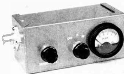
Fig. 17-51 — The completed Millimatch. At the left is the sensitivity control, R6. S1 is in the center, and M1 at the right.
