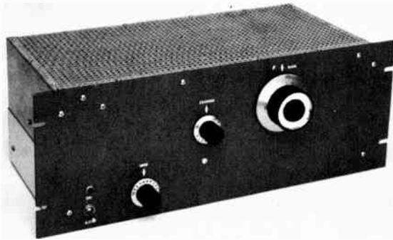
Fig. 7-31 — The 144-MHz amplifier is built in conventional rack-and-panel style, with the entire top of cane metal, to provide free air flow. Controls are grid-circuit tuning, C2, lower left; output loading capacitor, C5, center; and plate-circuit tuning, C4, with vernier dial, right. The slotted end of the Teflon shaft on C1 is visible as a white spot just below the loading control.
