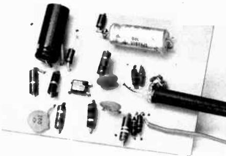
Fig. 1 — The solid-state T-R switch constructed on an etched circuit board of the pattern shown in *QST* for April, 1971, p. 32. The circuit could also be built on a piece of insulated or perforated board.
