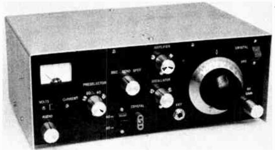
Fig. 10-33 — Front view of the cw transceiver. The chassis and cabinet are homemade, and consist of two U-shaped pieces of thick aluminum stock. The panel is painted dark green to permit the white decal labels to stand out prominently.
