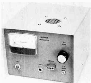
Fig. 1 — This is the completed transmitter for 160- to 20-meter operation. The plate tuning control is at the upper right, and just below, the loading capacitor, C2.
