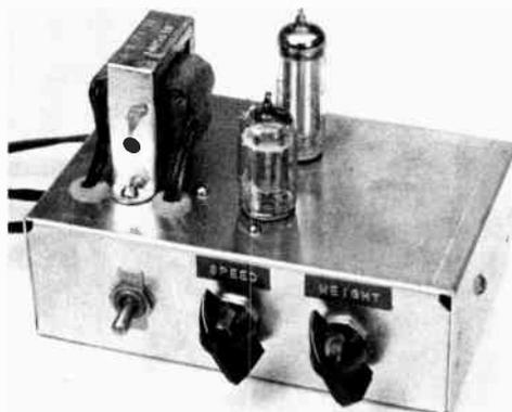
Fig. 11-11 — The single-tube keyer, housed in a 4 x 6 x 2-inch aluminum chassis. Power switch, speed and weight controls are mounted along the front apron. On top are the power transformer, the 12AU7 and 6B2 regulator.
