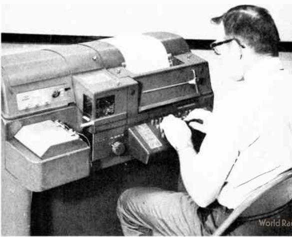
The Teletype Corp. Model 28ASR teleprinter is used by many amateurs. In addition to the keyboard and page printer, this model contains facilities for making and sending perforated tapes.
