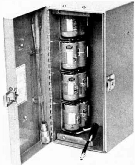
Fig. 10-59 — Eight size D cells are series connected to provide 12 volts. They are mounted in Keystone holders on the back wall of the bond box. The 1/4-inch diameter hole in the front of the cabinet (upper right of photo) permits final calibration of the receiver (C20) after the installation is completed. The hole is opposite the shaft of C20.
