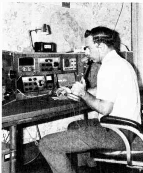
This modern-day operating position, built by W1ETU, is made from plywood and uses steel angle brackets to hold the wooden panels together. Cut outs in the console permit easy access to the equipment while enclosing the station wiring. This type of construction is ideal when the operating position is accessible to small children.
