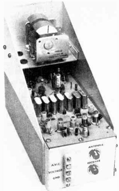
Fig. 8-51 — The front-end tuning capacitor, C1, is mounted on a small shelf just above the toroid coils. The rear section of the main circuit board contains the crystal oscillator. The crystals are soldered directly into the board. The capacitors that go with the oscillator-tank coils are connected across the terminals of the pc-mount coil forms. Most of the chokes and resistors are mounted vertically to save space.
