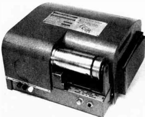
Fig. 15D-1 — Western Union Telefax transceiver. Some machines of this type have been made available to amateurs. The drum accommodates a sheet of paper measuring approximately 4 1/2 X 6 1/2 inches.
