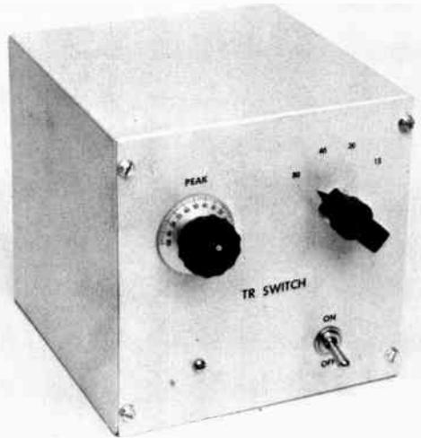
The vacuum-tube T-R switch shown in Figs. 1 through 4 differs in several ways from the preceding example. It contains its own power supply and consequently can be used with any transmitter/receiver combination without "borrowing" power. It will add gain and front-end selectivity to the receiver. A home made switch-coil-capacitor is shown in the unit, enabling the constructor to build his own.
