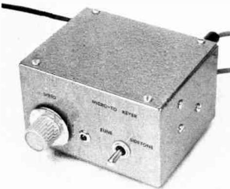
Fig. 11-14 — This electronic speed keyer is 100-percent solid state and uses both integrated circuits and bipolar transistors. It operates over a speed range of 10 to 50 wpm and contains its own built-in monitor. This circuit was originally described in *QST*, August, 1967, by K3CUW.
