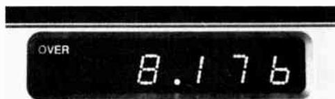
Fig. 6-12 — A 5-digit readout using light-emitting diodes.
