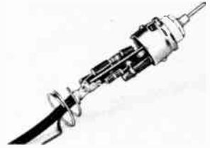
Fig. 17-58 — Inside the probe. The 1N34A diode, calibrating resistor, and input capacitor are mounted tight to the terminal strip with shortest leads possible. Spaghetti tubing is placed on the diode leads to prevent accidental short circuits. The tube-shield spring and flexible-copper grounding lead are soldered to the cable braid (the cable is RG-58/U coax). The tip can be either a phone tip or a short pointed piece of heavy wire.
