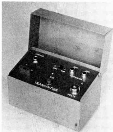
Fig. 1 — This version of the solid-state transmitter is housed in a small recipe box. All controls and jacks are accessible from the top panel.
