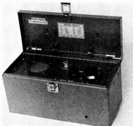
Fig. 10-54 — The 2-meter transceiver is housed in a legal-bond box. A homemade dial-calibration chart for the receiver is pasted on the inside of the lid. Two plastic cable clamps serve as holders for the two-section 1/4-wavelength whip antenna (inside lid) when the unit is not in use. The antenna is held together at the center by a homemade 1/4-inch diameter threaded coupling.
