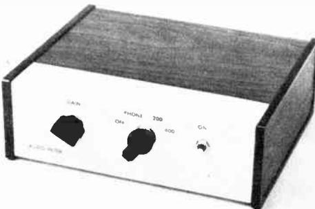
Fig. 8-45 — The phone/cw audio filter. (The basic filter designs were done by K1PLP, and the unit shown was constructed by W1ETU.)
