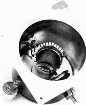
Fig. 7-47 — Interior of the plate circuit assembly, showing the center conductor with its ring of finger stock, the output-coupling loop, left, and the disk-type tuning capacitor, right.
