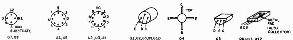
Base connections for the semiconductors used in the 2-meter transceiver.
