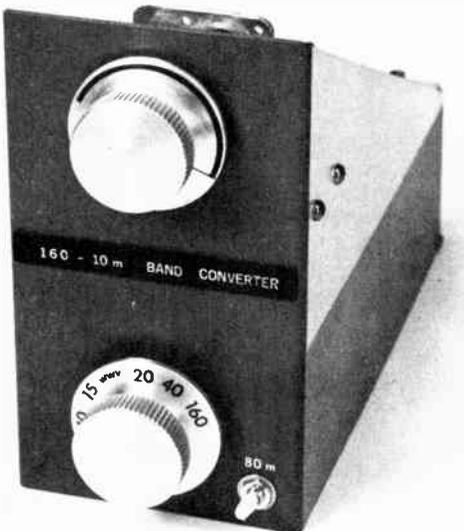
Front view of the hf converter. The upper knob controls the PRESLECTOR capacitor, while the lower control is for the band switch. The small switch to the lower right disconnects the converter from the antenna line.
