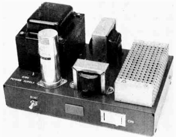
Fig. 1 — A top-chassis view of the general-purpose power supply. T1, at the far left, is a transformer from a discarded TV set. The high-wattage resistors are housed in the perforated shield at the far right. The bottom of the chassis is enclosed and has four rubber feet attached to the cover plate.
