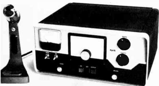
The ssb transmitter uses a minimum number of panel controls. Push-button switches activate the power supply and the output-metering function. A J. W. Miller MD-4 dial, LMB CO-1 cabinet and Simpson Wide-Vue meter lend a modern appearance to the unit.
