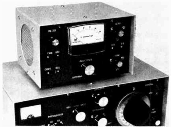
The QRP console is shown atop the QRP transmitter. These electrically compatible units have look-alike decor with green panels, white labels, and lye-bath finished aluminum covers. Kurz-Kasch 700 Series knobs are used on both pieces of gear (Catalog No. 112, Kurz-Kasch, Inc., Dayton, Ohio 45401).
