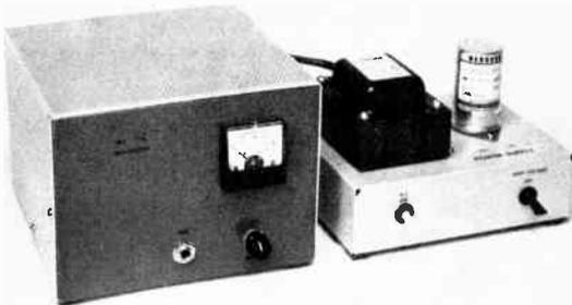
Fig. 14-35 — The front view of the 10-meter fm transmitter reveals only the plate-current meter, microphone-gain control and microphone jack.
