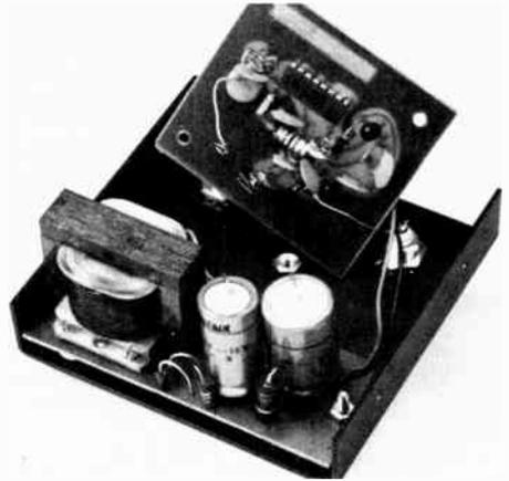
This 250-MHz prescaler uses the Fairchild U6B95 H 9059X IC. A power supply and an output amplifier complete the device.
