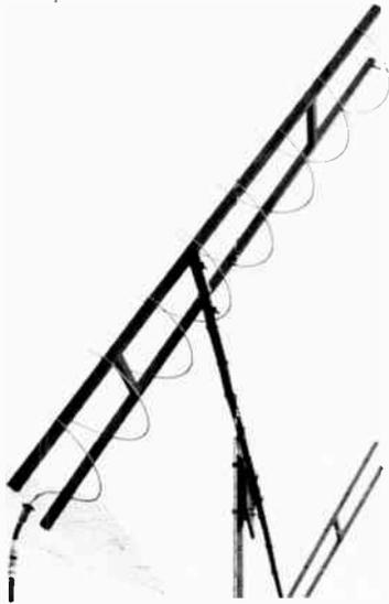
Fig. 22-20 — An 8-turn 432-MHz helical array, wound from aluminum clothesline wire. Left-hand polarization is shown. Each turn is one wavelength, with a pitch of 0.25 wavelength. Feed is with 50-ohm coax, through an 84-ohm  $Q$  section.
