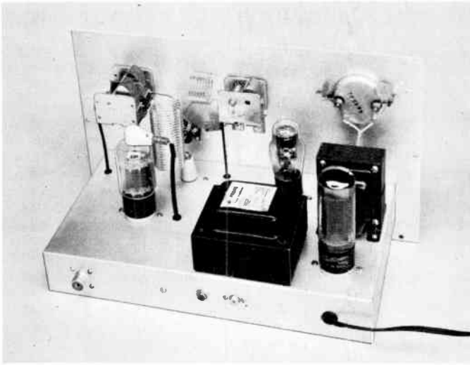
Fig. 6-37—Rear view of the transmitter showing the placement of components above chassis. The loading capacitor, C_6 , is at the left, L_3 is the vertical coil and L_2 the horizontal one. Rubber grommets are used to prevent chafing and to furnish additional insulation on the leads coming from below chassis.
