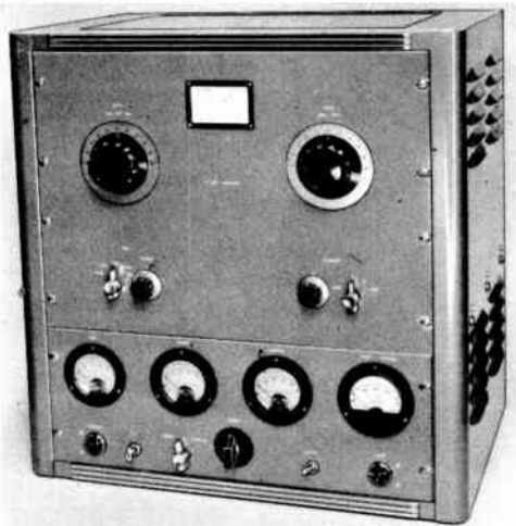
Fig. 6-68—The kilowatt 4-400A amplifier and its control unit are mounted in a 21-inch gray hommer-tone rack cabinet (Bud CR-1727). Shelf brackets (Bud SA-1350) are mounted on both sides of the cabinet to hold the amplifier chassis. Below the meters, from left to right: filament pilot light, key-type a.c. switch, Class AB 1 /C bias switch, screen autotransformer, plate switch and plate pilot light.
