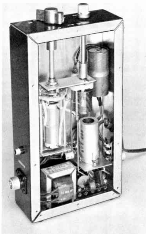
Fig. 8-16—The electronic t.r. switch is built in a 5 \times 9 \times 2\frac{1}{2} -inch chassis; the bottom plate has been removed to show the placement of parts. Although two receiver outlets are shown on the near face (a phono jack and a coaxial receptacle), only one is required, depending upon one's choice of cable termination.
