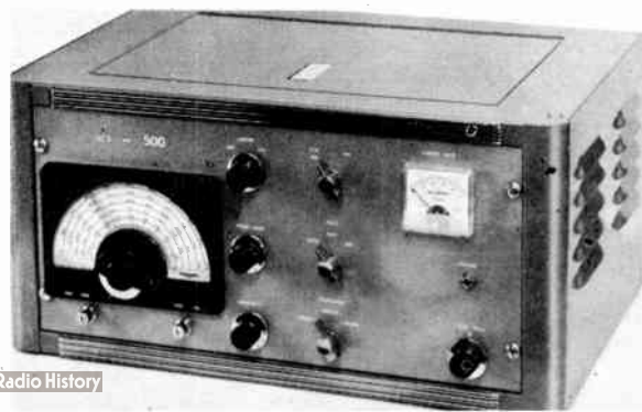
Fig. 5-51—The DCS-500 double-conversion superheterodyne. Left bottom, antenna trimmer, 100-kc. calibrator switch; center, left, top to bottom, noise-limiter switch, volume control, sensitivity control; center, right, b.f.o. switch, a.g.c. speed, selectivity; right, headphone jack, b.f.o. pitch control. The dial is a National ICN. Front panel is 8 1/4 inches high; the receiver is mounted in a Bud CR-1741 rack cabinet.
