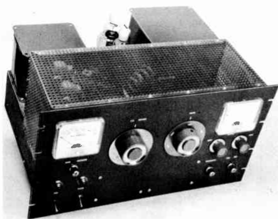
Fig. 6-64—This amplifier operates at a plate input of approximately 500 watts, uses a pair of 811As in grounded-grid, and is complete with power supply on a 13 \times 17 \times 4 -inch chassis. The rack panel is 10\frac{1}{2} by 19 inches. Front-panel controls include the plate tuning capacitor and band switch in the center, filament and plate power switches with their pilot lights at the lower left, sensitivity control and forward-reflected power switch for the directional coupler at the lower right, variable loading capacitor and auxiliary loading-capacitor switch underneath the 0.1 milliammeter at the right, and the grid-cathode milliammeter with its switch at the upper left. The filter choke, 866As and plate transformer occupy the rear section of the chassis.
