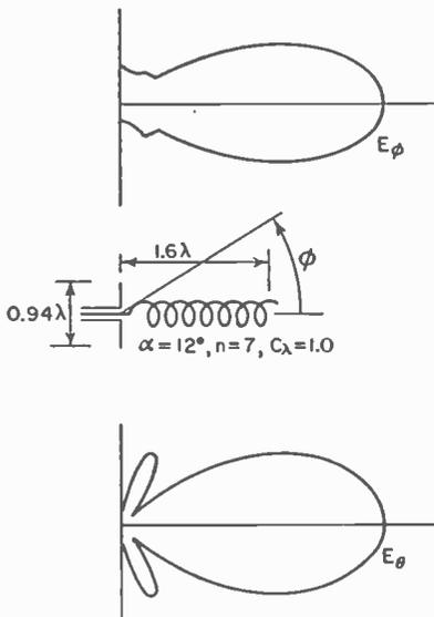
FIG. 7-7. Field patterns of  $12^\circ$ , 7-turn helix radiating in the axial mode. The helix circumference is 1 wavelength. Both  $E_\phi$  and  $E_\theta$  patterns are shown as a function of  $\phi$ .  $E_\phi$  is in the plane of the page, and  $E_\theta$  is normal to the page.
