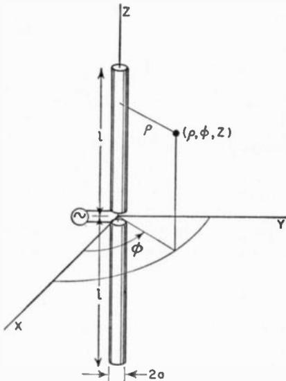
FIG. 9-1. Symmetrical center-fed cylindrical antenna with relation to coordinates.
