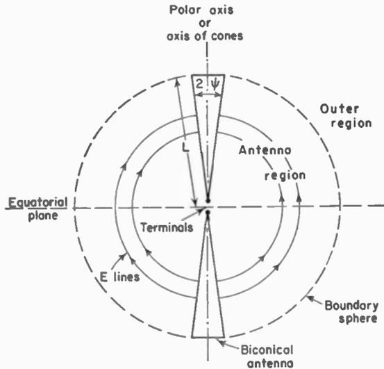
FIG. 1-4. Schelkunoff's biconical antenna with boundary sphere.
