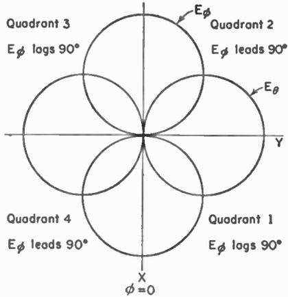
FIG. 2-23. Field patterns for source of Example 3.
