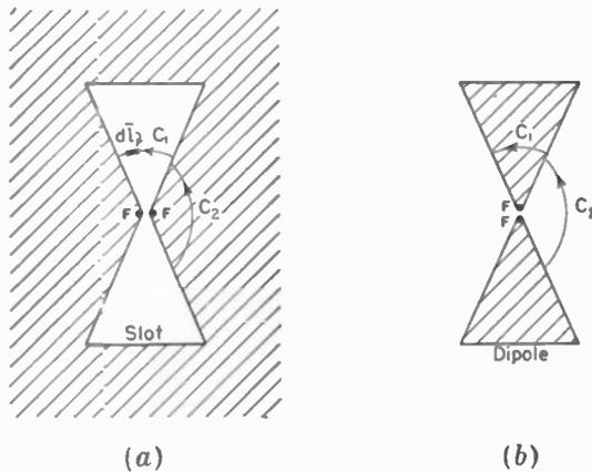
FIG. 13-16. Slot antenna and complementary dipole antenna.
