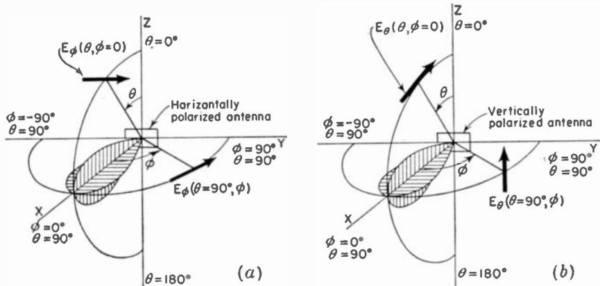
FIG. 15-3. Vertical and horizontal plane patterns for horizontally polarized antenna (a) and vertically polarized antenna (b).
