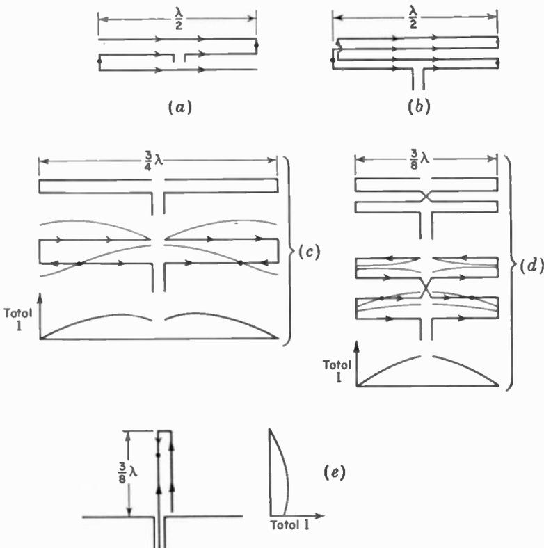
FIG. 14-26. (a). Three-wire folded  $\frac{1}{2}$ -wavelength dipole, (b) four-wire folded  $\frac{1}{2}$ -wavelength dipole, (c) two-wire  $\frac{3}{4}$ -wavelength antenna, (d) four-wire  $\frac{3}{8}$ -wavelength antenna, and (e) two-wire  $\frac{3}{8}$ -wavelength stub antenna. Arrows indicate instantaneous current directions, and dots indicate current minimum points.
