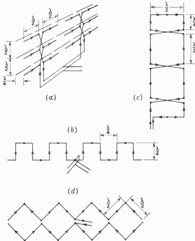
FIG. 14-23. (a) Array of  $\frac{1}{2}$ -wavelength dipoles with reflectors, (b) symmetrical Bruce antenna, (c) Sterba curtain array, and (d) Chireix-Mesny array. Arrows indicate instantaneous current directions, and dots indicate current minimum points.
