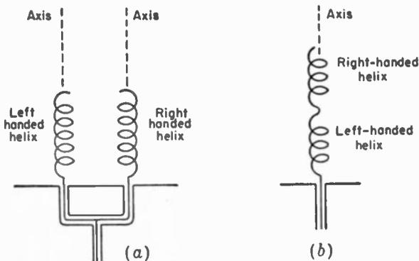
FIG. 7-38. Helical antenna arrangements for producing linear polarization.
