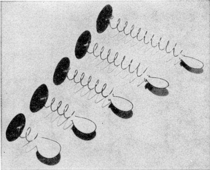
FIG. 7-21. Models showing effect of number of turns on measured field patterns. Helices have  $12.2^\circ$  pitch angle and 2, 4, 6, 8, 10 turns. Patterns shown are average of measured  $E_\theta$  and  $E_\phi$  patterns.
