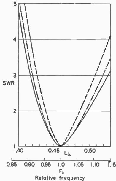
FIG. 14-44. SWR as a function of antenna length  $L$  in wavelengths and as a function of the frequency (the resonant frequency  $F_0$  is taken as unity). The SWR curves are for the same three cases of Fig. 14-43.
