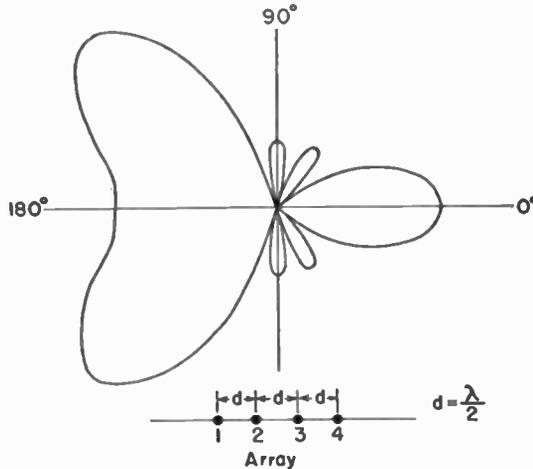
FIG. 4-23. Field pattern of end-fire array of four isotropic point sources of equal amplitude spaced  $\frac{1}{2}$  wavelength apart. The phasing is adjusted for increased directivity ( $\delta = -\frac{3}{4}\pi$ ).
