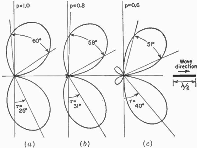
FIG. 5-16. Far-field patterns of linear  $\frac{1}{2}$ -wavelength antenna carrying a uniform traveling wave (to right) for three conditions of relative phase velocity ( $p = 1.0, 0.8,$  and  $0.6$ ). The tilt angle  $\tau$  and the half-power beam widths are indicated for each pattern.
