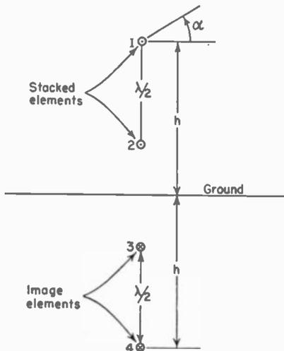
FIG. 11-31. Array of stacked horizontal  $\frac{1}{2}$ -wavelength elements.
