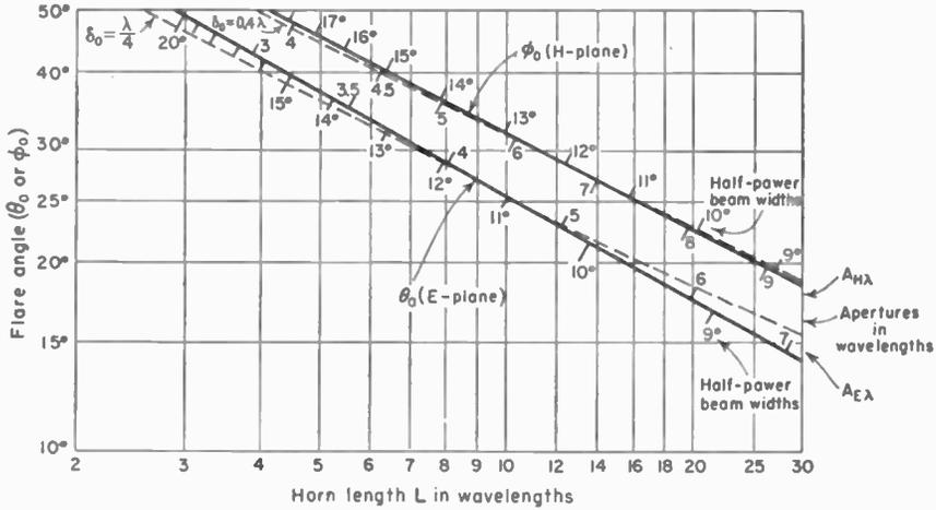
FIG. 13-22. Experimentally determined optimum dimensions for rectangular horn antennas. Solid curves give relation of flare angle  $\theta_0$  in  $E$  plane and flare angle  $\phi_0$  in  $H$  plane to horn length (see Fig. 13-20). The corresponding half-power beam widths and apertures in wavelengths are indicated along the curves. Dashed curves show calculated dimensions for  $\delta_0 = 0.25 \lambda$  and  $0.4 \lambda$ .
