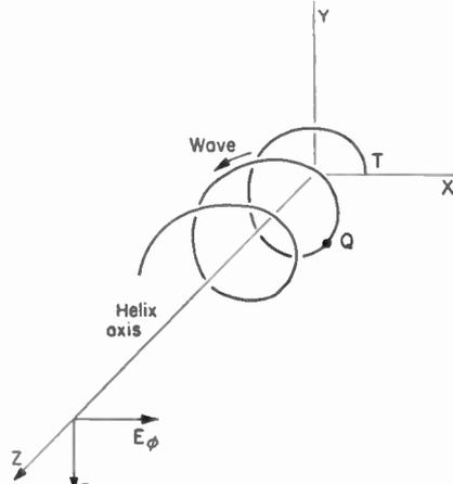
FIG. 7-28. Field components in the direction of the helix axis.
