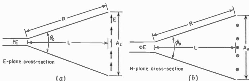
FIG. 13-20.  $E$ -plane and  $H$ -plane cross sections.
