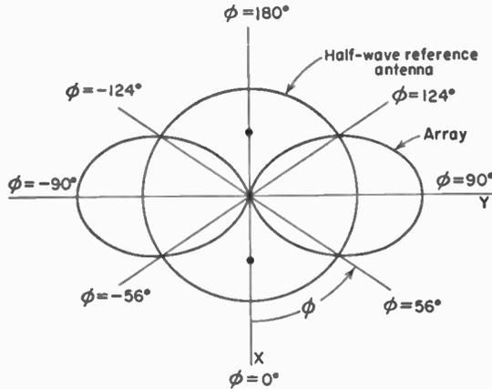
FIG. 11-4. Horizontal plane pattern of broadside array of two vertical in-phase  $\frac{1}{2}$ -wavelength elements spaced  $\frac{1}{2}$  wavelength. The pattern of a single vertical  $\frac{1}{2}$ -wavelength reference antenna with the same power input is shown for comparison.
