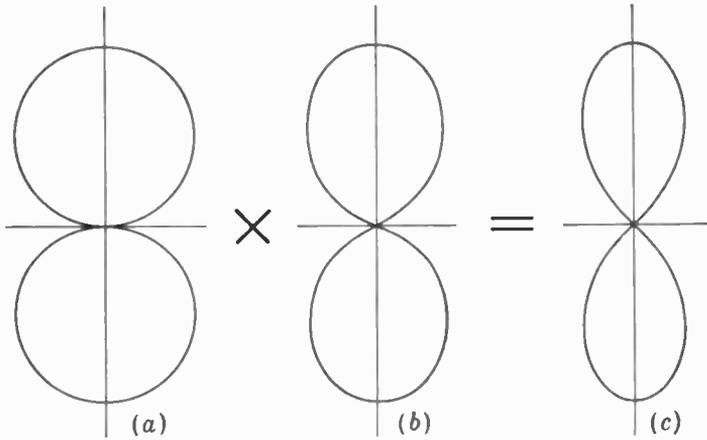
FIG. 4-8. Example of pattern multiplication. Two nonisotropic but identical point sources of same amplitude and phase, spaced  $\frac{1}{2}$  wavelength apart, and arranged as in Fig. 4-7, produce the pattern shown at (c). The individual source has the pattern shown at (a), which, when multiplied by the pattern of an array of two isotropic point sources (of the same amplitude and phase) as shown at (b), yields the total array pattern of (c).
