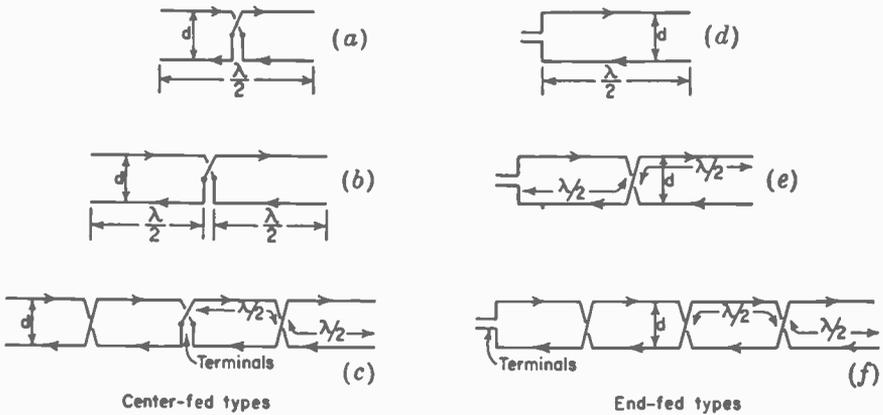
FIG. 11-16. Six types of flat-top beam antennas.
