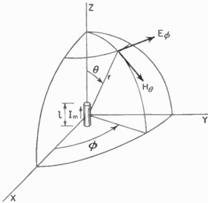
FIG. 6-5. Relation of short magnetic dipole to coordinates.
