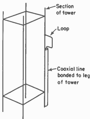
FIG. 15-19b. Current sampling loop on broadcast-station tower.
