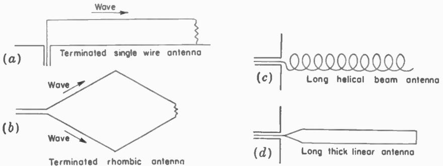
FIG. 5-14. Various antennas having essentially a single traveling wave.
