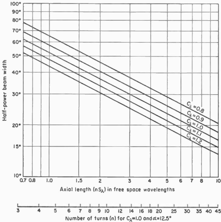
FIG. 7-22. Half-power beam width of axial mode helical antenna as a function of the axial length and circumference in free-space wavelengths and also as a function of the number of turns for  $C_\lambda = 1.0$  and  $\alpha = 12.5^\circ$ .
