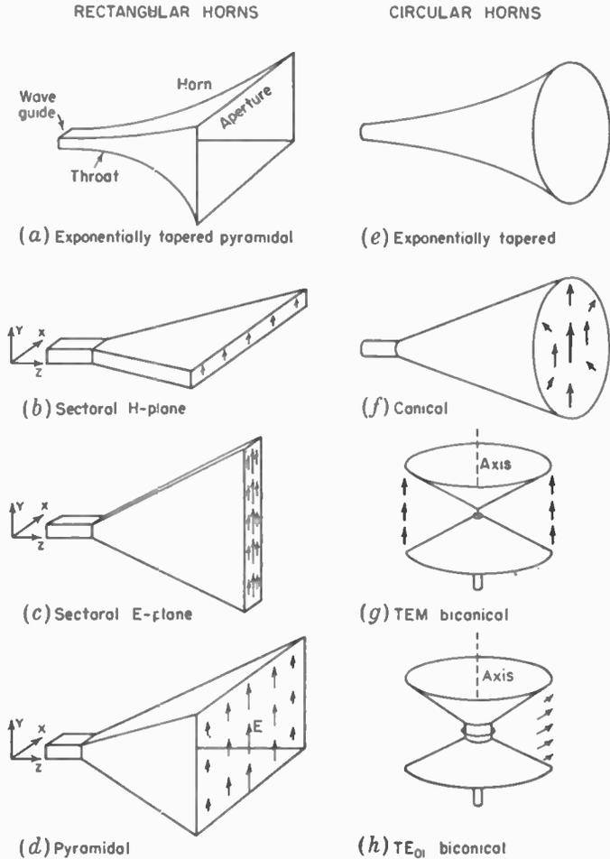
FIG. 13-18. Types of rectangular and circular horn antennas.
