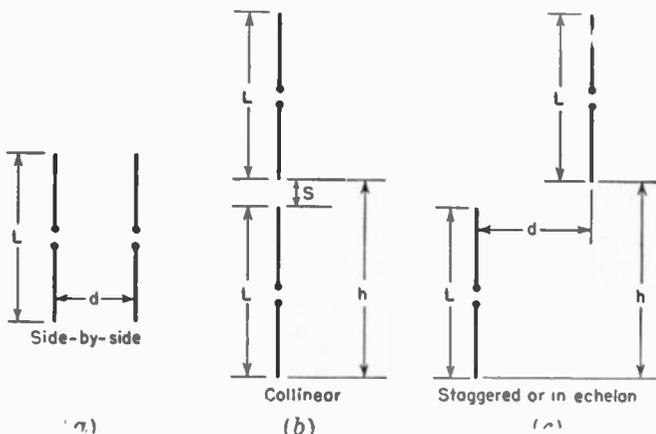
FIG. 10-10. Three arrangements of two parallel antennas.
