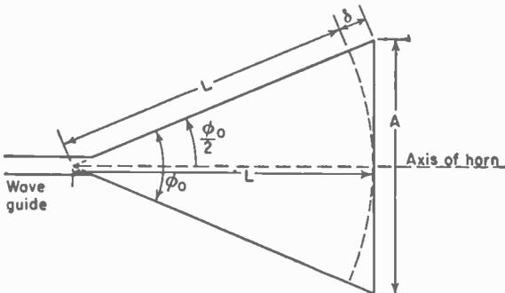
FIG. 13-19. Construction for finding path difference  $\delta$ .
