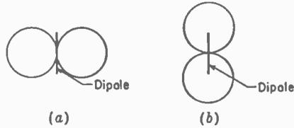
FIG. 5-6. Near- and far-field patterns of  $E_\theta$  and  $H_\phi$  components for short dipole (a) and near-field pattern of  $E_r$  component (b).
