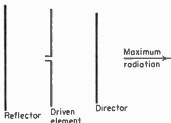
FIG. 11-39. Three-element array.
