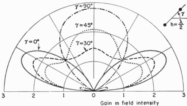
FIG. 11-29. Vertical-plane patterns for horizontal two-element flat-top beam antenna with  $\frac{1}{4}$  wavelength spacing at an average height of  $\frac{1}{2}$  wavelength above ground for tilt angles  $\gamma = 0^\circ, 30^\circ, 45^\circ,$  and  $90^\circ$ . Patterns give gain in field intensity over a single  $\frac{1}{2}$ -wavelength antenna in free space with the same power input.
