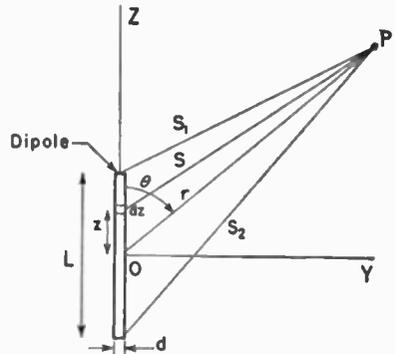
FIG. 5-3. Geometry for short dipole.
