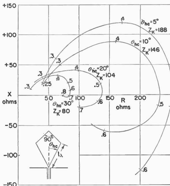
FIG. 8-13. Measured input impedance of single cones with ground plane as a function of cone length in wavelengths ( $l_\lambda$ ). Impedance curves are presented for cones with half-angles of  $5^\circ$ ,  $10^\circ$ ,  $20^\circ$ , and  $30^\circ$ .
