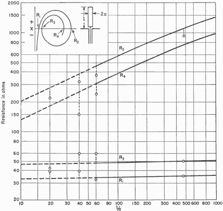
FIG. 9-12. Resonant resistance of cylindrical stub antenna with ground plane as a function of the length-to-radius ratio ( $l/a$ ). Curves are shown for the first four resonances. For cylindrical center-fed antennas (total length  $2l$ ) multiply the resistance by 2.
