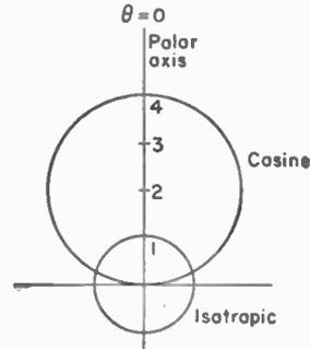
FIG. 2-7. Power patterns of unidirectional cosine source compared with isotropic source for same power radiated by both.
