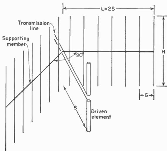
FIG. 12-13. Grid-type reflector.
