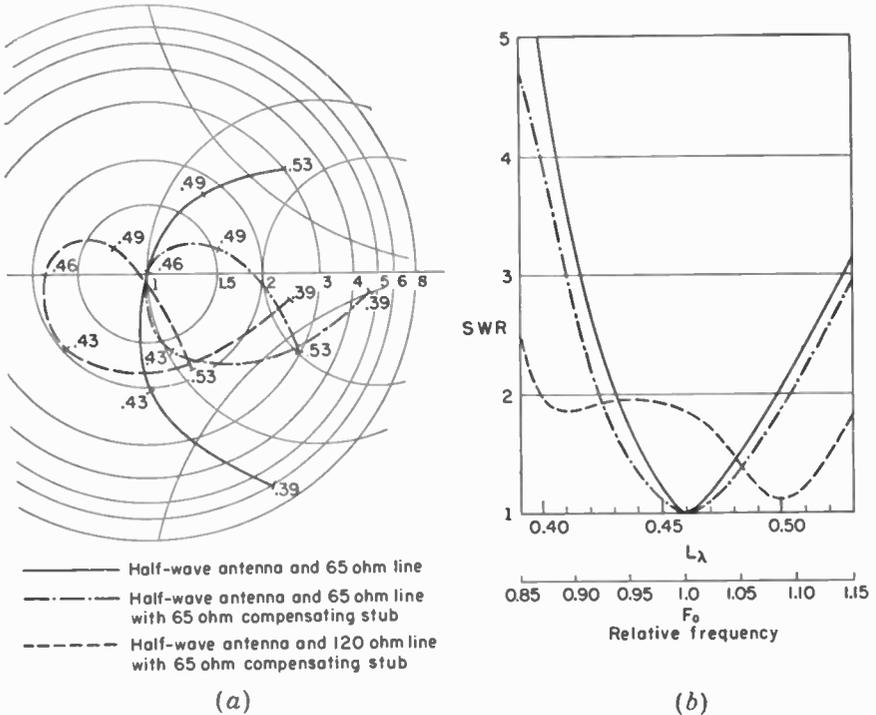
FIG. 14-45. Normalized impedance (a) and SWR (b) for cylindrical  $\frac{1}{4}$ -wavelength dipole ( $L/D = 60$ ) fed directly with 65-ohm line as in Fig. 14-42a (solid curves); with 65-ohm line and 65-ohm  $\frac{1}{2}$ -wavelength compensating stub as in Fig 14-42f (dash-dot curves); and with a 120-ohm line and 65-ohm  $\frac{1}{2}$ -wavelength compensating stub (dashed curves).
