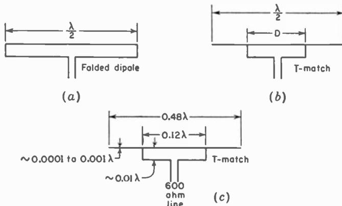
FIG. 14-27. Folded dipole and T-match antennas.
