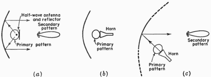
FIG. 12-18.2. Parabolic reflectors with various feed arrangements.
