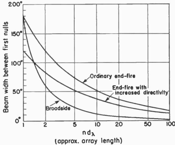
FIG. 4-26. Beam width between first nulls as a function of  $nd_\lambda$  for arrays of  $n$  isotropic point sources of equal amplitude. For long arrays,  $nd_\lambda$  is approximately equal to the array length.
