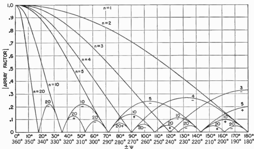
FIG. 4-20. Universal field-pattern chart for arrays of various numbers  $n$  of isotropic point sources of equal amplitude and spacing. Charts for all integral values of  $n$  from 1 through 24 are included in the Appendix.
