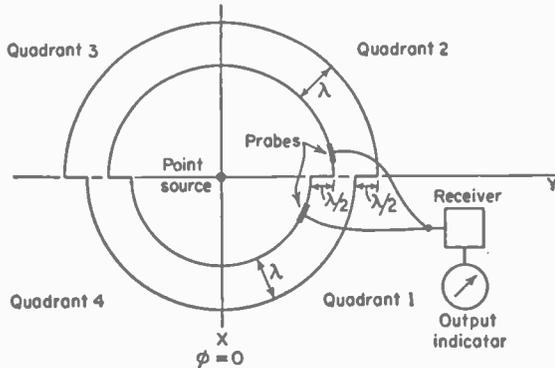
FIG. 2-22. Constant phase contours for source of Example 2.
