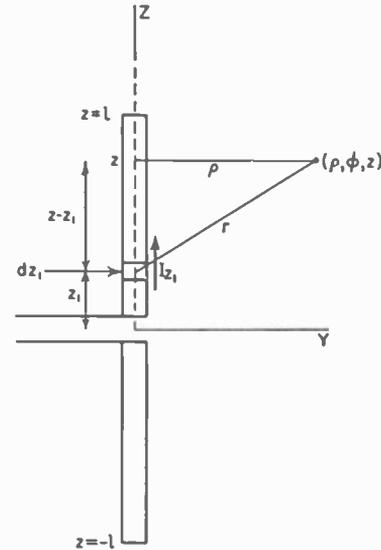
FIG. 9-3. Construction for obtaining vector potential  $A_s$ .
