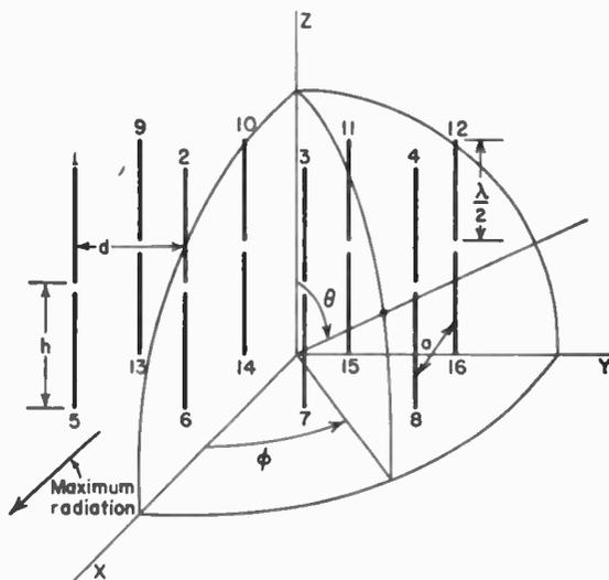
FIG. 11-17. Array of 16  $\frac{1}{2}$ -wavelength elements.
