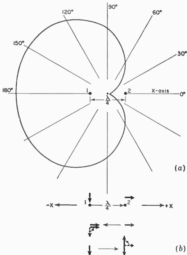
FIG. 4-5. (a) Relative field pattern of two isotropic sources of same amplitude and in phase quadrature for a spacing of  $\frac{1}{4}$  wavelength. Source 2 leads source 1 by  $90^\circ$ . (b) Vector diagrams illustrating field reinforcement in  $-x$  direction and field cancellation in  $+x$  direction.
