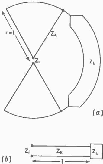
FIG. 8-9. Finite or terminated biconical antenna and equivalent transmission line.
