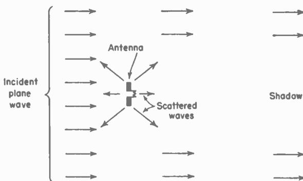
FIG. 3-4. Shadow cast by a receiving antenna.
