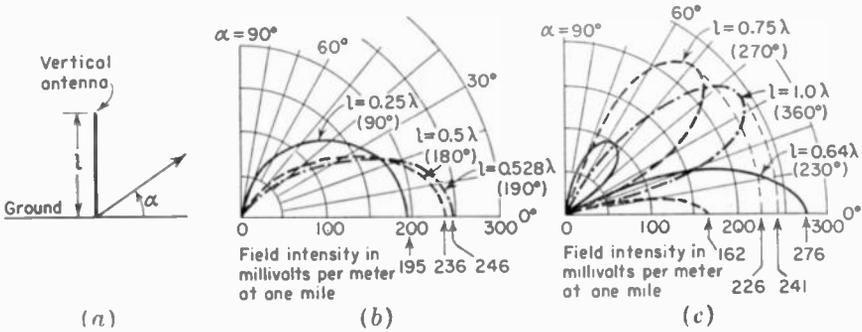
FIG. 11-36. Vertical-plane field patterns of vertical antennas for several values of antenna height  $l$ . The field intensity is expressed in millivolts per meter at a distance of 1 mile for 1 kilowatt input. Perfectly conducting ground and zero loss resistance are assumed.
