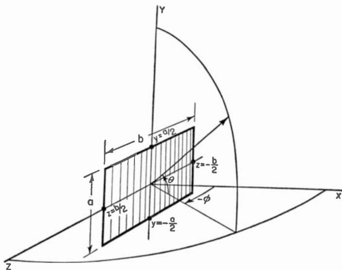
FIG. 4-13. Rectangular broadside array of height  $a$  and length  $b$  with relation to coordinates.
