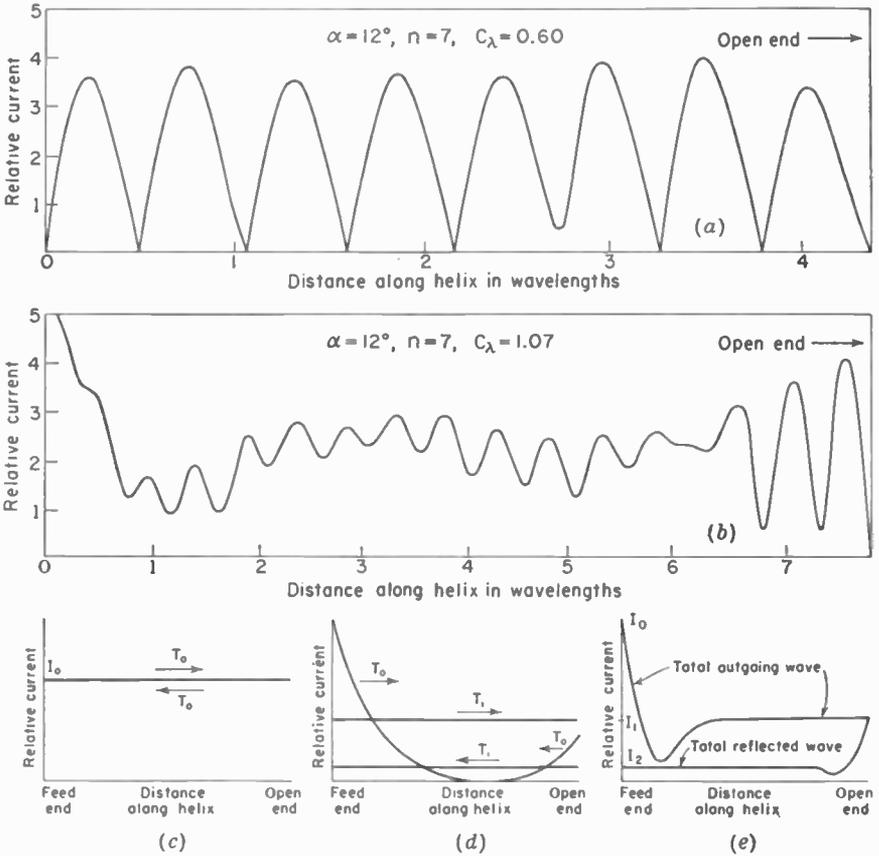
FIG. 7-13. (a) Measured current distribution on helix of 0.6 wavelength circumference. (b) Measured current distribution on same helix at higher frequency ( $C_\lambda = 1.07$ ) with radiation in the axial mode.
