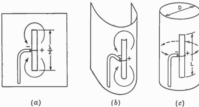
FIG. 14-33. Evolution of slotted cylinder from slotted sheet.
