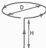
tain a circularly polarized far field at all points at which the field is not zero. The loop is circular and is horizontal, and the linear conductor of length  $H$  is vertical. Assume  $D$  and  $H$  small compared to the wavelength, and assume the current of uniform magnitude and in phase over the system.
