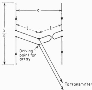
FIG. 11-8. End-fire array of two linear  $\frac{1}{2}$ -wavelength elements with arrangement for driving elements with currents of equal magnitude but opposite phase.
