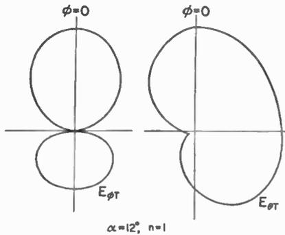
FIG. 7-25. Calculated single turn patterns for  $12^\circ$  helix.
