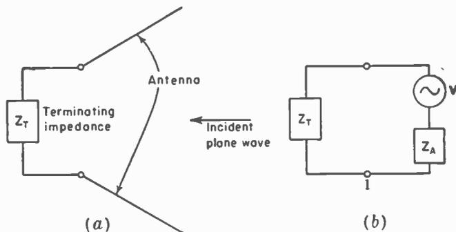
FIG. 3-2. Schematic diagram of antenna terminated in impedance  $Z_T$  with plane wave incident on antenna (a) and equivalent circuit (b).
