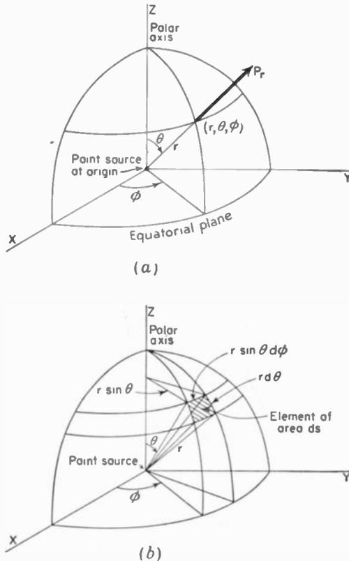
FIG. 2-2. Spherical coordinates for a point source of radiation in free space.
