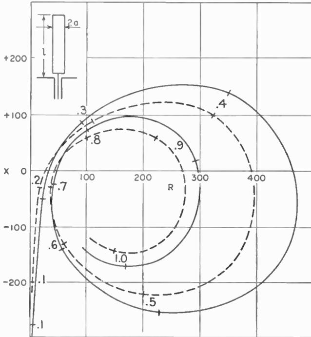
FIG. 9-10. Comparison of calculated (solid curve) and measured (dashed curve) input impedance ( $R + jX$ ) in ohms for cylindrical stub antenna with ground plane for length-to-radius ratio ( $l/a$ ) of 60.
