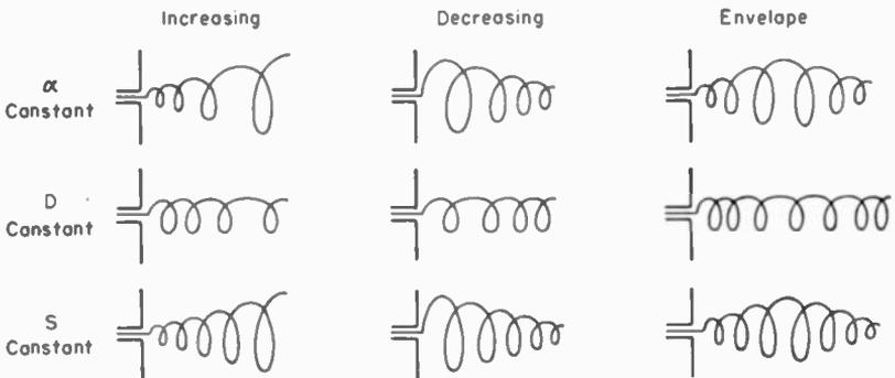
FIG. 7-36. Types of tapered axial mode helical antennas.
