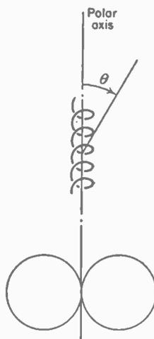
FIG. 7-6. A small helix and its radiation pattern.
