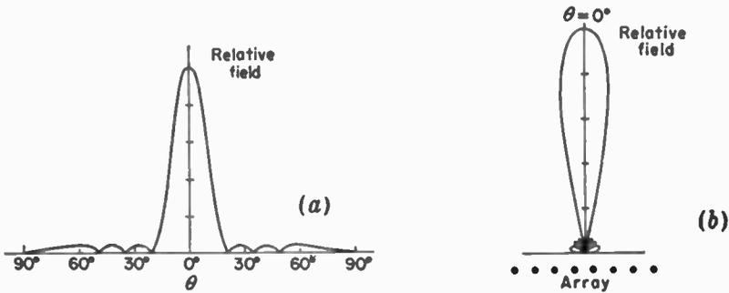
FIG. 4-35. Relative field pattern of broadside array of eight isotropic sources spaced  $\frac{1}{2}$  wavelength apart. The amplitude distribution gives a minimum beam width for a side-lobe level one-twentieth of the main lobe. The pattern is shown in rectangular coordinates at (a) and in polar at (b). Both diagrams show the pattern only from  $-90^\circ$  to  $+90^\circ$ , the other half of the pattern being identical.
