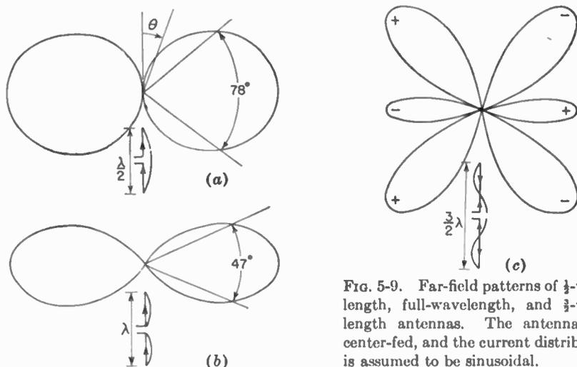
FIG. 5-9. Far-field patterns of  $\frac{1}{2}$ -wavelength, full-wavelength, and  $\frac{3}{2}$ -wavelength antennas. The antennas are center-fed, and the current distribution is assumed to be sinusoidal.
