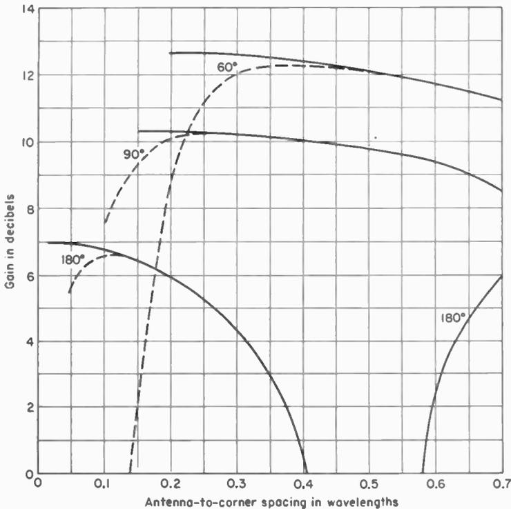
FIG. 12-9. Gain of corner reflector antennas over a  $\frac{1}{2}$ -wavelength antenna in free space with the same power input as a function of the antenna-to-corner spacing. Gain is in the direction  $\phi = 0$  and is shown for zero loss resistance (solid curves) and for an assumed loss resistance of 1 ohm ( $R_{1L} = 1$  ohm) (dashed curves).
