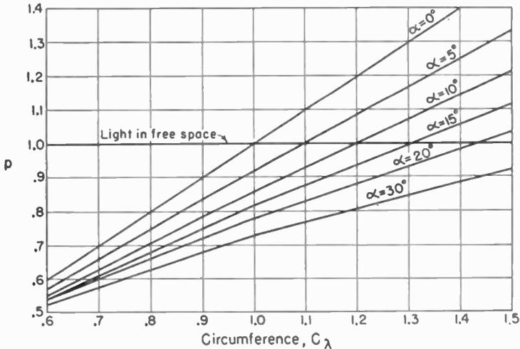
FIG. 7-17. Relative phase velocity  $p$  for different pitch angles  $\alpha$  as a function of the helix circumference in free-space wavelengths  $C_\lambda$  for the condition of in-phase fields in the axial direction.
