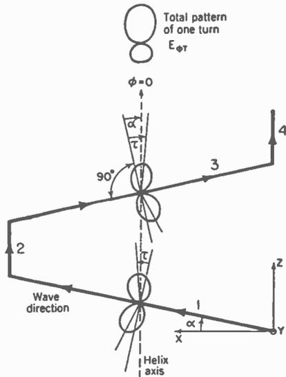
FIG. 7-26. Individual  $E_\phi$  patterns of elements 1 and 3 and total pattern of single turn,  $E_{\phi T}$ . The single turn is shown in plan view (in  $x$ - $z$  plane of Fig. 7-23). The single turn and coordinate axes have been rotated around the  $y$  axis so that the  $z$ -direction ( $\phi = 0$ ) is toward the top of the page.
