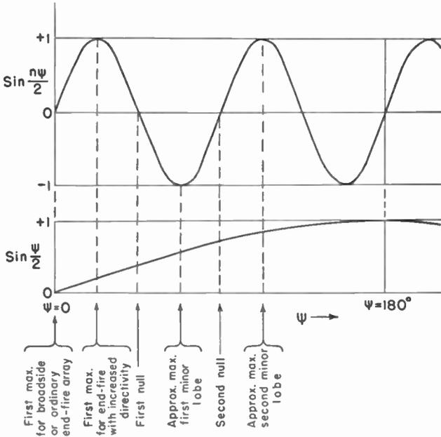
FIG. 4-28. Graphs of the numerator ( $\sin n\psi/2$ ) and denominator ( $\sin \psi/2$ ) of the array factor as functions of  $\psi$ , showing the values of  $\psi$  corresponding to maxima and nulls of a field pattern for the case  $n = 8$ .
