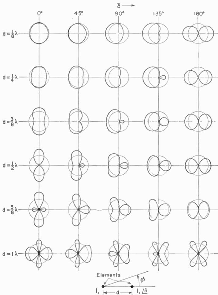
FIG. 11-11. Horizontal-plane field patterns of two vertical elements as a function of the phase difference  $\delta$  and spacing  $d$ . (After G. H. Brown.) Both elements are the same length and have currents of equal magnitude. The circles indicate the field intensity of a single reference element of the same length with the same power input.
