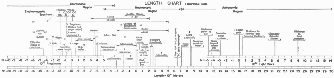
FIG. 1-3. Length chart. The main scale gives lengths in meters, the length being expressed by the exponent  $N$  where the length in meters equals  $10^N$ . Thus,  $N = \log_{10}(\text{length})$ . For example, 1 light-second =  $3 \times 10^8$  meters so that for this length,  $N = \log_{10} 3 + 8 = 8.48$ . Two auxiliary scales give lengths also in angstrom units and in light-years.
