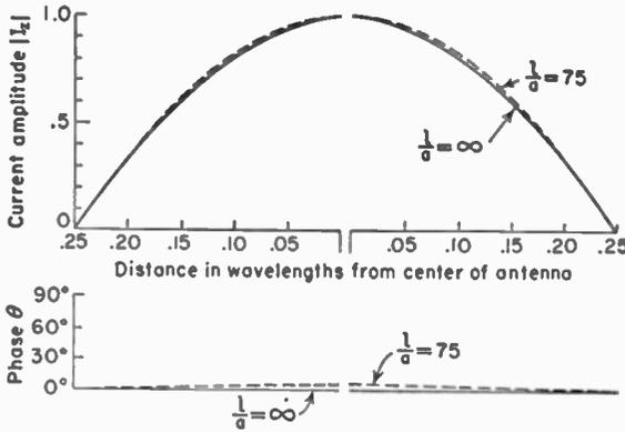
Fig. 9-6. Relative current amplitude and phase along a center-fed  $\frac{1}{2}$ -wavelength cylindrical antenna ( $2l = \lambda/2$ ) for total length-to-diameter ratios ( $l/a$ ) of 75 and infinity (after King and Harrison). Distance from the center of the antenna is expressed in wavelengths.
