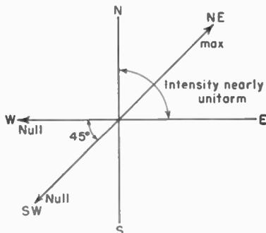
Design a four-vertical-tower array to fulfill these requirements. The currents are to be equal in magnitude in all towers, but the phase may be adjusted to any relationship. There is also no restriction on the spacing or geometrical arrangements of the towers. Plot the field pattern.
