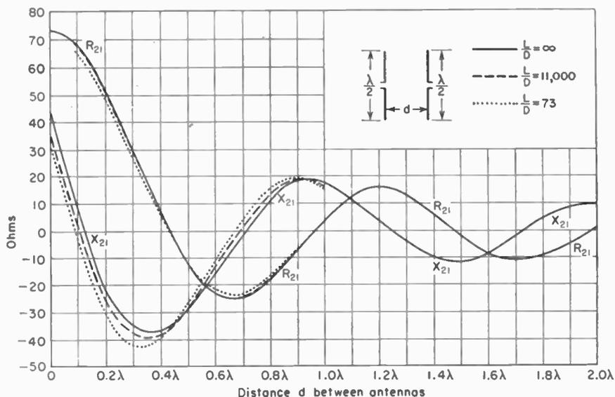
FIG. 10-12. Curves of mutual resistance ( $R_{21}$ ) and reactance ( $X_{21}$ ) of two parallel side-by-side linear  $\frac{1}{2}$ -wavelength antennas as a function of distance between them. Solid curves are for infinitesimally thin antennas as calculated from Carter's formulas. Dashed and dotted curves between 0 and  $1.0 \lambda$  spacing are from Tai's data for antennas with  $L/D$  ratios of 11,000 and 73 respectively.
