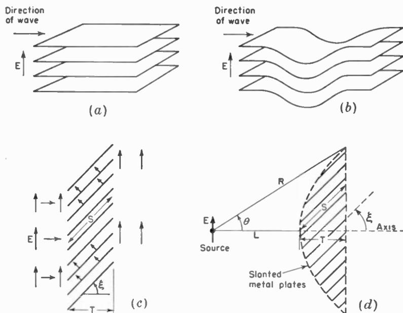
FIG. 14-18. (a)  $H$ -plane stack of flat metal plates. (b)  $H$ -plane stack with increased path length. (c) Slanted  $H$ -plane plates. (d)  $H$ -plane metal-plate lens using slanted plate construction.
