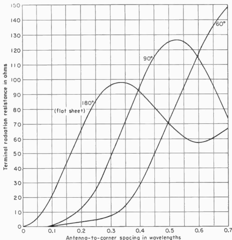
FIG. 12-11. Terminal radiation resistance of driven  $\frac{1}{4}$ -wavelength antenna as a function of the antenna-to-corner spacing for corner reflectors of three corner angles.
