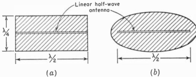
FIG. 3-7. (a) Maximum effective aperture of linear  $\frac{1}{2}$ -wavelength antenna is approximately represented by rectangle  $\frac{1}{2}$  by  $\frac{1}{4}$  wavelength on a side. (b) Maximum effective aperture of linear  $\frac{1}{2}$ -wavelength antenna represented by elliptical area of 0.13 square wavelength.
