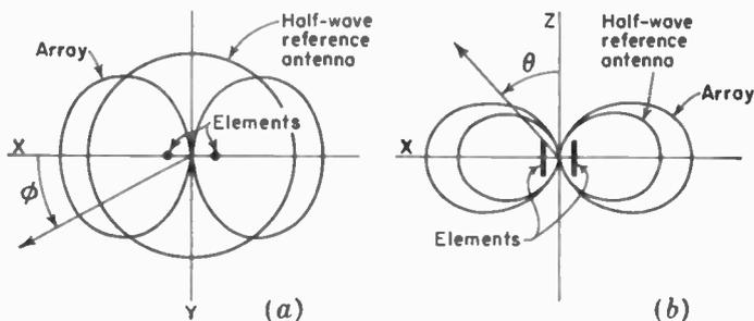
FIG. 11-9. Horizontal plane pattern (a) and vertical plane pattern (b) of end-fire array of two vertical  $\frac{1}{2}$ -wavelength elements with  $\frac{1}{2}$ -wavelength spacing. The patterns of a vertical  $\frac{1}{2}$ -wavelength reference antenna with the same power input are shown for comparison.
