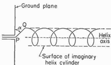
FIG. 7-15. Terminal arrangement of helical beam antenna.
