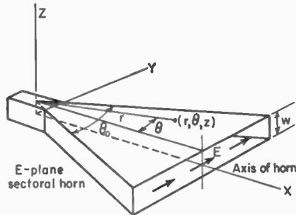
FIG. 13-23. Cylindrical coordinates for  $E$ -plane sectoral horn.
