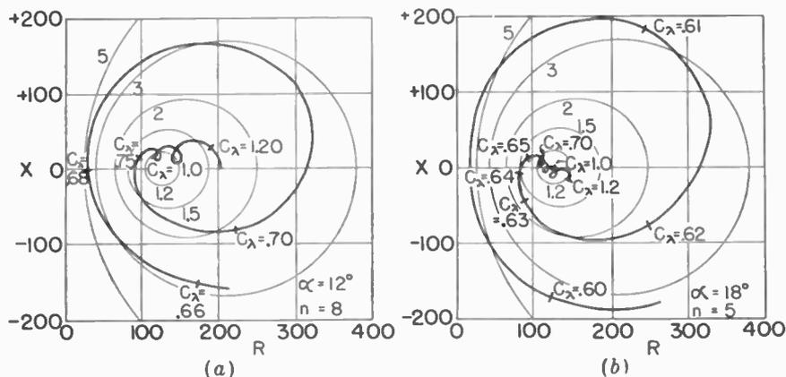
FIG. 7-14. Measured impedance spiral for  $12^\circ$ , 8-turn helix (a) and  $18^\circ$ , 5-turn helix (b). The helices are of fixed physical size. The impedance (resistance  $R$  and reactance  $X$ , in ohms) is shown as a function of frequency, the circumference in wavelengths at a given frequency being indicated at intervals along the spirals.
