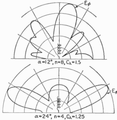
FIG. 7-8. Examples of multilobed and conical patterns.
