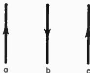
(b) is in antiphase. The self-resistance of each antenna is 100 ohms, while the mutual resistances are:  $R_{ab} = R_{bc} = 40$  ohms and  $R_{ac} = -10$  ohms. What is the radiation resistance of each of the antennas? The resistances are referred to the terminals, which are in the same location in all antennas.
