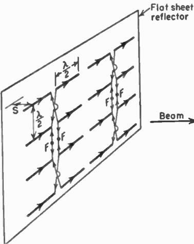
FIG. 12-5. Array of  $\frac{1}{2}$ -wavelength elements with flat sheet reflector (billboard or mattress antenna).
