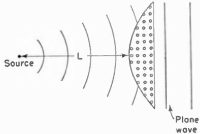
FIG. 14-6. Artificial dielectric lens of metal spheres.
