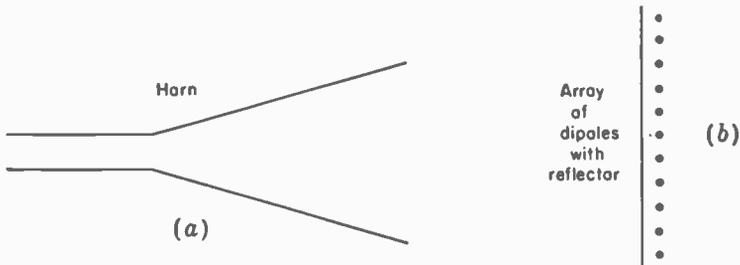
FIG. 4-42. Electromagnetic horn antenna and array of dipoles with reflector.
