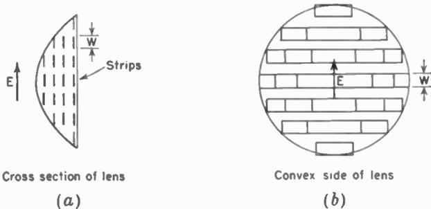
FIG. 14-7. Artificial dielectric lens of flat metal strips.
