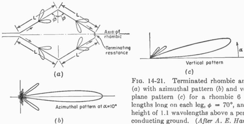
FIG. 14-21. Terminated rhombic antenna (a) with azimuthal pattern (b) and vertical plane pattern (c) for a rhombic 6 wavelengths long on each leg,  $\phi = 70^\circ$ , and at a height of 1.1 wavelengths above a perfectly conducting ground. (After A. E. Harper.)
