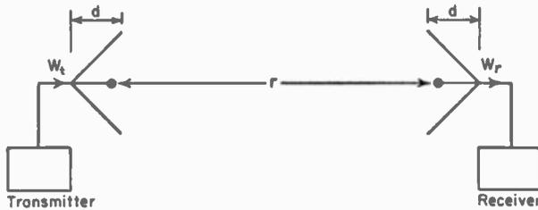
FIG. 15-13. Absolute gain measurements with two identical antennas.
