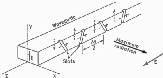
FIG. 13-5. Broadside array of slots in wave guide.
