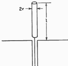
FIG. 10-19. Cylindrical stub antenna.
