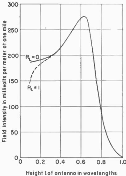
FIG. 11-35. Field intensity at the ground (zero elevation angle) at a distance of 1 mile from a vertical antenna with 1 kilowatt input as a function of its height  $l$ . Perfectly conducting ground is assumed. The solid curve is for an assumed loss resistance  $R_L = 0$  and the dashed curve for  $R_L = 1$  ohm.
