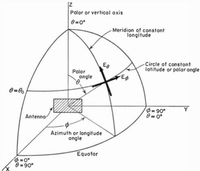
FIG. 15-1. Antenna and coordinates for pattern measurements.
