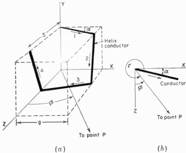
FIG. 7-23. Square helix used in calculating single-turn pattern.
