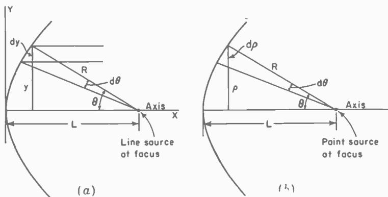
FIG. 12-19. Cross sections of cylindrical parabola (a) and of paraboloid of revolution (b).
