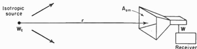
FIG. 3-8. Free-space transmission circuit consisting of isotropic source and receiving horn of maximum effective aperture  $A_{em}$ .
