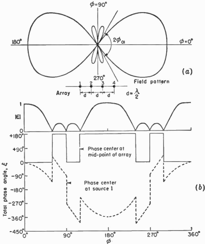
FIG. 4-22. (a) Field pattern of ordinary end-fire array of four isotropic point sources of same amplitude. Spacing is  $\frac{1}{2}$  wavelength, and the phase angle  $\delta = -\pi$ . (b) Field pattern in rectangular coordinates and phase patterns of same array with phase center at mid-point and at source 1. The reference direction for phase is at  $\phi = 0$ .
