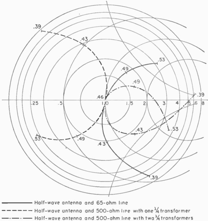
FIG. 14-43. Normalized impedance variation for cylindrical  $\frac{1}{2}$ -wavelength dipole antenna ( $L/D = 60$ ) fed directly by 65-ohm line (solid), by a 500-ohm line with one  $\frac{1}{4}$ -wavelength transformer (dashed), and by a 500-ohm line with two  $\frac{1}{4}$ -wavelength transformers in series (dash-dot).
