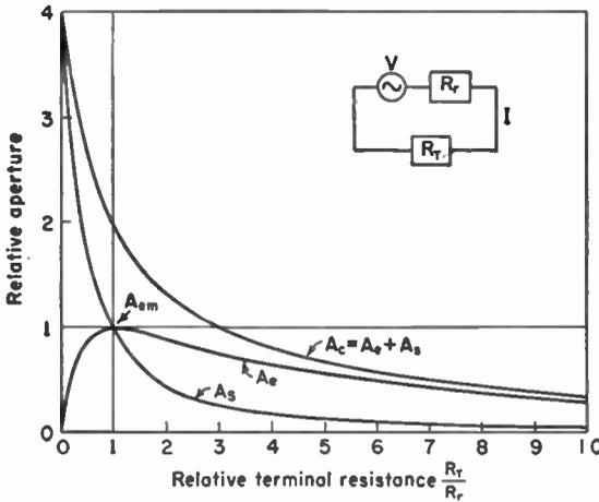
FIG. 3-3. Variation of effective aperture  $A_e$ , scattering aperture  $A_s$ , and collecting aperture  $A_c$  as a function of the relative terminal resistance  $R_r/R_r$  of a small antenna. It is assumed that  $R_L = X_A = X_T = 0$ .
