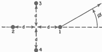
The spacing  $d$  between each source and the center point of the array is  $3\lambda/8$ . Sources 1 and 2 are in phase, and sources 3 and 4 in opposite phase with respect to 1 and 2.
