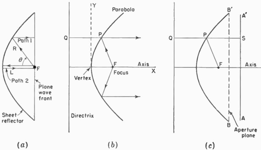
FIG. 12-15. Parabolic reflectors.
