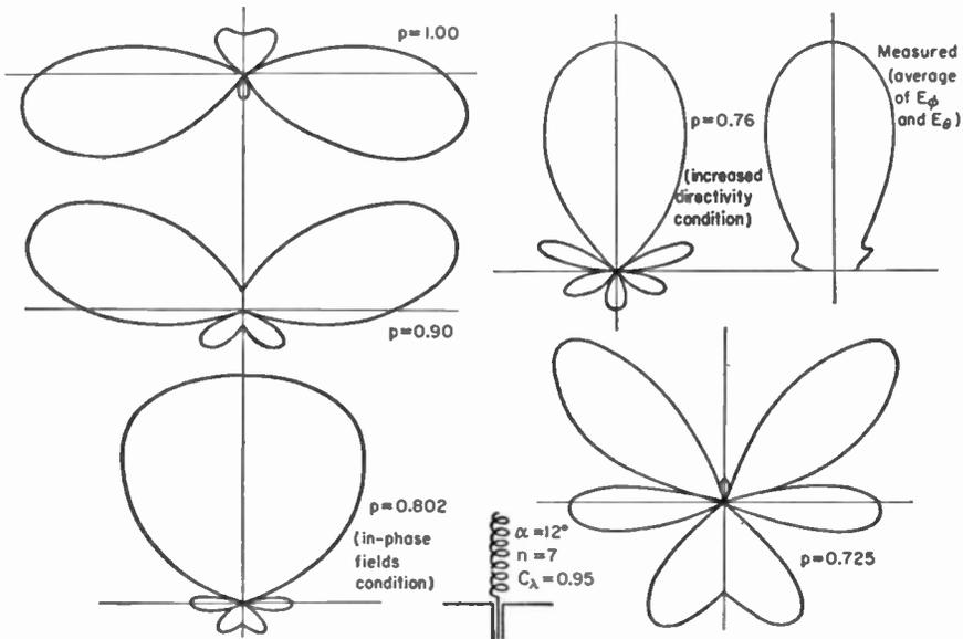
FIG. 7-20. Array factor patterns for  $12^\circ$ , 7-turn helix with  $C_\lambda = 0.95$ . Patterns are shown for  $p = 1, 0.9, 0.802$  (in-phase fields or ordinary end-fire condition),  $0.76$  (increased directivity), and  $0.725$ . A measured curve is also presented. All patterns are adjusted to the same maximum.
