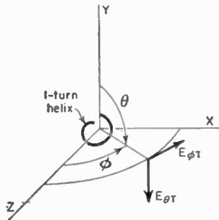
FIG. 7-24. Field components with relation to single-turn helix.
