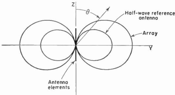
FIG. 11-5. Vertical-plane pattern of broadside array of two vertical in-phase  $\frac{1}{2}$ -wavelength elements spaced  $\frac{1}{2}$  wavelength. The pattern of a single vertical  $\frac{1}{2}$ -wavelength reference antenna with the same power input is shown for comparison.
