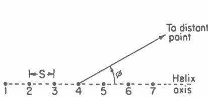
FIG. 7-16. Array of isotropic point sources, each source representing 1 turn of the helix.
