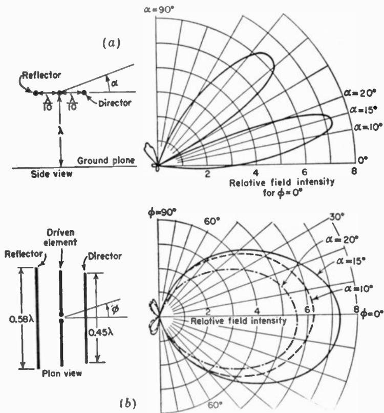
FIG. 11-40. Measured vertical plane pattern (a) and horizontal plane patterns (b) at three elevation angles for a three-element array located 1 wavelength above a large ground plane. (Patterns by D. C. Cleckner, Antenna Laboratory, The Ohio State University.)
