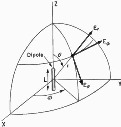
FIG. 5-2. Relation of dipole to coordinates.
