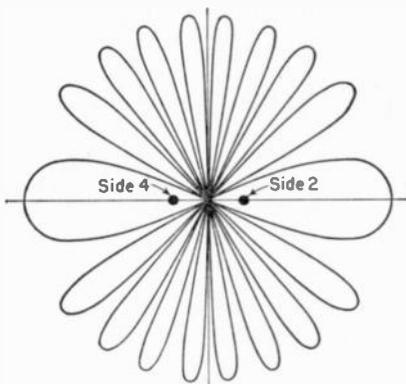
FIG. 6-15. Pattern of square loop with uniform, in-phase current. The loop is 4.44 wavelengths on a side. The pattern is in a plane normal to the plane of the loop and through the line  $AA'$  of Fig. 6-14.
