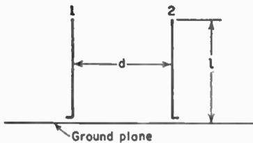
FIG. 10-13. Two coupled linear parallel stub antennas.
