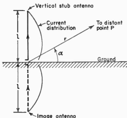
FIG. 11-33. Vertical stub antenna above a ground plane.
