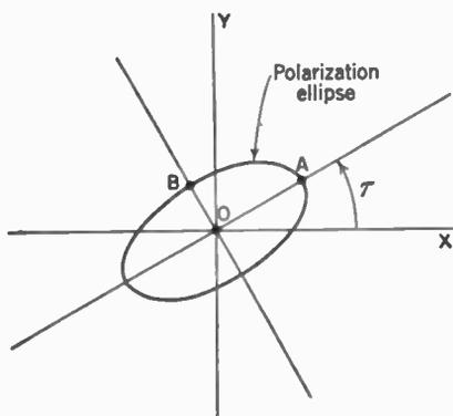
FIG. 15-22. Polarization ellipse.
