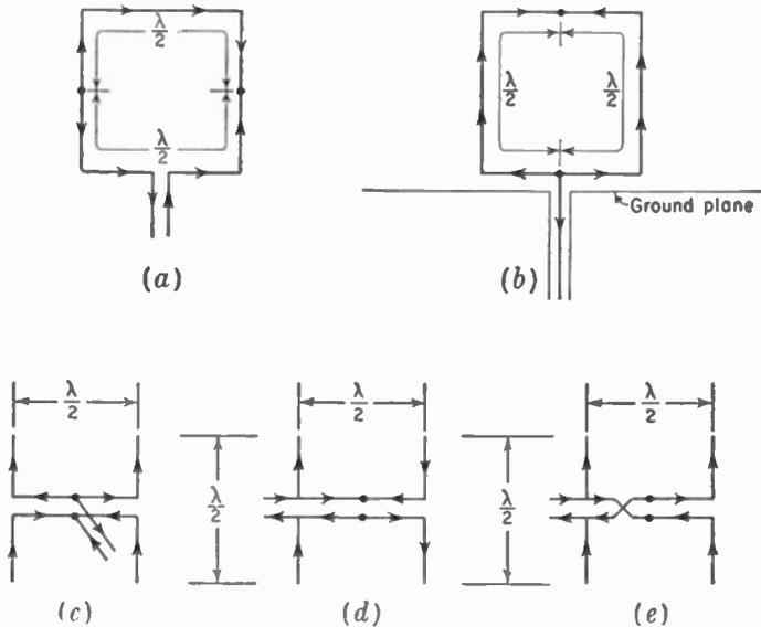
FIG. 14-24. (a) Loop with two-wire feed, (b) loop with one-wire feed, (c) center-fed broadside array of two  $\frac{1}{2}$ -wavelength dipoles, (d) end-fed end-fire array of two  $\frac{1}{2}$ -wavelength dipoles, and (e) end-fed broadside array of two  $\frac{1}{2}$ -wavelength dipoles. Arrows indicate instantaneous current directions, and dots indicate current minimum points.
