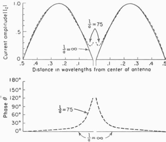
FIG. 9-7. Relative current amplitude and phase along a center-fed full-wavelength cylindrical antenna ( $2l = \lambda$ ) for total length-to-diameter ratios ( $l/a$ ) of 75 and infinity (after King and Harrison). Distance from the center of the antenna is expressed in wavelengths.
