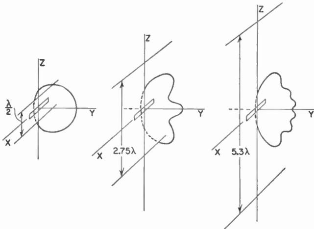
FIG. 13-10. Measured  $\phi$ -plane patterns of  $\frac{1}{4}$ -wavelength boxed-in slot antennas in finite sheets of three lengths  $L = 0.5, 2.75,$  and  $5.3$  wavelengths. The width of the slots is  $0.1$  wavelength. (After Dorne and Lazarus.)
