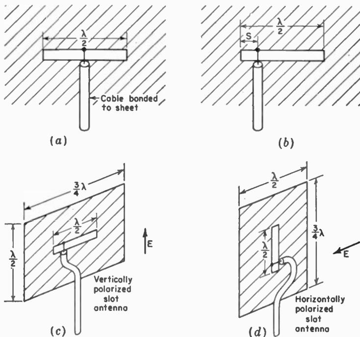
FIG. 13-2. Slot antennas fed by coaxial transmission lines.
