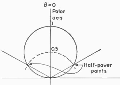
FIG. 2-6. Unidirectional cosine power pattern.
