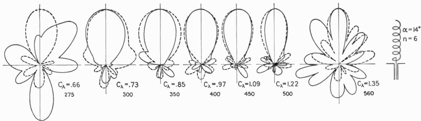
FIG. 7-33. Measured field patterns of  $14^\circ$ , 6-turn helix. Patterns are characteristic of the axial mode of radiation over a range of circumferences from about 0.73 to 1.22 wavelengths. Both the circumference and the frequency (in Mc) are indicated. The solid patterns are for the horizontally polarized field component ( $E_\phi$ ) and the dashed for the vertically polarized ( $E_\theta$ ). Both are adjusted to the same maximum.
