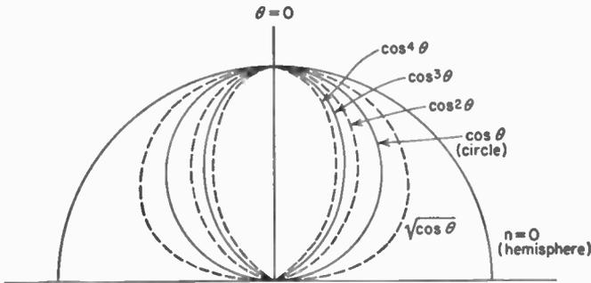
FIG. 2-12. Unidirectional  $\cos^n \theta$  power patterns for various values of  $n$ .
