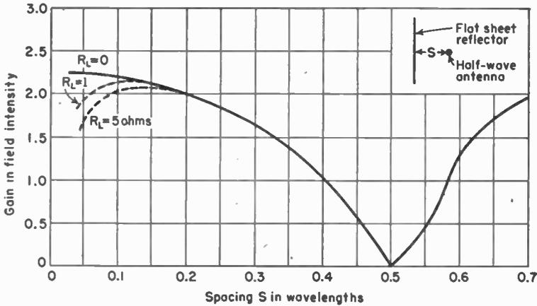
FIG. 12-4. Gain in field intensity of  $\frac{1}{2}$ -wavelength dipole antenna at distance  $S$  from flat sheet reflector. Gain is relative to  $\frac{1}{2}$ -wavelength dipole antenna in free space with the same power input. Gain is in direction  $\phi = 0$  and is shown for an assumed loss resistance  $R_L = 0, 1, \text{ and } 5 \text{ ohms}$ .
