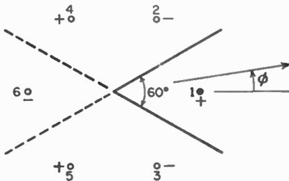
FIG. 12-8. 60° corner reflector with images used in analysis.
