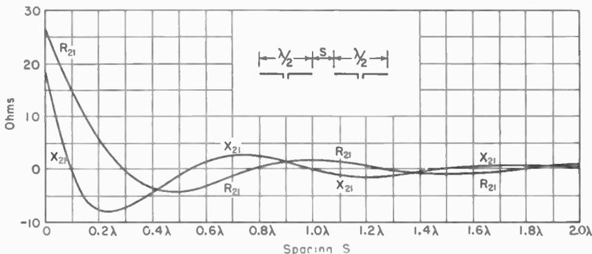
FIG. 10-14. Curves of mutual resistance ( $R_{21}$ ) and reactance ( $X_{21}$ ) of two parallel collinear infinitesimally thin  $\frac{1}{2}$ -wavelength antennas as a function of the spacing  $s$  between adjacent ends.
