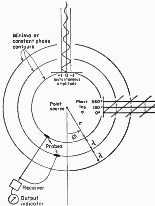
FIG. 2-20. Illustration for Example 1. Phase of  $E_\phi$  of point source radiating uniformly in  $\phi$  plane is a function of  $r$  but is independent of  $\phi$ . Phase lag  $\eta$  increases linearly with distance  $r$ .
