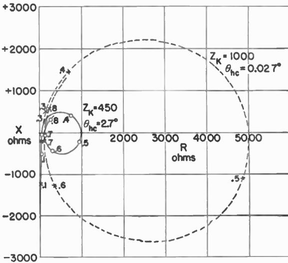
FIG. 8-12. Calculated input impedance of biconical antennas with  $2.7^\circ$  half-cone angle (solid curve) and with  $0.027^\circ$  half-cone angle (dashed curve). The resistance  $R$  and reactance  $X$  of the input impedance  $Z_i$  are represented as a function of the length  $l$  of one cone in wavelengths, the length being indicated in 0.1-wavelength intervals.
