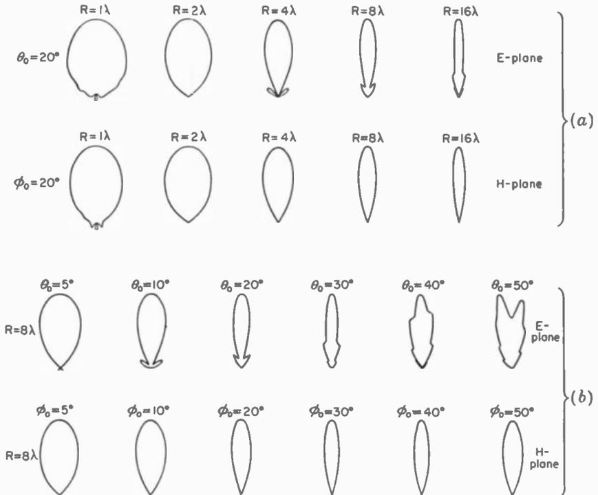
FIG. 13-21. Measured  $E$ - and  $H$ -plane patterns of rectangular horns as a function of flare angle and horn length. (After Rhodes.)
