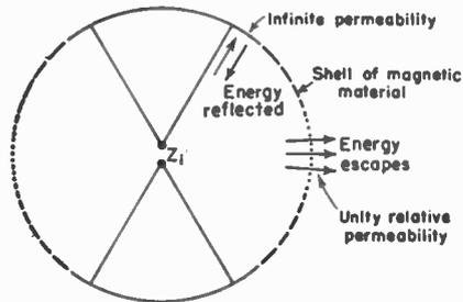
FIG. 8-8. Finite biconical antenna with boundary sphere replaced by a shell of magnetic material.
