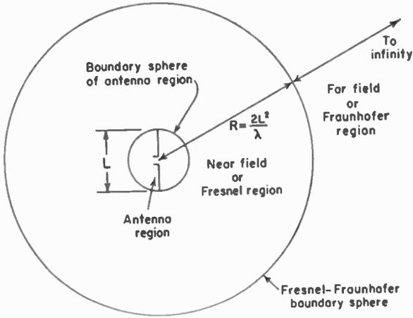
FIG. 1-7. Antenna region, Fresnel region, and Fraunhofer region.
