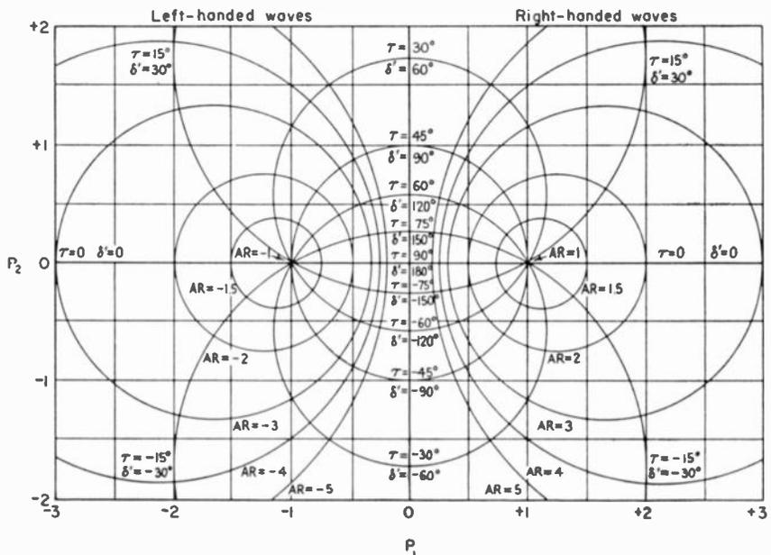
FIG. 15-33a. Rumsev and Tice type of wave polarization chart.
