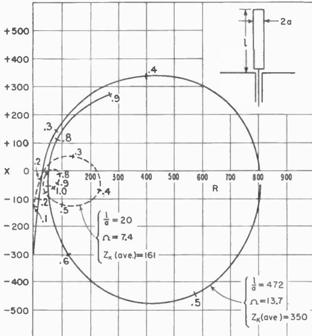
FIG. 9-11. Measured input impedance ( $R + jX$ ) in ohms of cylindrical stub antenna with ground plane for length-to-radius ratio ( $l/a$ ) of 20 and 472.
