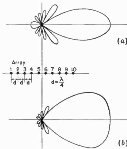
FIG. 4-24. Field patterns of end-fire arrays of 10 isotropic point sources of equal amplitude spaced  $\frac{1}{4}$  wavelength apart. The pattern at (a) has the phase adjusted for increased directivity ( $\delta = -0.6\pi$ ), while the pattern at (b) has the phasing of an ordinary end-fire array ( $\delta = -0.5\pi$ ).
