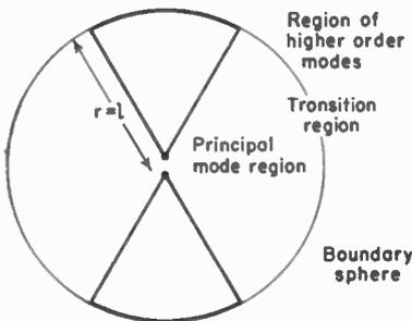
FIG. 8-7. Schelkunoff's finite biconical antenna and boundary sphere.
