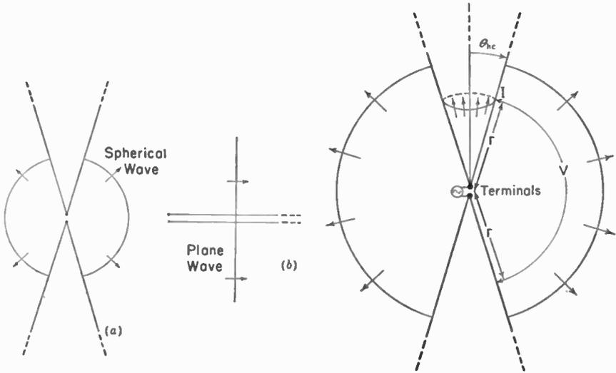
FIG. 8-1. An infinite biconical antenna (a) is analogous to an infinite uniform transmission line (b).
