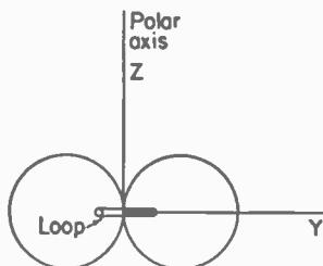
FIG. 6-6. Far-field pattern for a small loop.
