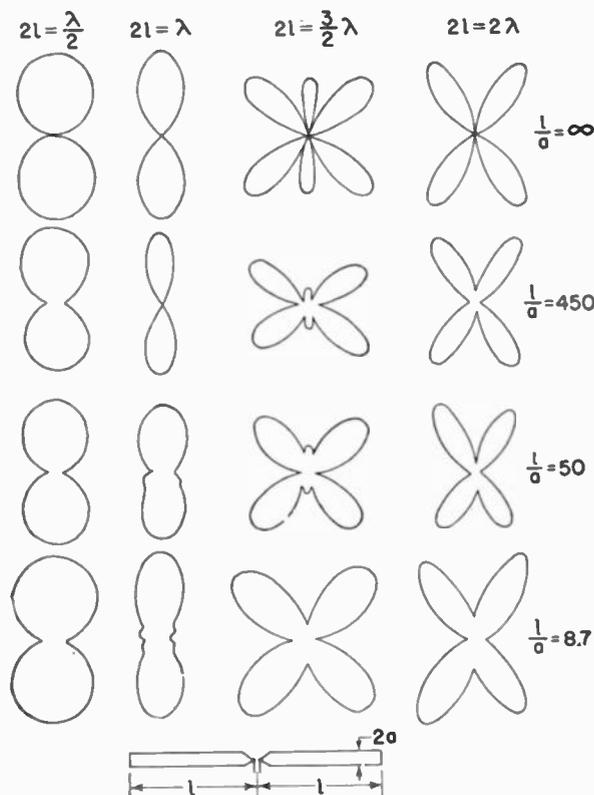
FIG. 9-13. Field patterns of cylindrical center-fed linear antennas of total length  $2l$  as a function of the total length-to-diameter ratio ( $l/a$ ) and also as a function of the total length ( $2l$ ) in wavelengths.
