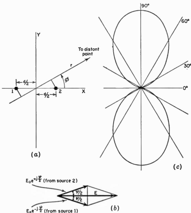
FIG. 4-1. (a) Relation to coordinate system of two isotropic point sources separated by a distance  $d$ . (b) Vector addition of the fields from two isotropic points sources of equal amplitude and same phase located as in (a). (c) Field pattern of two isotropic point sources of equal amplitude and same phase located as in (a) for the case where the separation  $d$  is  $\frac{1}{2}$  wavelength.
