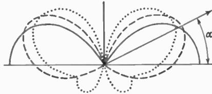
FIG. 14-30. Vertical-plane patterns of  $\frac{1}{4}$ -wavelength stub antenna on infinite ground plane (solid), and on finite ground planes several wavelengths in diameter (dashed) and about 1 wavelength in diameter (dotted).
