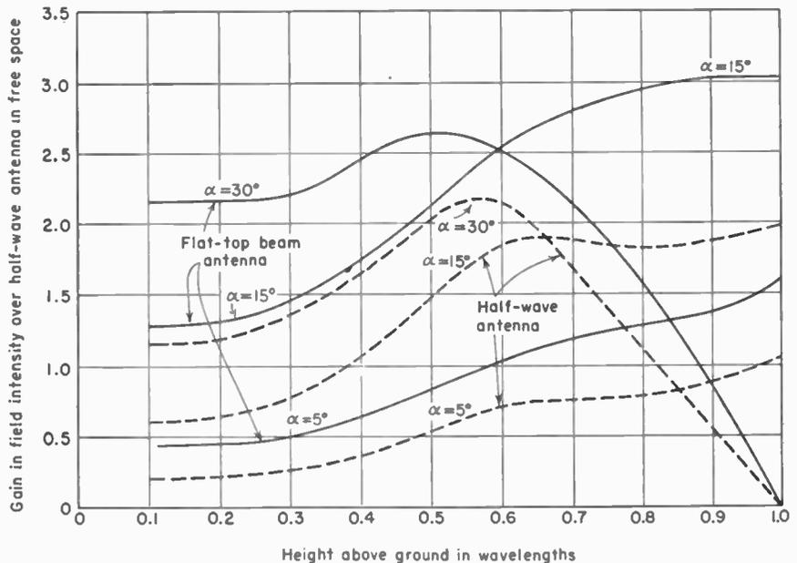
FIG. 11-27. Gain in field intensity of two-element flat-top beam antenna with  $\frac{1}{2}$  wavelength spacing (solid curves) and of a single  $\frac{1}{2}$ -wavelength antenna (dashed curves) as a function of the height above a perfectly conducting ground. Gains are relative to a single  $\frac{1}{2}$ -wavelength antenna in free space with the same power input. Curves are given for elevation angles  $\alpha = 5^\circ, 15^\circ,$  and  $30^\circ$ .
