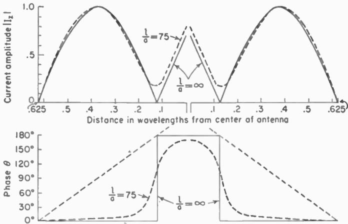
FIG. 9-8. Relative current amplitude and phase along a center-fed  $1\frac{1}{4}$ -wavelength cylindrical antenna ( $2l = 1\frac{1}{4}\lambda$ ) for total length-to-diameter ratios ( $l/a$ ) of 75 and infinity (after King and Harrison). Distance from the center of the antenna is expressed in wavelengths.
