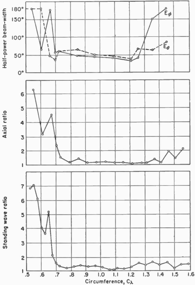
FIG. 7-34. Summary of measured performance of  $14^\circ$ , 6-turn helix. The curves show the half-power beam width for both field components, the axial ratio in the direction of the helix axis, and the SWR on a 53-ohm line as a function of the circumference in free-space wavelengths ( $C_\lambda$ ).
