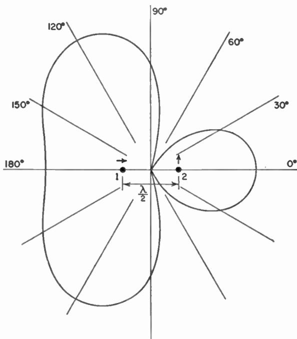
FIG. 4-4. Relative field pattern of two isotropic point sources of same amplitude and in phase quadrature for a spacing of  $\frac{1}{2}$  wavelength. The source to the right leads that to the left by  $90^\circ$ .
