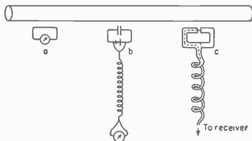
FIG. 15-17. Sampling loops for current distribution measurements.
