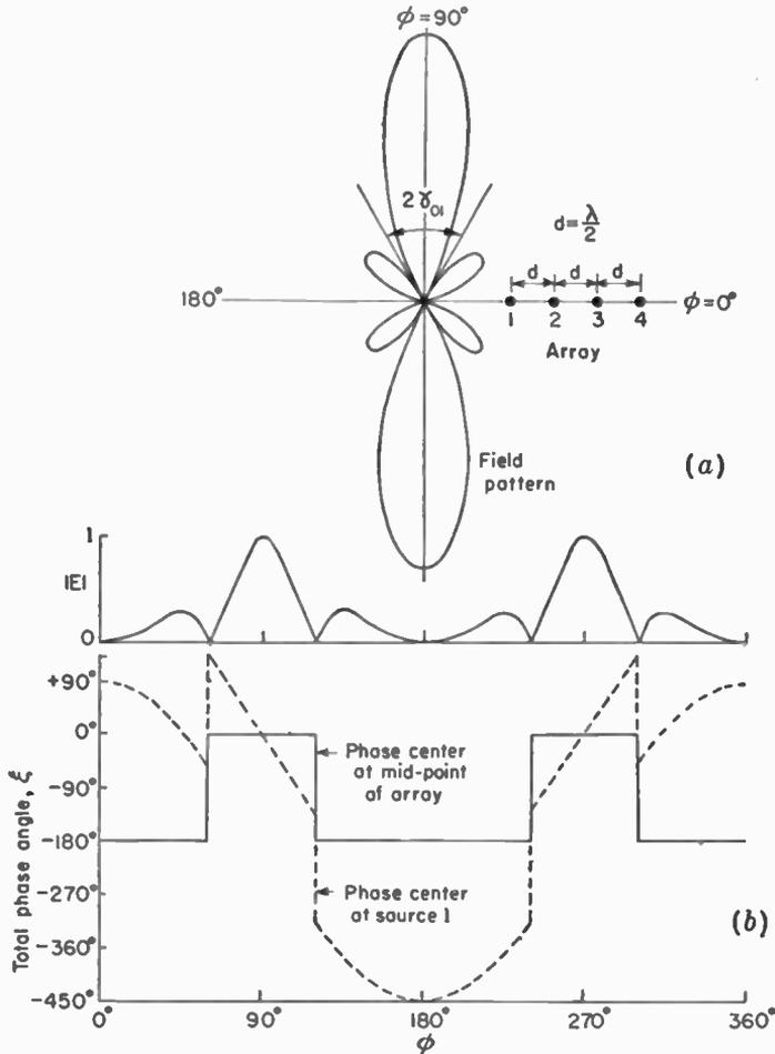
FIG. 4-21. (a) Field pattern of broadside array of four isotropic point sources of same amplitude and phase. The spacing between sources in  $\frac{1}{2}$  wavelength. (b) Field pattern in rectangular coordinates and phase patterns of same array with phase center at midpoint and at source 1. The reference direction for phase is taken at  $\phi = 90^\circ$ .
